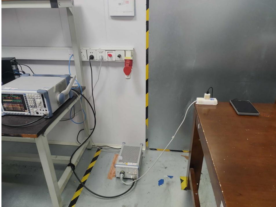
Conducted emissions at AC power line (150kHz-30MHz)
