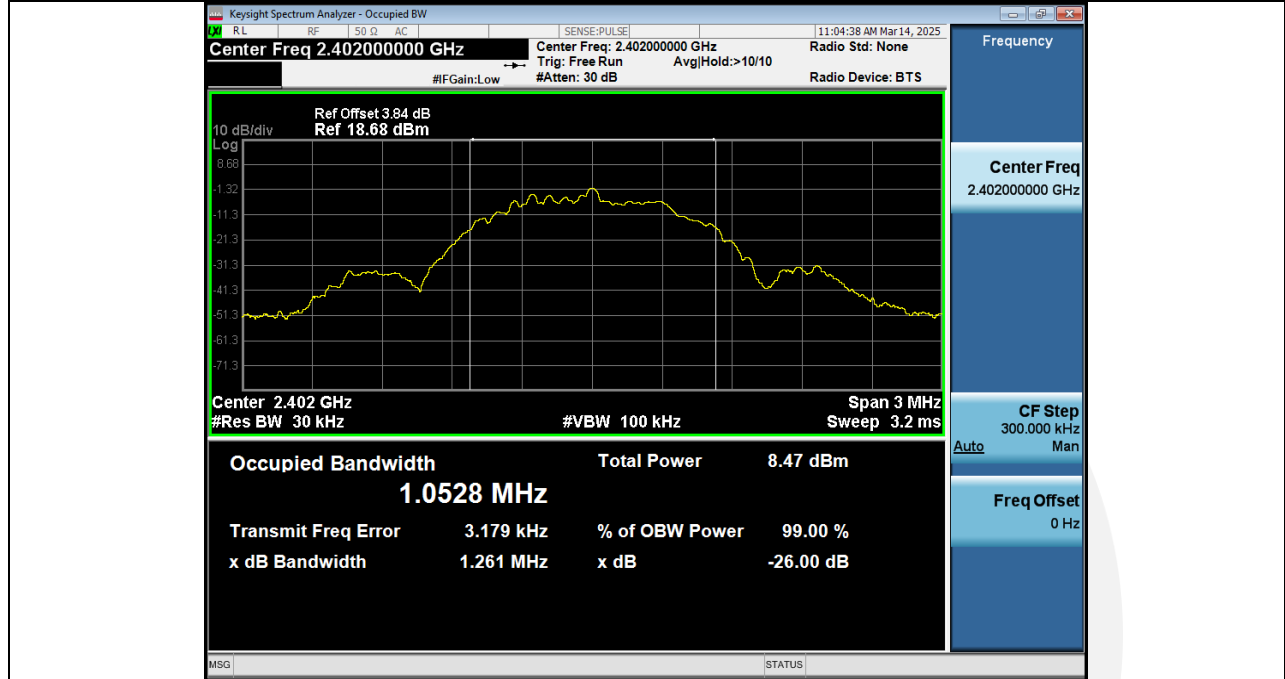
99% Occupied Bandwidth NVNT ANT1 1Mbps 2402
