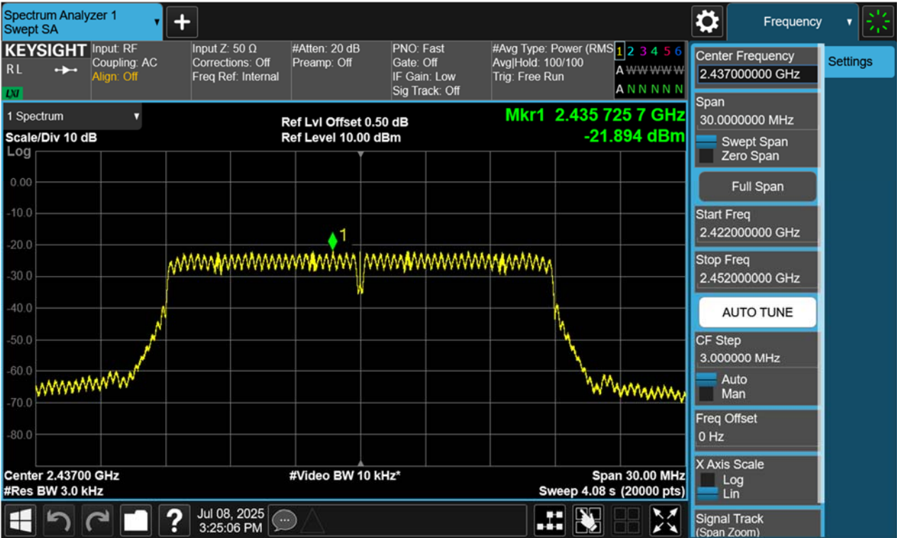
Figure 17: Power Spectral Density, 802.11n(HT20), 2437MHz
