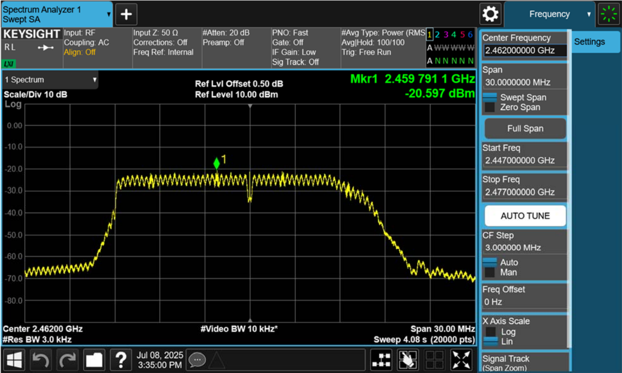
Figure 18: Power Spectral Density, 802.11n(HT20), 2462MHz
