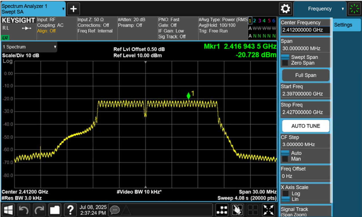
Figure 13: Power Spectral Density, 802.11g, 2412MHz
