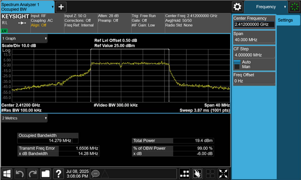
Figure 8: 6dB Bandwidth, 802.11n(HT20), 2437MHz
