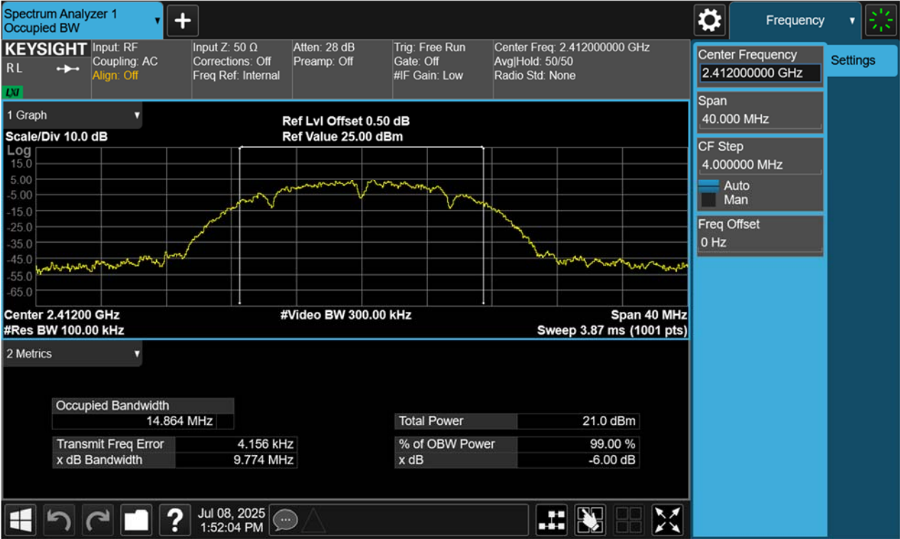
Figure 2: 6dB Bandwidth, 802.11b, 2437MHz
