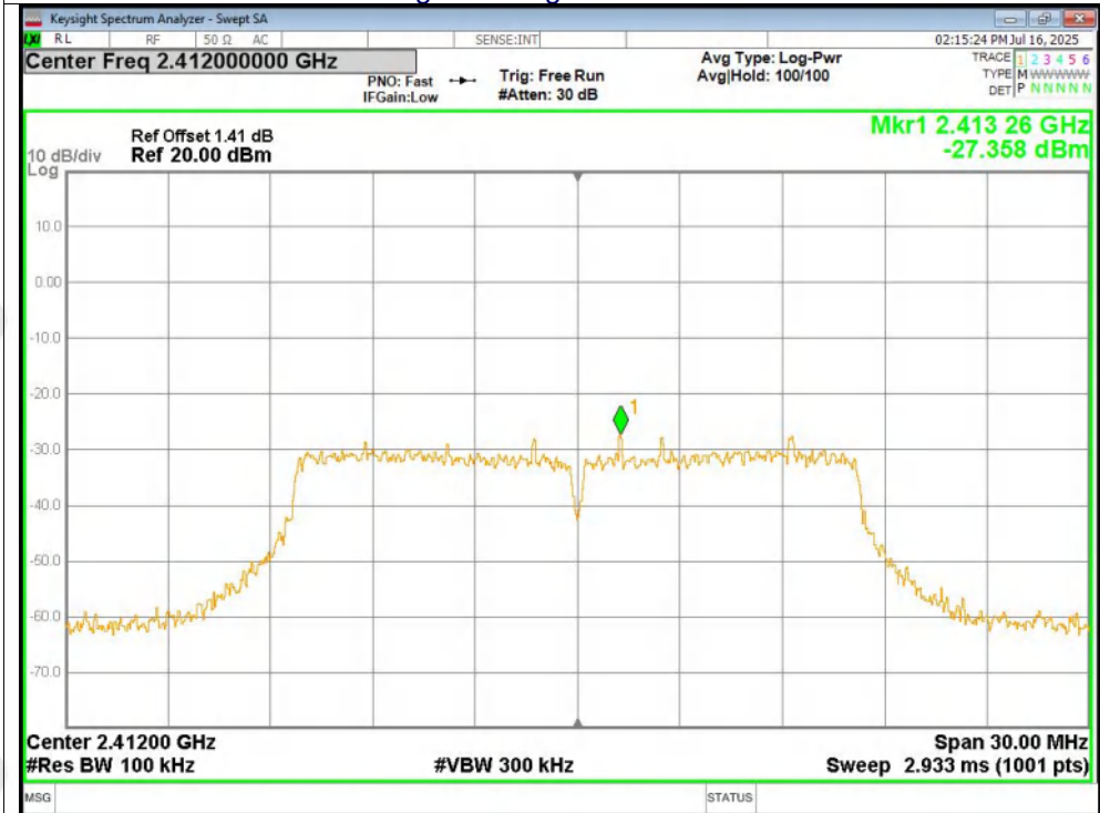
Band Edge NVNT g 2412MHz Ant1 Emission
