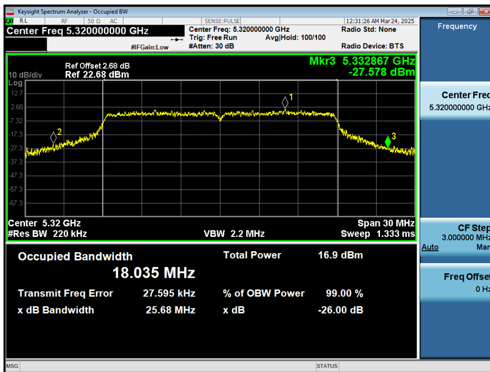
-26dB Bandwidth NVNT ac20 5320MHz Ant1
