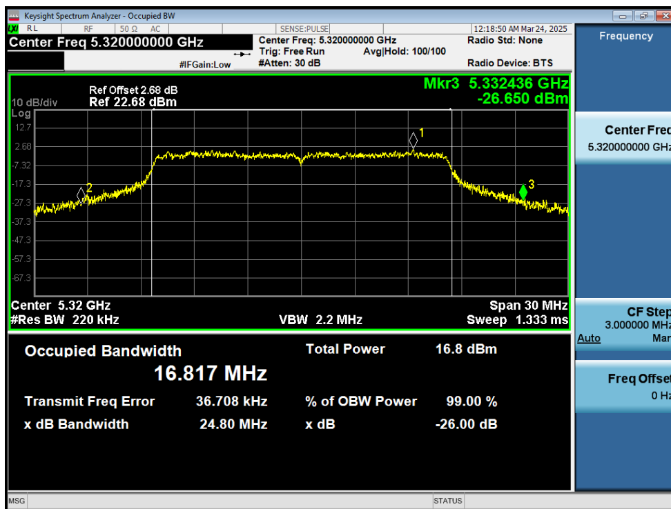
-26dB Bandwidth NVNT a 5320MHz Ant1
