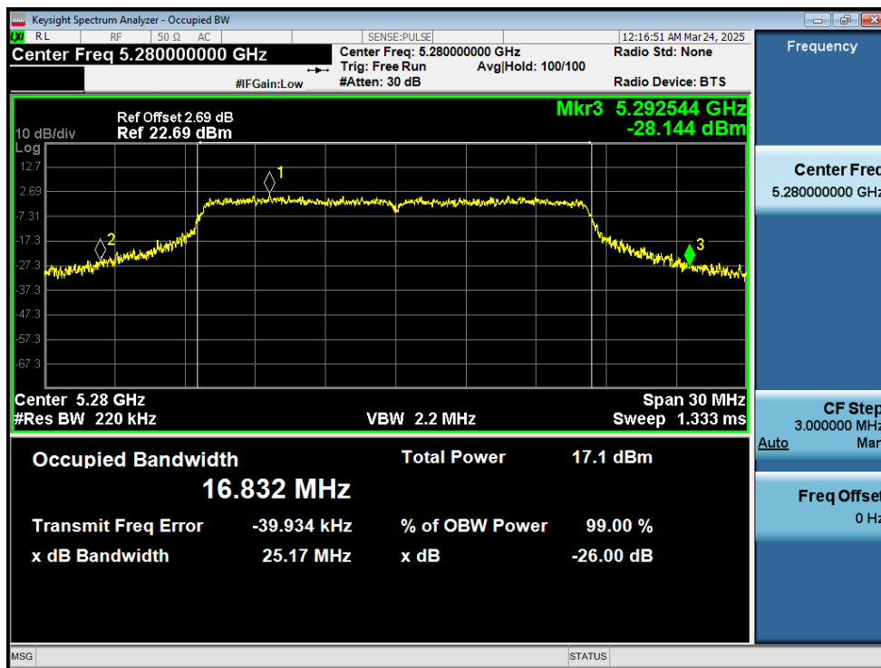
-26dB Bandwidth NVNT a 5280MHz Ant1
