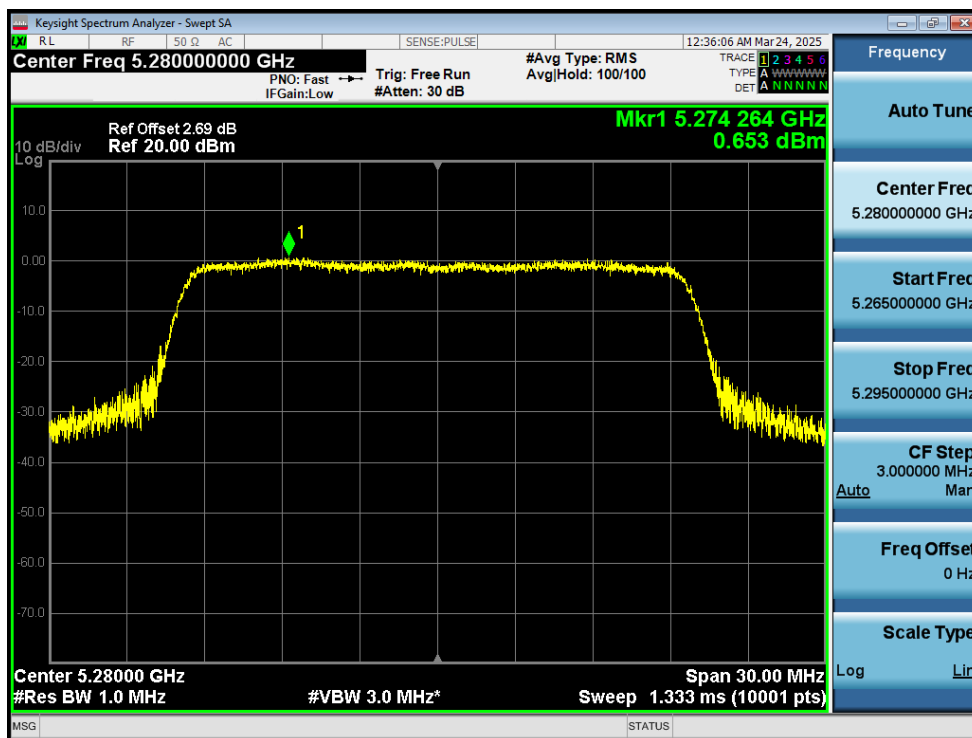
PSD NVNT ax20 5280MHz Ant1
