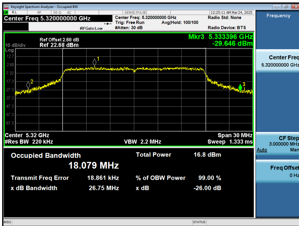
-26dB Bandwidth NVNT n20 5320MHz Ant1
