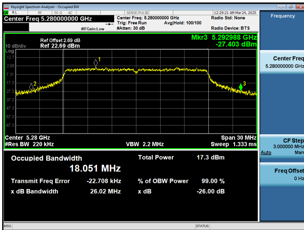
-26dB Bandwidth NVNT ac20 5280MHz Ant1
