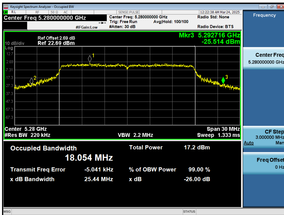
-26dB Bandwidth NVNT n20 5280MHz Ant1
