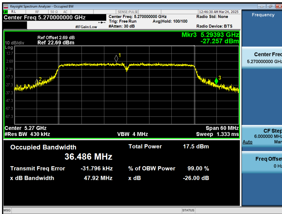
-26dB Bandwidth NVNT ac40 5270MHz Ant1
