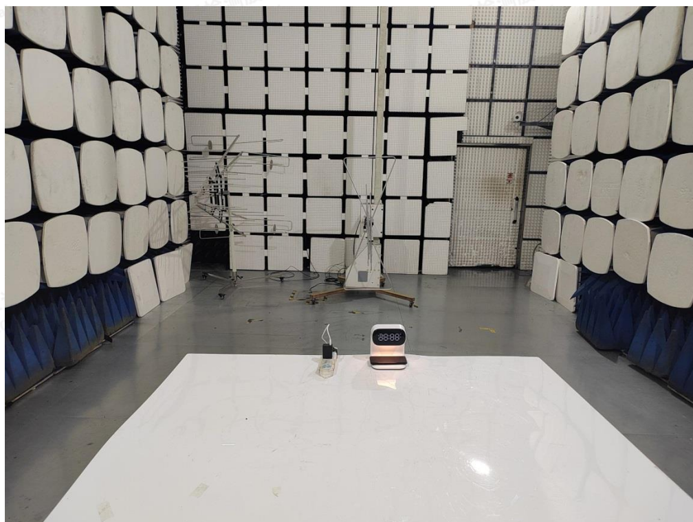
Radiated Emission below 1GHz-AC adapter charge mode
