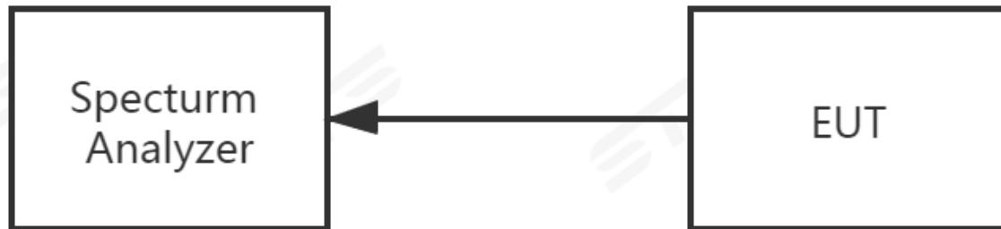
The EUT is connected to the Spectrum Analyzer; the RF load attached to the EUT antenna terminal is 50Ohm; the path loss as the factor is calibrated to correct the reading.
