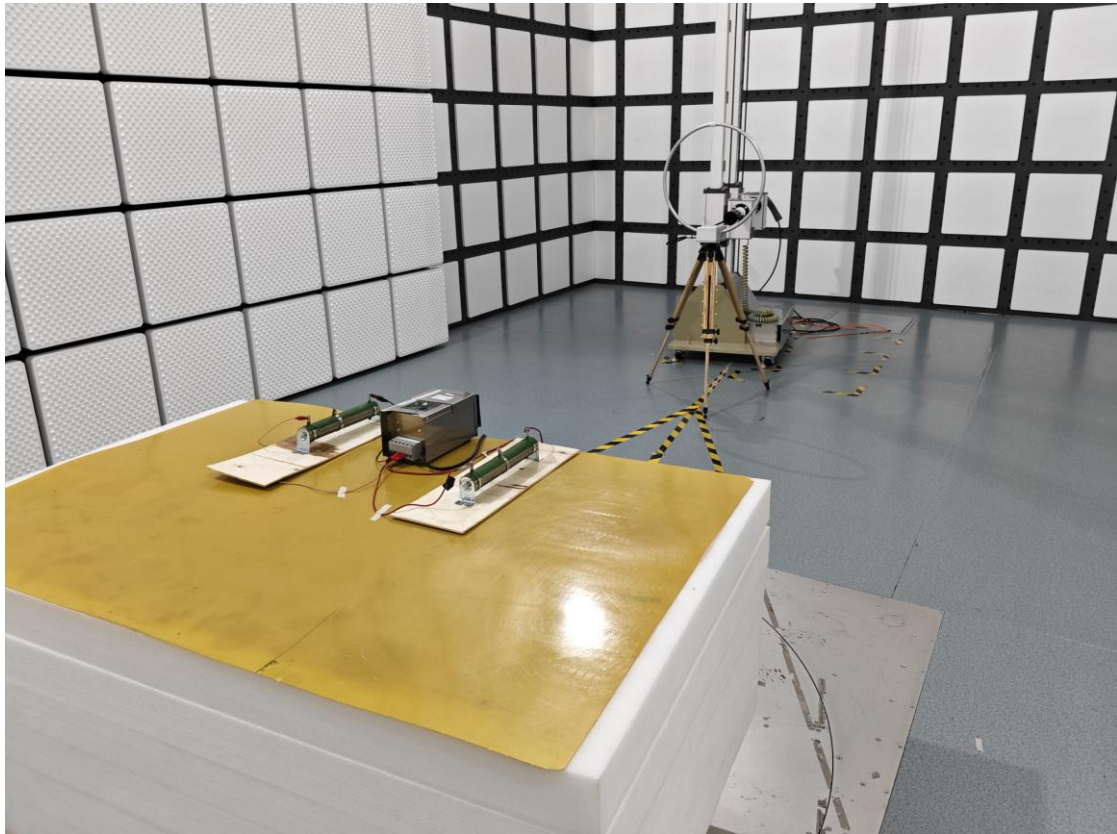
Radiated Spurious Emissions Test View (9kHz-30MHz)
