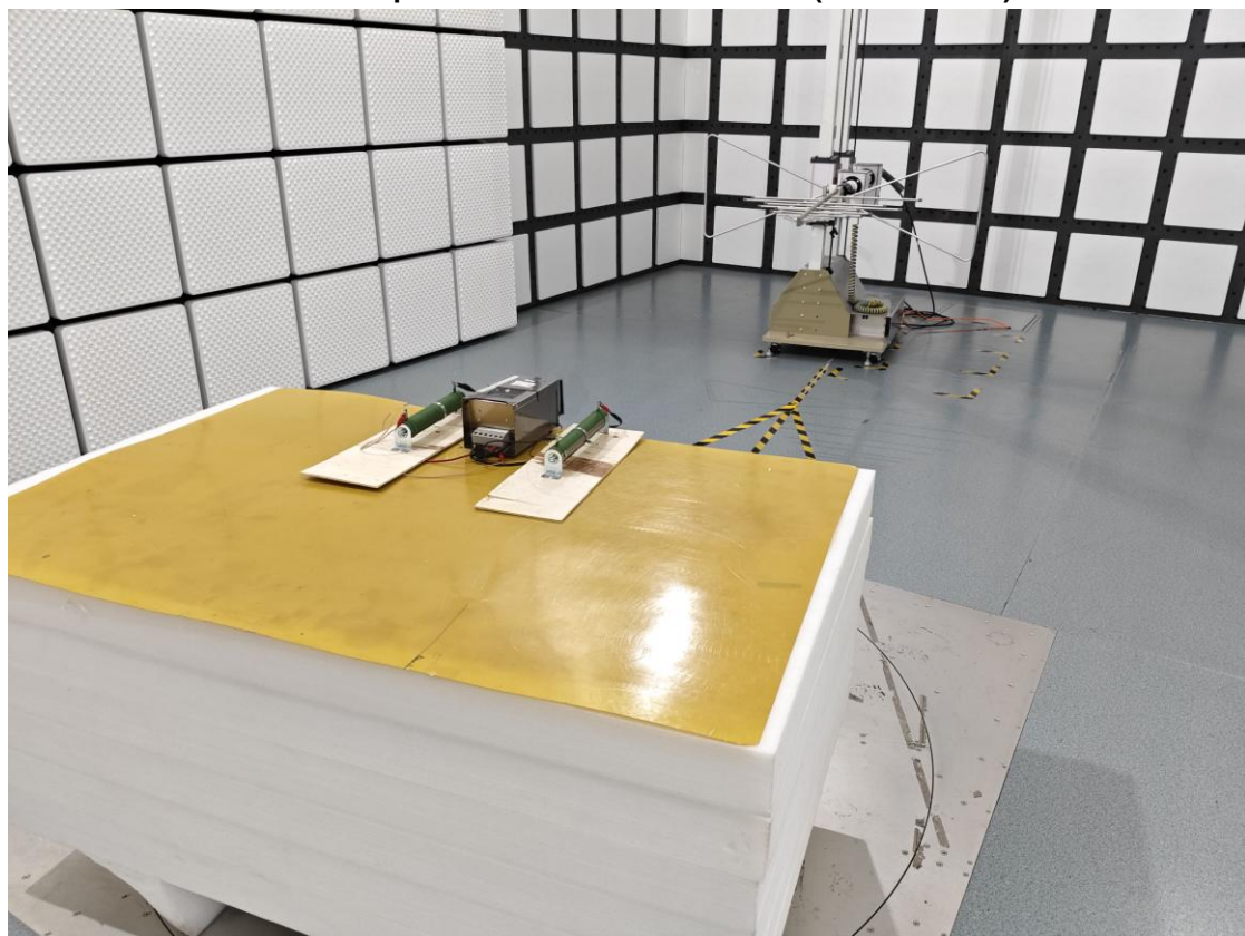
Radiated Spurious Emissions Test View (30MHz-1GHz)
