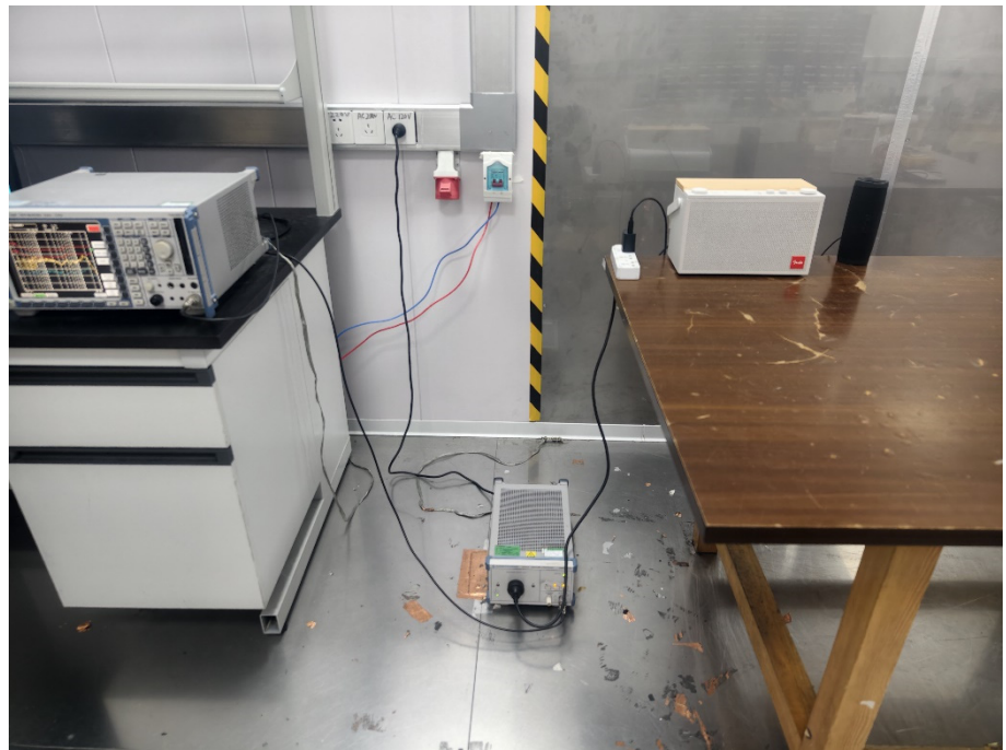
Conducted Emission Test Setup
