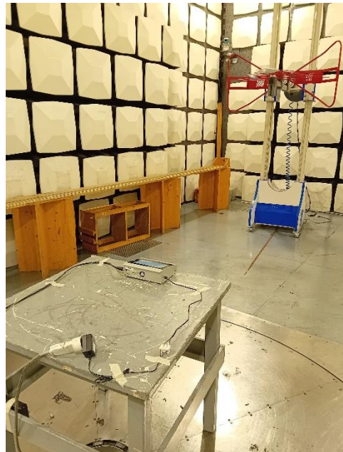
Test Setup – AC Power Line Conducted Emissions
