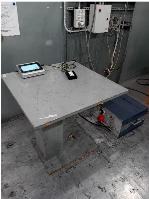
Test Setup – AC Power Line Conducted Emissions
