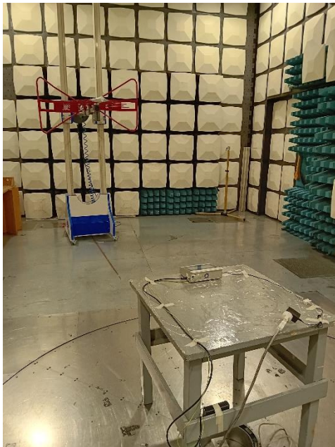
Test Setup – AC Power Line Conducted Emissions
