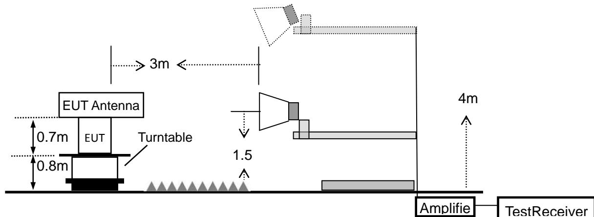
Note: the antenna of the EUT was located at a height of 1.5 m above the floor.
