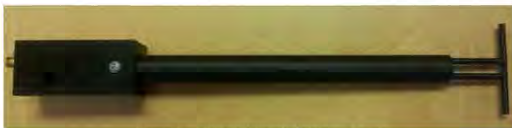
Figure 1 – MVG COMOSAR Validation Dipole
