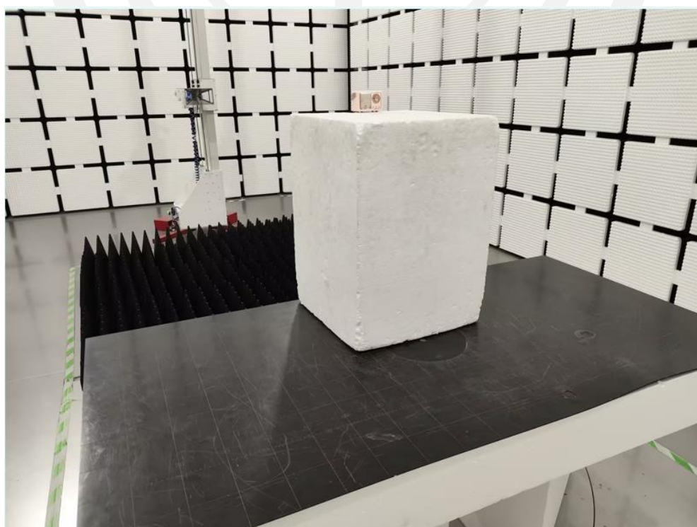
Spurious Radiation Emissions Test (>1G)
