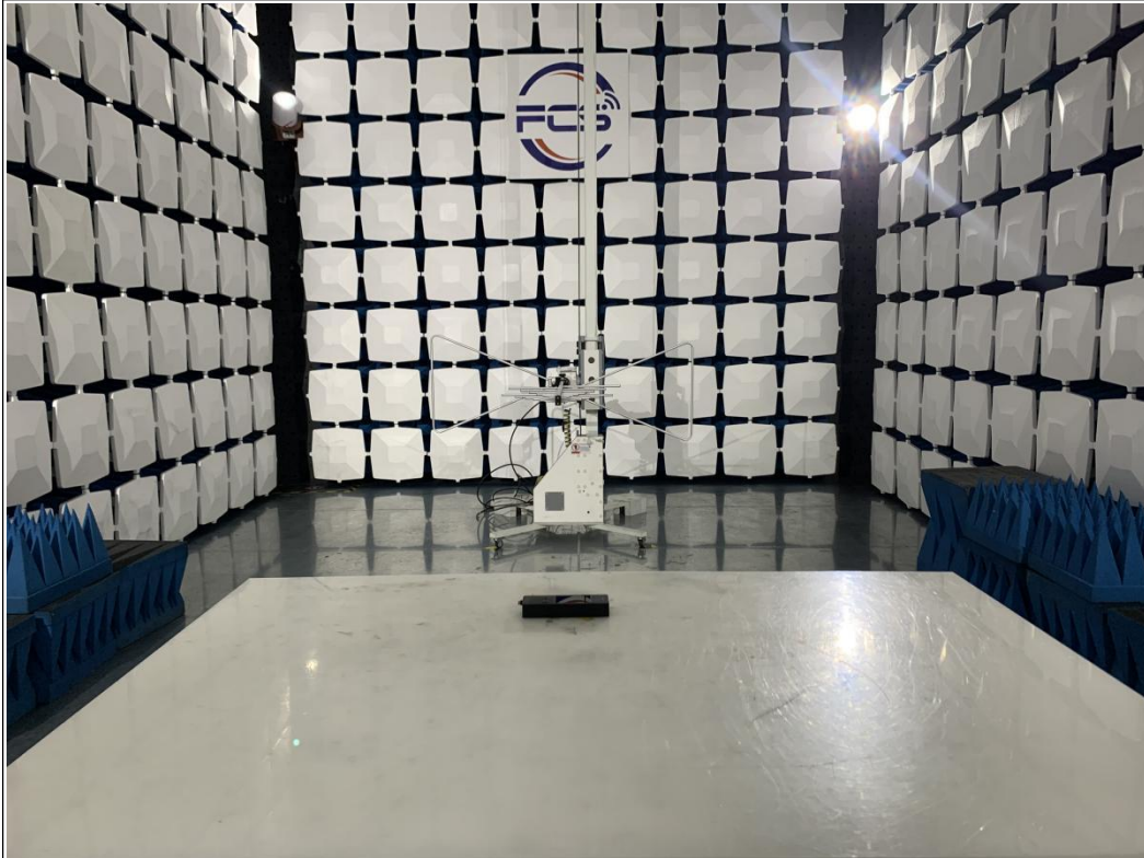
Above 1GHz for radiated emission test setup
