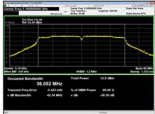
(802.11 n40) 26dB Bandwidth plot on channel 46
