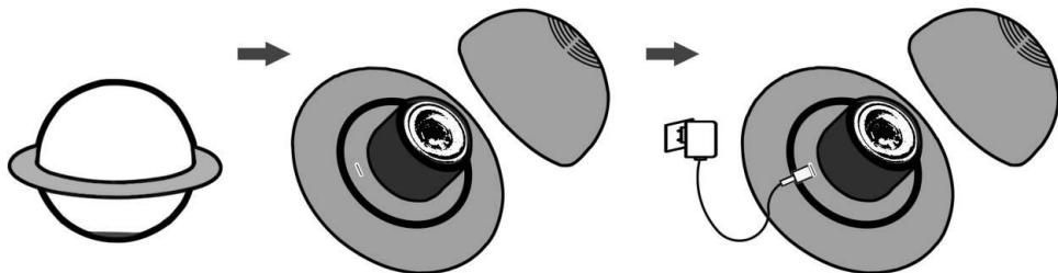
If the speaker is power off, and just open the top hemisphere and charge it by your type-c cable with a 5V charger. It will take around 3 hours fully charging.
