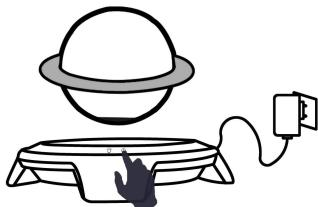
Touch the switch on the right for 2 seconds and the speaker emits a warning tone, and the Saturn ring lights on. Touch the switch on the right for 2 seconds, and the speaker emits a warning tone, and the speaker is off and its Saturn ring lights is also off.
