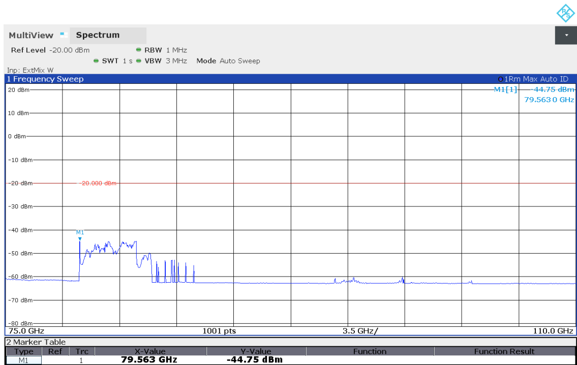
Plots No. 18: Radiated Emission, 75 GHz to 110 GHz, Horizontal / Vertical Polarization
