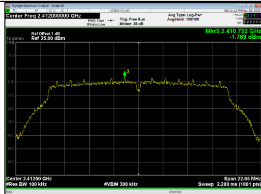
In-Band Reference Level IEEE 802.11g_Channel 1_20MHz_Antenna 0
