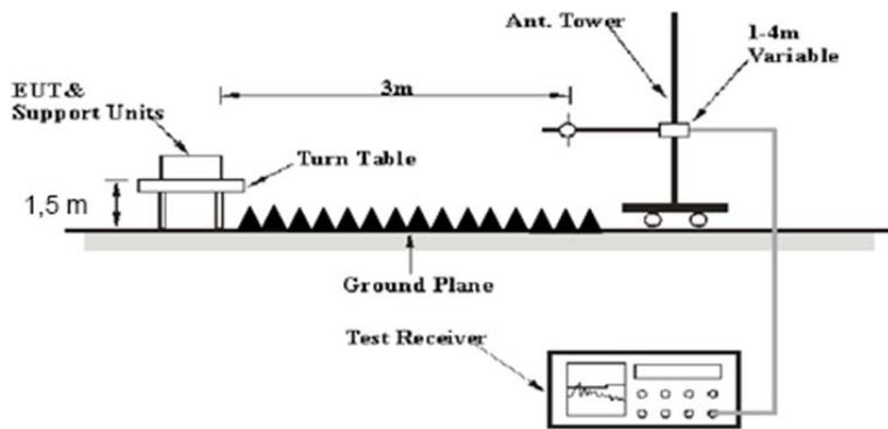
The radiated emissions were performed in the 3 meters distance, using the setup accordance with the ANSI C63.10-2020. The specification used was the FCC 15.209, and FCC 15.247 limits.
