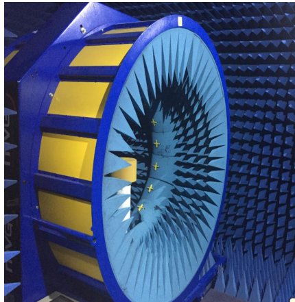
图示1/Figure 1: 3D暗室。3D Anechoic Chamber
