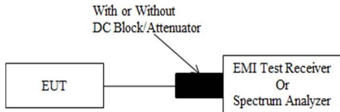
A short RF cable with low cable loss connected to the EUT antenna port, the insert loss of this RF cable/attenuator was offset into the setting of test equipment.
