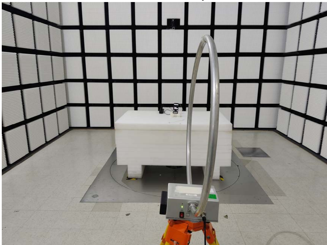
Radiated Emission 9 kHz-30 MHz Perpendicular View
