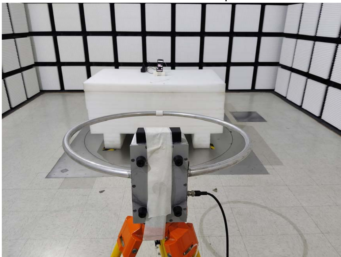
Radiated Emission 9 kHz-30 MHz Ground-parallel View
