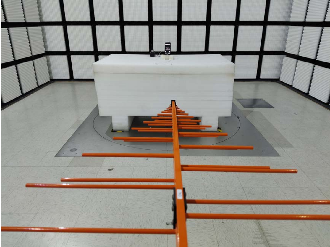
Radiated Emission 30 MHz-1 GHz View
