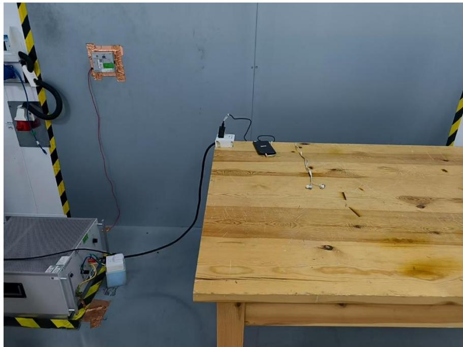
**Set-up for Radiated Emission (RE), Below 1GHz**
