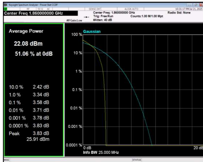
Band2 QPSK BW=20MHz Channel=18900 RB Size=1 Position=#0
