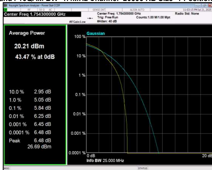
Band4 16QAM BW=10MHz Channel=20000 RB Size=1 Position=#0
