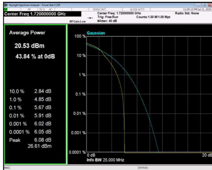
Band4 16QAM BW=20MHz Channel=20175 RB Size=1 Position=#0
