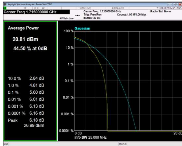
Band4 16QAM BW=10MHz Channel=20175 RB Size=1 Position=#0
