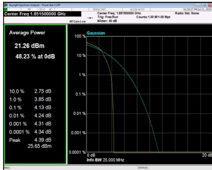
Band2 16QAM BW=3MHz Channel=18900 RB Size=1 Position=#0
