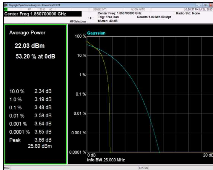
Band2 QPSK BW=1.4MHz Channel=18900 RB Size=1 Position=#0
