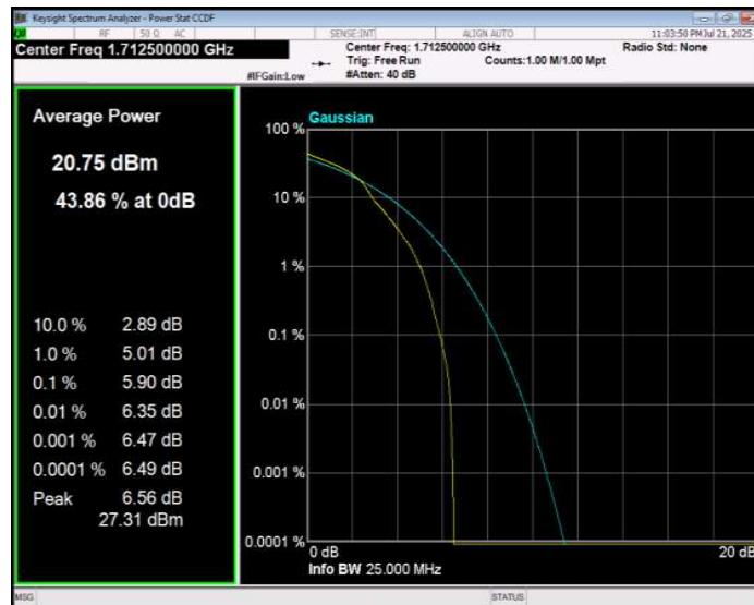
Band4 16QAM BW=5MHz Channel=20175 RB Size=1 Position=#0
