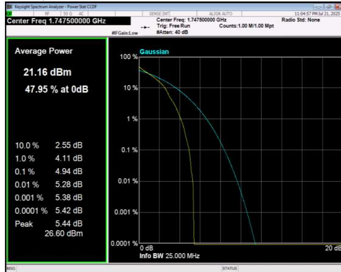
Band4 QPSK BW=20MHz Channel=20050 RB Size=1 Position=#0
