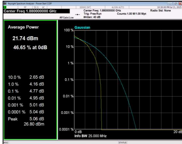
Band2 QPSK BW=5MHz Channel=19175 RB Size=1 Position=#0
