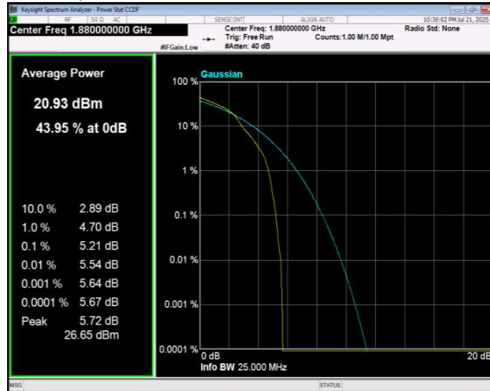
Band2 16QAM BW=5MHz Channel=19175 RB Size=1 Position=#0
