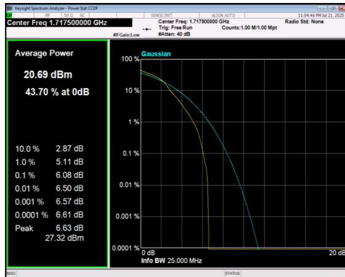
Band4 16QAM BW=15MHz Channel=20175 RB Size=1 Position=#0
