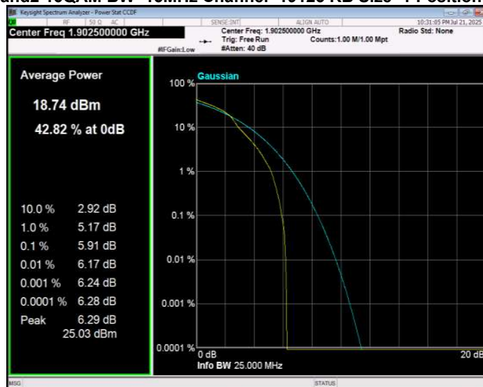
Band2 16QAM BW=20MHz Channel=18700 RB Size=1 Position=#0
