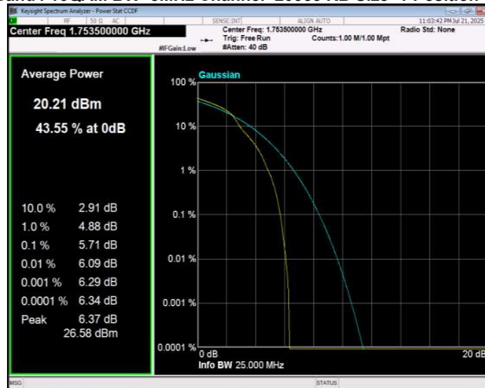
Band4 16QAM BW=5MHz Channel=19975 RB Size=1 Position=#0
