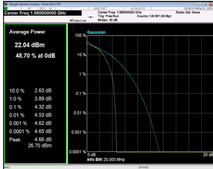
Band2 QPSK BW=3MHz Channel=19185 RB Size=1 Position=#0
