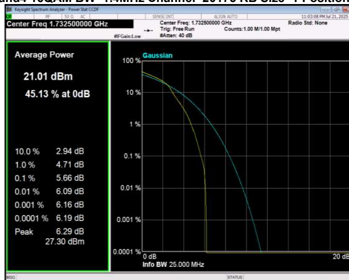
Band4 16QAM BW=1.4MHz Channel=20393 RB Size=1 Position=#0
