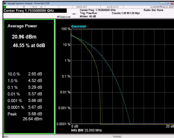
Band4 QPSK BW=5MHz Channel=19975 RB Size=1 Position=#0
