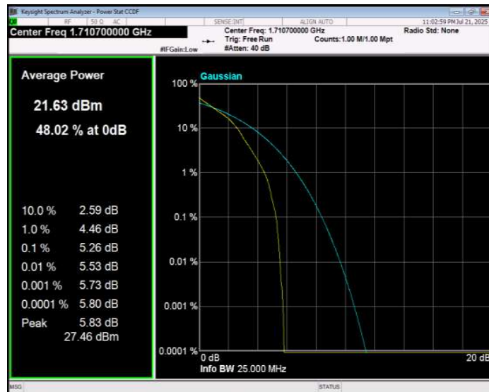
Band4 QPSK BW=1.4MHz Channel=20175 RB Size=1 Position=#0
