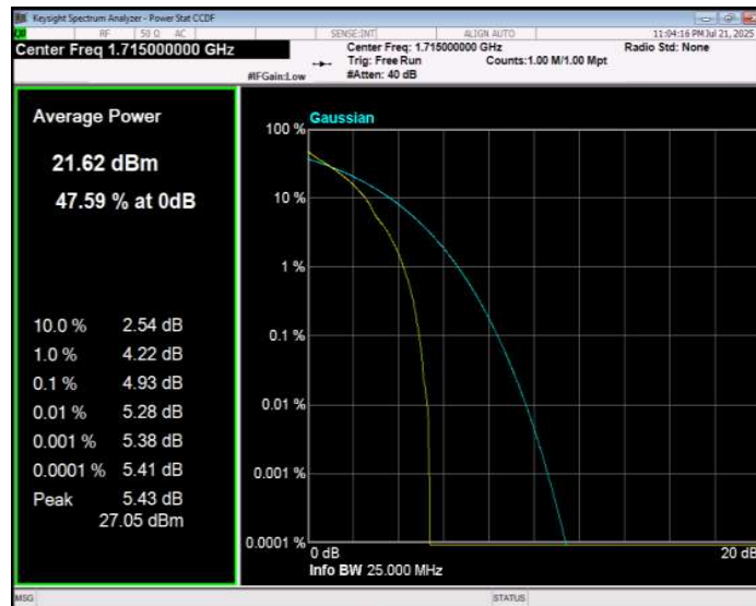
Band4 QPSK BW=10MHz Channel=20175 RB Size=1 Position=#0
