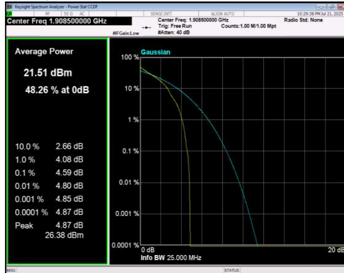
Band2 QPSK BW=5MHz Channel=18625 RB Size=1 Position=#0
