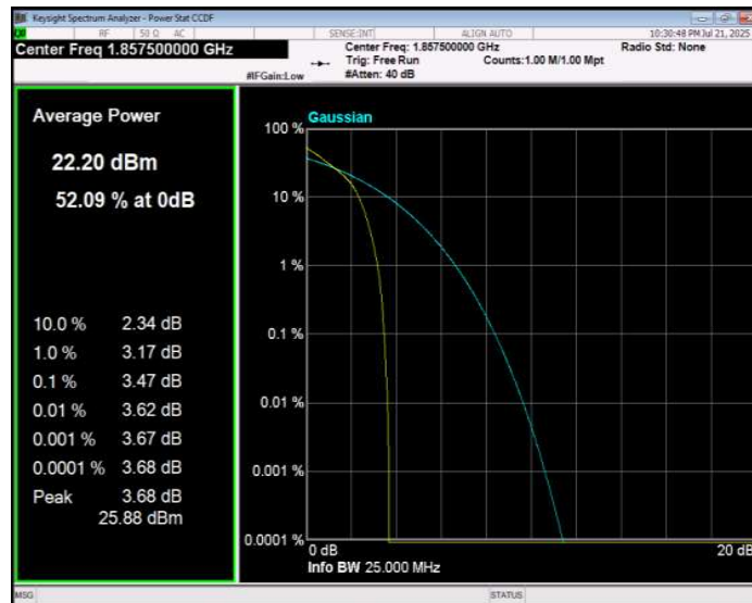
Band2 QPSK BW=15MHz Channel=18900 RB Size=1 Position=#0
