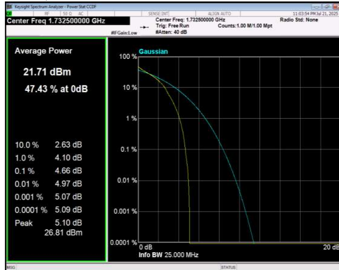
Band4 QPSK BW=5MHz Channel=20375 RB Size=1 Position=#0
