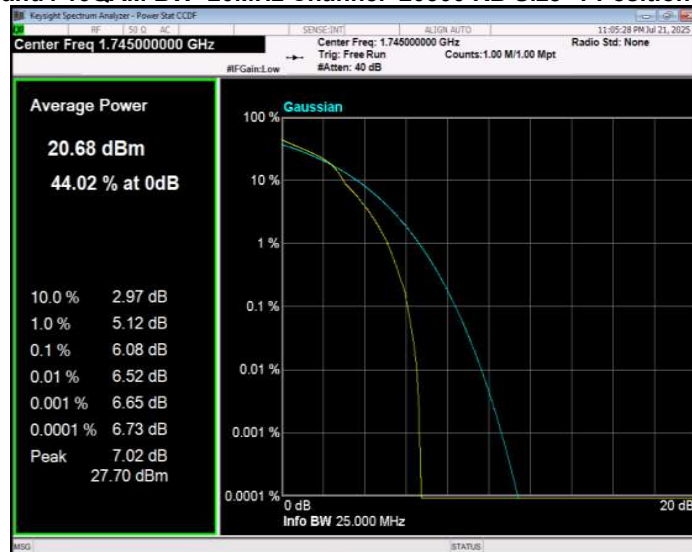
Band4 16QAM BW=3MHz Channel=19965 RB Size=1 Position=#0
