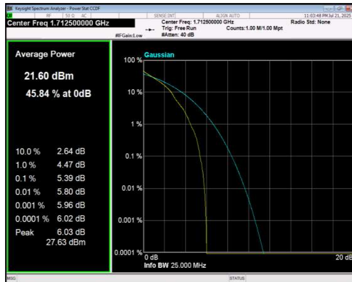
Band4 QPSK BW=5MHz Channel=20175 RB Size=1 Position=#0
