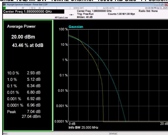
Band2 16QAM BW=15MHz Channel=19125 RB Size=1 Position=#0
