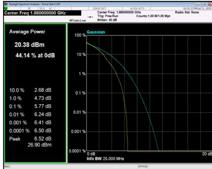
Band2 QPSK BW=20MHz Channel=19100 RB Size=1 Position=#0
