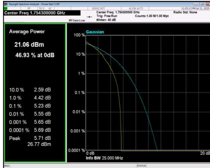
Band4 QPSK BW=10MHz Channel=20000 RB Size=1 Position=#0
