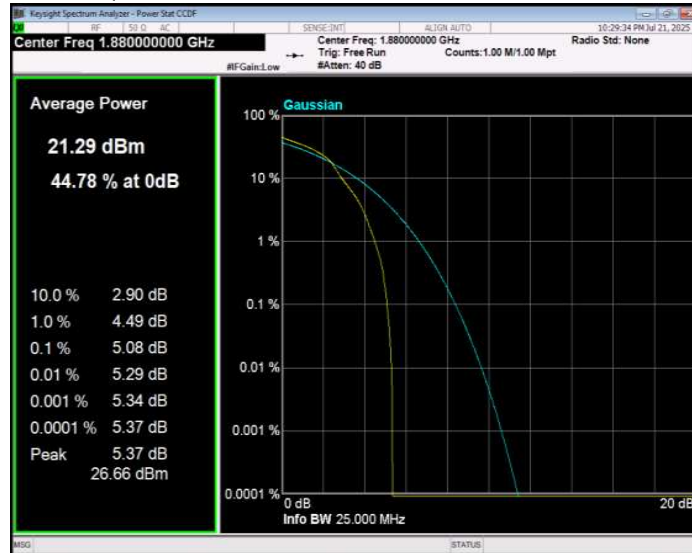
Band2 16QAM BW=3MHz Channel=19185 RB Size=1 Position=#0
