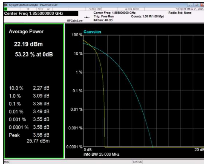
Band2 QPSK BW=10MHz Channel=18900 RB Size=1 Position=#0
