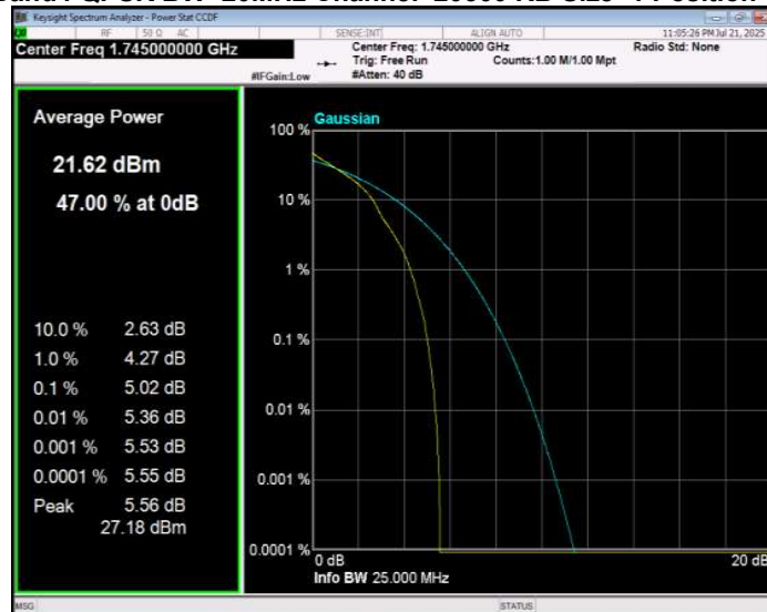
Band4 QPSK BW=3MHz Channel=19965 RB Size=1 Position=#0
