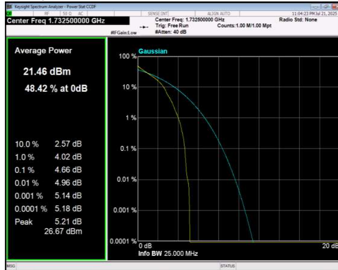
Band4 QPSK BW=10MHz Channel=20350 RB Size=1 Position=#0
