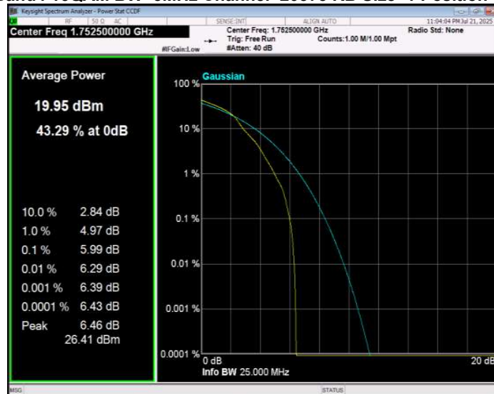
Band4 QPSK BW=1.4MHz Channel=19957 RB Size=1 Position=#0
