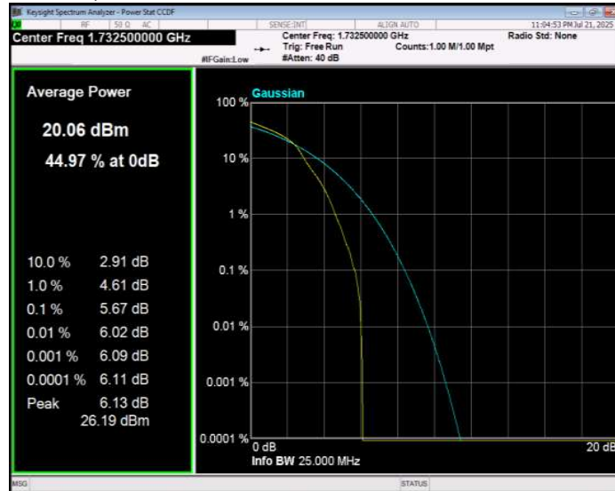
Band4 16QAM BW=15MHz Channel=20325 RB Size=1 Position=#0
