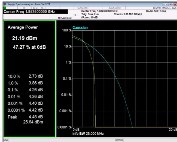
Band2 16QAM BW=5MHz Channel=18900 RB Size=1 Position=#0
