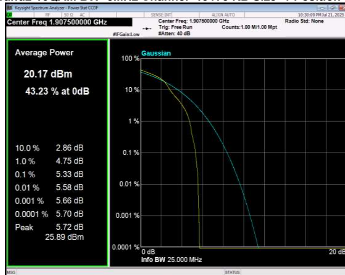
Band2 QPSK BW=1.4MHz Channel=18607 RB Size=1 Position=#0
