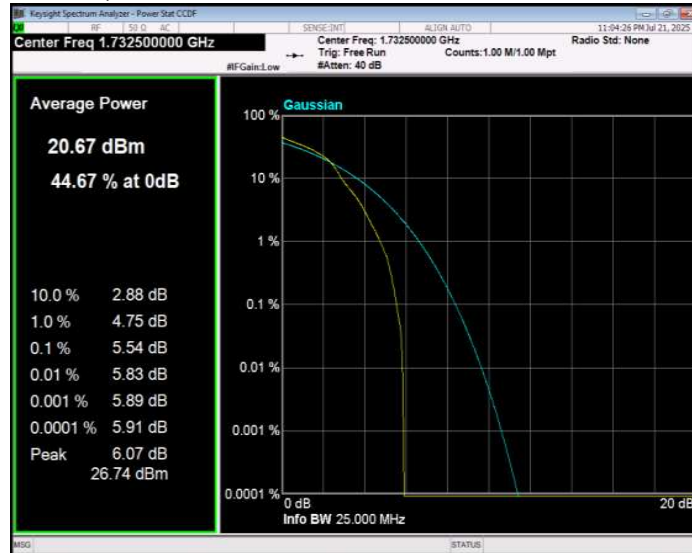
Band4 16QAM BW=10MHz Channel=20350 RB Size=1 Position=#0
