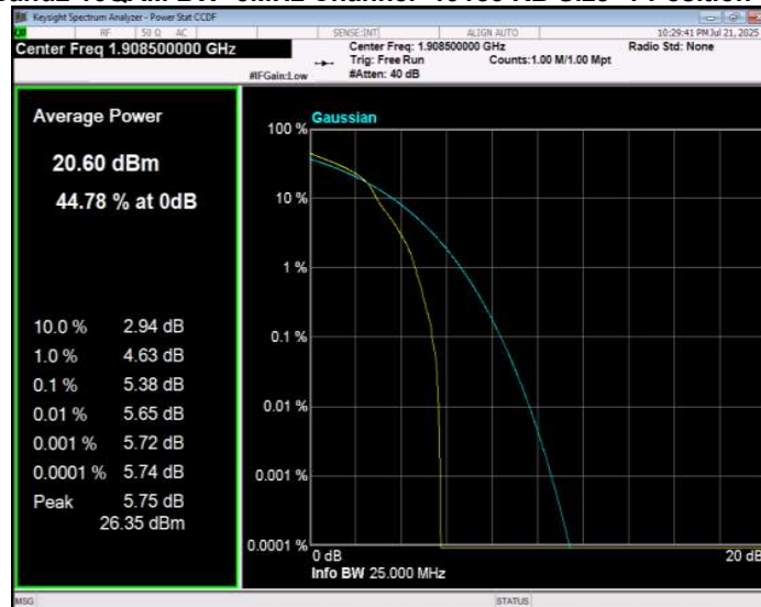
Band2 16QAM BW=5MHz Channel=18625 RB Size=1 Position=#0
