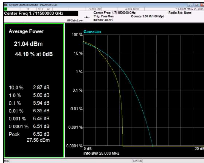
Band4 16QAM BW=3MHz Channel=20175 RB Size=1 Position=#0
