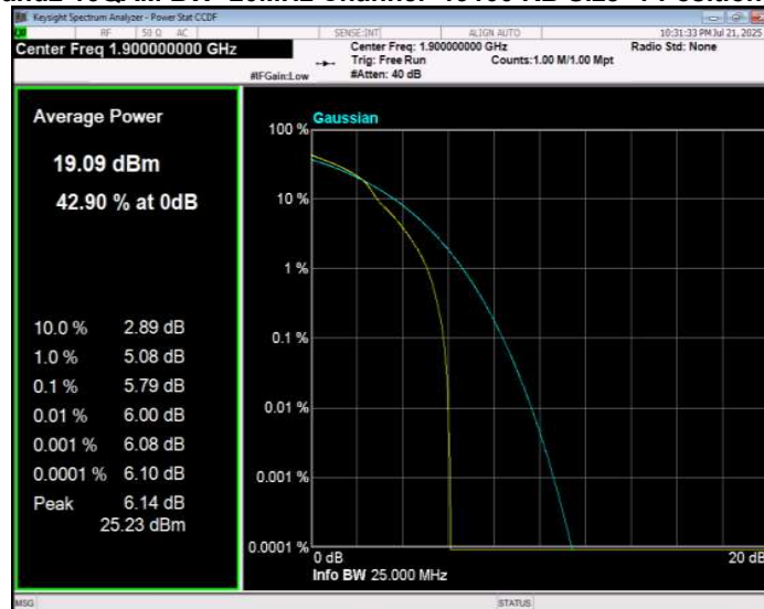
Band2 16QAM BW=3MHz Channel=18615 RB Size=1 Position=#0
