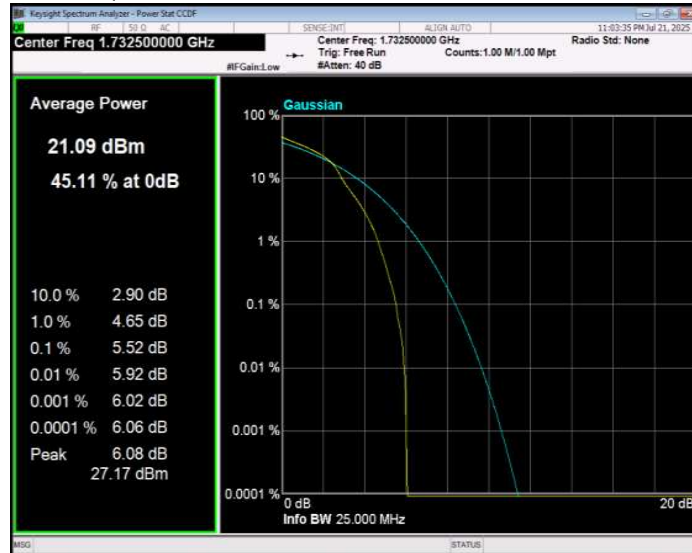
Band4 16QAM BW=3MHz Channel=20385 RB Size=1 Position=#0
