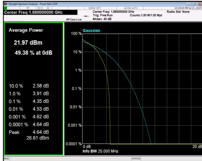
Band2 QPSK BW=1.4MHz Channel=19193 RB Size=1 Position=#0
