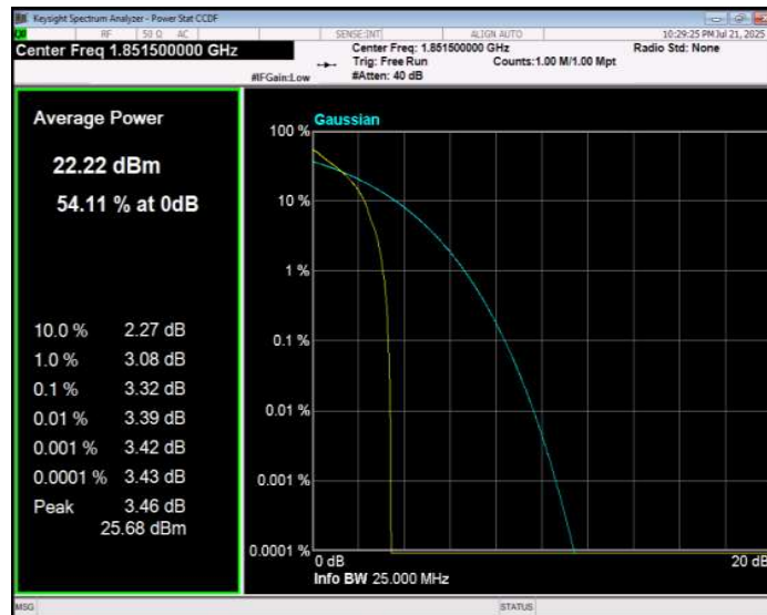
Band2 QPSK BW=3MHz Channel=18900 RB Size=1 Position=#0
