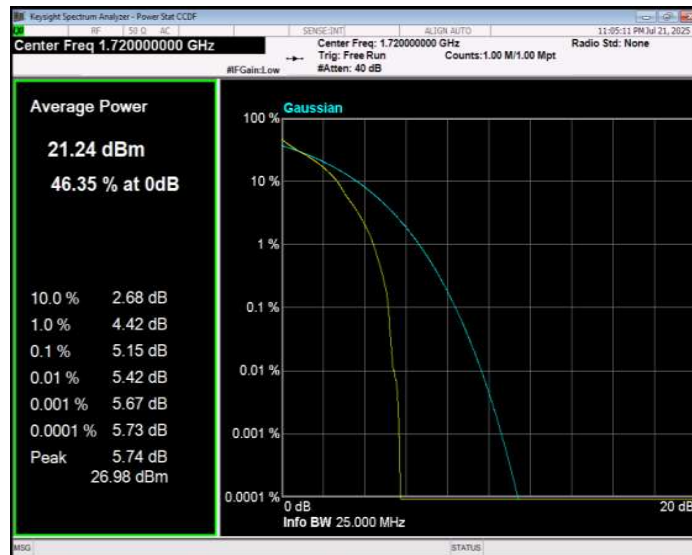
Band4 QPSK BW=20MHz Channel=20175 RB Size=1 Position=#0
