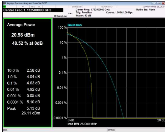
Band4 QPSK BW=15MHz Channel=20325 RB Size=1 Position=#0
