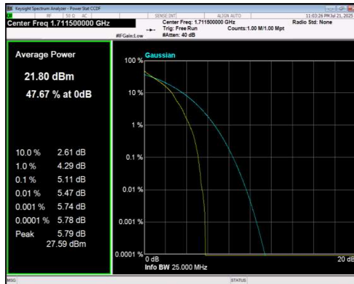
Band4 QPSK BW=3MHz Channel=20175 RB Size=1 Position=#0
