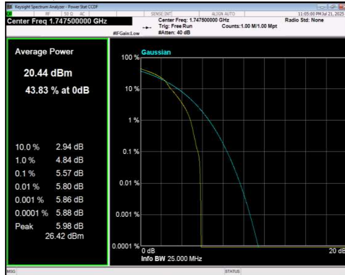
Band4 16QAM BW=20MHz Channel=20050 RB Size=1 Position=#0
