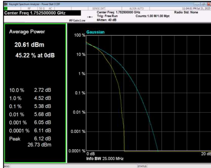
Band4 QPSK BW=5MHz Channel=20375 RB Size=1 Position=#0
