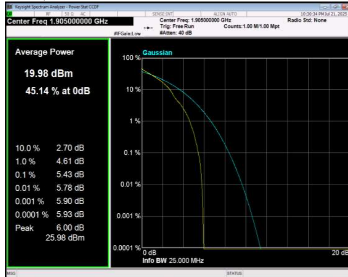
Band2 QPSK BW=15MHz Channel=18675 RB Size=1 Position=#0
