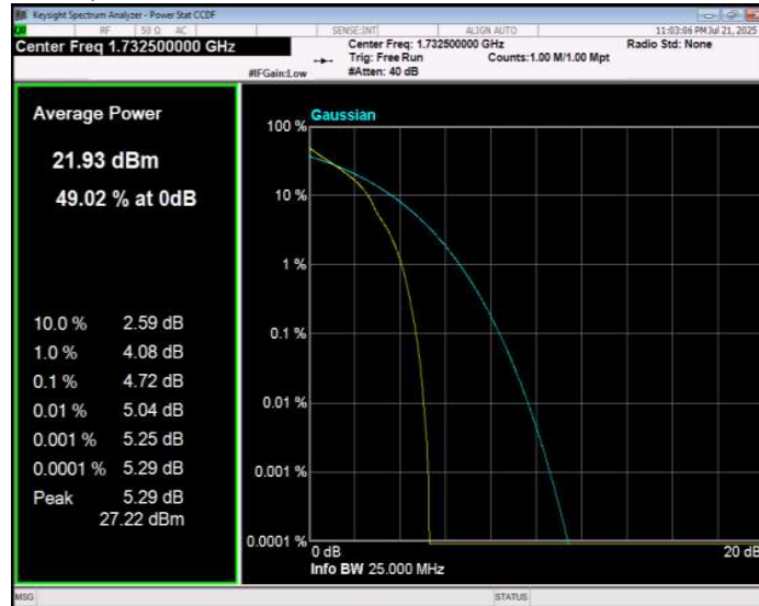
Band4 QPSK BW=1.4MHz Channel=20393 RB Size=1 Position=#0
