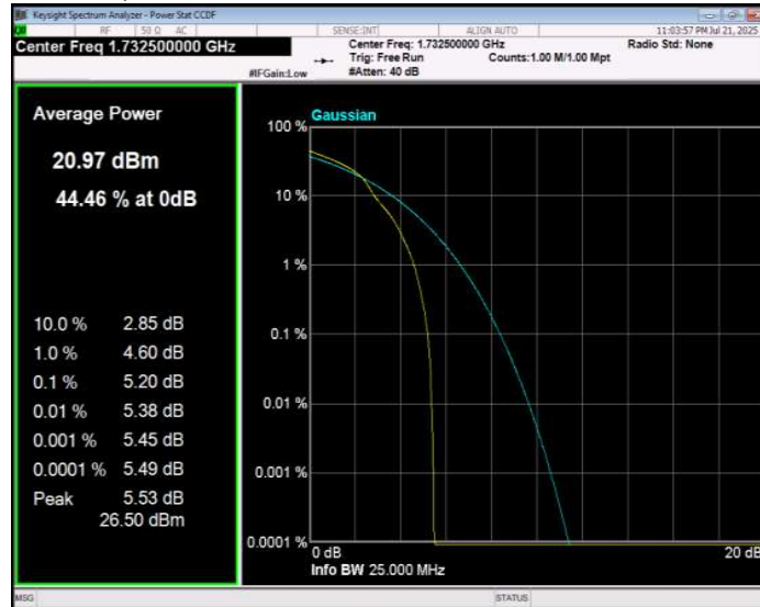
Band4 16QAM BW=5MHz Channel=20375 RB Size=1 Position=#0
