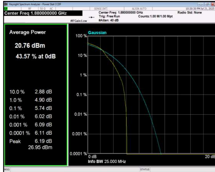
Band2 16QAM BW=10MHz Channel=19150 RB Size=1 Position=#0
