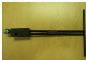
Figure 1 – MVG COMOSAR Validation Dipole
