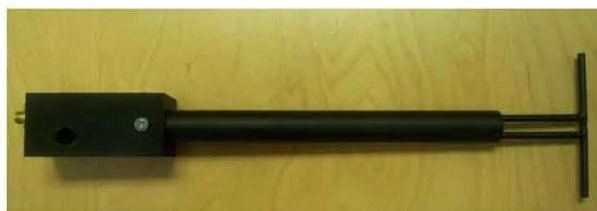
Figure 1 – MVG COMOSAR Validation Dipole
