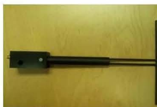
Figure 1 – MVG COMOSAR Validation Dipole
