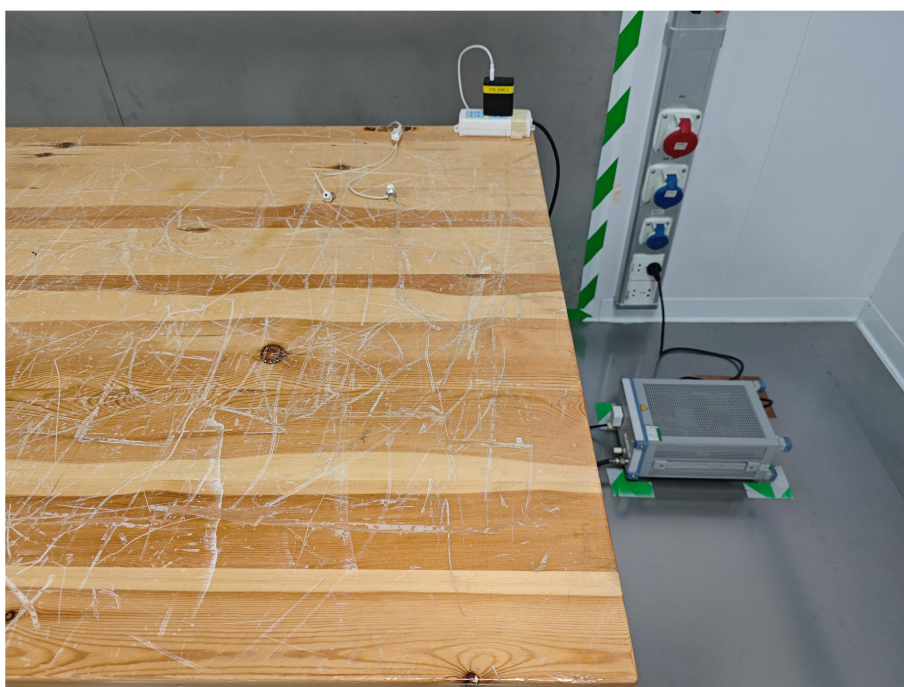
Conduction Emissions Test Setup
