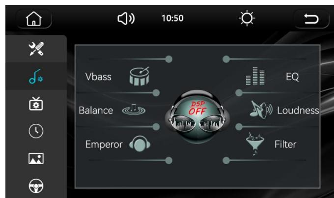
Adjust the volume for the right front, front left, rear right, rear left speakers, and the subwoofer. Before making any adjustments, press "DSP OFF" in the center to activate and enable the "DSP" feature.
