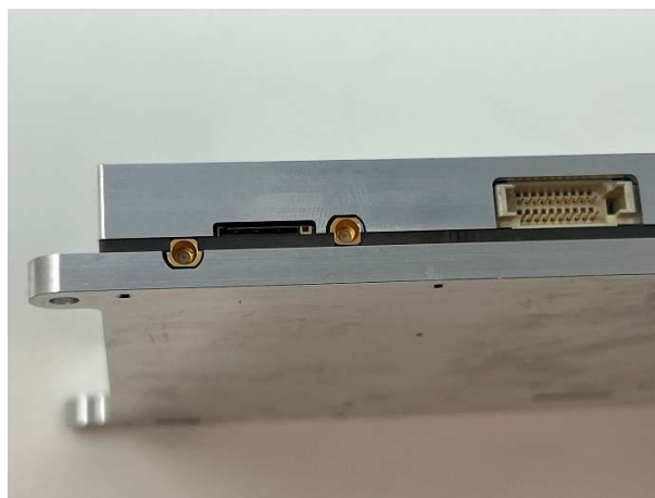
Figure 8 - Gotonomi Multilink LTE Antenna ports. Main antenna connector bottom left, diversity antenna connector closer to the centre
