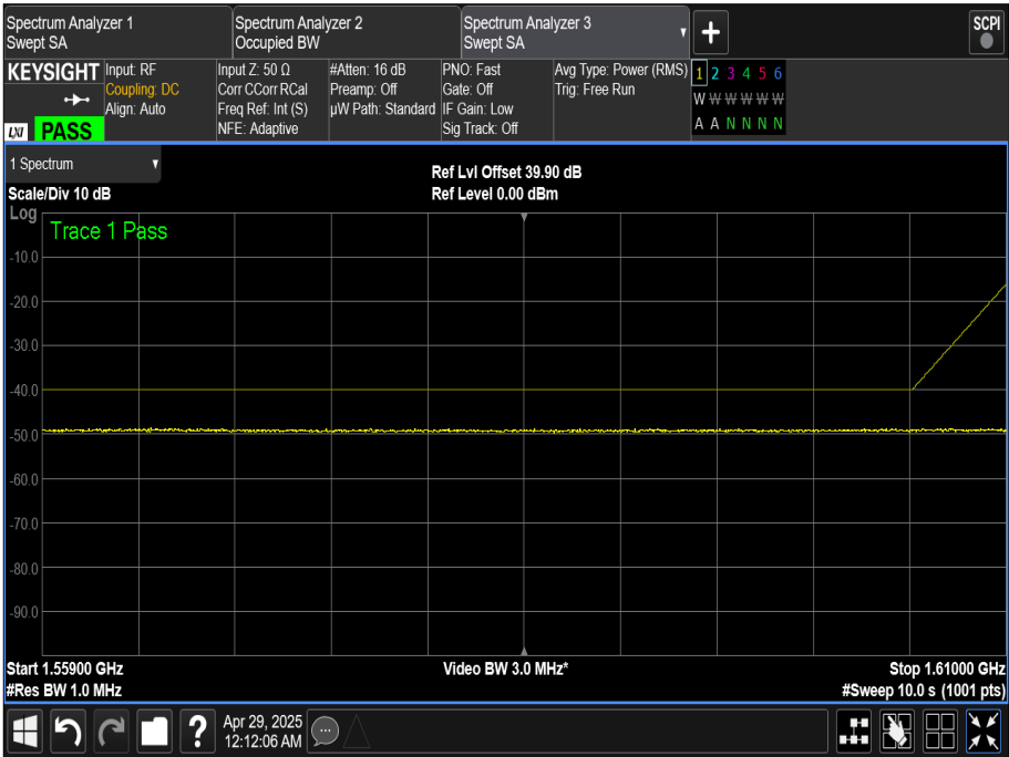
Figure 74 - 1626.712 MHz – Broadband Emission Results
