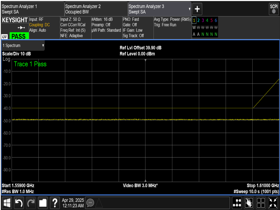
Figure 76 - 1643.500 MHz – Broadband Emission Results
