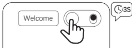
Power on status Press and hold the power button for 3 seconds to shut down the device.
