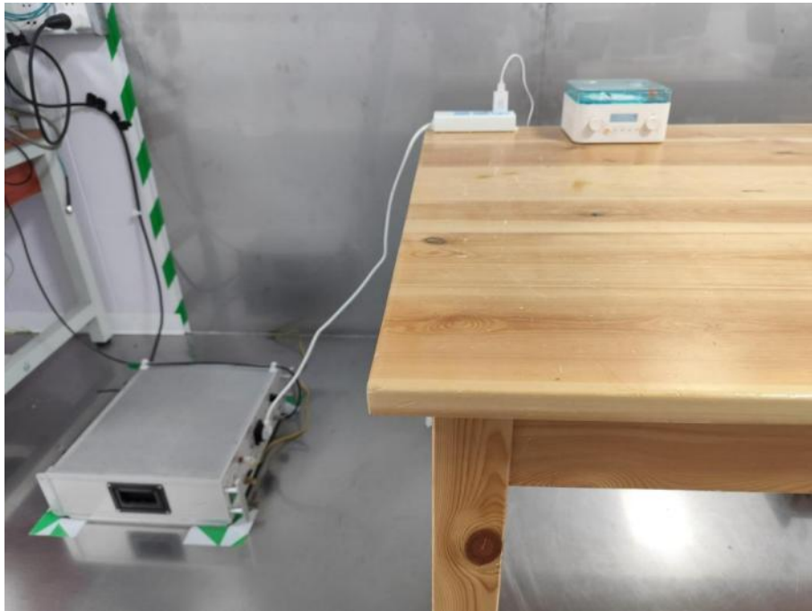
Conducted Emission at AC power line
