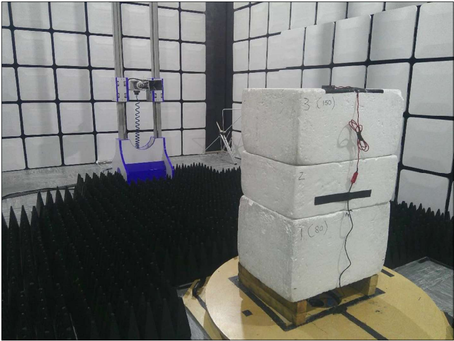
Figure 60 - Test Setup - 1 GHz to 8 GHz X Plane
