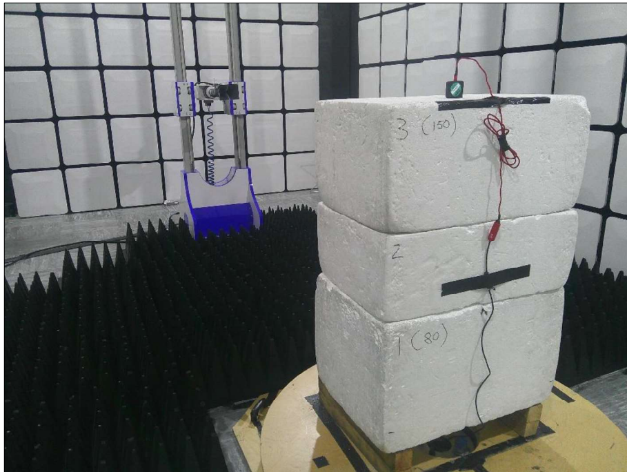
Figure 61 - Test Setup - 1 GHz to 8 GHz Y Plane
