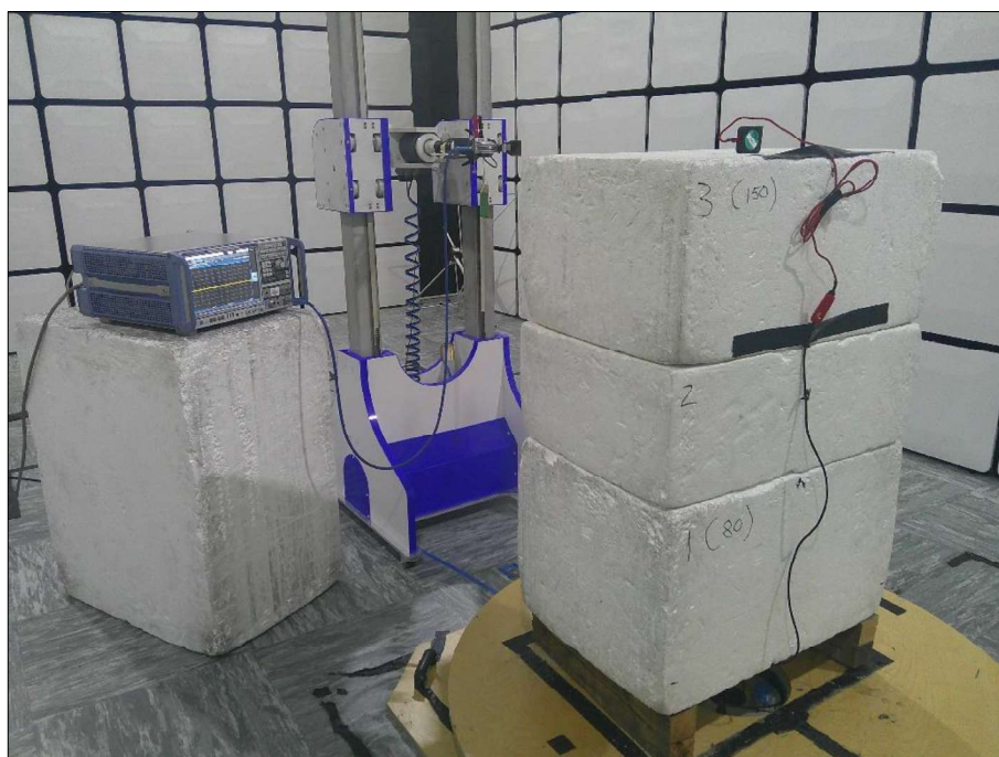
Figure 68 - Test Setup - 18 GHz to 25 GHz Z Plane
