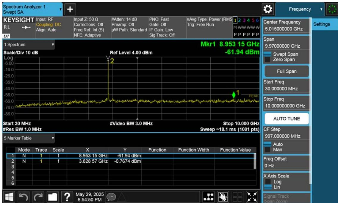
n77(3700~3980 MHz)\_30 M\_Conducted Spurious(30 M-10 G)\_High\_BPSK\_1RB
