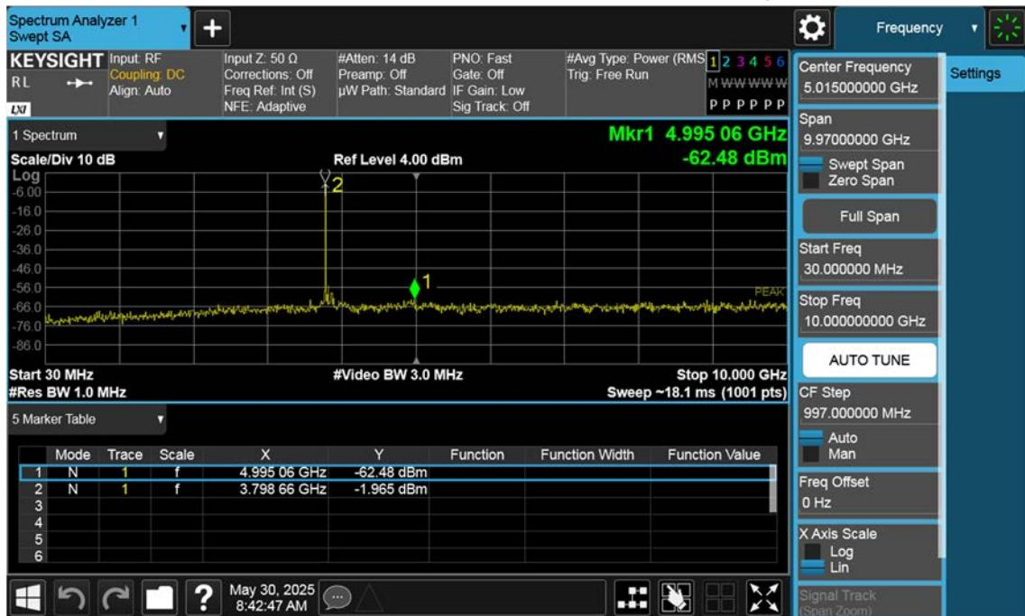
n77(3700~3980 MHz)\_100 M\_Conducted Spurious(30 M-10 G)\_Low\_BPSK\_1RB
