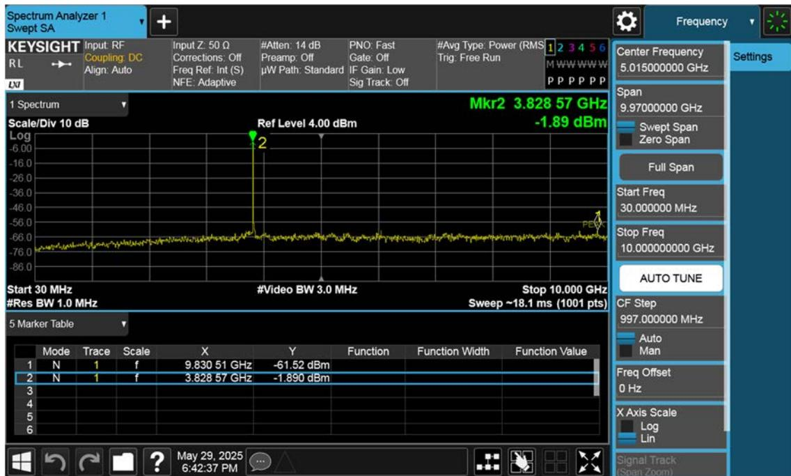
n77(3700~3980 MHz)\_25 M\_Conducted Spurious(30 M-10 G)\_High\_BPSK\_1RB
