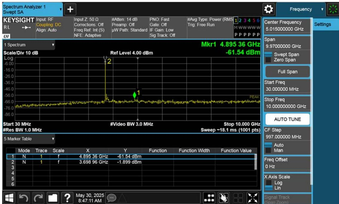
n77(3700~3980 MHz)\_100 M\_Conducted Spurious(30 M-10 G)\_Mid\_BPSK\_1RB
