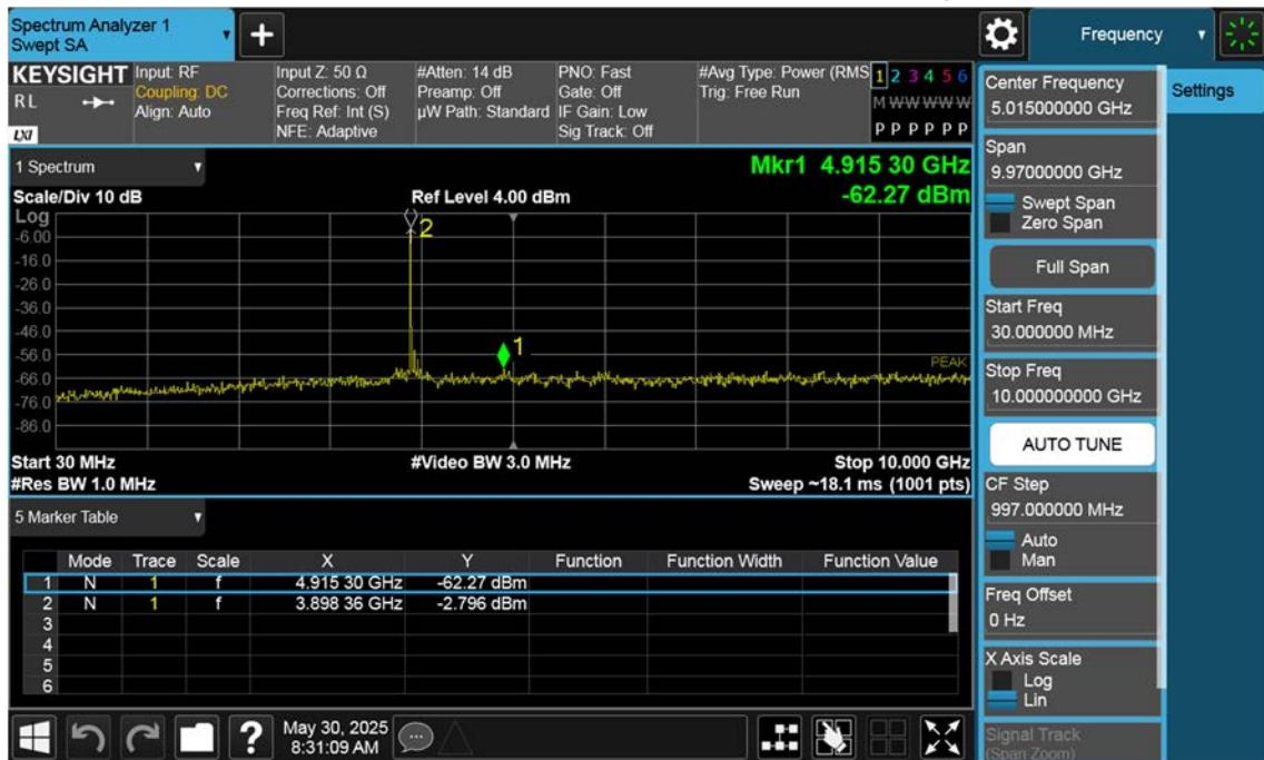
n77(3700~3980 MHz)\_90 M\_Conducted Spurious(30 M-10 G)\_Low\_BPSK\_1RB
