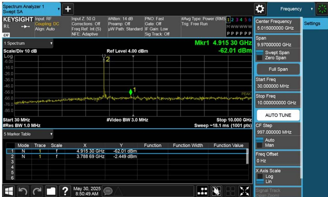
n77(3700~3980 MHz)\_100 M\_Conducted Spurious(30 M-10 G)\_High\_BPSK\_1RB
