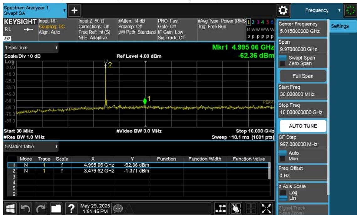
n77(3450~3550 MHz)\_40 M\_Conducted Spurious(30 M-10 G)\_High\_BPSK\_1RB
