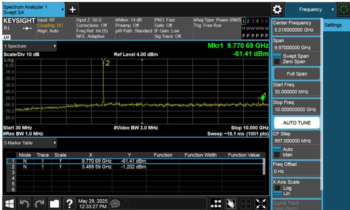
n77(3450~3550 MHz)\_20 M\_Conducted Spurious(30 M-10 G)\_High\_BPSK\_1RB
