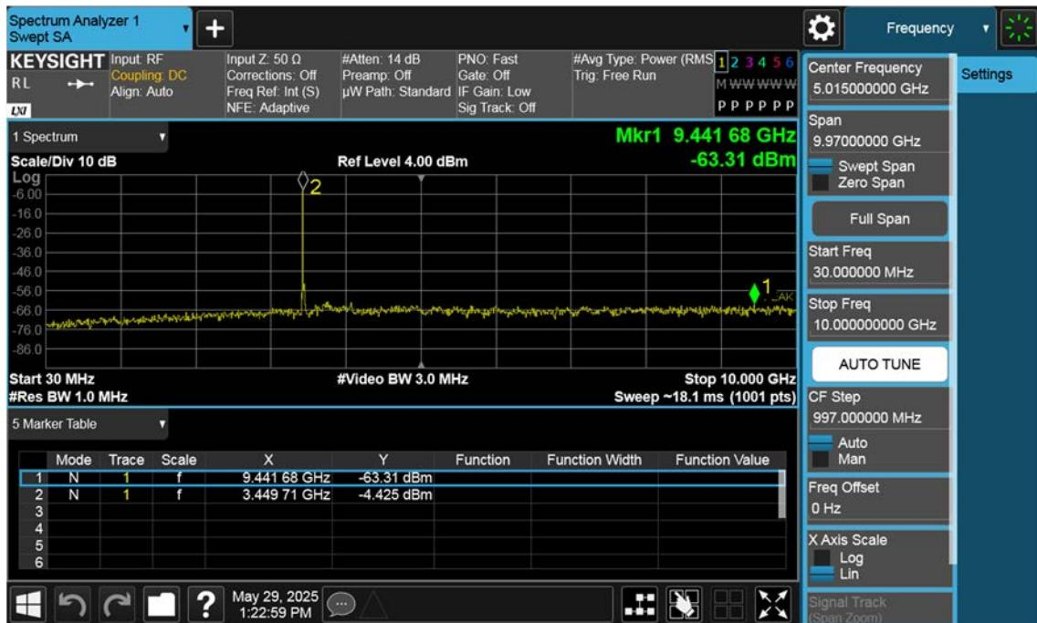
n77(3450~3550 MHz)\_25 M\_Conducted Spurious(30 M-10 G)\_Mid\_BPSK\_1RB
