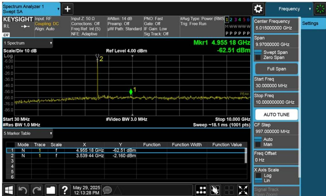
n77(3450~3550 MHz)\_15 M\_Conducted Spurious(30 M-10 G)\_Low\_BPSK\_1RB
