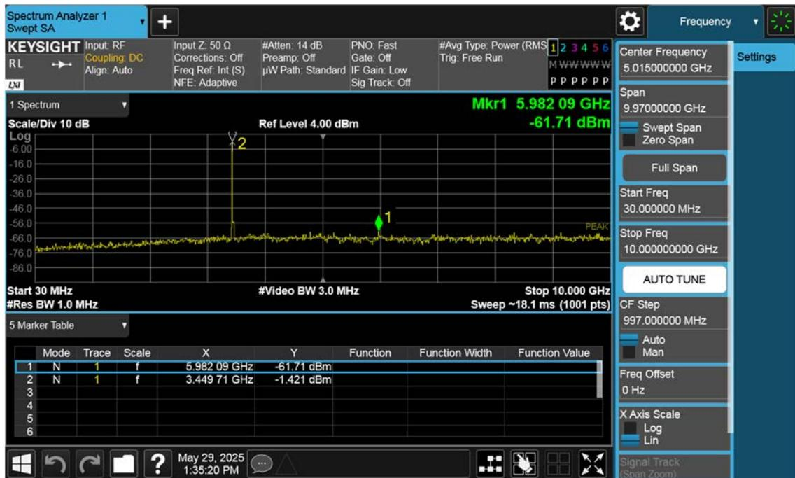
n77(3450~3550 MHz)\_30 M\_Conducted Spurious(30 M-10 G)\_Mid\_BPSK\_1RB
