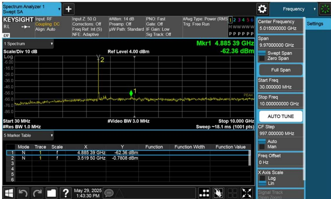
n77(3450~3550 MHz)\_40 M\_Conducted Spurious(30 M-10 G)\_Low\_BPSK\_1RB
