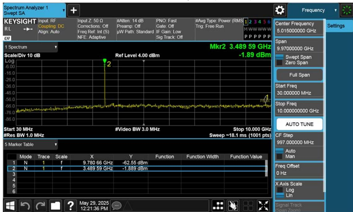
n77(3450~3550 MHz)\_15 M\_Conducted Spurious(30 M-10 G)\_High\_BPSK\_1RB
