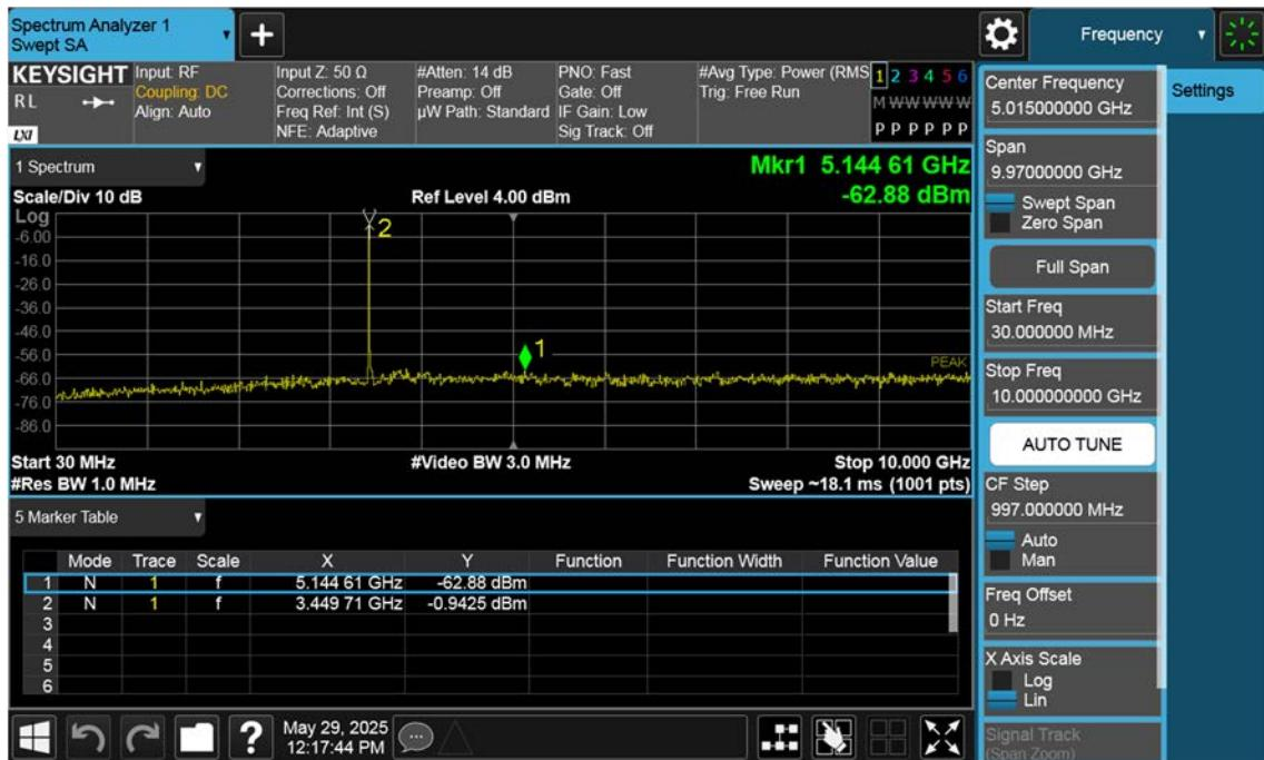
n77(3450~3550 MHz)\_15 M\_Conducted Spurious(30 M-10 G)\_Mid\_BPSK\_1RB
