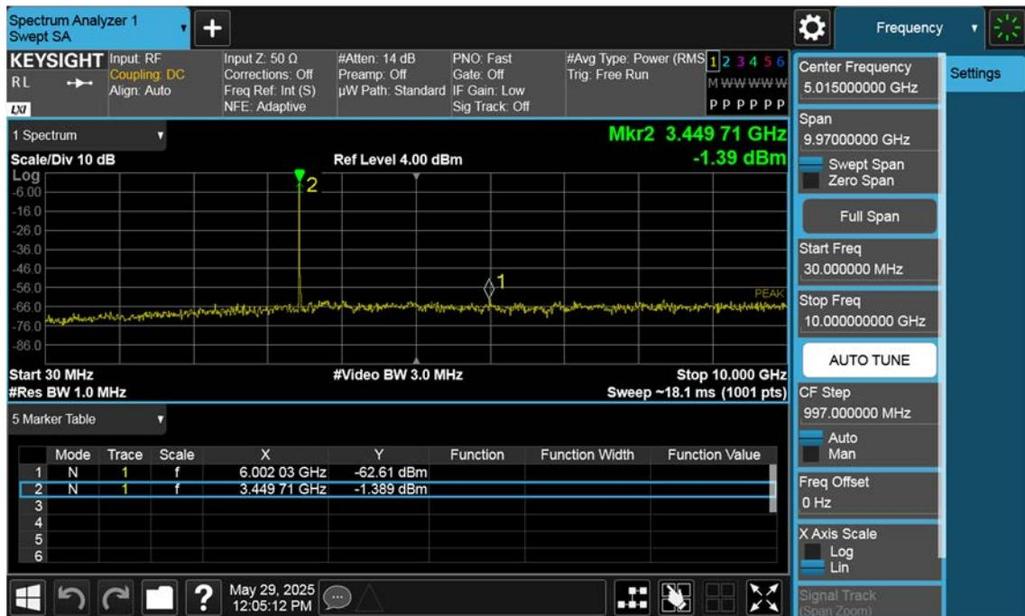
n77(3450~3550 MHz)\_10 M\_Conducted Spurious(30 M-10 G)\_Mid\_BPSK\_1RB
