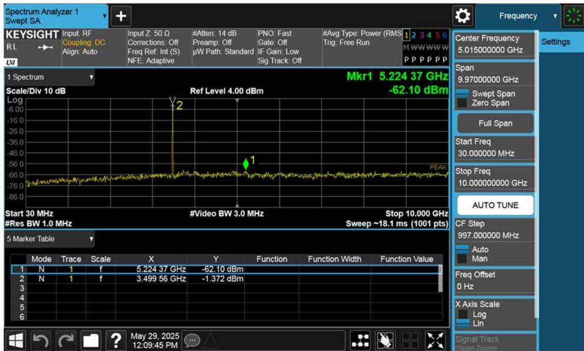
n77(3450~3550 MHz)\_10 M\_Conducted Spurious(30 M-10 G)\_High\_BPSK\_1RB
