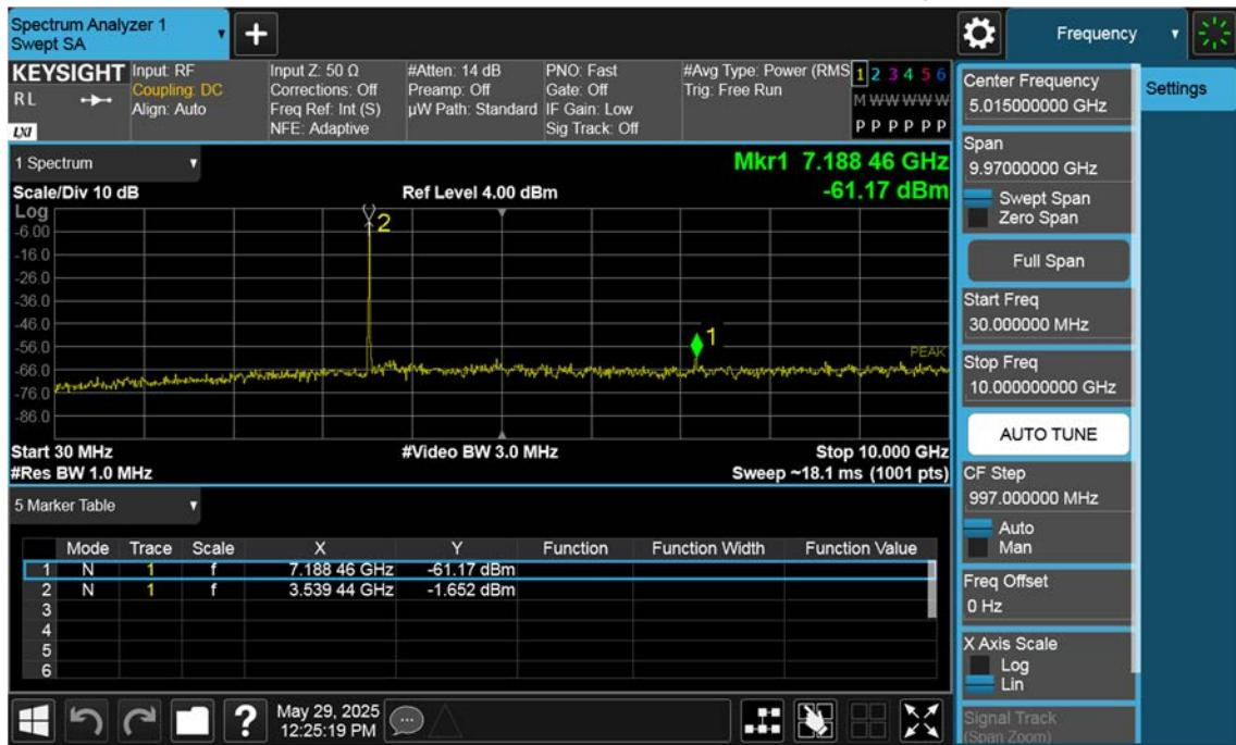
n77(3450~3550 MHz)\_20 M\_Conducted Spurious(30 M-10 G)\_Low\_BPSK\_1RB
