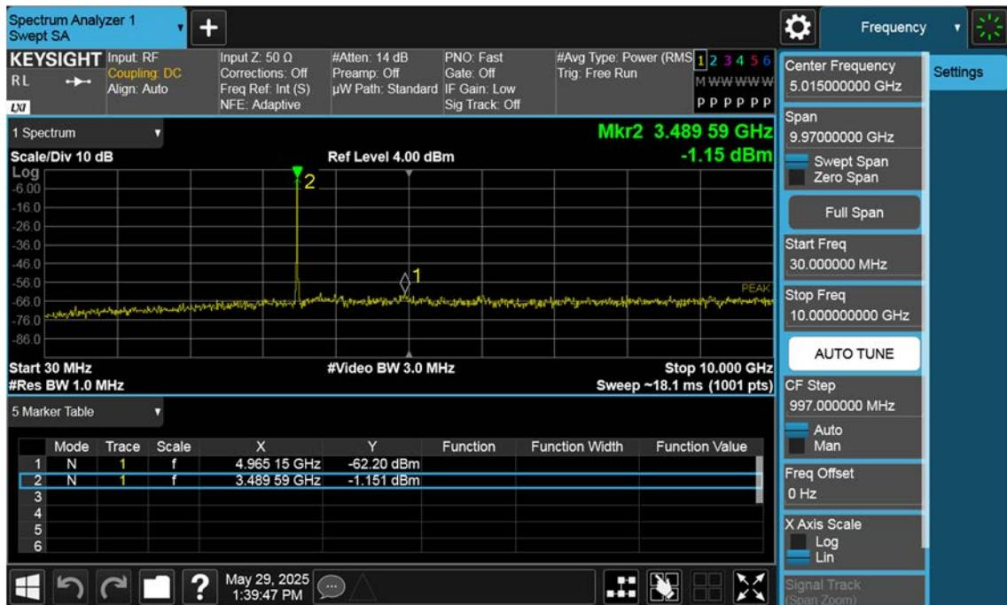
n77(3450~3550 MHz)\_30 M\_Conducted Spurious(30 M-10 G)\_High\_BPSK\_1RB
