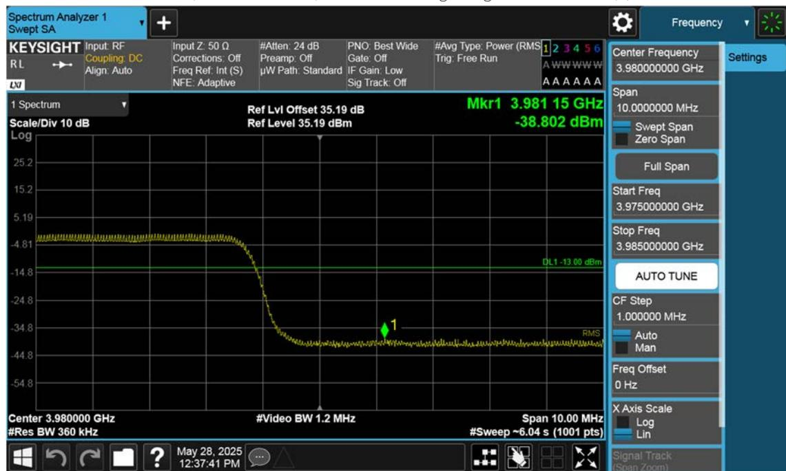
n77(3700~3980 MHz)\_80 M\_Band Edge\_High\_BPSK\_1RB(1)
