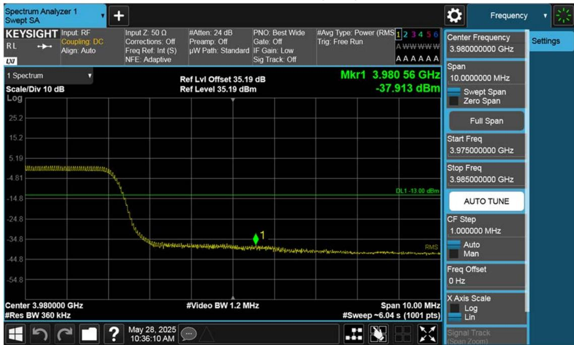
n77(3700~3980 MHz)\_50 M\_Band Edge\_High\_BPSK\_1RB(1)
