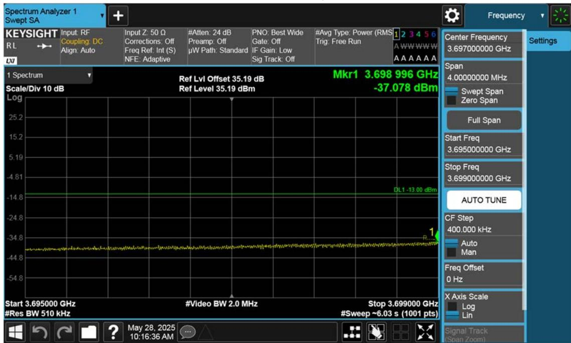
n77(3700~3980 MHz)\_40 M\_Band Edge\_Low\_BPSK\_1RB(2)
