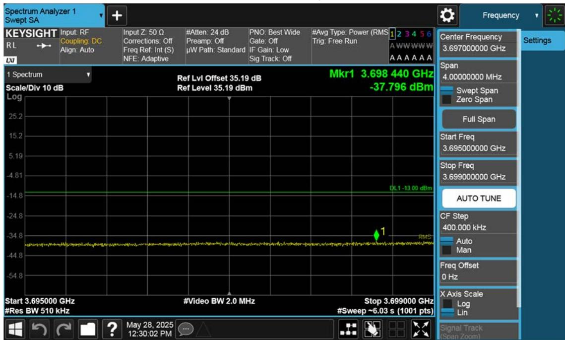
n77(3700~3980 MHz)\_80 M\_Band Edge\_Low\_BPSK\_1RB(2)
