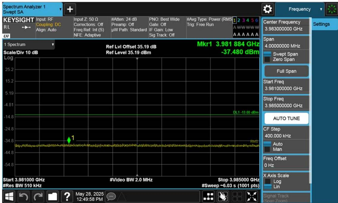
n77(3700~3980 MHz)\_90 M\_Band Edge\_High\_BPSK\_1RB(2)
