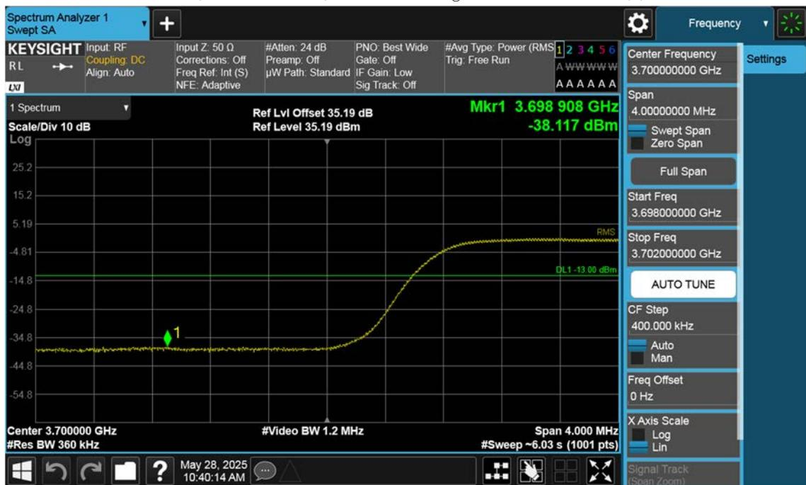
n77(3700~3980 MHz)\_60 M\_Band Edge\_Low\_BPSK\_1RB(1)
