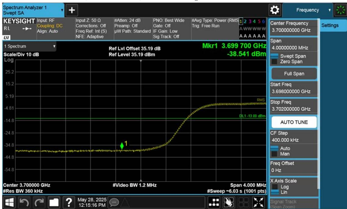
n77(3700~3980 MHz)\_70 M\_Band Edge\_Low\_BPSK\_1RB(1)
