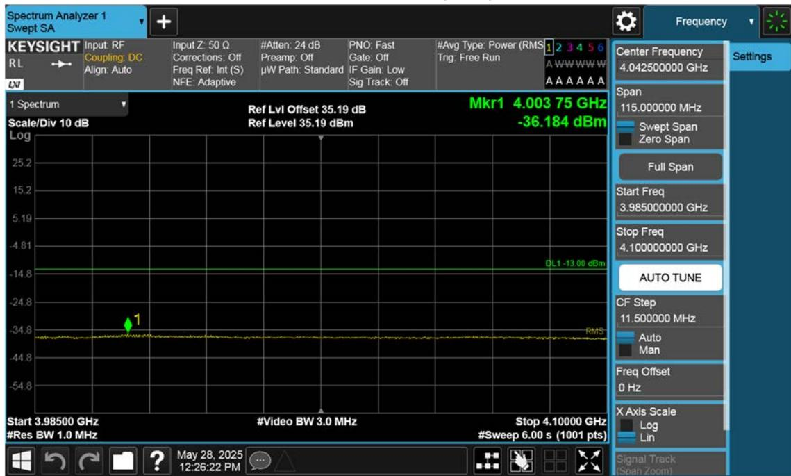
n77(3700~3980 MHz)\_70 M\_Band Edge\_High\_BPSK\_1RB(3)
