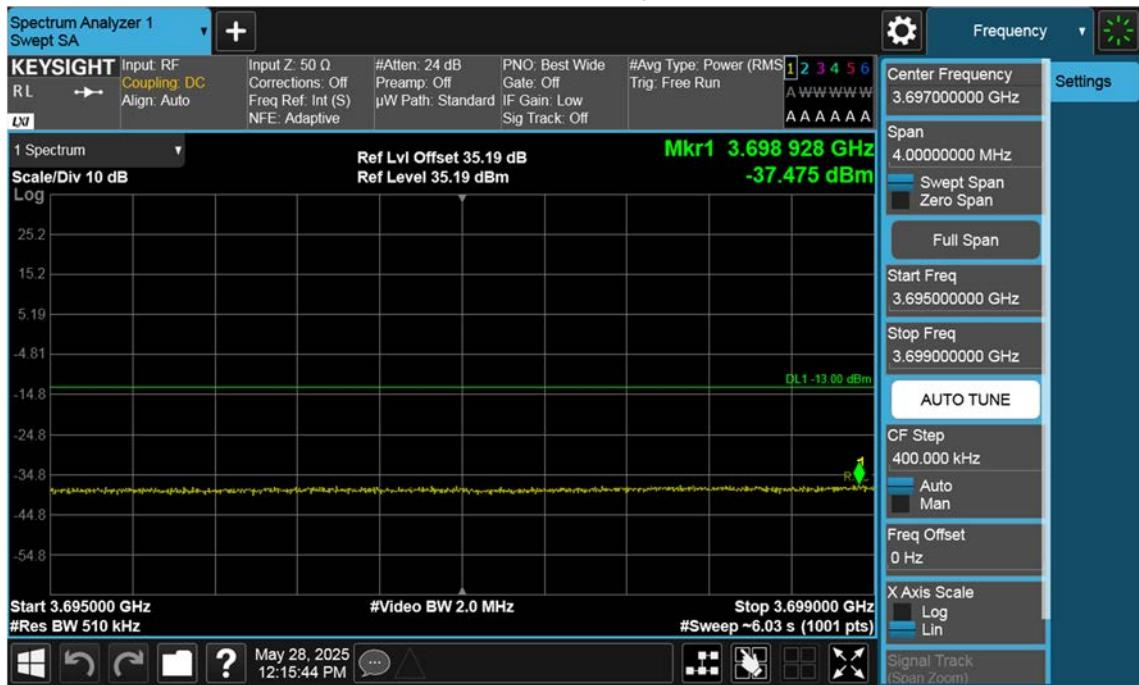
n77(3700~3980 MHz)\_70 M\_Band Edge\_Low\_BPSK\_1RB(2)
