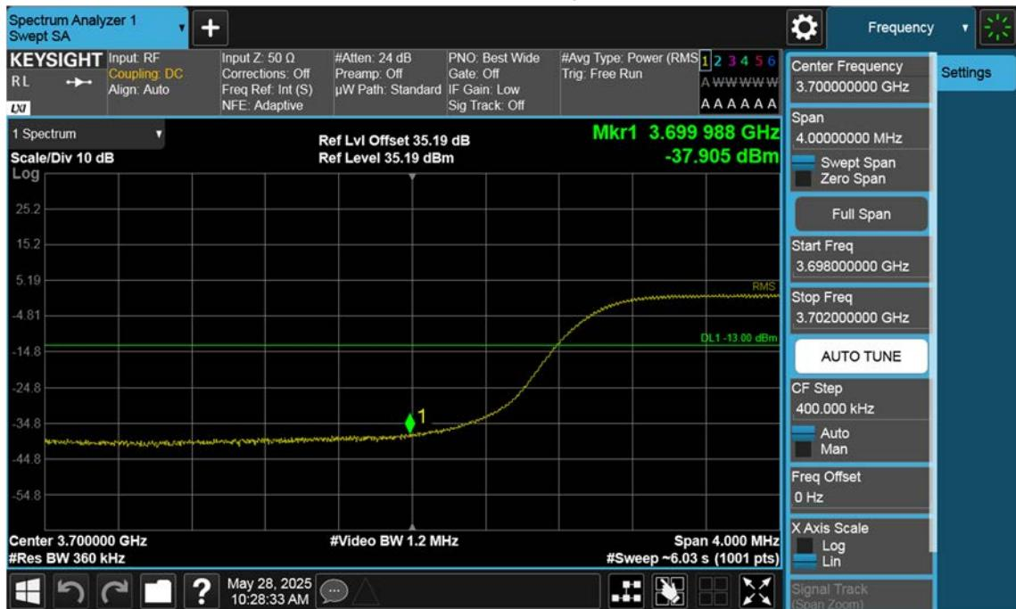
n77(3700~3980 MHz)\_50 M\_Band Edge\_Low\_BPSK\_1RB(1)
