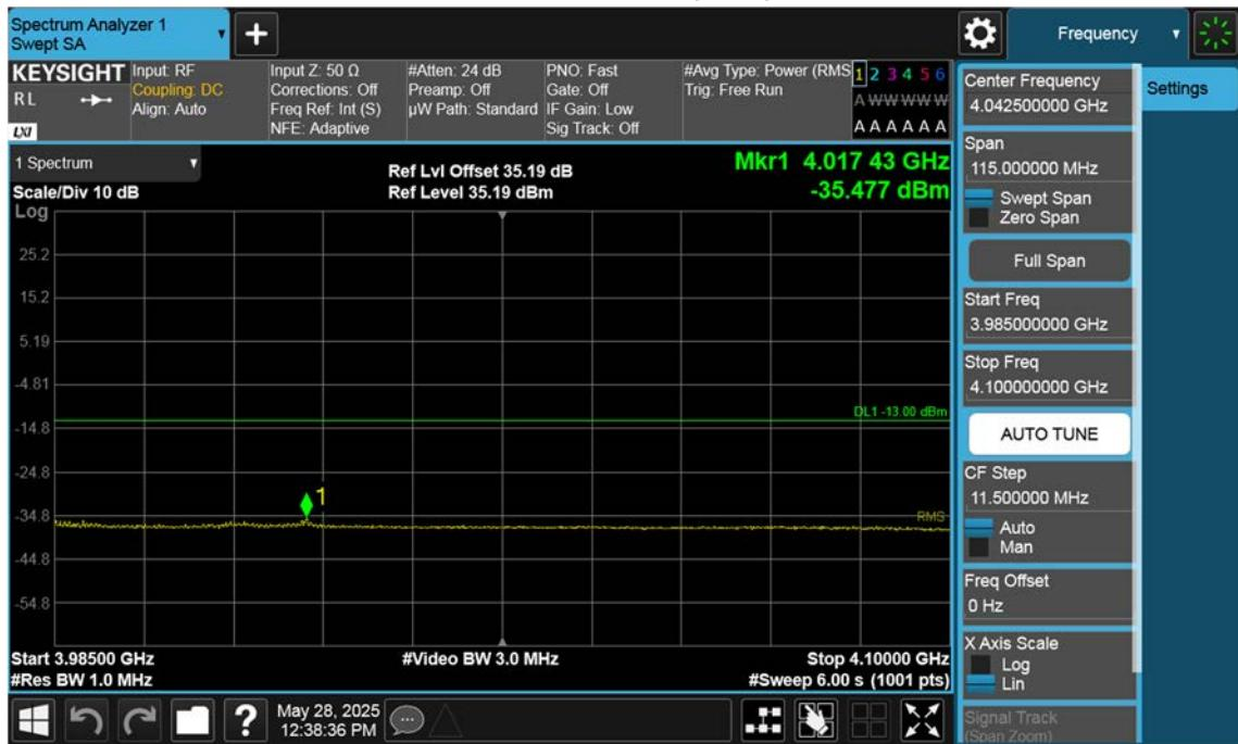
n77(3700~3980 MHz)\_80 M\_Band Edge\_High\_BPSK\_1RB(3)
