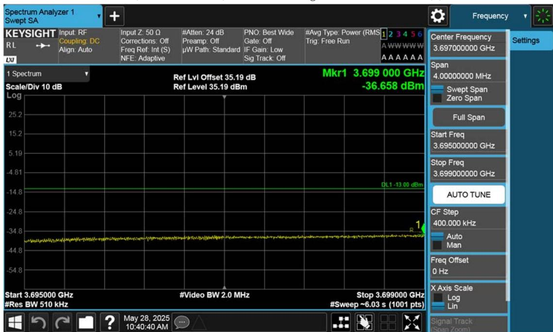
n77(3700~3980 MHz)\_60 M\_Band Edge\_Low\_BPSK\_1RB(2)
