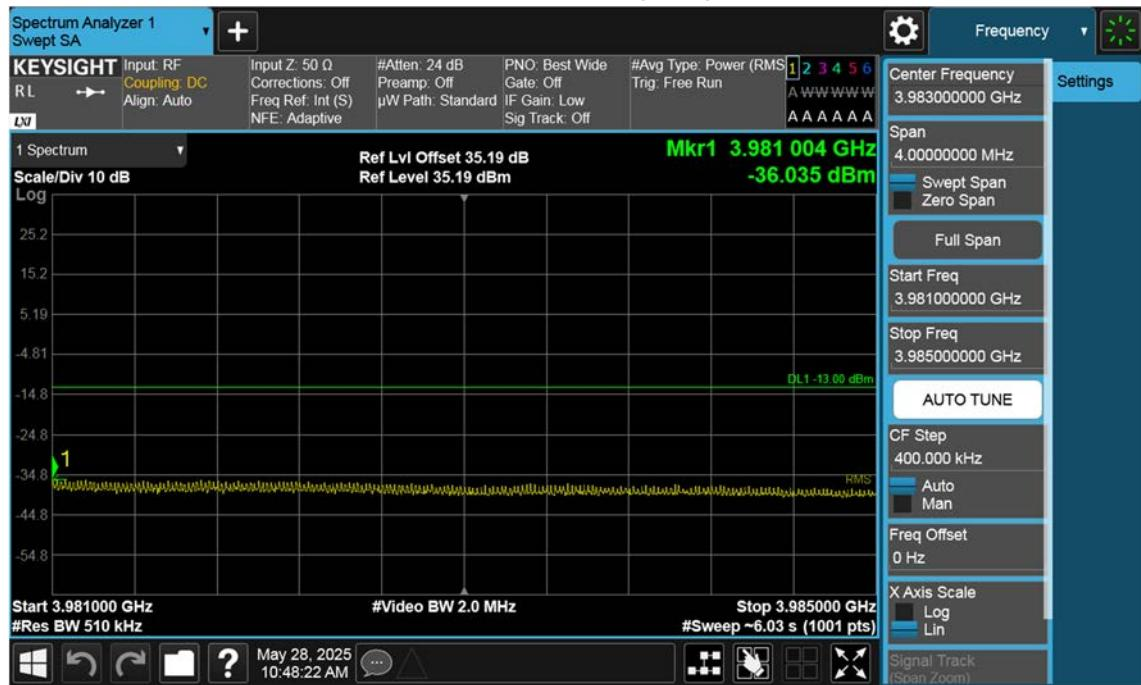
n77(3700~3980 MHz)\_60 M\_Band Edge\_High\_BPSK\_1RB(2)
