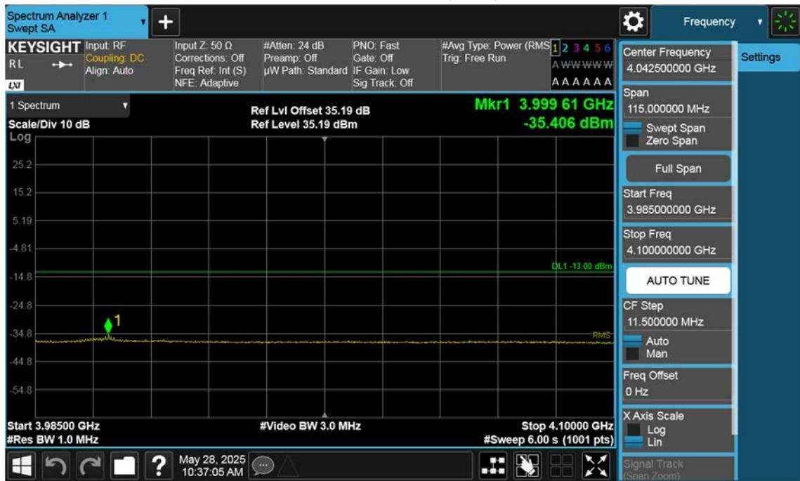
n77(3700~3980 MHz)\_50 M\_Band Edge\_High\_BPSK\_1RB(3)
