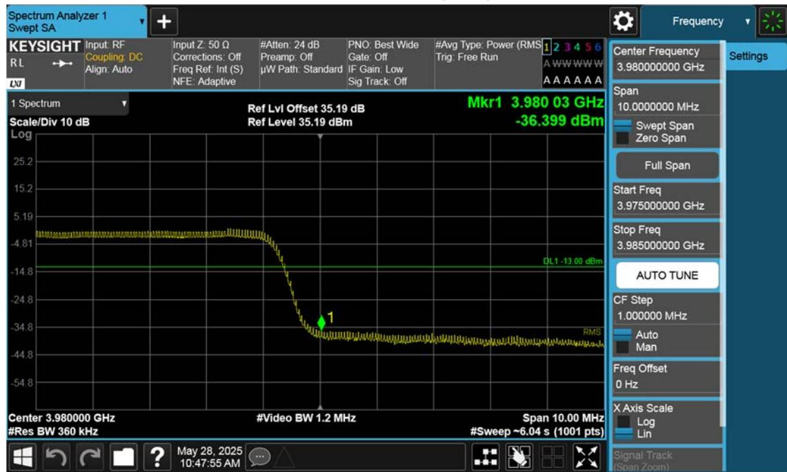
n77(3700~3980 MHz)\_60 M\_Band Edge\_High\_BPSK\_1RB(1)
