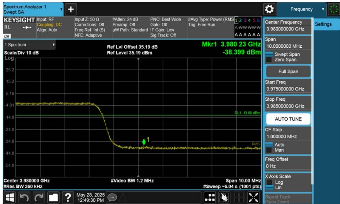
n77(3700~3980 MHz)\_90 M\_Band Edge\_High\_BPSK\_1RB(1)
