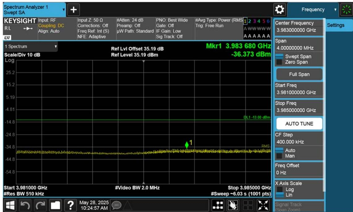
n77(3700~3980 MHz)\_40 M\_Band Edge\_High\_BPSK\_1RB(2)
