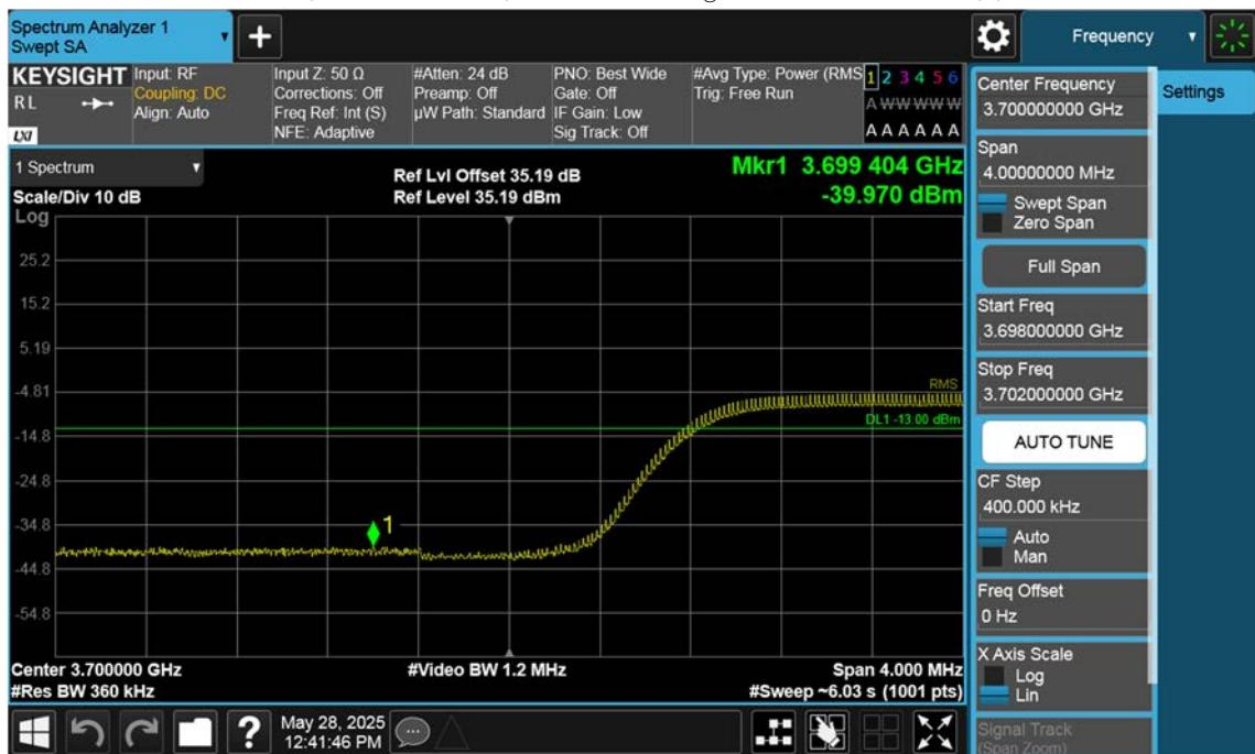
n77(3700~3980 MHz)\_90 M\_Band Edge\_Low\_BPSK\_1RB(1)
