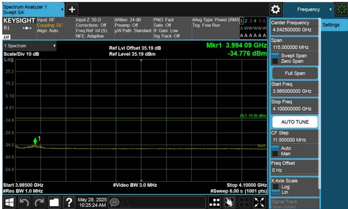
n77(3700~3980 MHz)\_40 M\_Band Edge\_High\_BPSK\_1RB(3)
