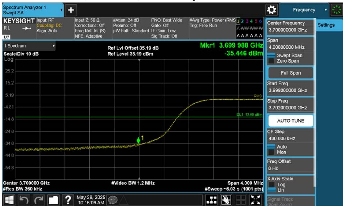
n77(3700~3980 MHz)\_40 M\_Band Edge\_Low\_BPSK\_1RB(1)
