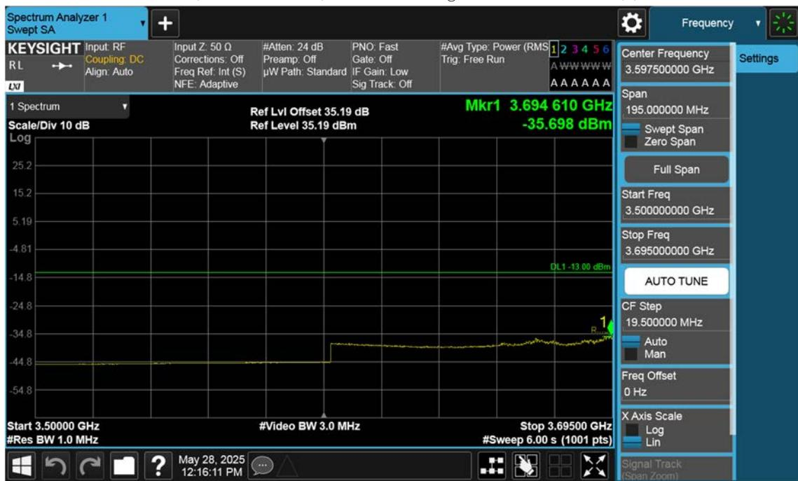
n77(3700~3980 MHz)\_70 M\_Band Edge\_Low\_BPSK\_1RB(3)
