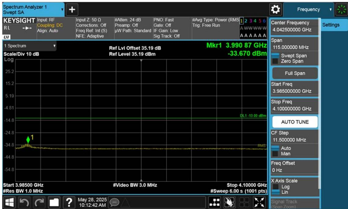
n77(3700~3980 MHz)\_30 M\_Band Edge\_High\_BPSK\_1RB(3)
