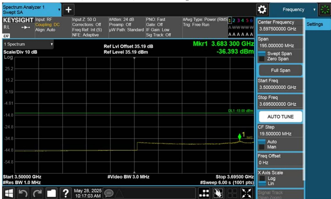
n77(3700~3980 MHz)\_40 M\_Band Edge\_Low\_BPSK\_1RB(3)
