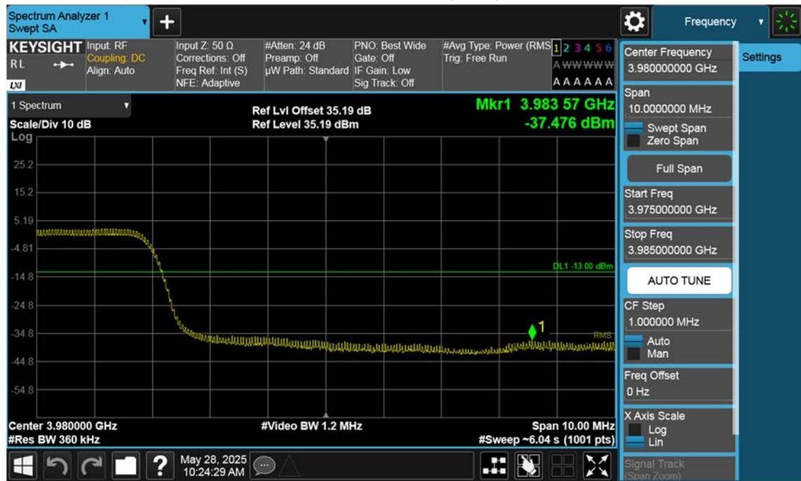
n77(3700~3980 MHz)\_40 M\_Band Edge\_High\_BPSK\_1RB(1)
