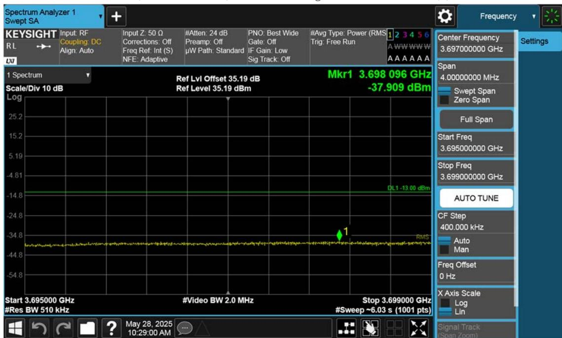
n77(3700~3980 MHz)\_50 M\_Band Edge\_Low\_BPSK\_1RB(2)
