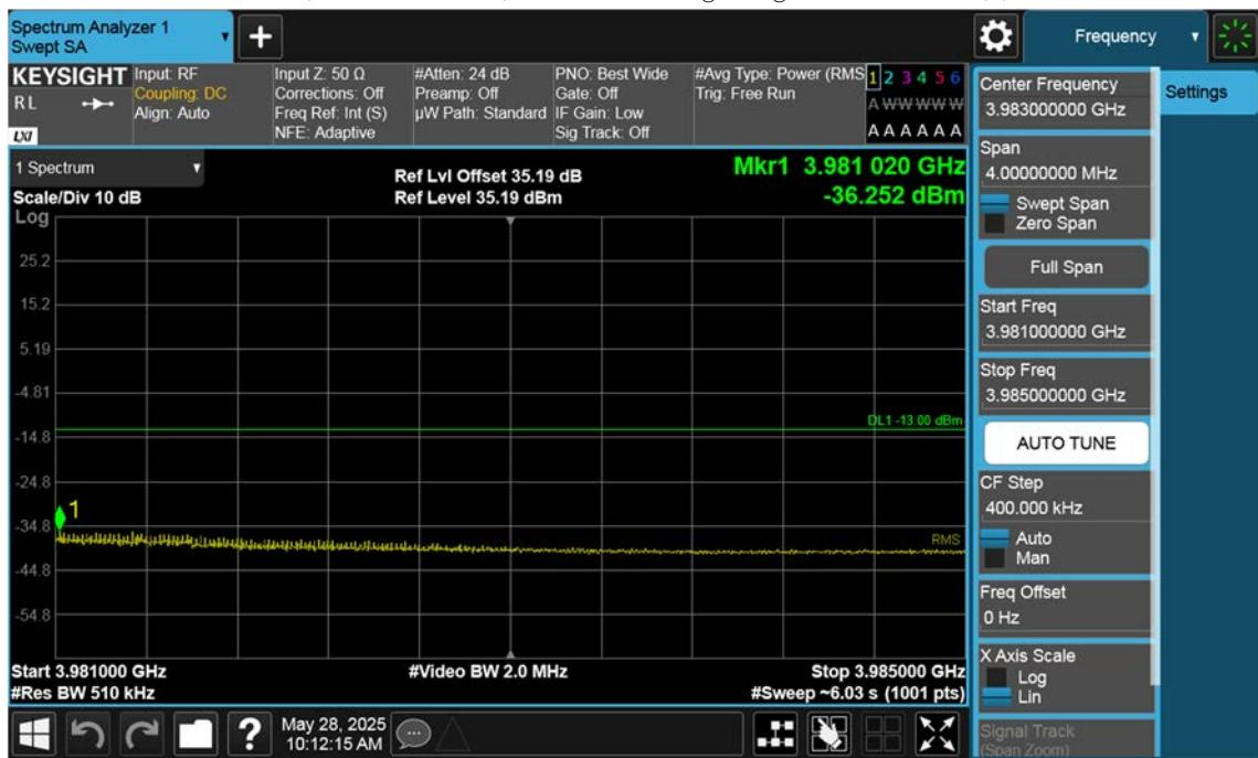
n77(3700~3980 MHz)\_30 M\_Band Edge\_High\_BPSK\_1RB(2)
