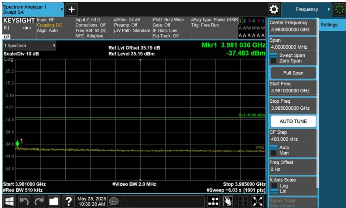
n77(3700~3980 MHz)\_50 M\_Band Edge\_High\_BPSK\_1RB(2)
