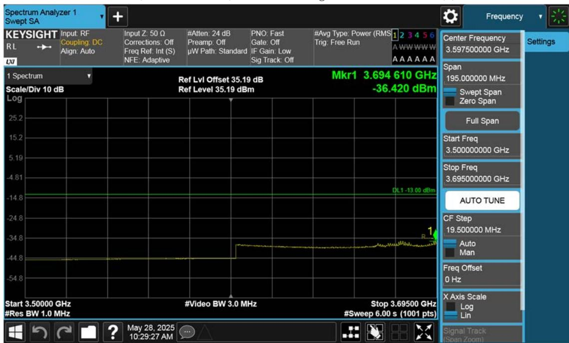
n77(3700~3980 MHz)\_50 M\_Band Edge\_Low\_BPSK\_1RB(3)
