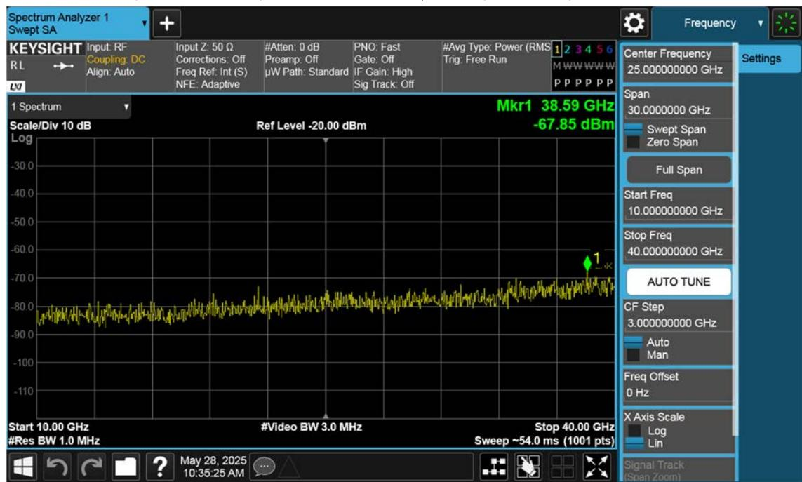
n77(3700~3980 MHz)\_50 M\_Conducted Spurious(Above10 G)\_High\_BPSK\_1RB
