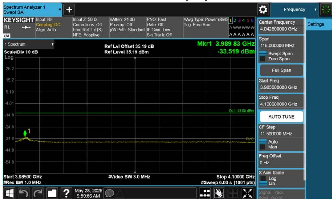
n77(3700~3980 MHz)\_25 M\_Band Edge\_High\_BPSK\_1RB(3)
