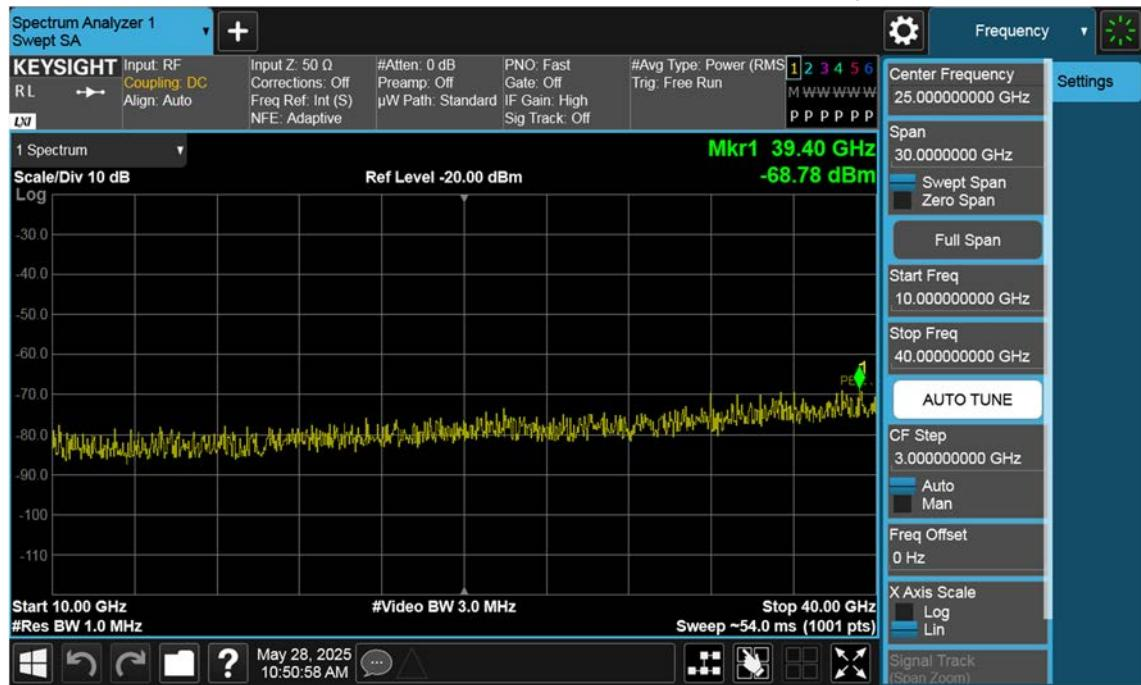
n77(3700~3980 MHz)\_70 M\_Conducted Spurious(Above10 G)\_Low\_BPSK\_1RB
