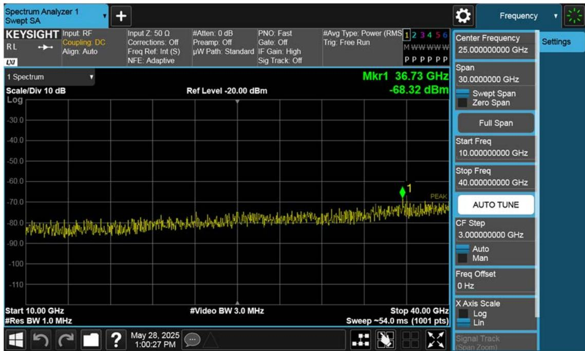
n77(3700~3980 MHz)\_100 M\_Conducted Spurious(Above10 G)\_High\_BPSK\_1RB
