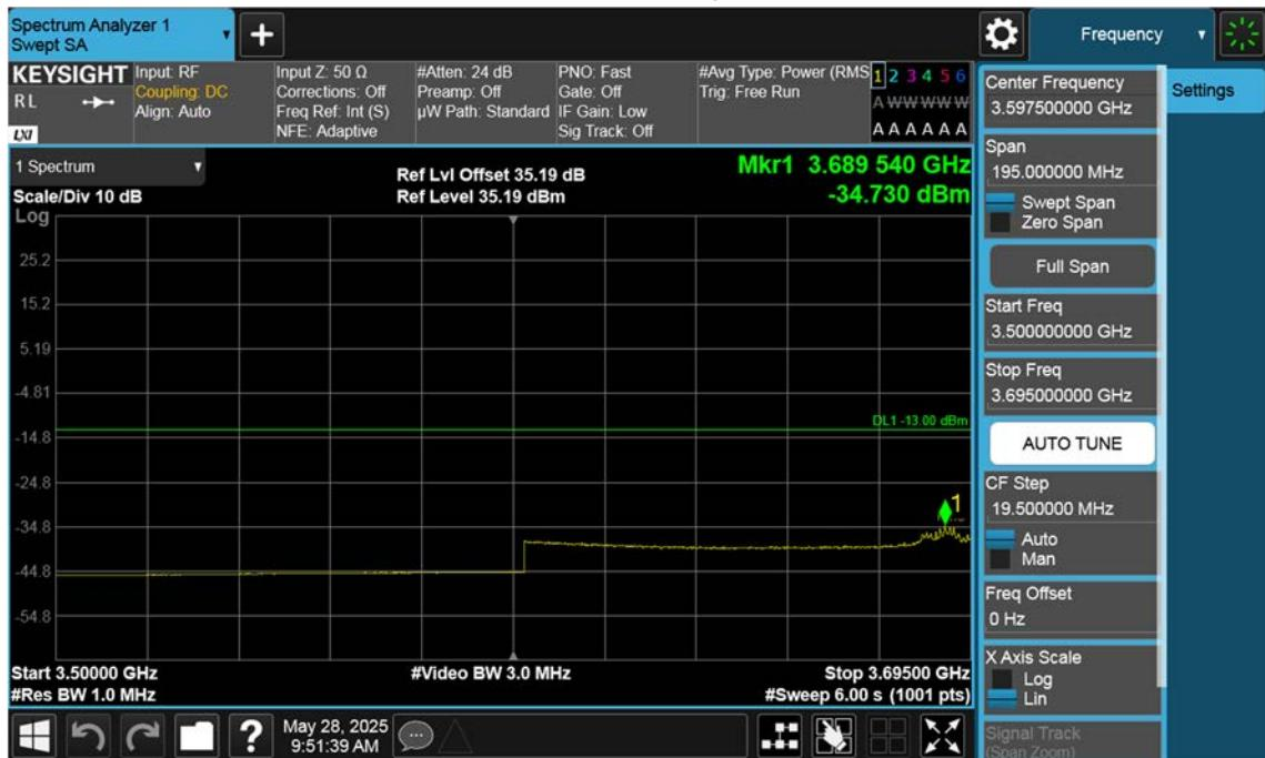
n77(3700~3980 MHz)\_25 M\_Band Edge\_Low\_BPSK\_1RB(3)
