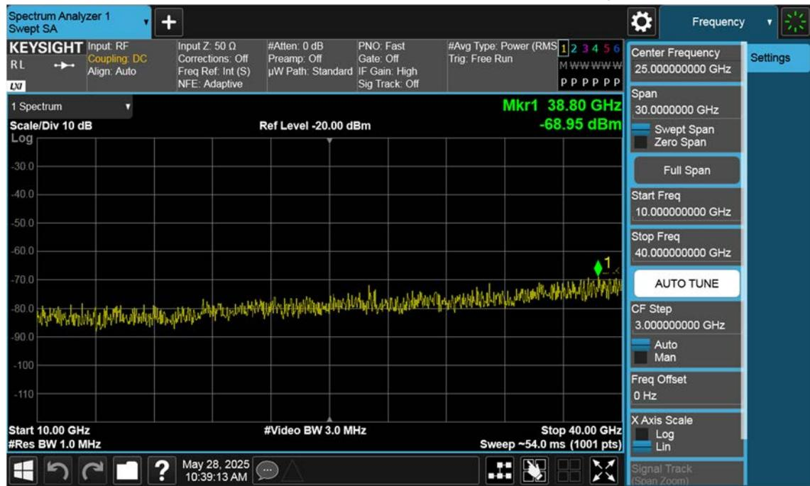
n77(3700~3980 MHz)\_60 M\_Conducted Spurious(Above10 G)\_Low\_BPSK\_1RB
