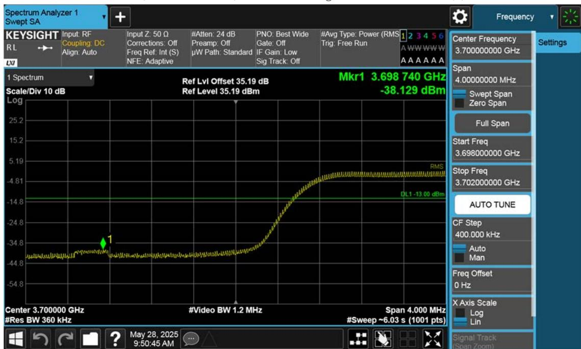
n77(3700~3980 MHz)\_25 M\_Band Edge\_Low\_BPSK\_1RB(1)
