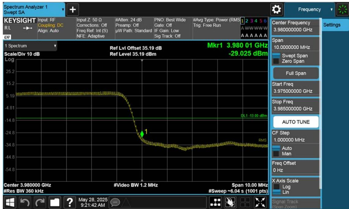
n77(3700~3980 MHz)\_10 M\_Band Edge\_High\_BPSK\_1RB(1)
