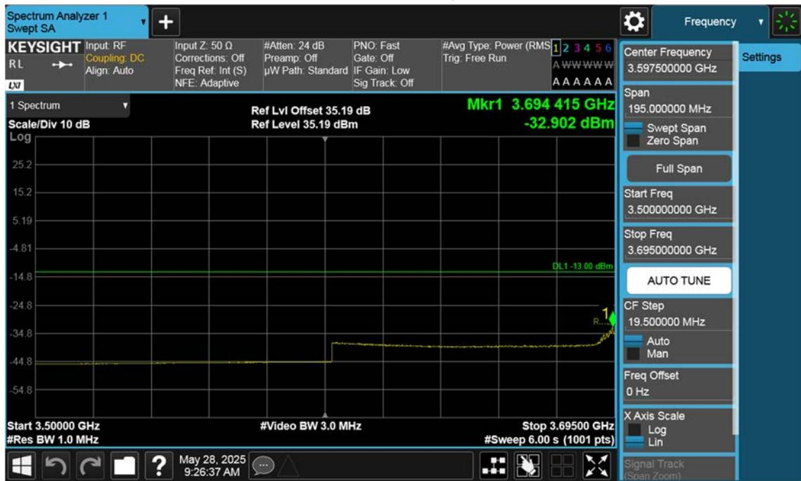
n77(3700~3980 MHz)\_15 M\_Band Edge\_Low\_BPSK\_1RB(3)
