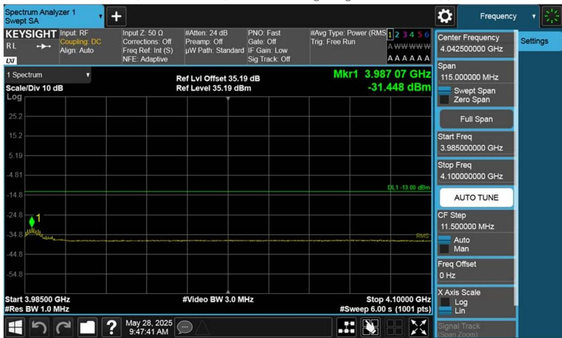
n77(3700~3980 MHz)\_20 M\_Band Edge\_High\_BPSK\_1RB(3)
