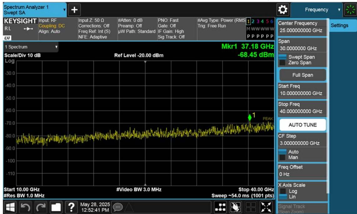
n77(3700~3980 MHz)\_100 M\_Conducted Spurious(Above10 G)\_Low\_BPSK\_1RB
