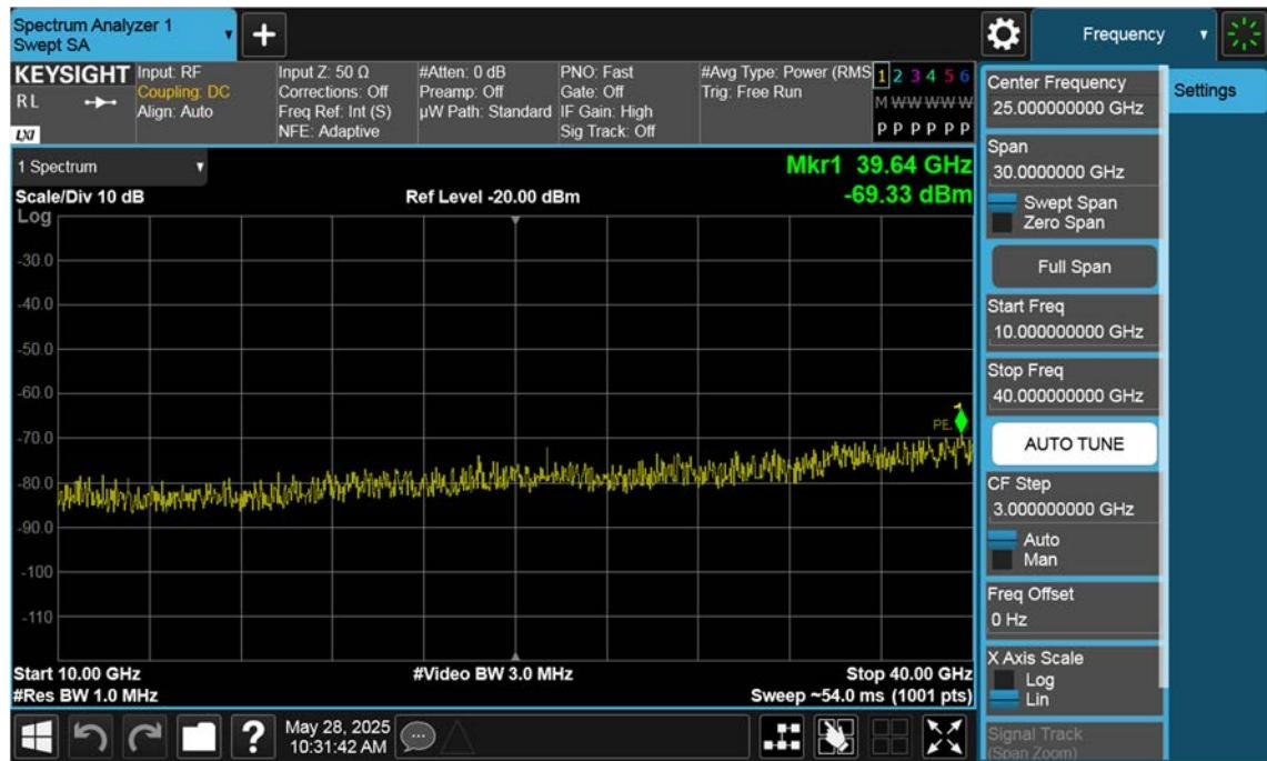
n77(3700~3980 MHz)\_50 M\_Conducted Spurious(Above10 G)\_Mid\_BPSK\_1RB
