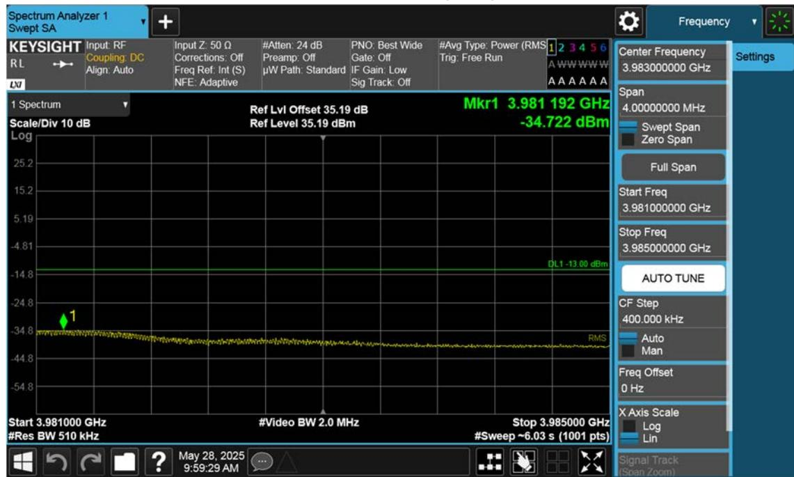
n77(3700~3980 MHz)\_25 M\_Band Edge\_High\_BPSK\_1RB(2)
