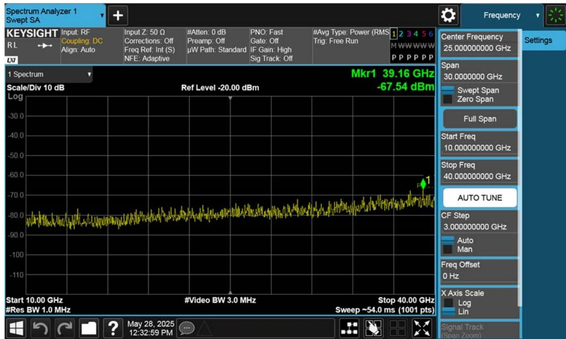
n77(3700~3980 MHz)\_80 M\_Conducted Spurious(Above10 G)\_Mid\_BPSK\_1RB
