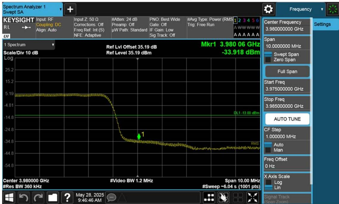
n77(3700~3980 MHz)\_20 M\_Band Edge\_High\_BPSK\_1RB(1)
