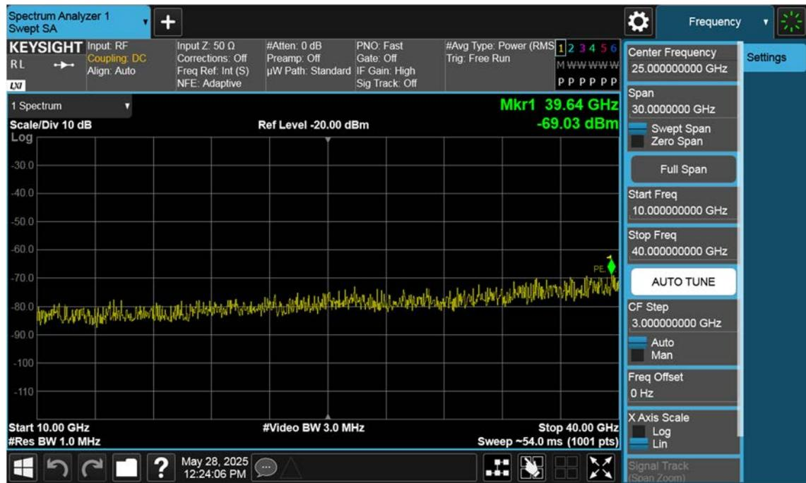
n77(3700~3980 MHz)\_70 M\_Conducted Spurious(Above10 G)\_High\_BPSK\_1RB
