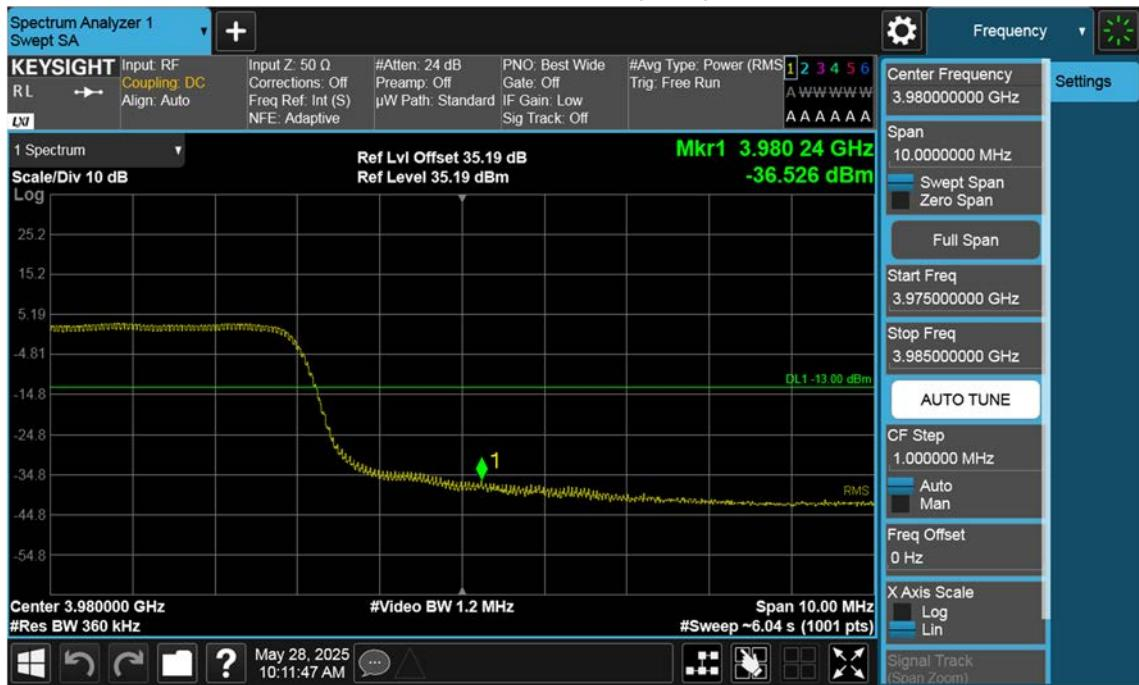
n77(3700~3980 MHz)\_30 M\_Band Edge\_High\_BPSK\_1RB(1)
