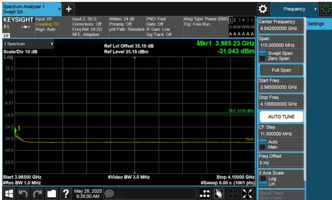
n77(3700~3980 MHz)\_15 M\_Band Edge\_High\_BPSK\_1RB(3)
