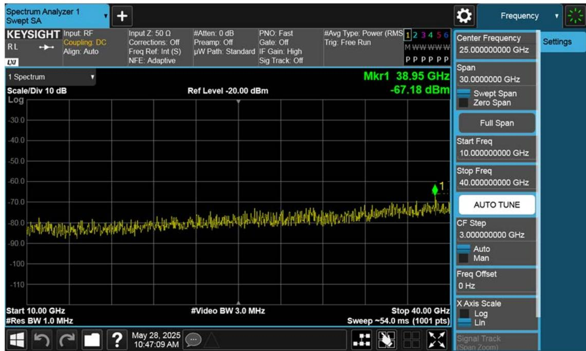
n77(3700~3980 MHz)\_60 M\_Conducted Spurious(Above10 G)\_High\_BPSK\_1RB
