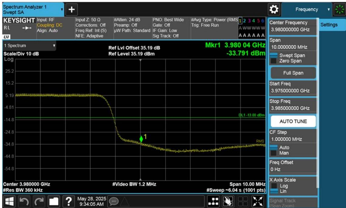
n77(3700~3980 MHz)\_15 M\_Band Edge\_High\_BPSK\_1RB(1)
