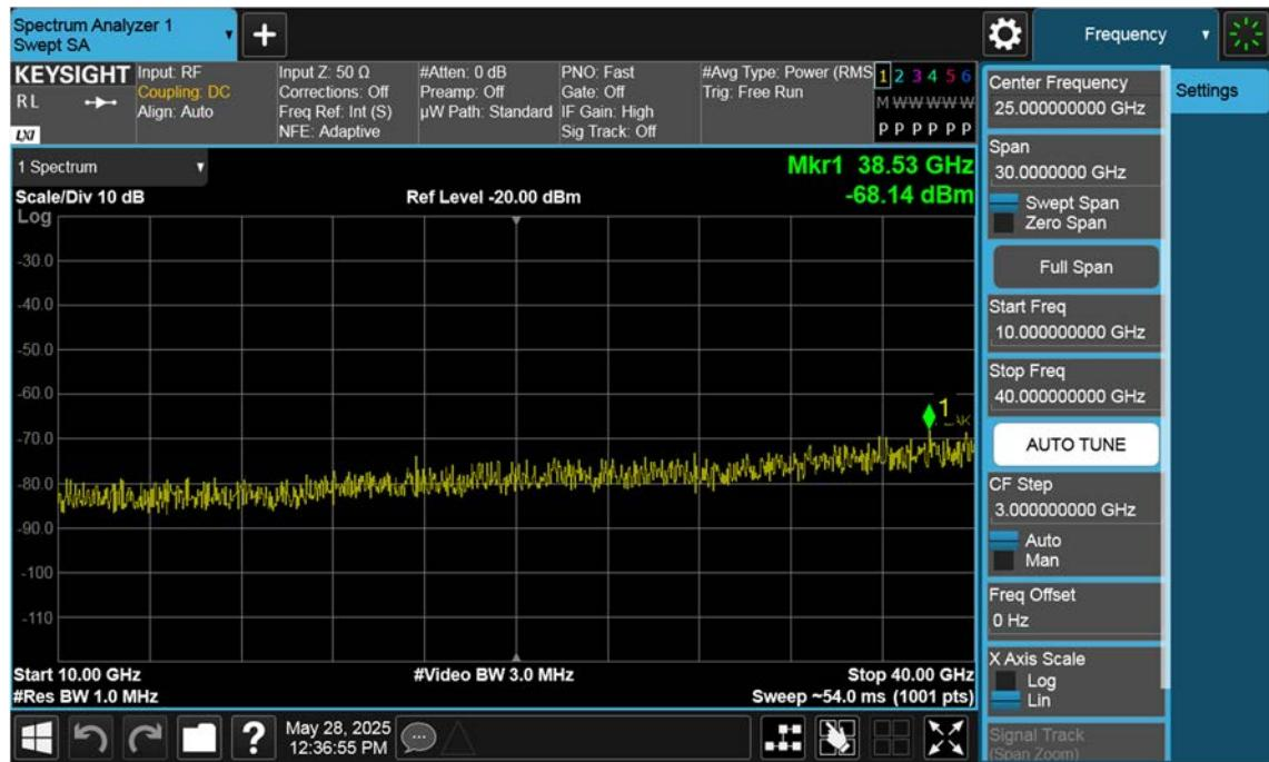
n77(3700~3980 MHz)\_80 M\_Conducted Spurious(Above10 G)\_High\_BPSK\_1RB
