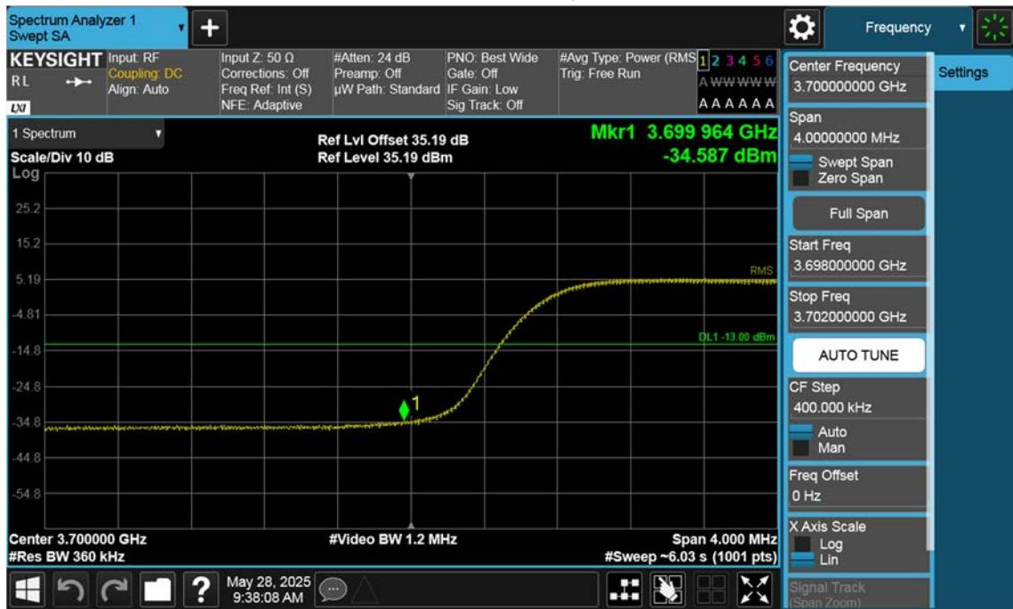
n77(3700~3980 MHz)\_20 M\_Band Edge\_Low\_BPSK\_1RB(1)
