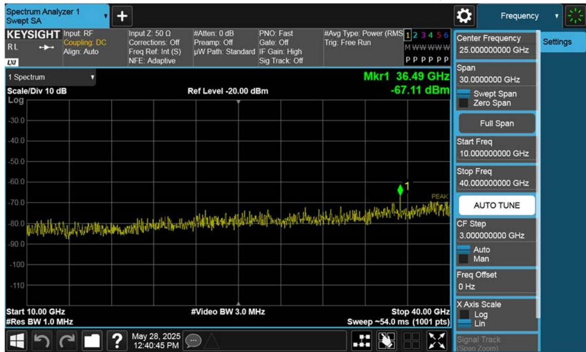
n77(3700~3980 MHz)\_90 M\_Conducted Spurious(Above10 G)\_Low\_BPSK\_1RB
