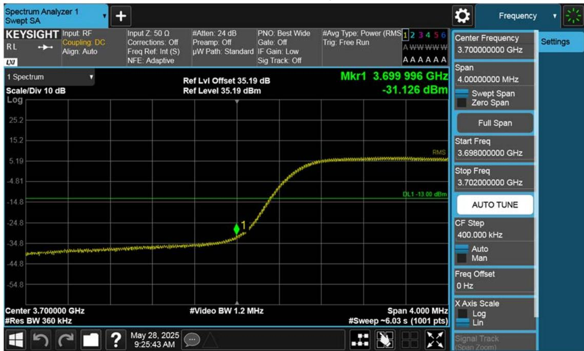
n77(3700~3980 MHz)\_15 M\_Band Edge\_Low\_BPSK\_1RB(1)
