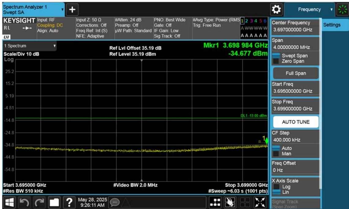
n77(3700~3980 MHz)\_15 M\_Band Edge\_Low\_BPSK\_1RB(2)
