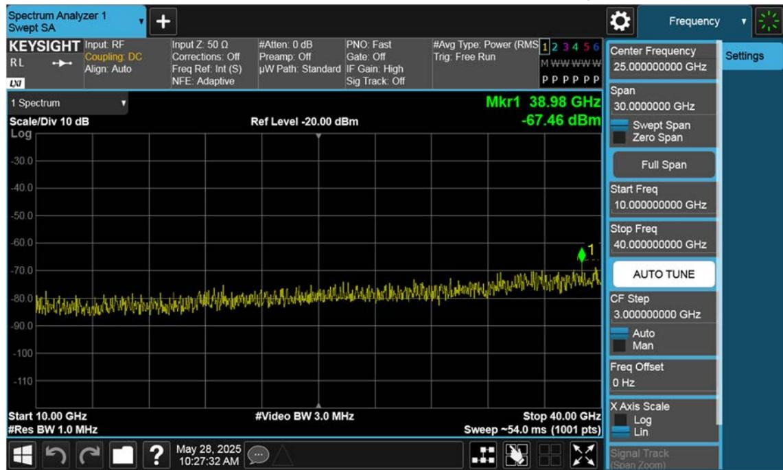
n77(3700~3980 MHz)\_50 M\_Conducted Spurious(Above10 G)\_Low\_BPSK\_1RB
