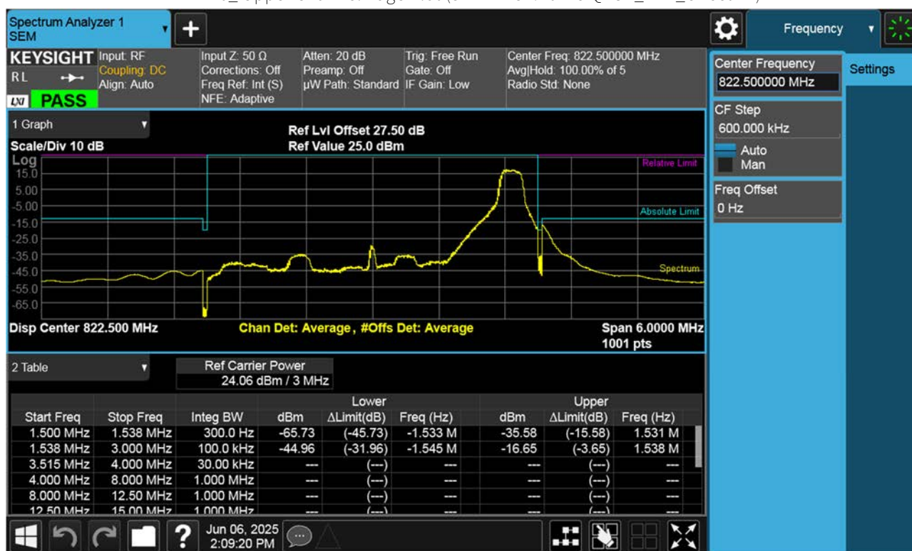
LTE B26_ Upper Channel Edge Plot (3 M BW Ch.26775 QPSK_RB1_Offset 14)
