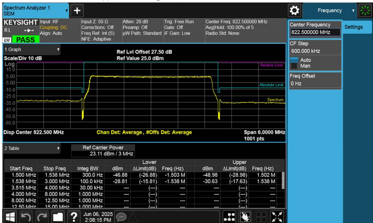
LTE B26_ Upper Channel Edge Plot (3 M BW Ch.26775 QPSK_RB15_Offset 0)
