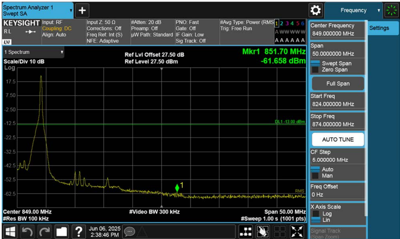
LTE B26_Mid Band Edge Plot (15 M BW Ch.26765 QPSK RB 1, Offset74)
