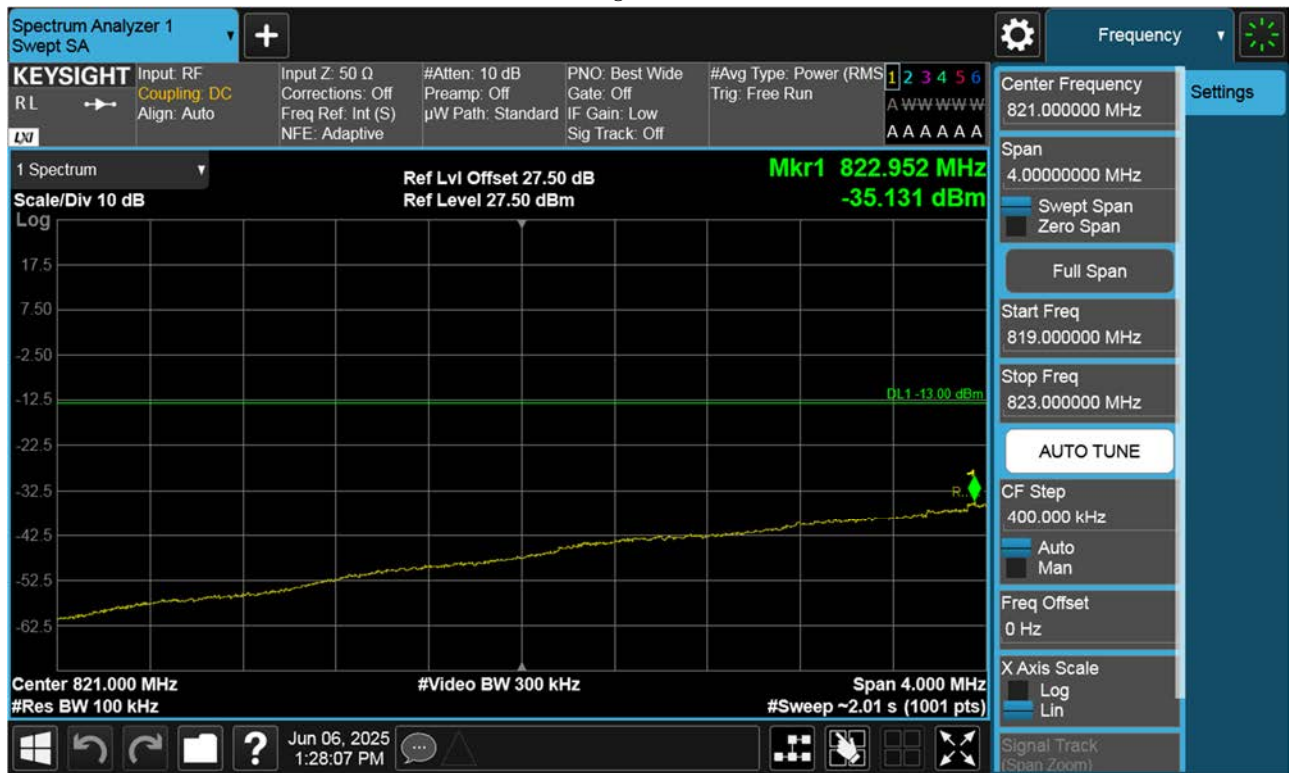
LTE B26_ Lower Extended Band Edge Plot (1.4 M BW Ch.26797 QPSK_RB6_0)
