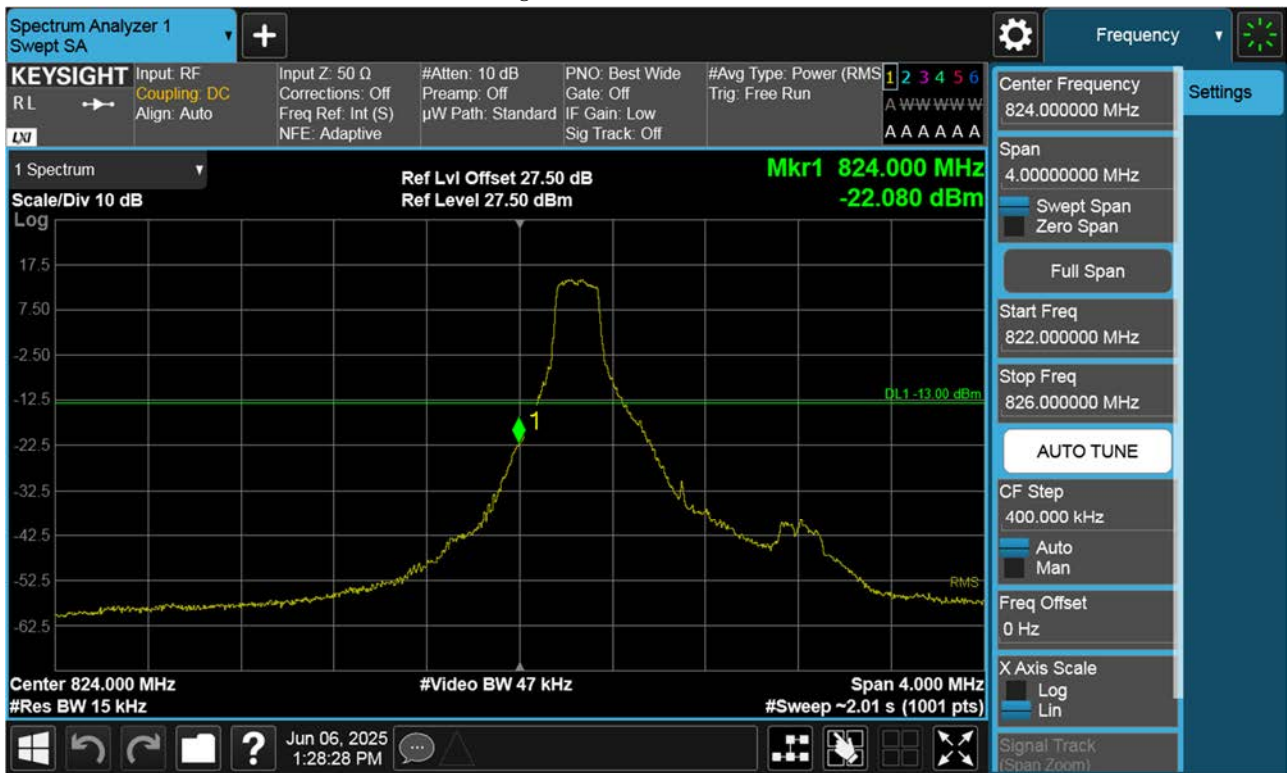
LTE B26_ Lower Band Edge Plot (1.4 M BW Ch.26797 QPSK_RB1_Offset 0)
