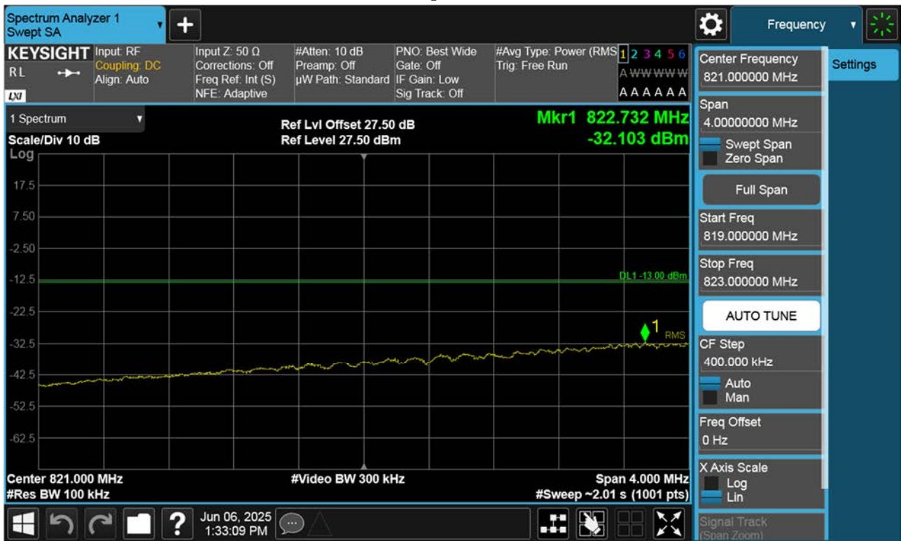
LTE B26_ Lower Extended Band Edge Plot (3 M BW Ch.26805 QPSK_RB15_0)
