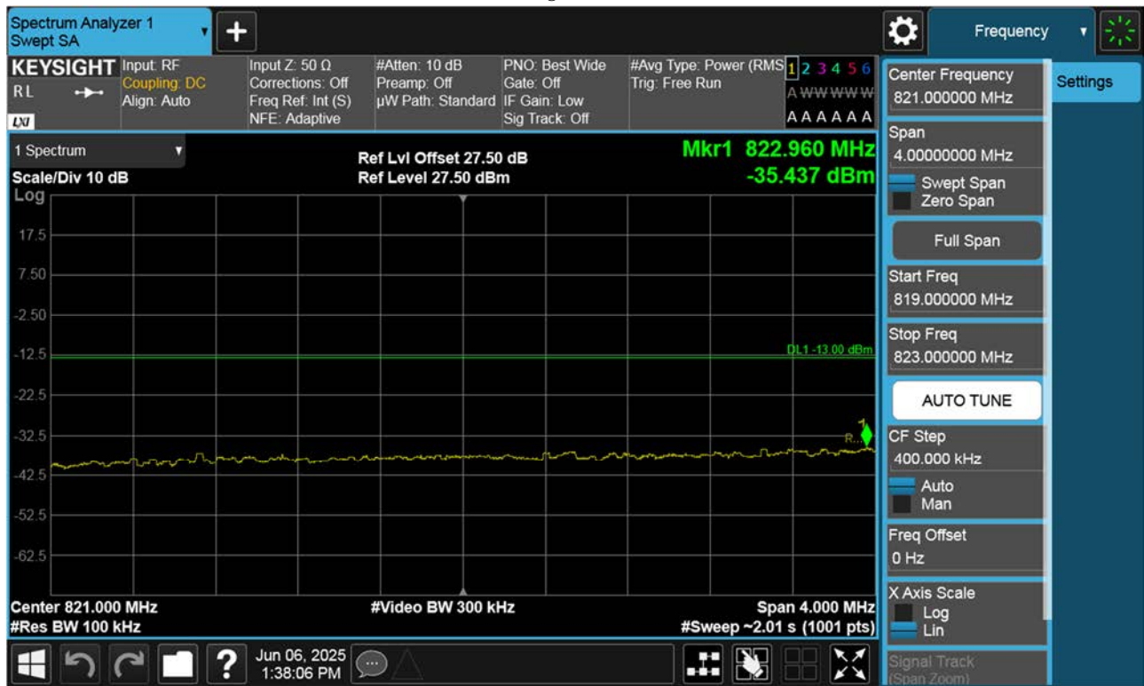
LTE B26_ Lower Extended Band Edge Plot (5 M BW Ch.26815 QPSK_RB25_0)
