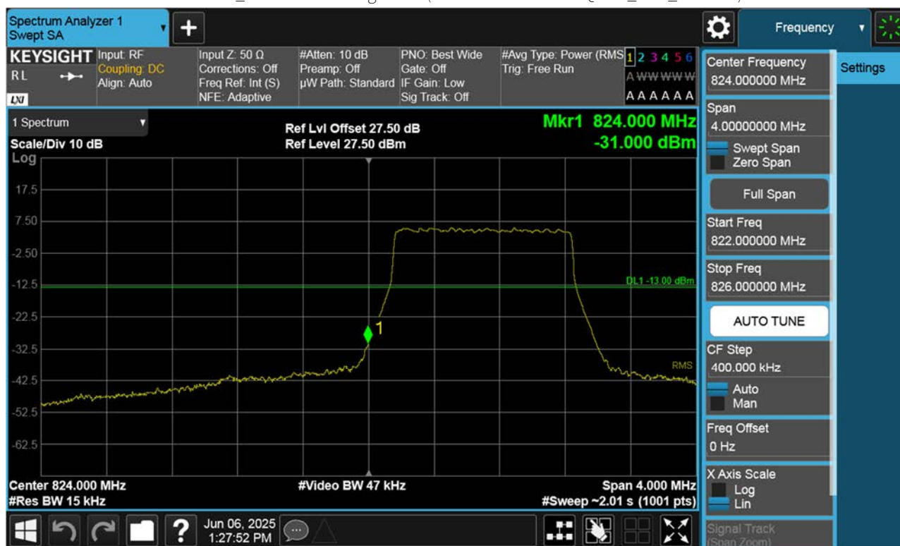
LTE B26_ Lower Band Edge Plot (1.4 M BW Ch.26797 QPSK_RB6_Offset 0)
