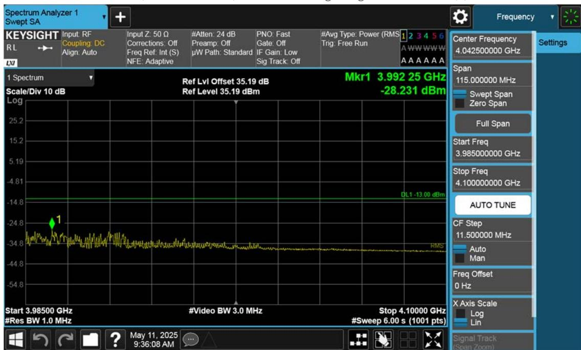
n77(3700~3980 MHz)\_70 M\_Band Edge\_High\_BPSK\_1RB(3)
