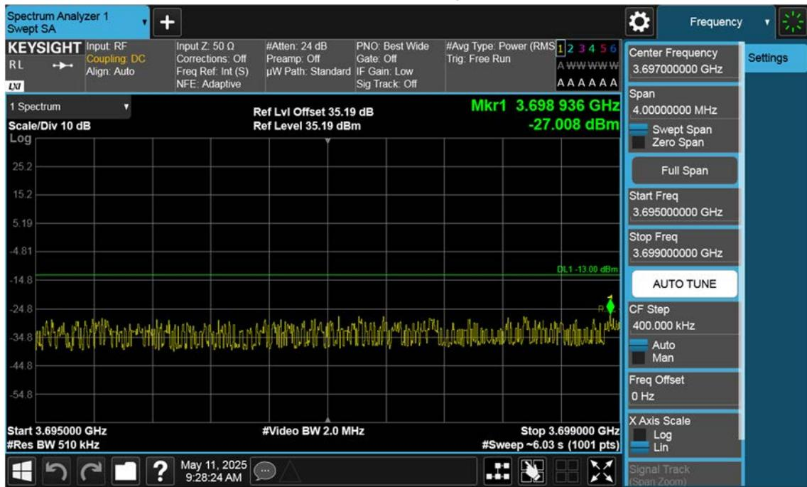
n77(3700~3980 MHz)\_70 M\_Band Edge\_Low\_BPSK\_1RB(2)
