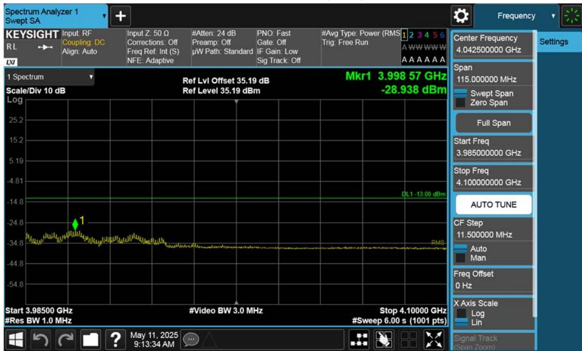
n77(3700~3980 MHz)\_50 M\_Band Edge\_High\_BPSK\_1RB(3)
