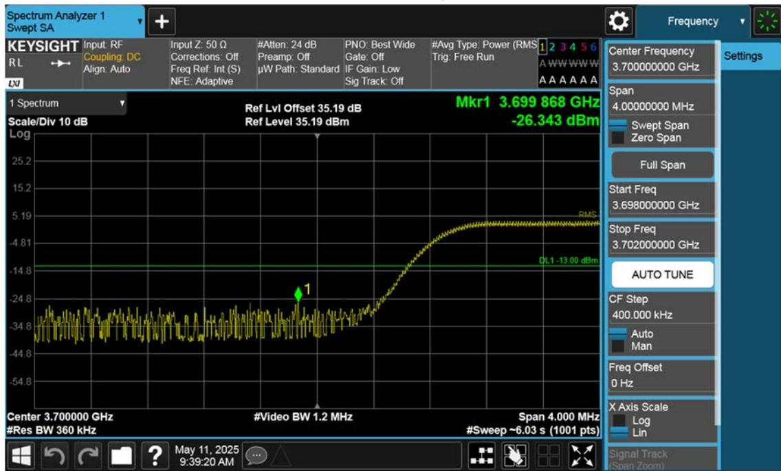
n77(3700~3980 MHz)\_80 M\_Band Edge\_Low\_BPSK\_1RB(1)
