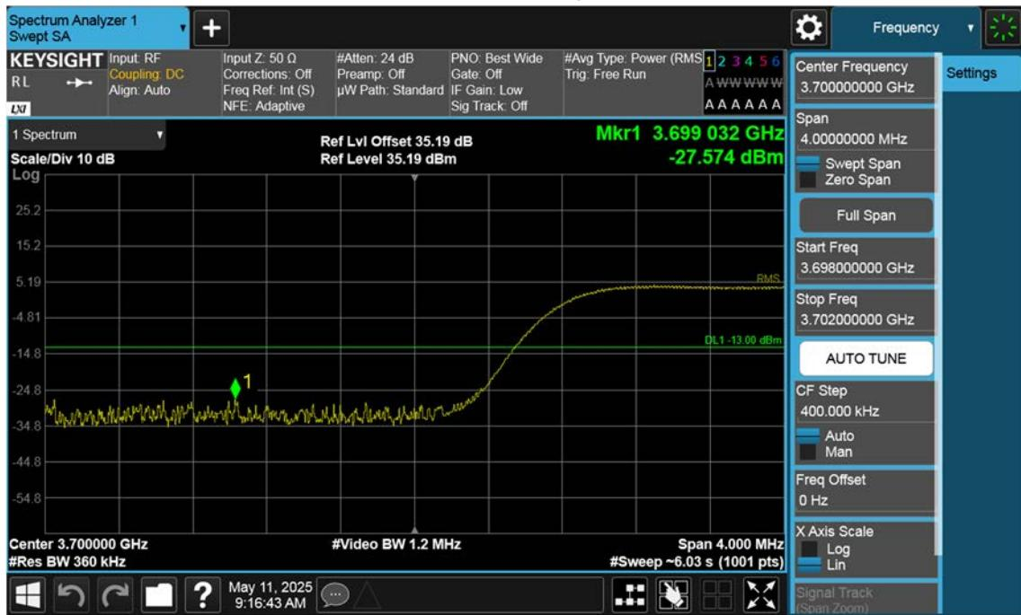
n77(3700~3980 MHz)\_60 M\_Band Edge\_Low\_BPSK\_1RB(1)
