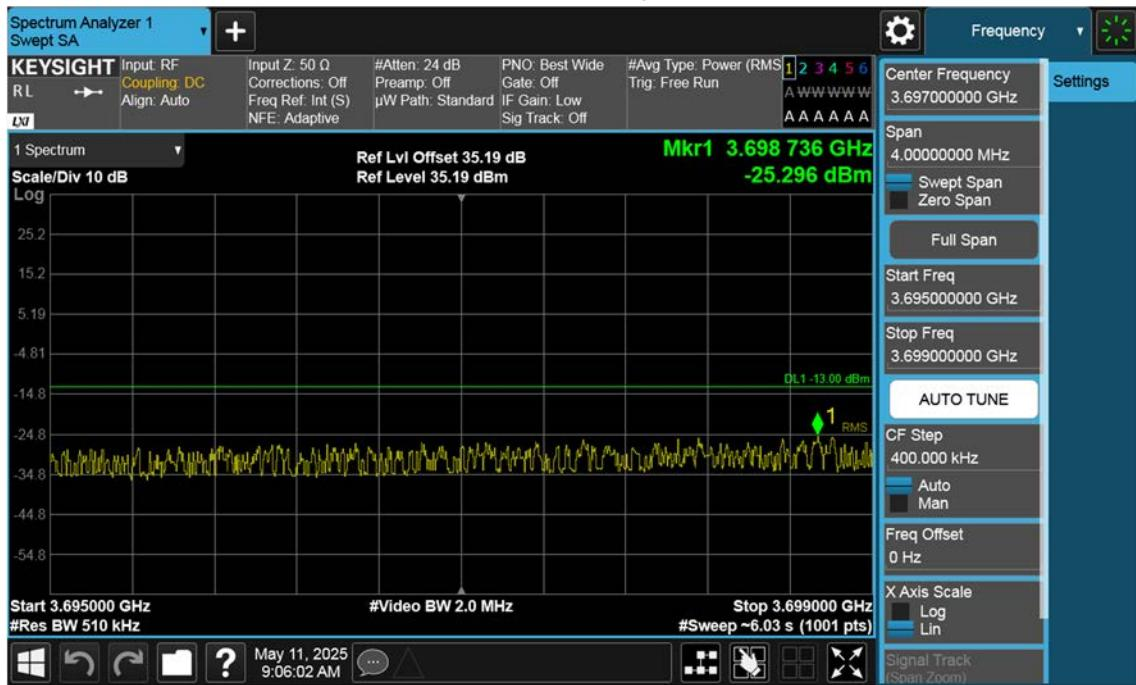
n77(3700~3980 MHz)\_50 M\_Band Edge\_Low\_BPSK\_1RB(2)
