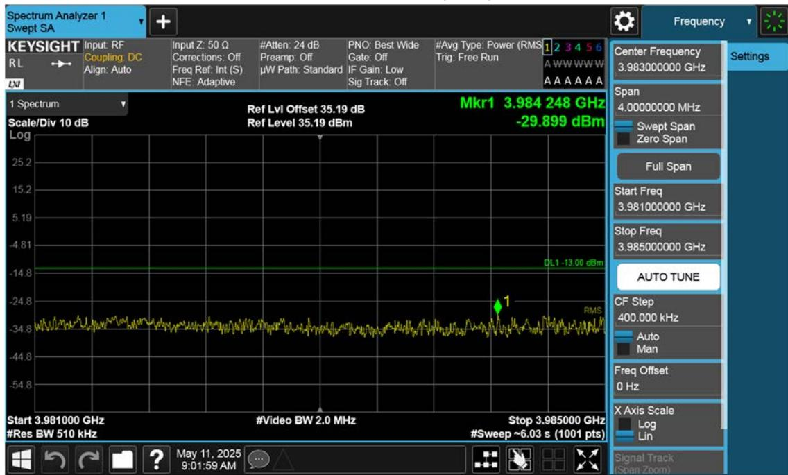
n77(3700~3980 MHz)\_40 M\_Band Edge\_High\_BPSK\_1RB(2)
