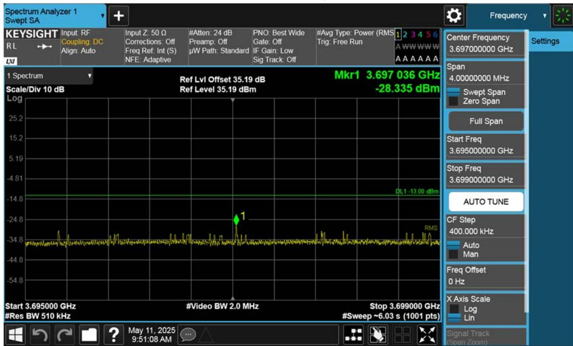
n77(3700~3980 MHz)\_90 M\_Band Edge\_Low\_BPSK\_1RB(2)
