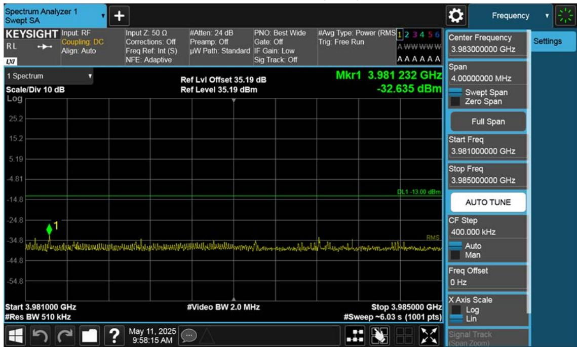
n77(3700~3980 MHz)\_90 M\_Band Edge\_High\_BPSK\_1RB(2)
