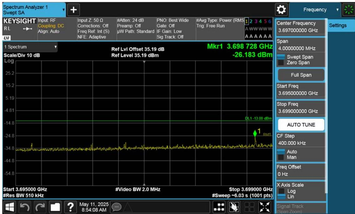
n77(3700~3980 MHz)\_40 M\_Band Edge\_Low\_BPSK\_1RB(2)
