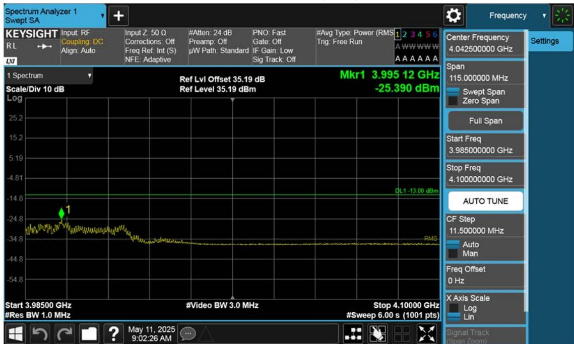
n77(3700~3980 MHz)\_40 M\_Band Edge\_High\_BPSK\_1RB(3)
