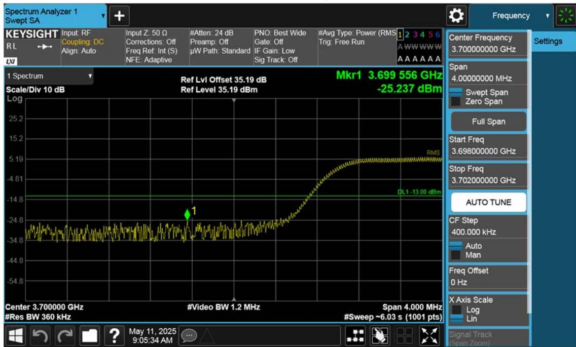
n77(3700~3980 MHz)\_50 M\_Band Edge\_Low\_BPSK\_1RB(1)
