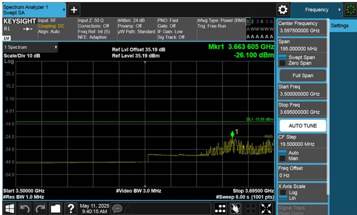
n77(3700~3980 MHz)\_80 M\_Band Edge\_Low\_BPSK\_1RB(3)
