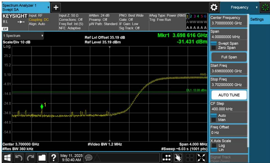
n77(3700~3980 MHz)\_90 M\_Band Edge\_Low\_BPSK\_1RB(1)
