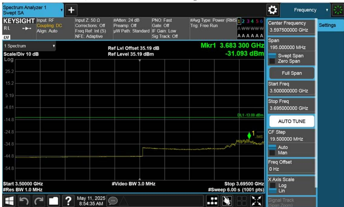
n77(3700~3980 MHz)\_40 M\_Band Edge\_Low\_BPSK\_1RB(3)
