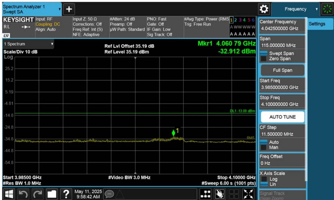
n77(3700~3980 MHz)\_90 M\_Band Edge\_High\_BPSK\_1RB(3)
