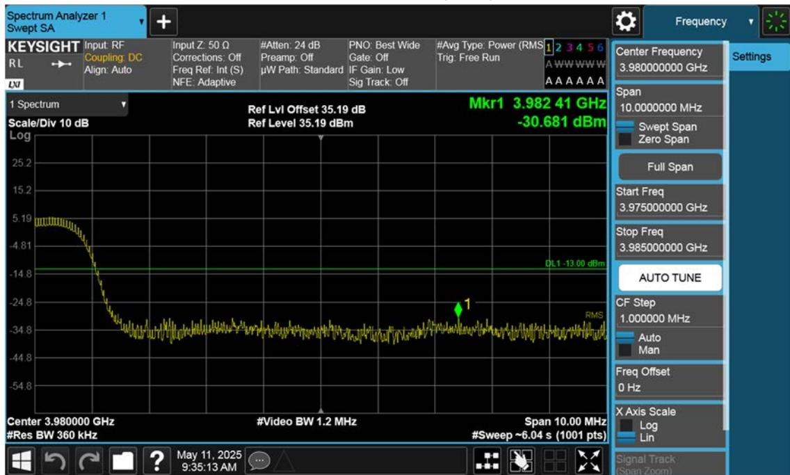
n77(3700~3980 MHz)\_70 M\_Band Edge\_High\_BPSK\_1RB(1)
