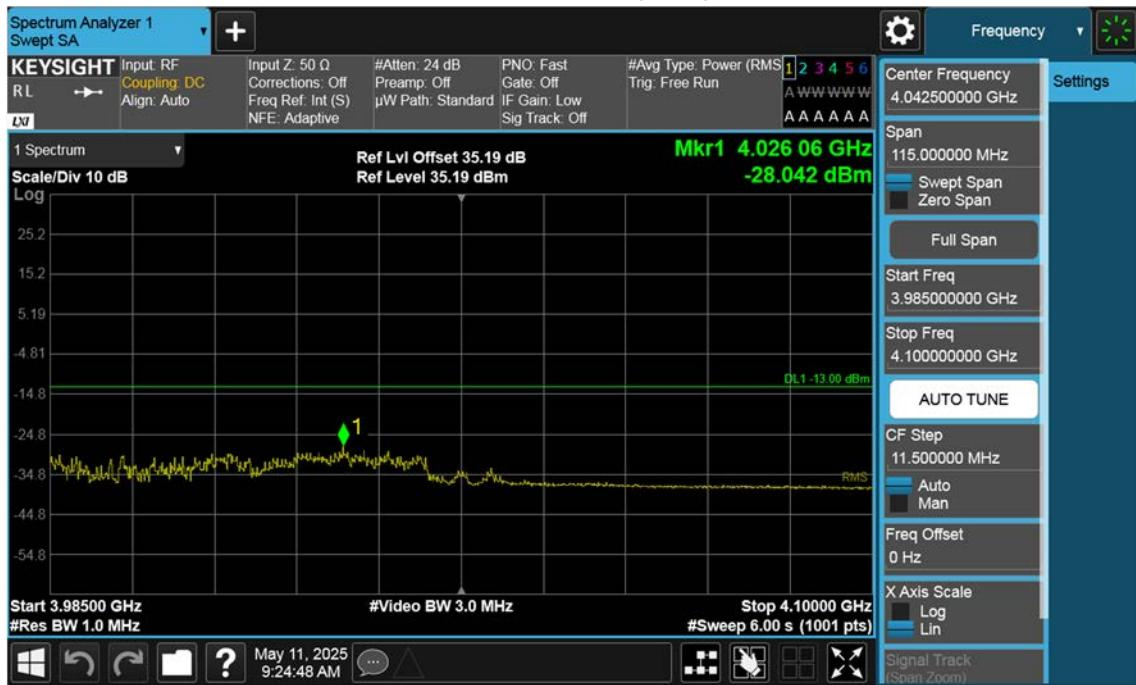
n77(3700~3980 MHz)\_60 M\_Band Edge\_High\_BPSK\_1RB(3)
