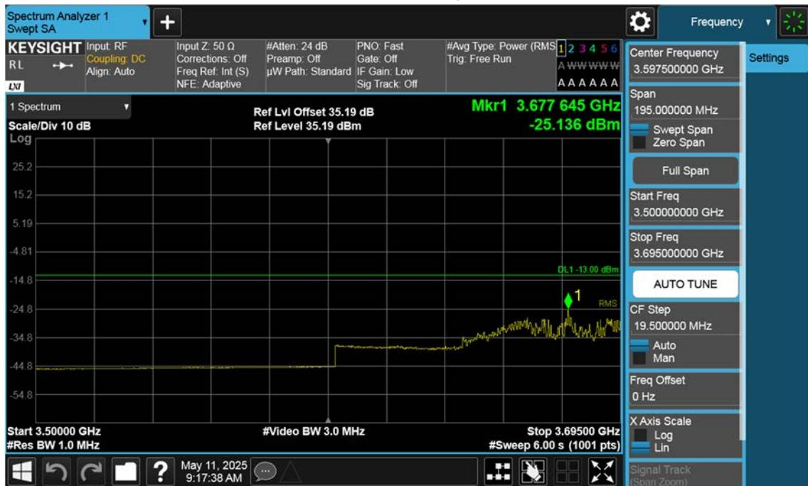
n77(3700~3980 MHz)\_60 M\_Band Edge\_Low\_BPSK\_1RB(3)
