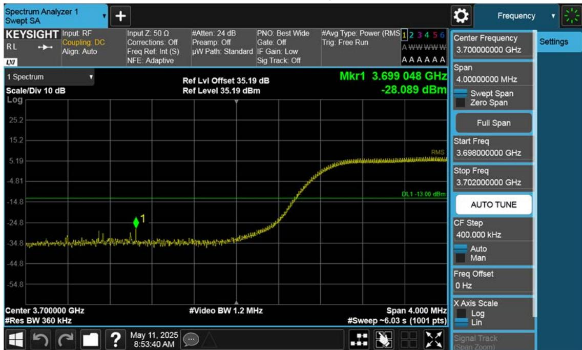
n77(3700~3980 MHz)\_40 M\_Band Edge\_Low\_BPSK\_1RB(1)
