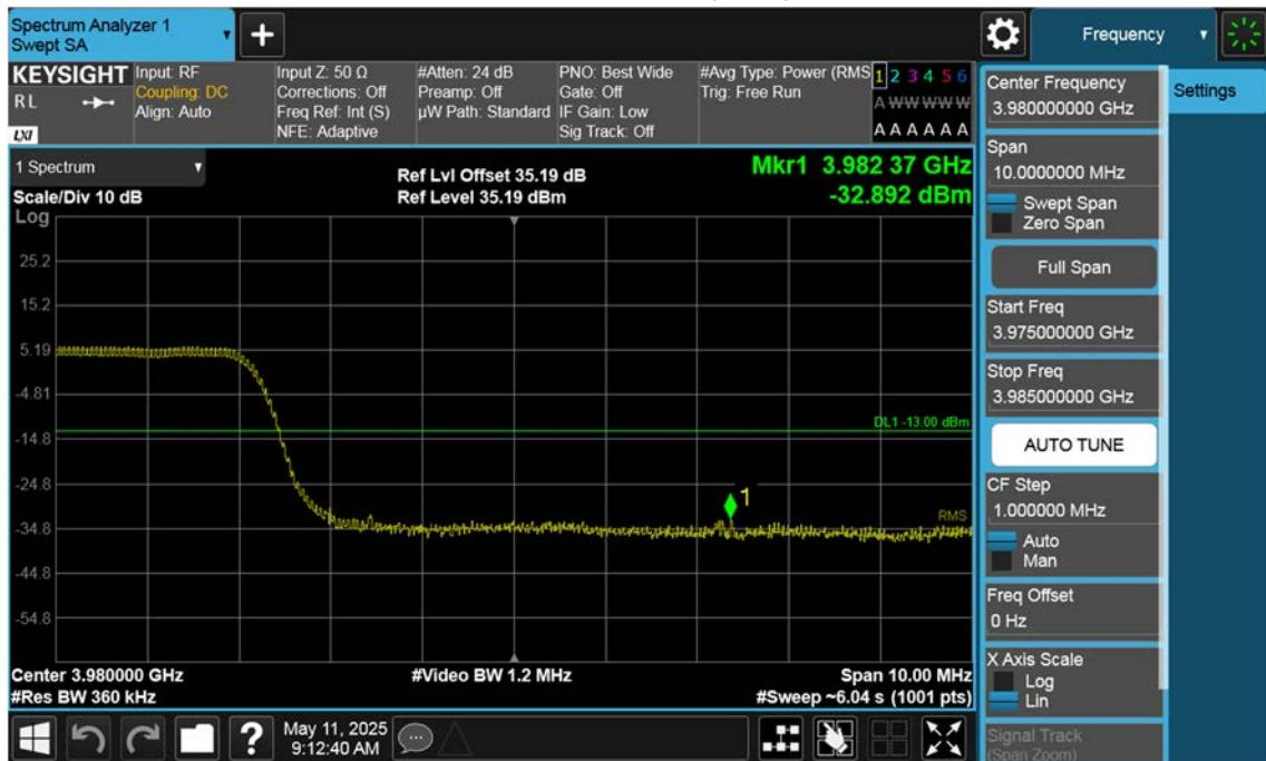
n77(3700~3980 MHz)\_50 M\_Band Edge\_High\_BPSK\_1RB(1)
