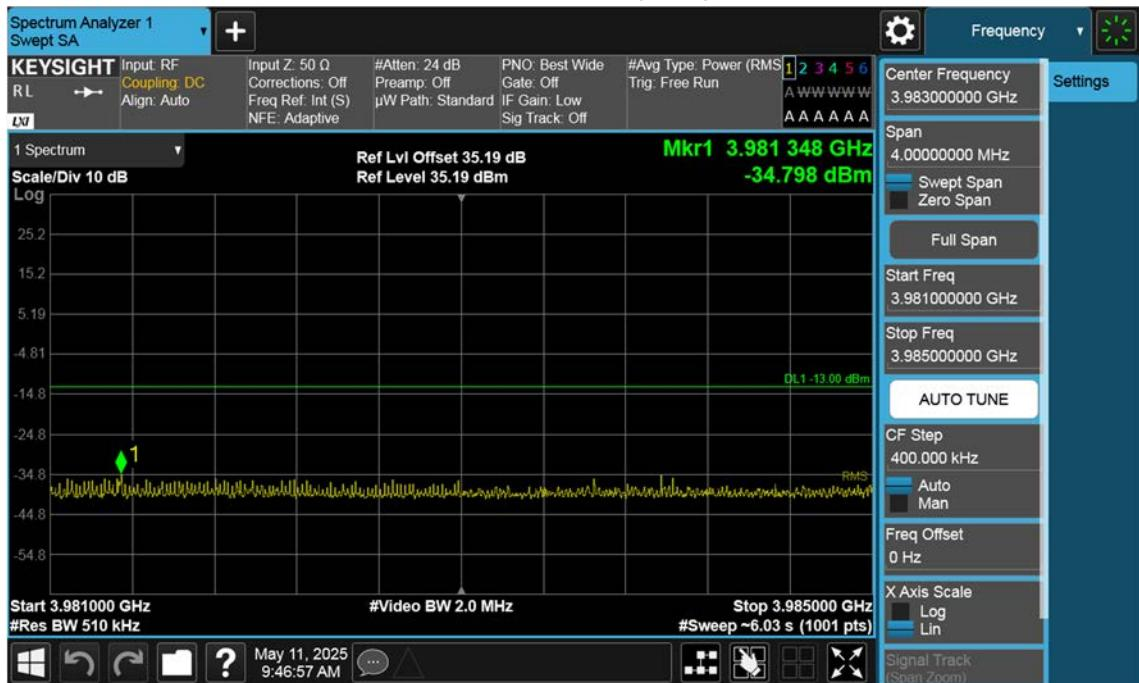
n77(3700~3980 MHz)\_80 M\_Band Edge\_High\_BPSK\_1RB(2)
