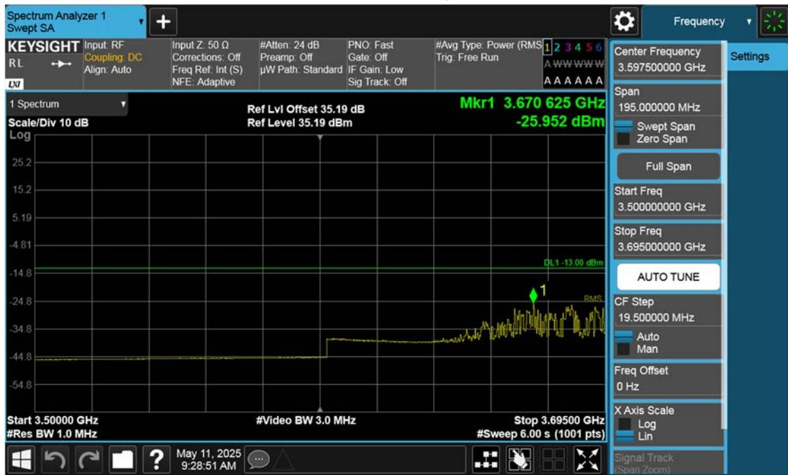
n77(3700~3980 MHz)\_70 M\_Band Edge\_Low\_BPSK\_1RB(3)
