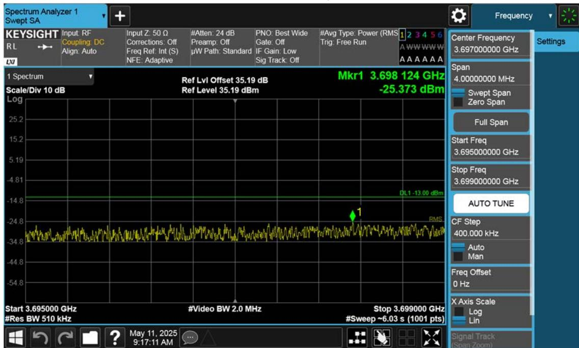
n77(3700~3980 MHz)\_60 M\_Band Edge\_Low\_BPSK\_1RB(2)
