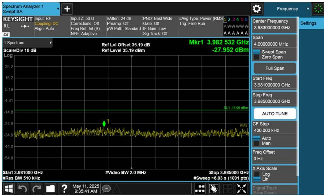
n77(3700~3980 MHz)\_70 M\_Band Edge\_High\_BPSK\_1RB(2)
