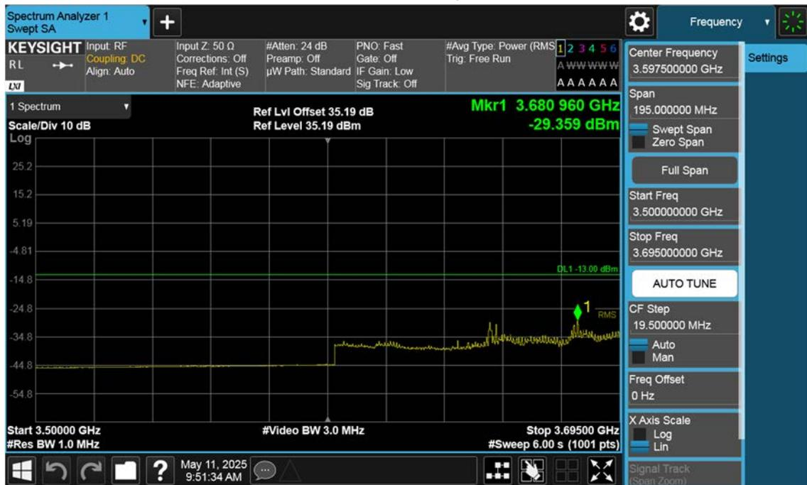
n77(3700~3980 MHz)\_90 M\_Band Edge\_Low\_BPSK\_1RB(3)
