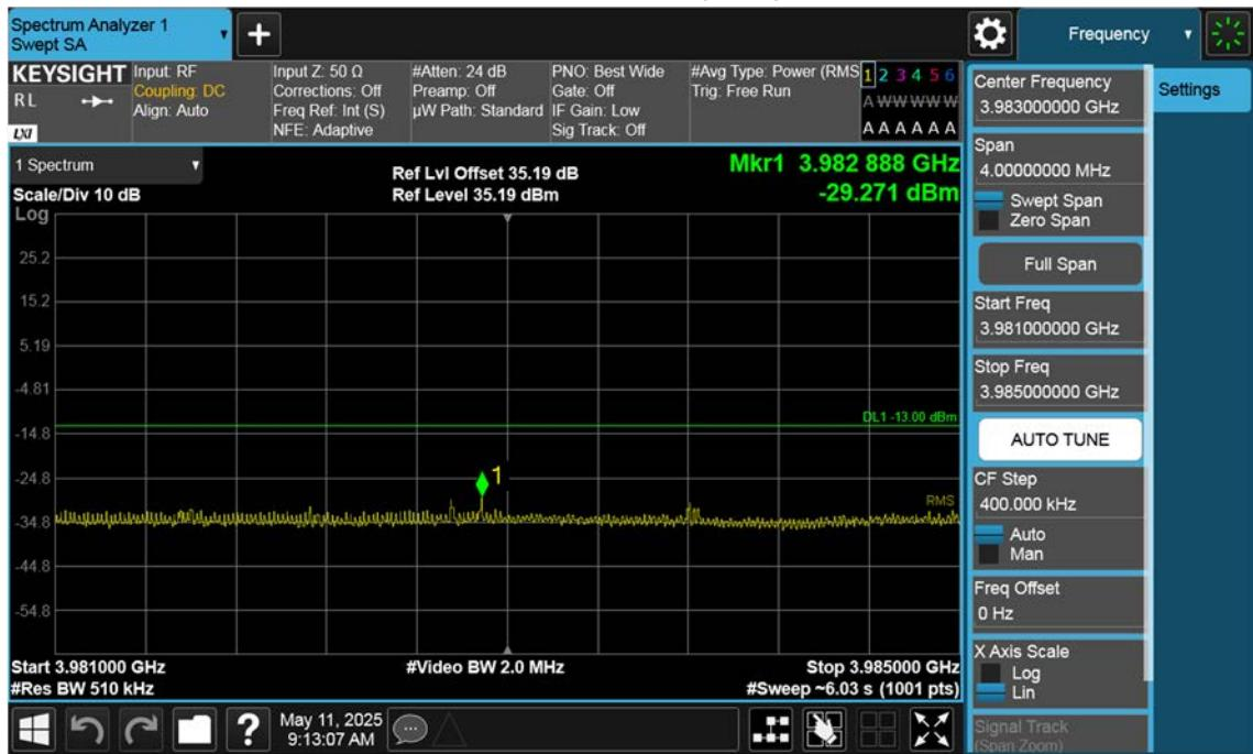
n77(3700~3980 MHz)\_50 M\_Band Edge\_High\_BPSK\_1RB(2)
