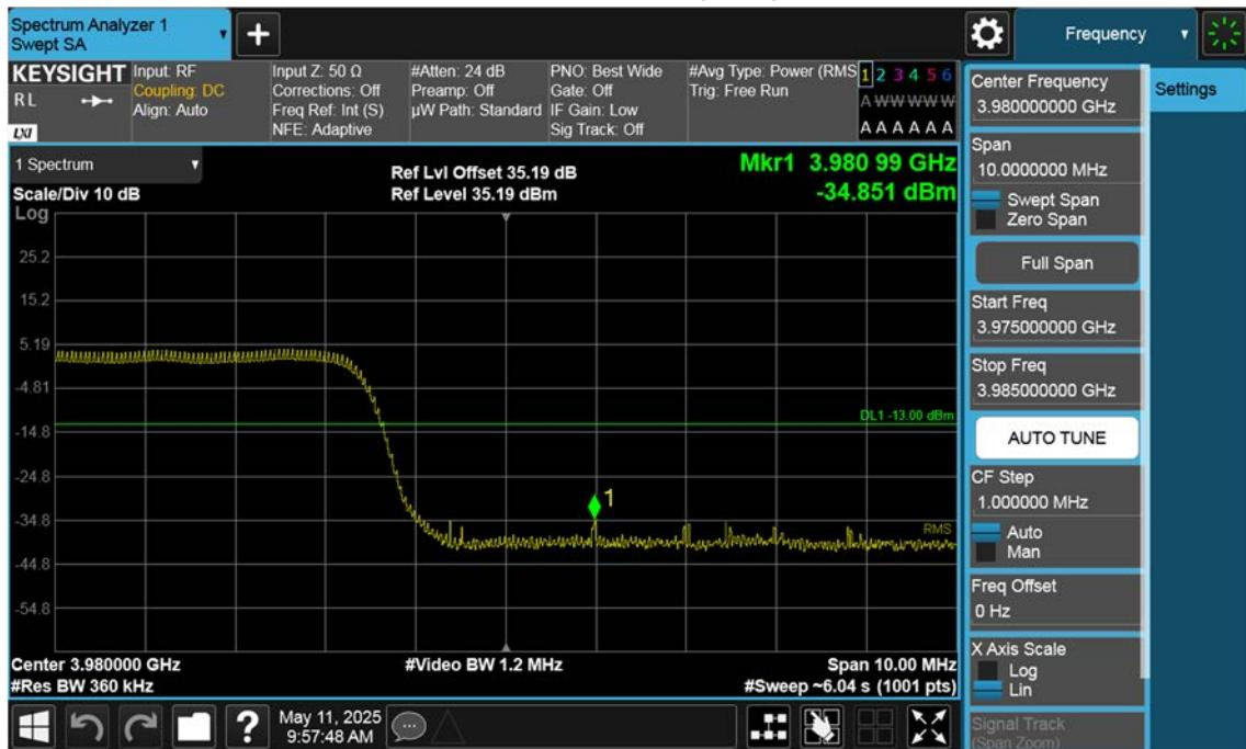
n77(3700~3980 MHz)\_90 M\_Band Edge\_High\_BPSK\_1RB(1)
