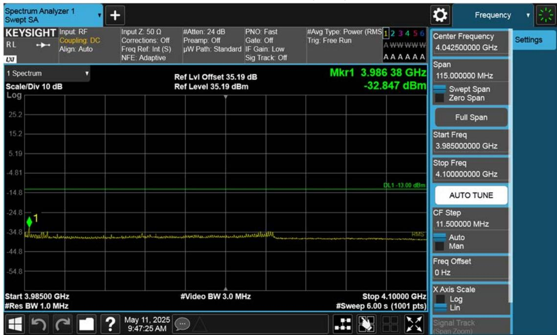
n77(3700~3980 MHz)\_80 M\_Band Edge\_High\_BPSK\_1RB(3)
