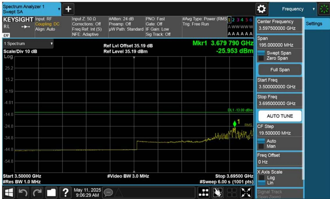
n77(3700~3980 MHz)\_50 M\_Band Edge\_Low\_BPSK\_1RB(3)
