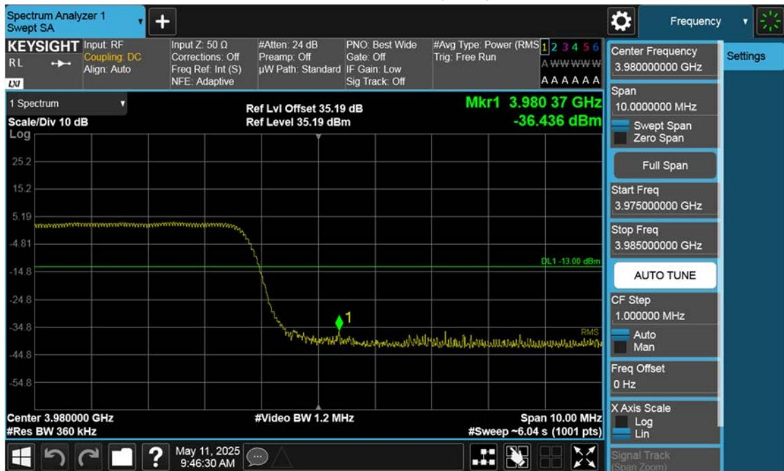
n77(3700~3980 MHz)\_80 M\_Band Edge\_High\_BPSK\_1RB(1)
