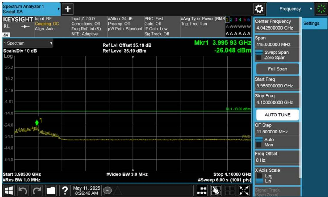
n77(3700~3980 MHz)\_20 M\_Band Edge\_High\_BPSK\_1RB(3)
