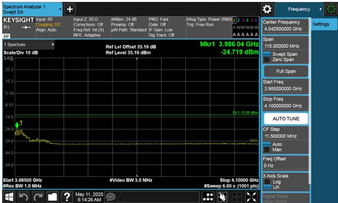
n77(3700~3980 MHz)\_15 M\_Band Edge\_High\_BPSK\_1RB(3)
