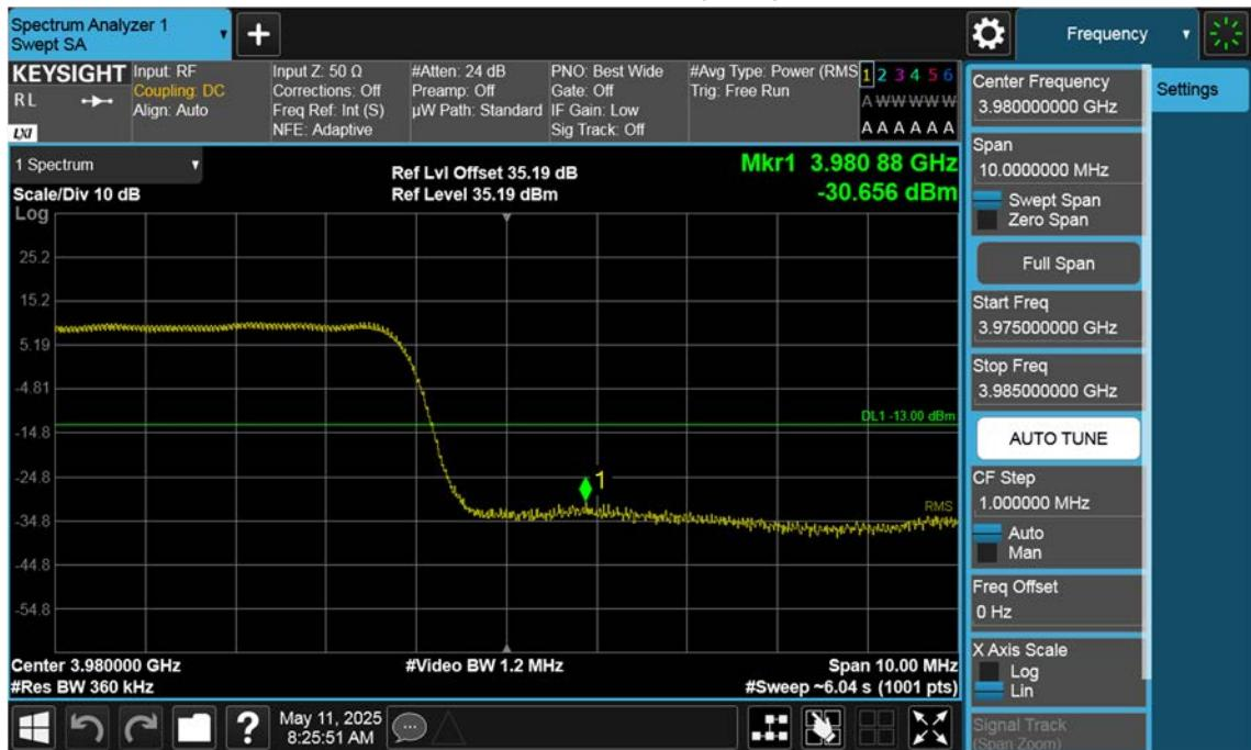
n77(3700~3980 MHz)\_20 M\_Band Edge\_High\_BPSK\_1RB(1)
