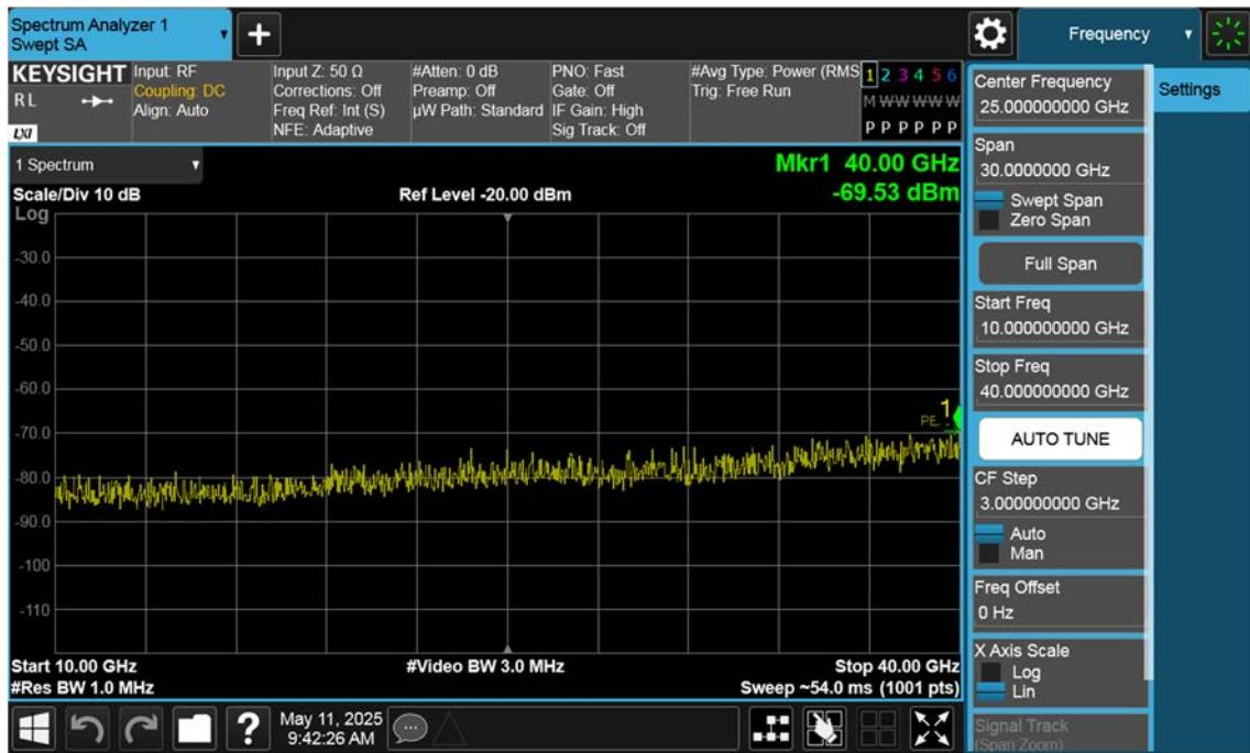
n77(3700~3980 MHz)\_80 M\_Conducted Spurious(Above10 G)\_Mid\_BPSK\_1RB
