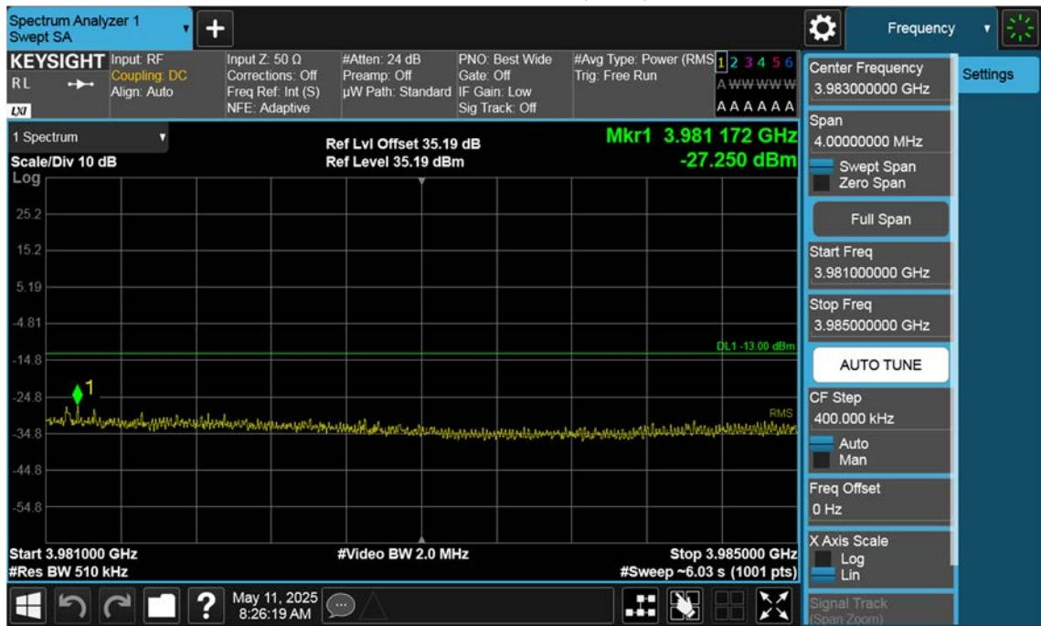
n77(3700~3980 MHz)\_20 M\_Band Edge\_High\_BPSK\_1RB(2)
