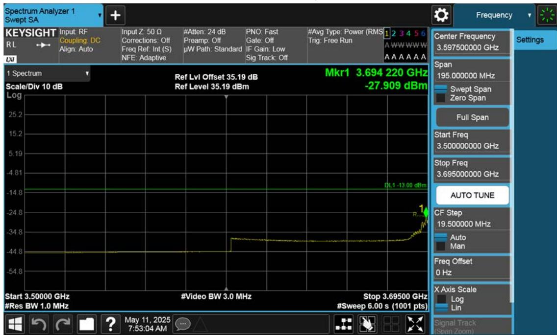
n77(3700~3980 MHz)\_10 M\_Band Edge\_Low\_BPSK\_1RB(3)
