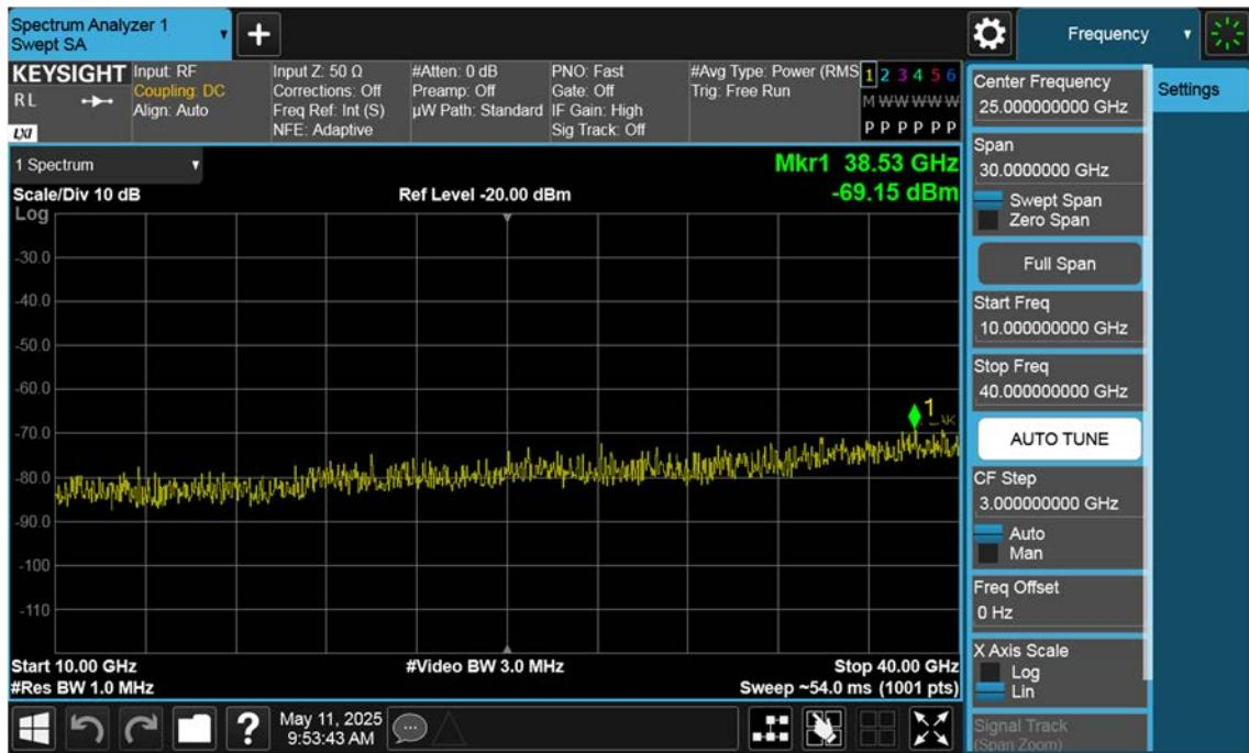
n77(3700~3980 MHz)\_90 M\_Conducted Spurious(Above10 G)\_Mid\_BPSK\_1RB
