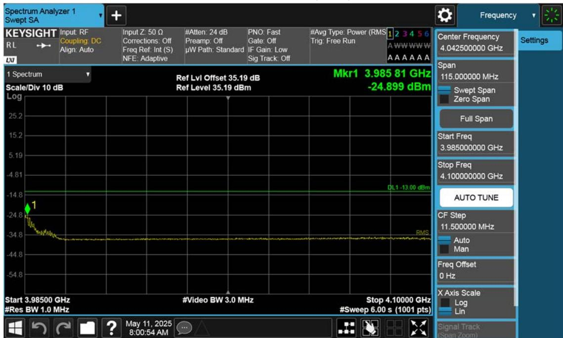
n77(3700~3980 MHz)\_10 M\_Band Edge\_High\_BPSK\_1RB(3)
