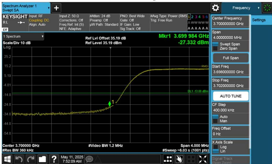
n77(3700~3980 MHz)\_10 M\_Band Edge\_Low\_BPSK\_1RB(1)
