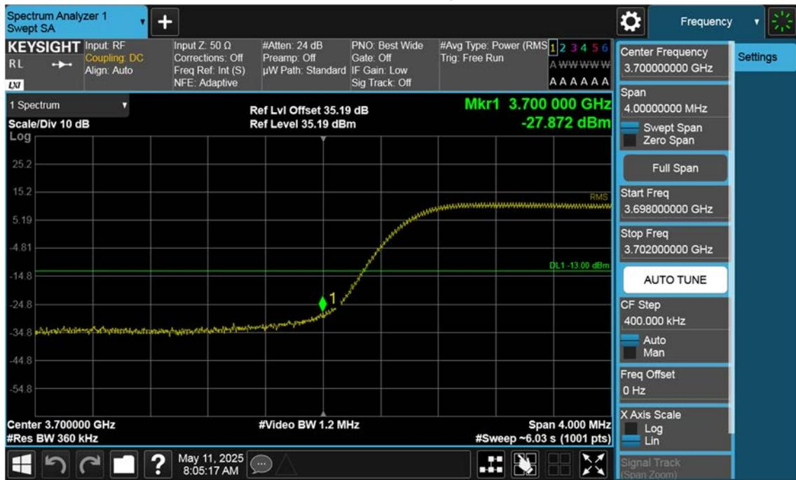
n77(3700~3980 MHz)\_15 M\_Band Edge\_Low\_BPSK\_1RB(1)
