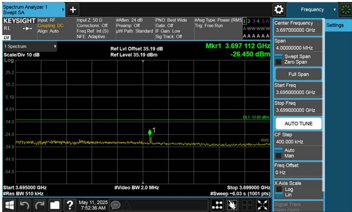
n77(3700~3980 MHz)\_10 M\_Band Edge\_Low\_BPSK\_1RB(2)
