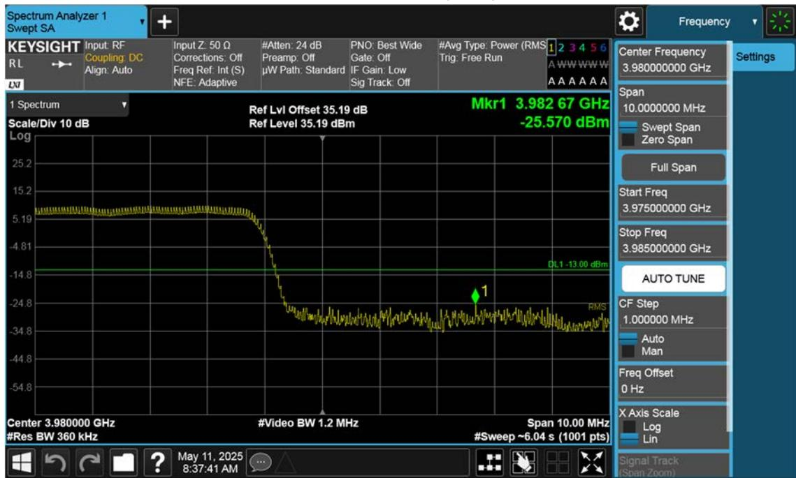
n77(3700~3980 MHz)\_25 M\_Band Edge\_High\_BPSK\_1RB(1)
