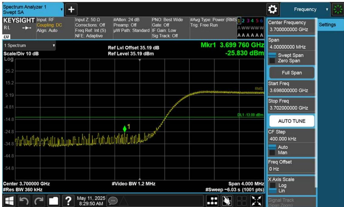
n77(3700~3980 MHz)\_25 M\_Band Edge\_Low\_BPSK\_1RB(1)
