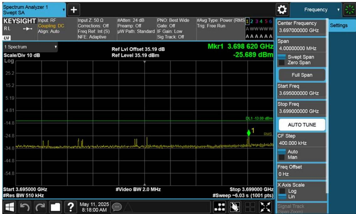
n77(3700~3980 MHz)\_20 M\_Band Edge\_Low\_BPSK\_1RB(2)
