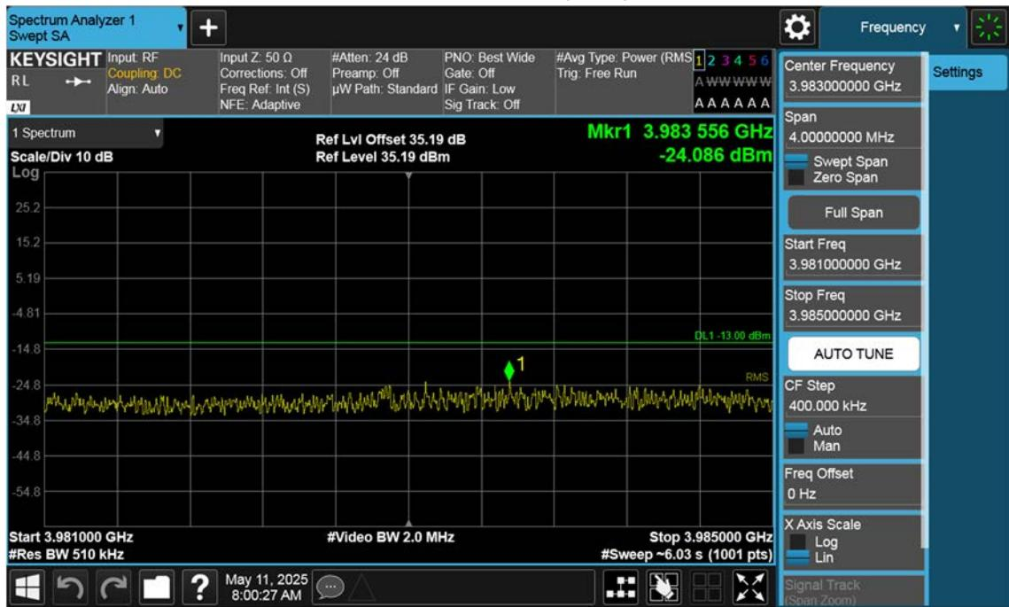
n77(3700~3980 MHz)\_10 M\_Band Edge\_High\_BPSK\_1RB(2)
