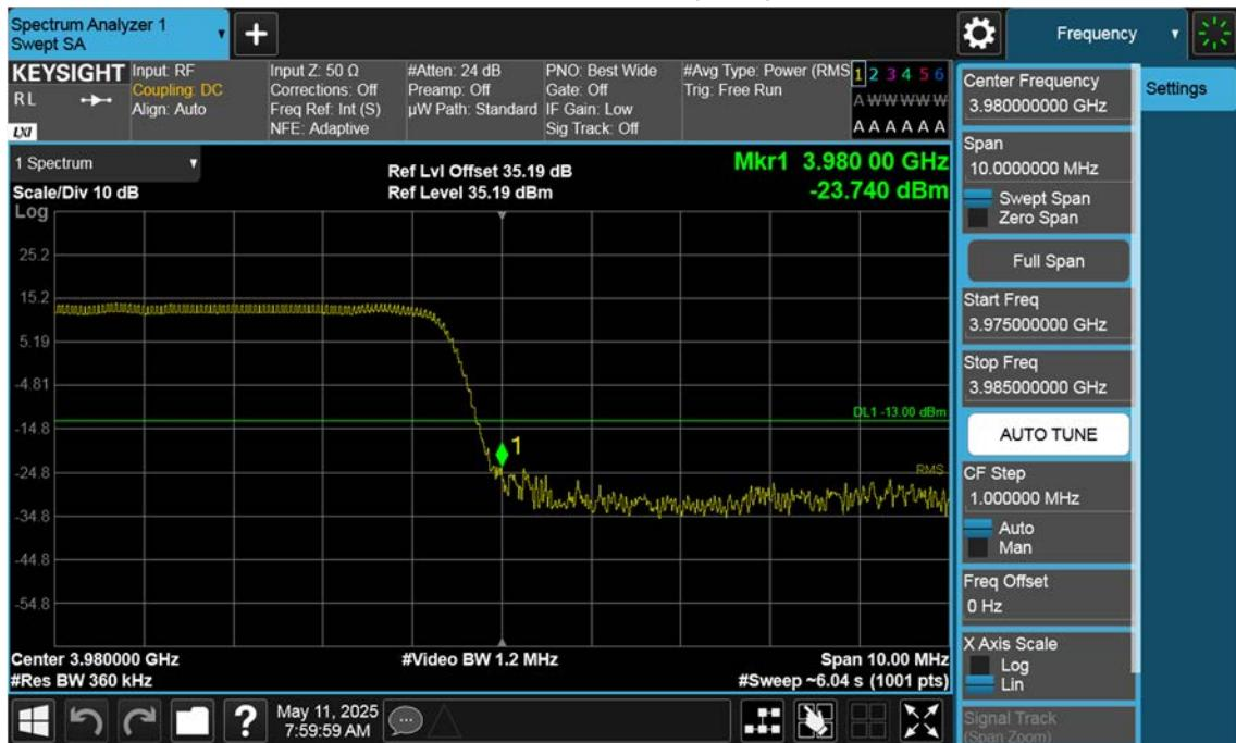
n77(3700~3980 MHz)\_10 M\_Band Edge\_High\_BPSK\_1RB(1)
