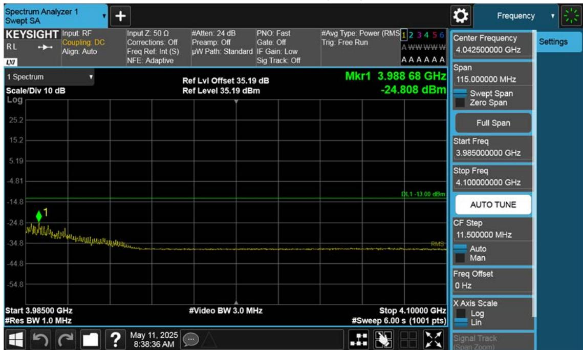
n77(3700~3980 MHz)\_25 M\_Band Edge\_High\_BPSK\_1RB(3)
