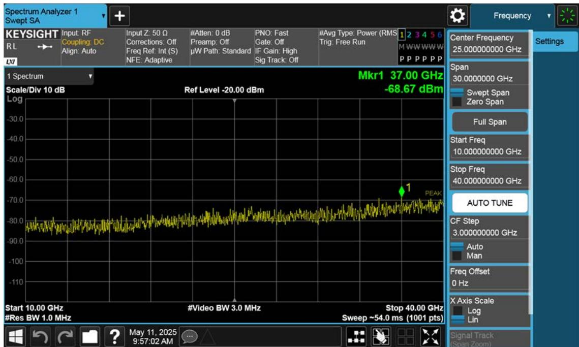
n77(3700~3980 MHz)\_90 M\_Conducted Spurious(Above10 G)\_High\_BPSK\_1RB
