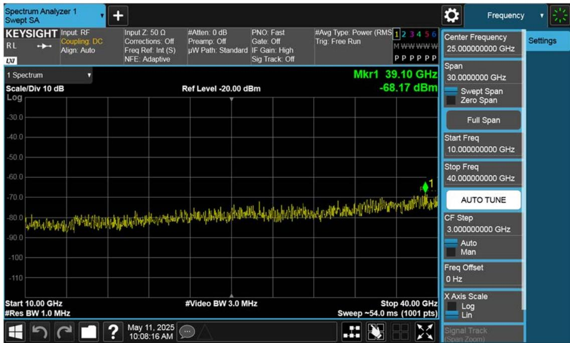
n77(3700~3980 MHz)\_100 M\_Conducted Spurious(Above10 G)\_High\_BPSK\_1RB
