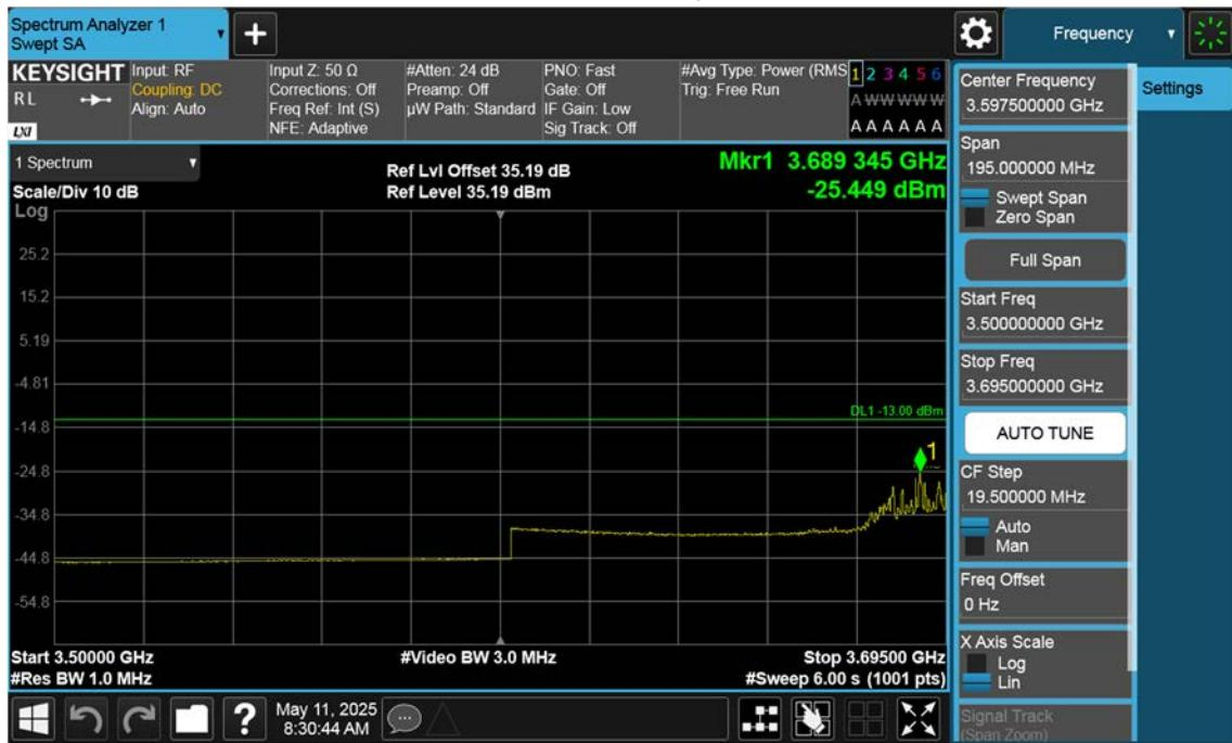
n77(3700~3980 MHz)\_25 M\_Band Edge\_Low\_BPSK\_1RB(3)
