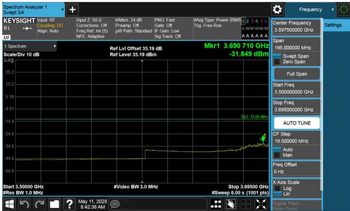
n77(3700~3980 MHz)\_30 M\_Band Edge\_Low\_BPSK\_1RB(3)
