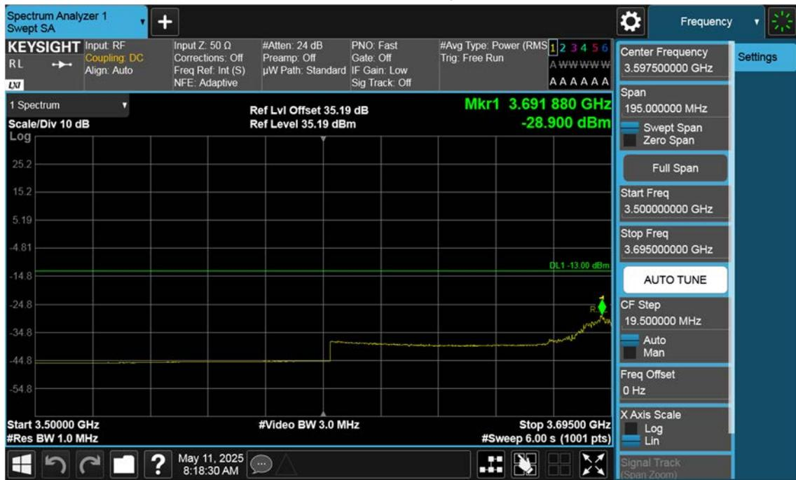
n77(3700~3980 MHz)\_20 M\_Band Edge\_Low\_BPSK\_1RB(3)
