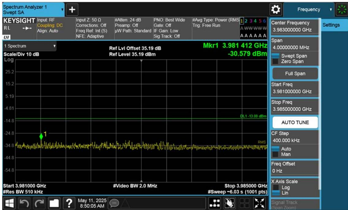
n77(3700~3980 MHz)\_30 M\_Band Edge\_High\_BPSK\_1RB(2)
