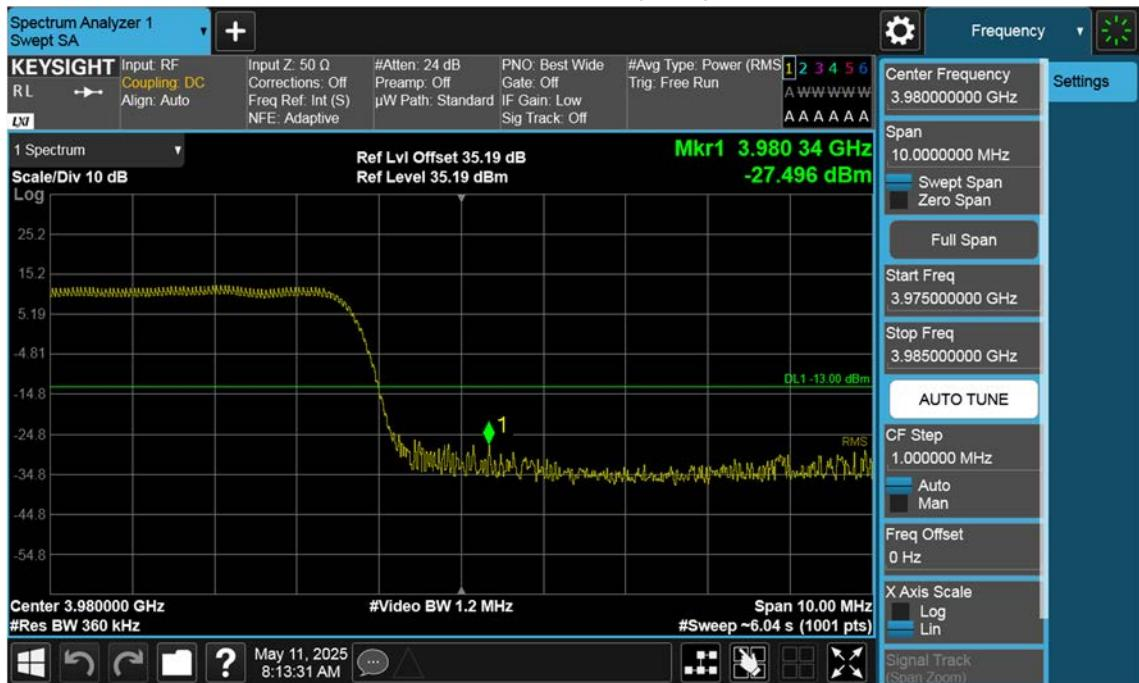
n77(3700~3980 MHz)\_15 M\_Band Edge\_High\_BPSK\_1RB(1)
