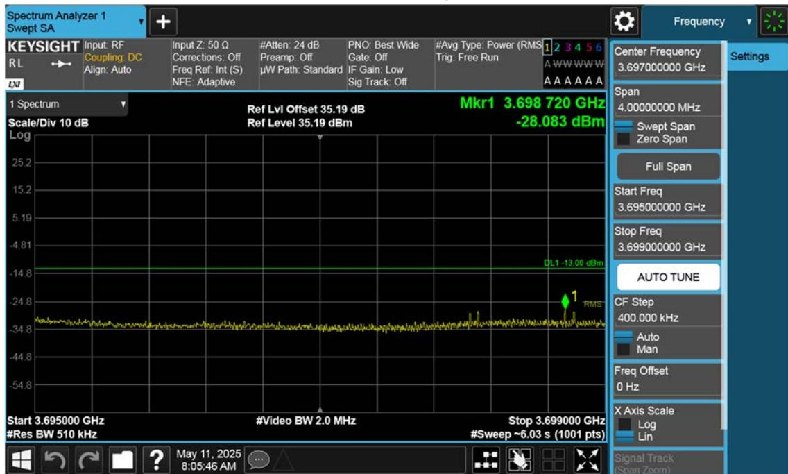
n77(3700~3980 MHz)\_15 M\_Band Edge\_Low\_BPSK\_1RB(2)
