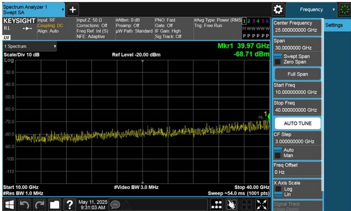
n77(3700~3980 MHz)\_70 M\_Conducted Spurious(Above10 G)\_Mid\_BPSK\_1RB
