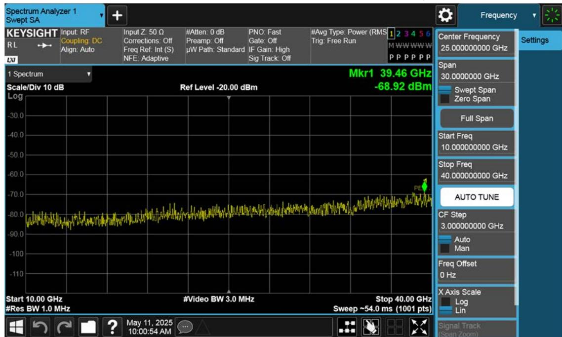
n77(3700~3980 MHz)\_100 M\_Conducted Spurious(Above10 G)\_Low\_BPSK\_1RB
