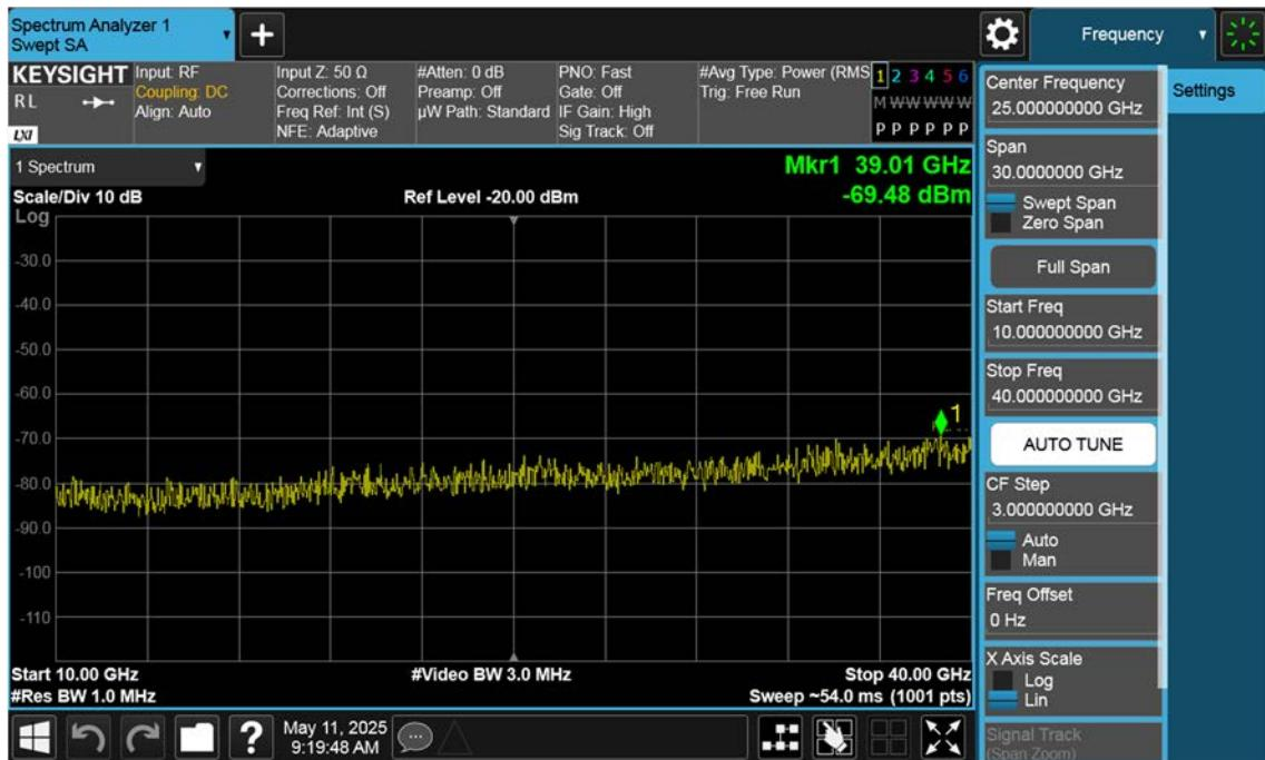
n77(3700~3980 MHz)\_60 M\_Conducted Spurious(Above10 G)\_Mid\_BPSK\_1RB
