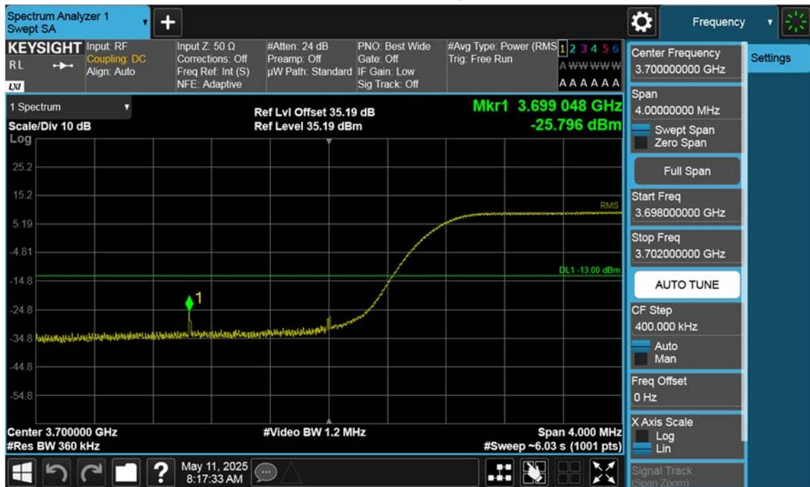
n77(3700~3980 MHz)\_20 M\_Band Edge\_Low\_BPSK\_1RB(1)
