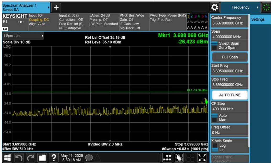
n77(3700~3980 MHz)\_25 M\_Band Edge\_Low\_BPSK\_1RB(2)
