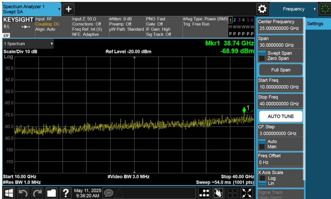
n77(3700~3980 MHz)\_80 M\_Conducted Spurious(Above10 G)\_Low\_BPSK\_1RB
