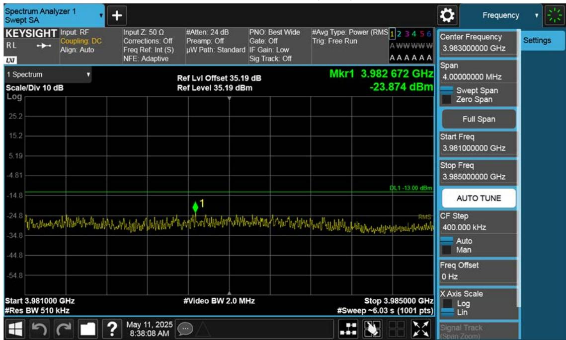
n77(3700~3980 MHz)\_25 M\_Band Edge\_High\_BPSK\_1RB(2)
