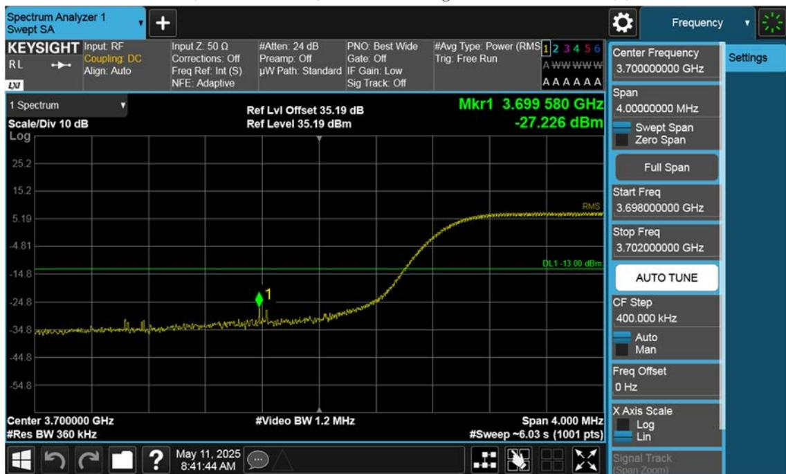
n77(3700~3980 MHz)\_30 M\_Band Edge\_Low\_BPSK\_1RB(1)
