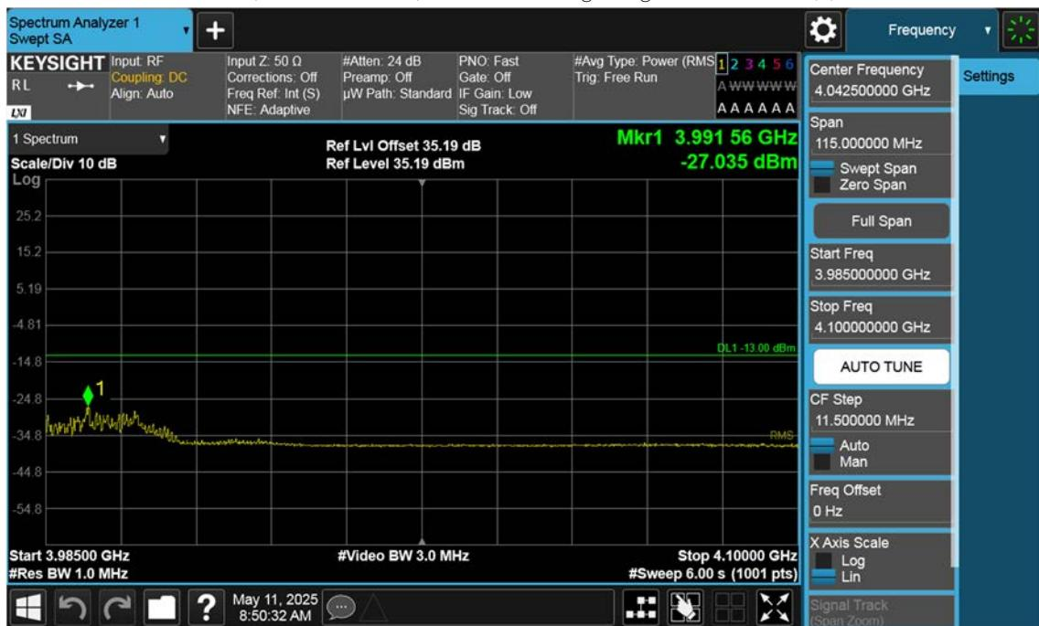
n77(3700~3980 MHz)\_30 M\_Band Edge\_High\_BPSK\_1RB(3)
