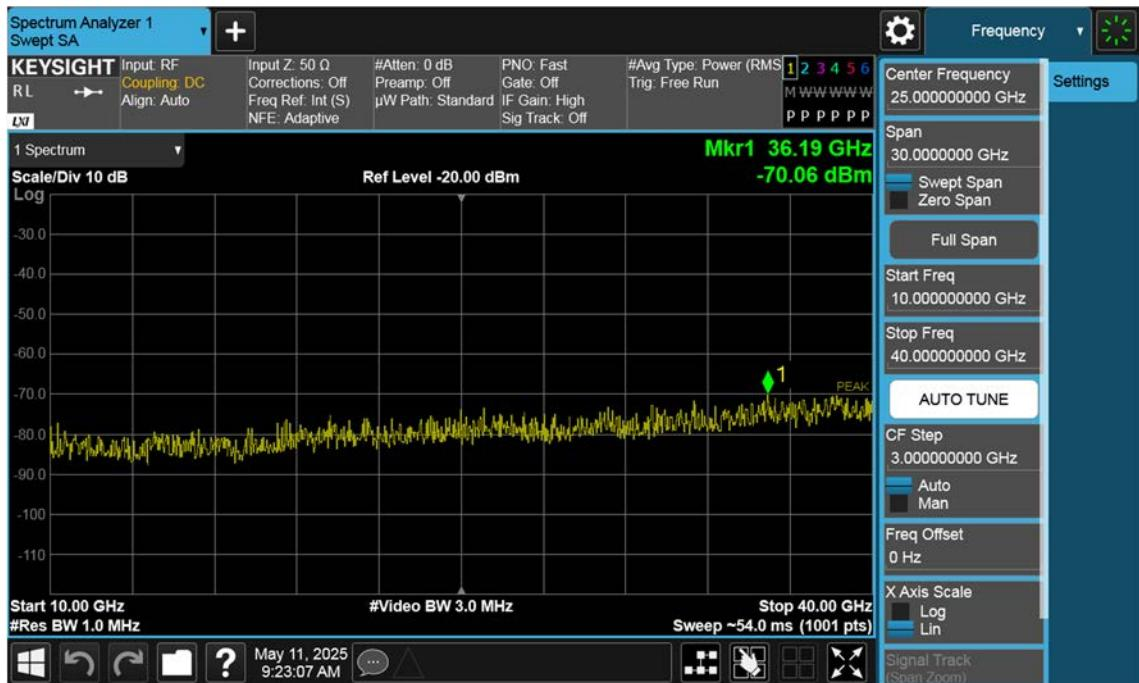
n77(3700~3980 MHz)\_60 M\_Conducted Spurious(Above10 G)\_High\_BPSK\_1RB
