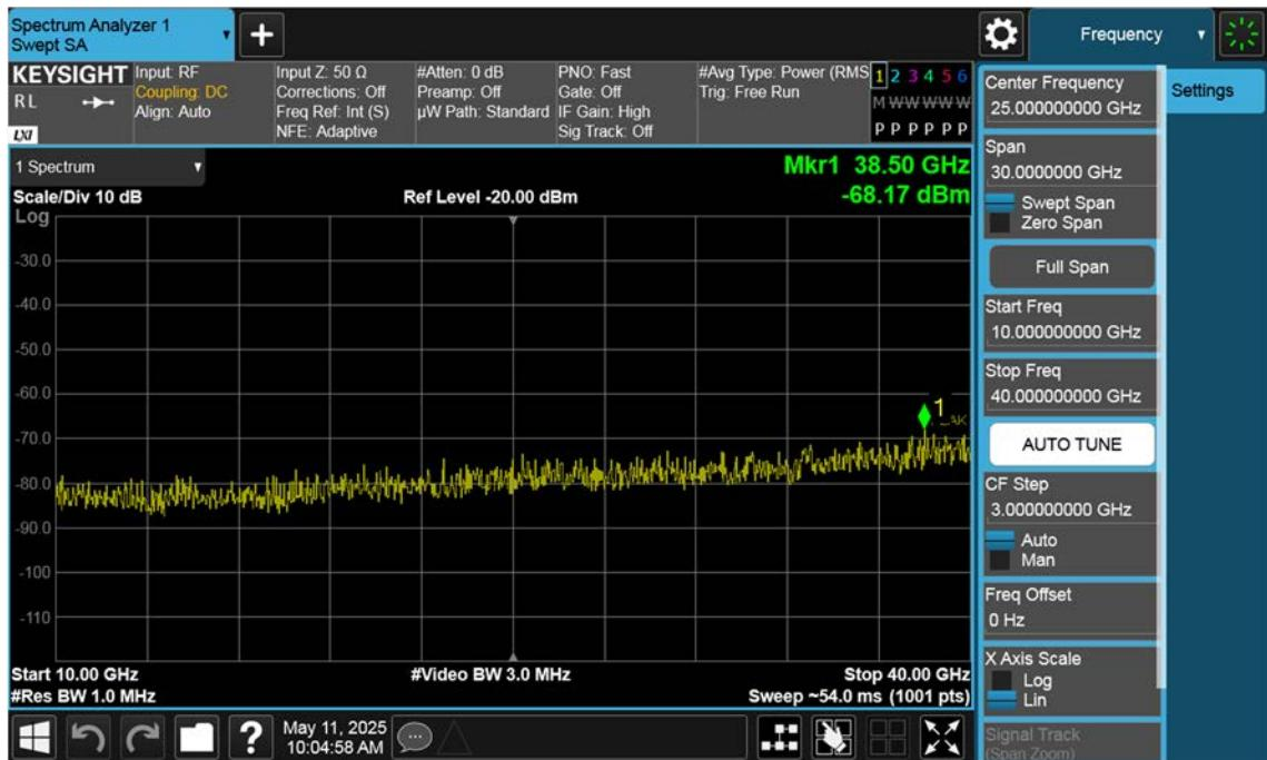
n77(3700~3980 MHz)\_100 M\_Conducted Spurious(Above10 G)\_Mid\_BPSK\_1RB
