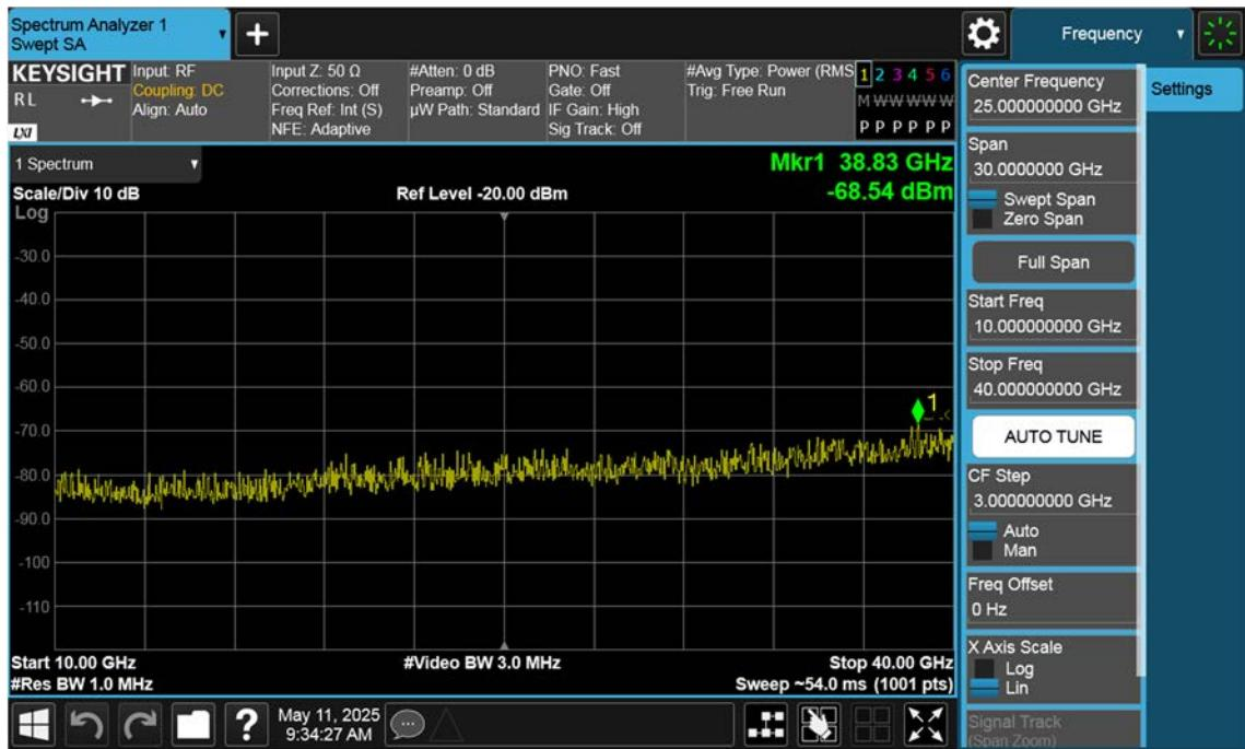
n77(3700~3980 MHz)\_70 M\_Conducted Spurious(Above10 G)\_High\_BPSK\_1RB
