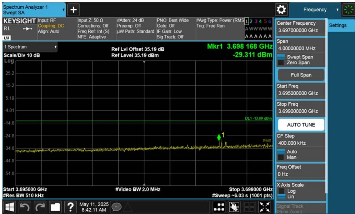
n77(3700~3980 MHz)\_30 M\_Band Edge\_Low\_BPSK\_1RB(2)
