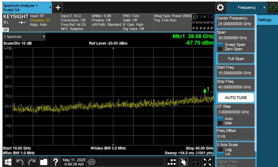
n77(3700~3980 MHz)\_90 M\_Conducted Spurious(Above10 G)\_Low\_BPSK\_1RB
