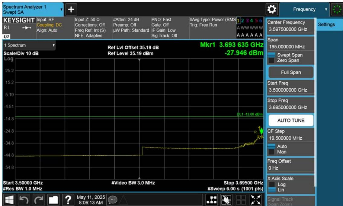
n77(3700~3980 MHz)\_15 M\_Band Edge\_Low\_BPSK\_1RB(3)
