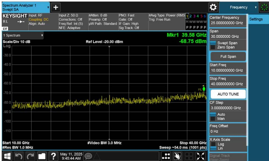
n77(3700~3980 MHz)\_80 M\_Conducted Spurious(Above10 G)\_High\_BPSK\_1RB
