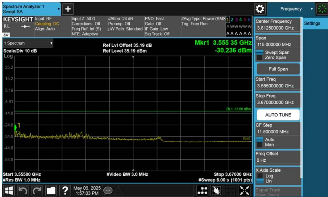
n77(3450~3550 MHz)\_80 M\_Band Edge\_High\_BPSK\_1RB(3)
