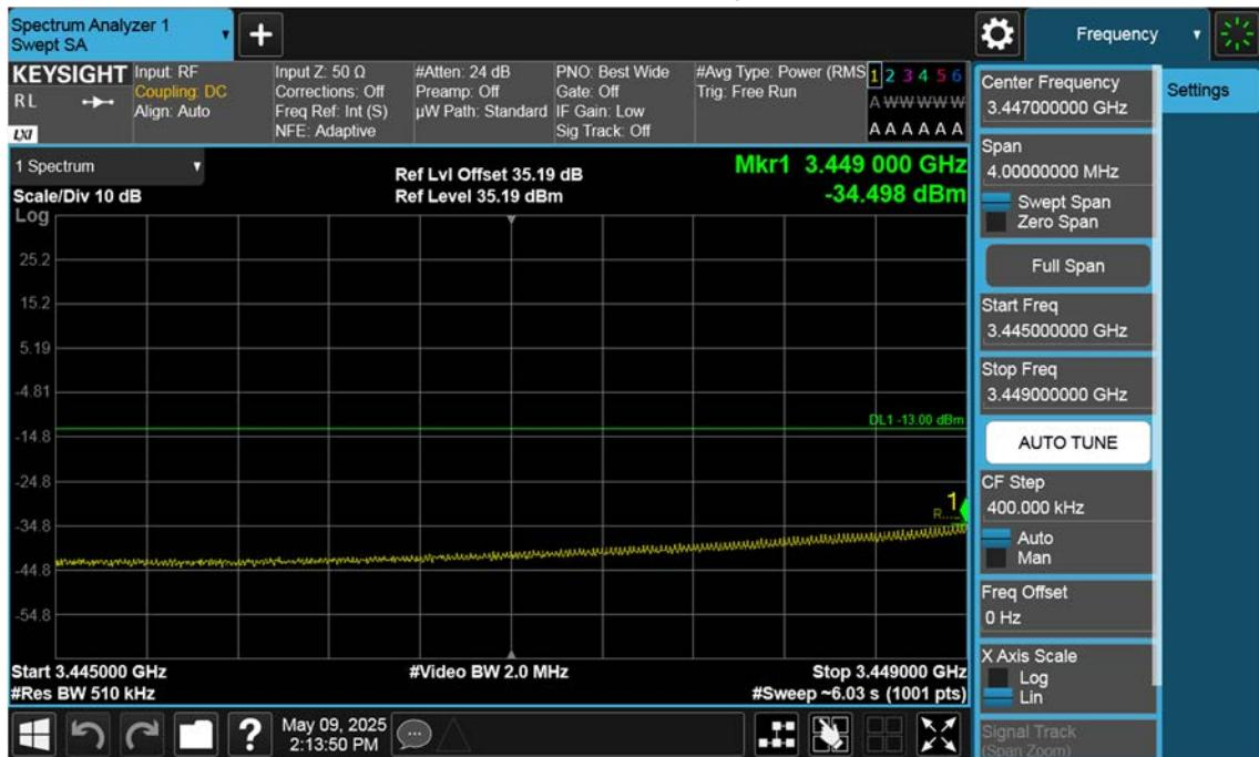
n77(3450~3550 MHz)\_100 M\_Band Edge\_Low\_BPSK\_FullIRB(3)
