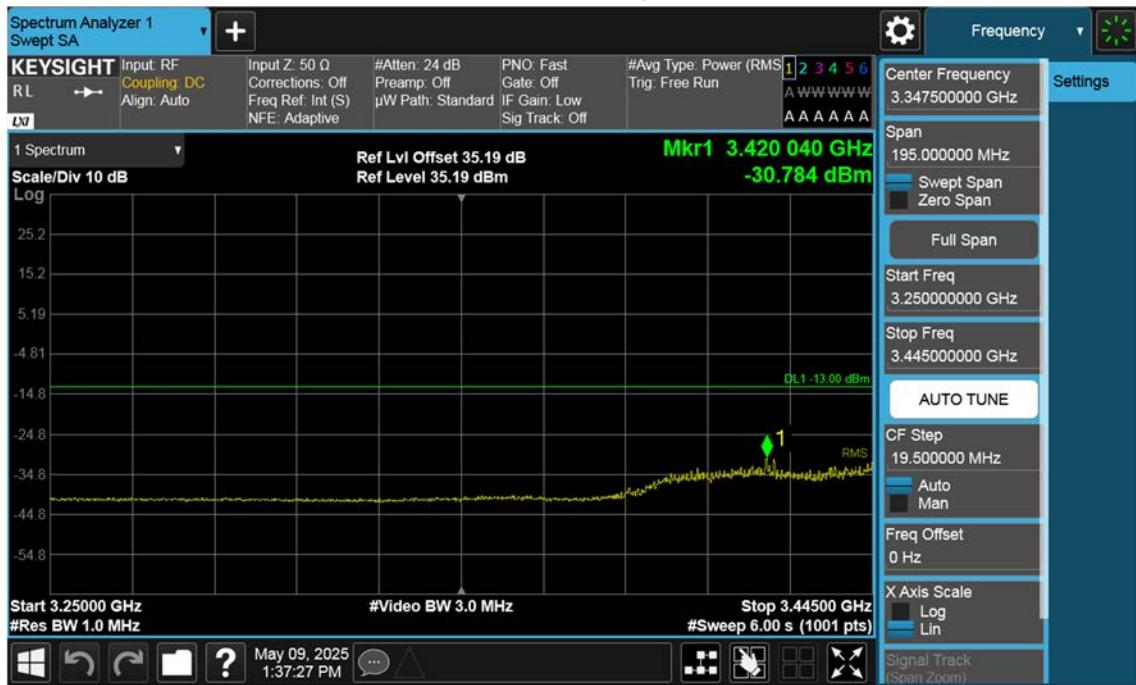
n77(3450~3550 MHz)\_70 M\_Band Edge\_Low\_BPSK\_1RB(3)
