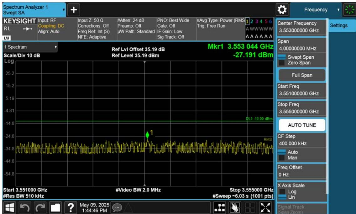
n77(3450~3550 MHz)\_70 M\_Band Edge\_High\_BPSK\_1RB(2)
