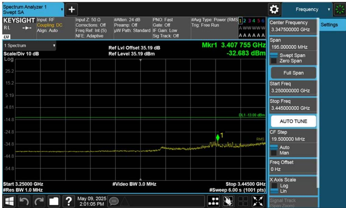
n77(3450~3550 MHz)\_90 M\_Band Edge\_Low\_BPSK\_1RB(3)
