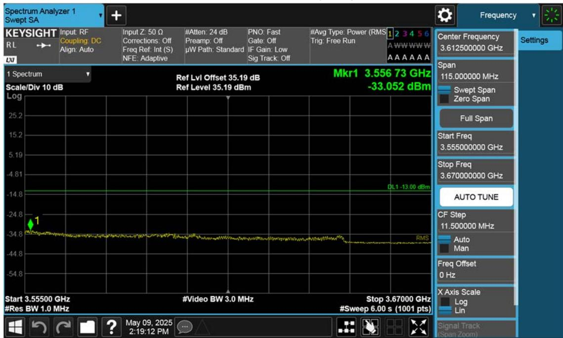
n77(3450~3550 MHz)\_100 M\_Band Edge\_High\_BPSK\_1RB(3)
