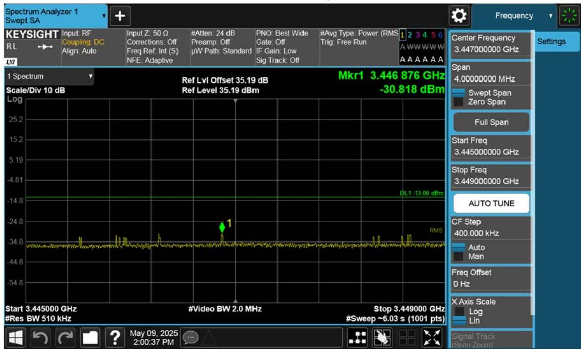
n77(3450~3550 MHz)\_90 M\_Band Edge\_Low\_BPSK\_1RB(2)
