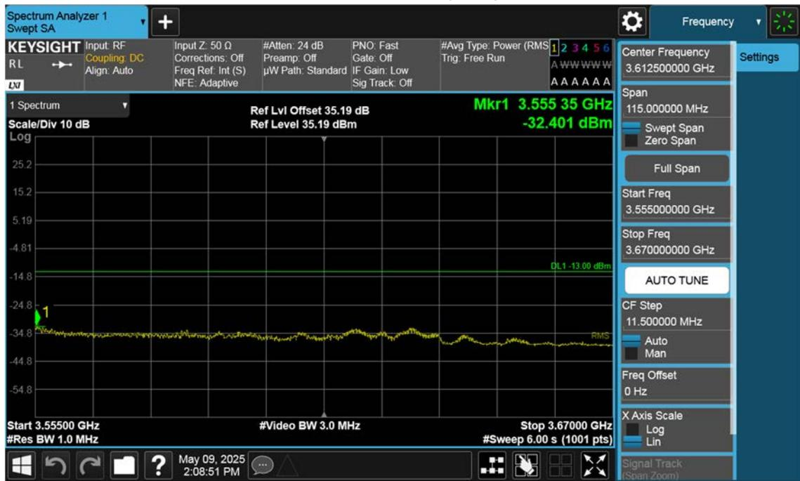
n77(3450~3550 MHz)\_90 M\_Band Edge\_High\_BPSK\_1RB(3)
