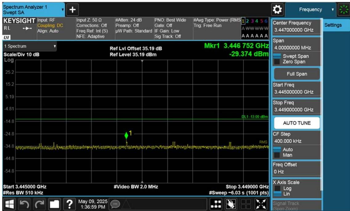
n77(3450~3550 MHz)\_70 M\_Band Edge\_Low\_BPSK\_1RB(2)
