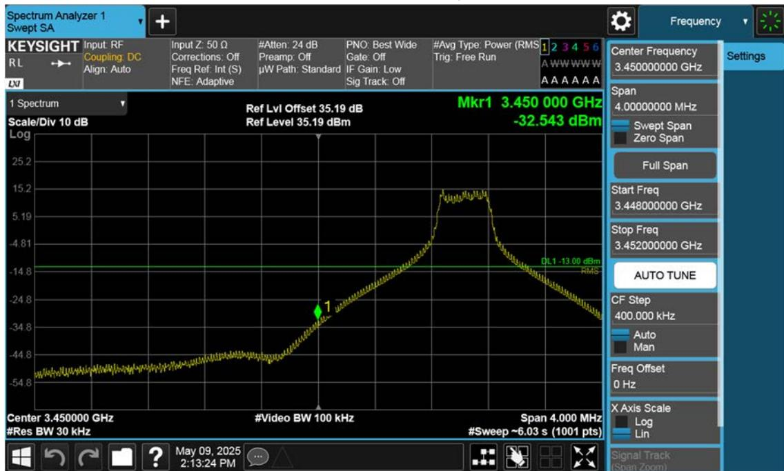
n77(3450~3550 MHz)\_100 M\_Band Edge\_Low\_BPSK\_FullIRB(2)
