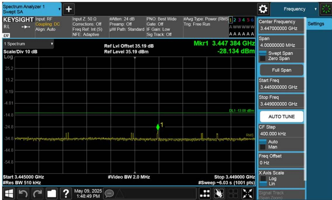
n77(3450~3550 MHz)\_80 M\_Band Edge\_Low\_BPSK\_1RB(2)
