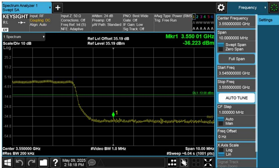
n77(3450~3550 MHz)\_100 M\_Band Edge\_High\_BPSK\_1RB(1)
