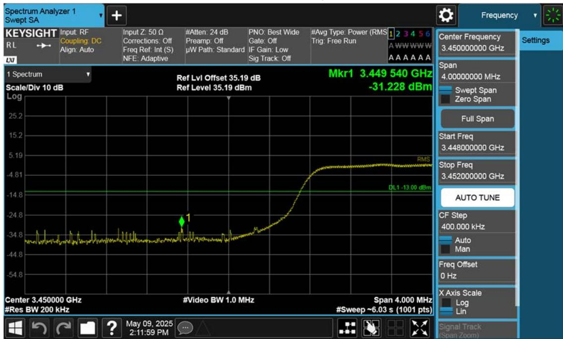
n77(3450~3550 MHz)\_100 M\_Band Edge\_Low\_BPSK\_1RB(1)
