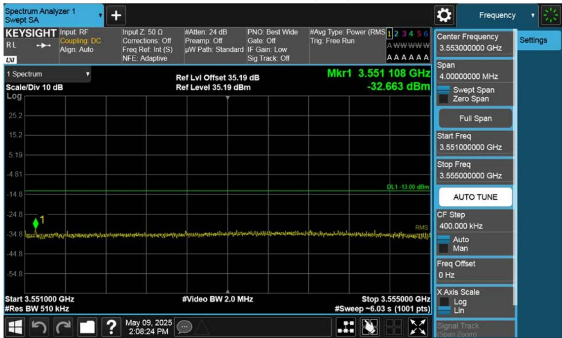
n77(3450~3550 MHz)\_90 M\_Band Edge\_High\_BPSK\_1RB(2)
