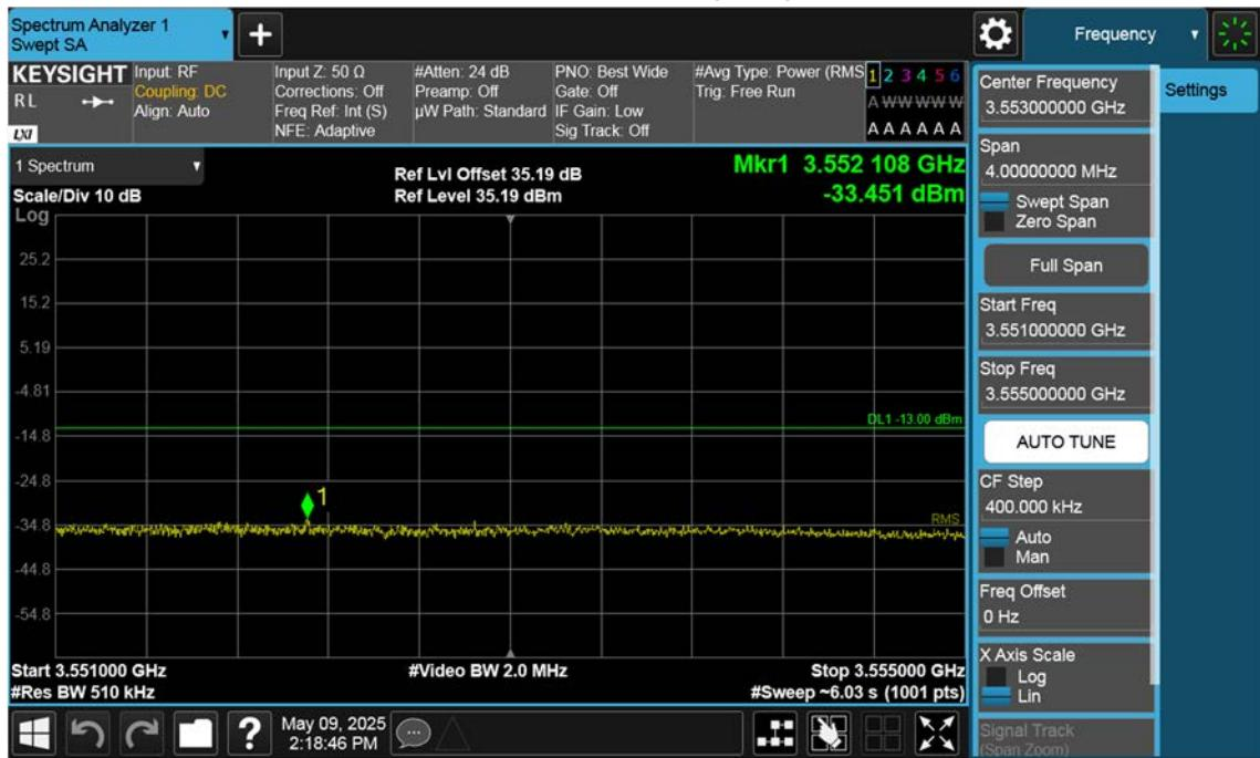
n77(3450~3550 MHz)\_100 M\_Band Edge\_High\_BPSK\_1RB(2)
