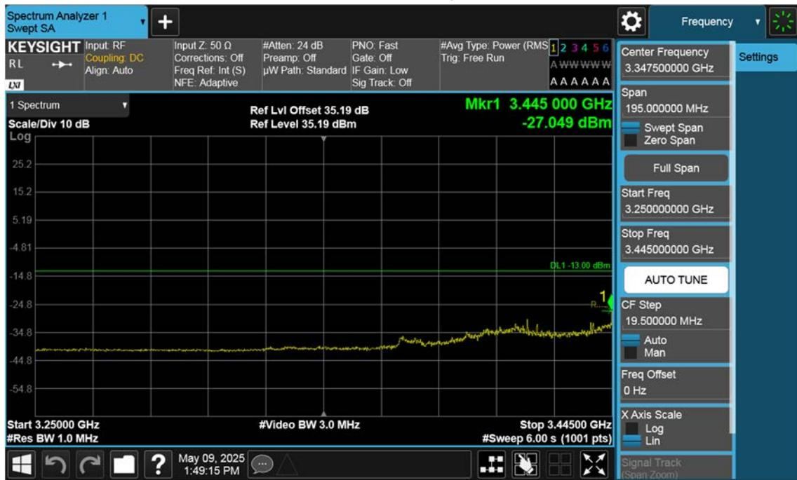
n77(3450~3550 MHz)\_80 M\_Band Edge\_Low\_BPSK\_1RB(3)
