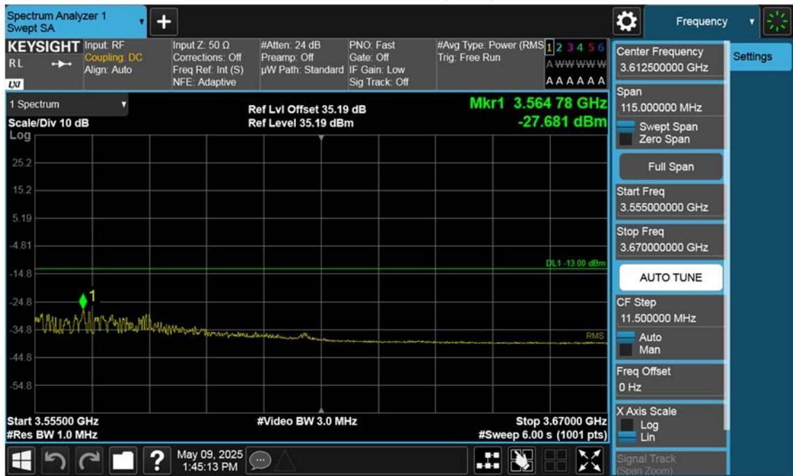
n77(3450~3550 MHz)\_70 M\_Band Edge\_High\_BPSK\_1RB(3)
