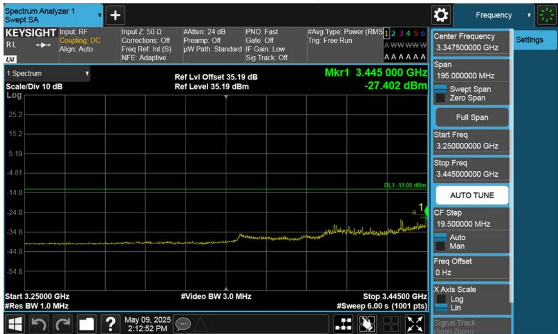
n77(3450~3550 MHz)\_100 M\_Band Edge\_Low\_BPSK\_1RB(3)
