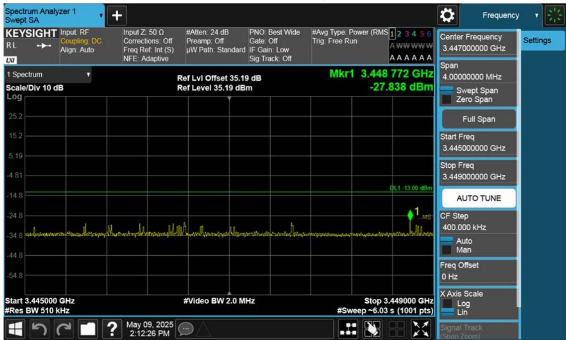
n77(3450~3550 MHz)\_100 M\_Band Edge\_Low\_BPSK\_1RB(2)
