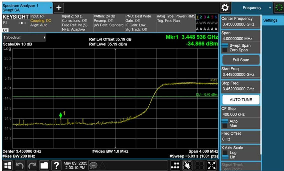
n77(3450~3550 MHz)\_90 M\_Band Edge\_Low\_BPSK\_1RB(1)
