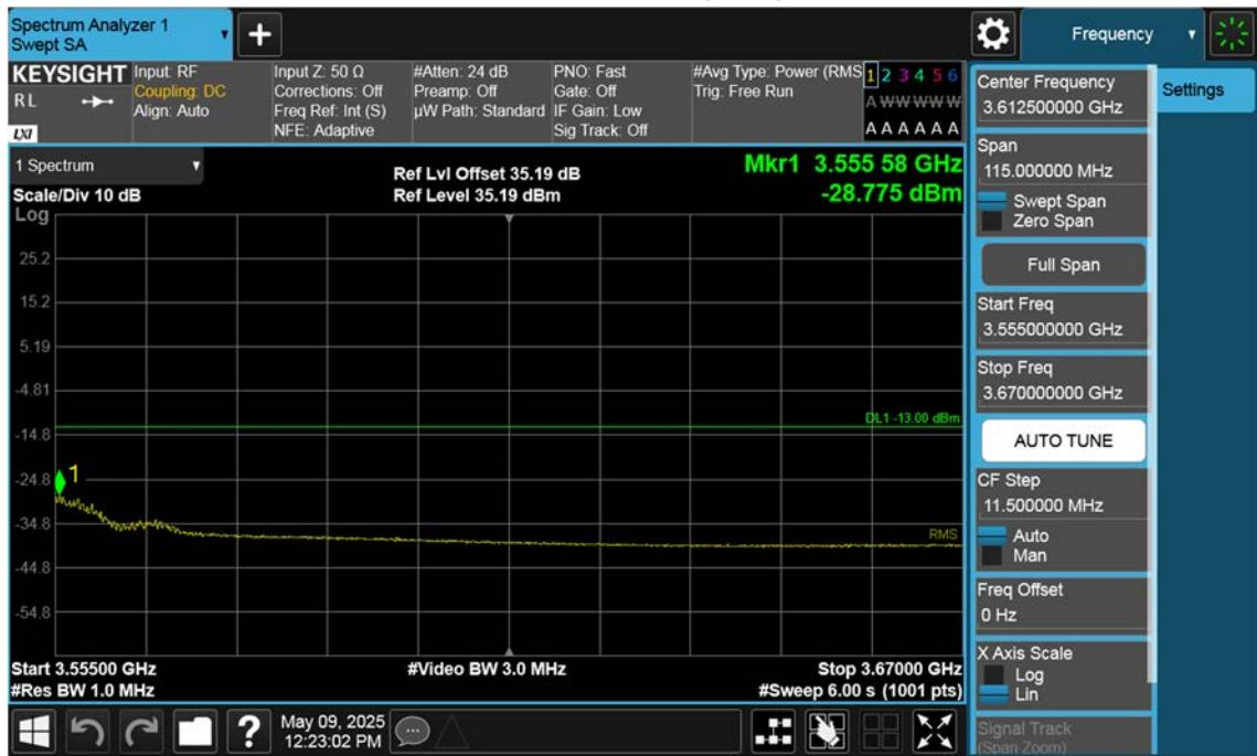
n77(3450~3550 MHz)\_15 M\_Band Edge\_High\_BPSK\_1RB(3)
