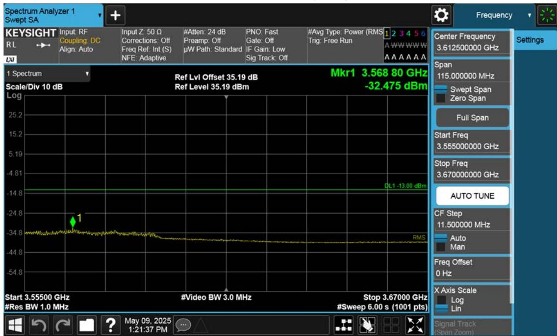
n77(3450~3550 MHz)\_50 M\_Band Edge\_High\_BPSK\_1RB(3)
