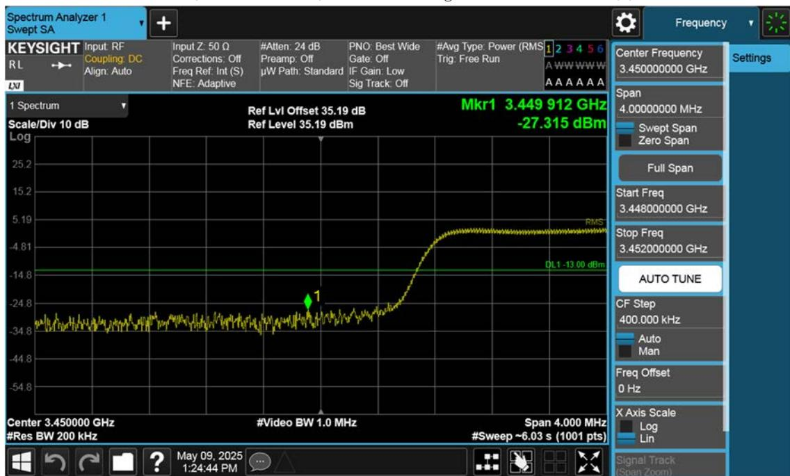
n77(3450~3550 MHz)\_60 M\_Band Edge\_Low\_BPSK\_1RB(1)
