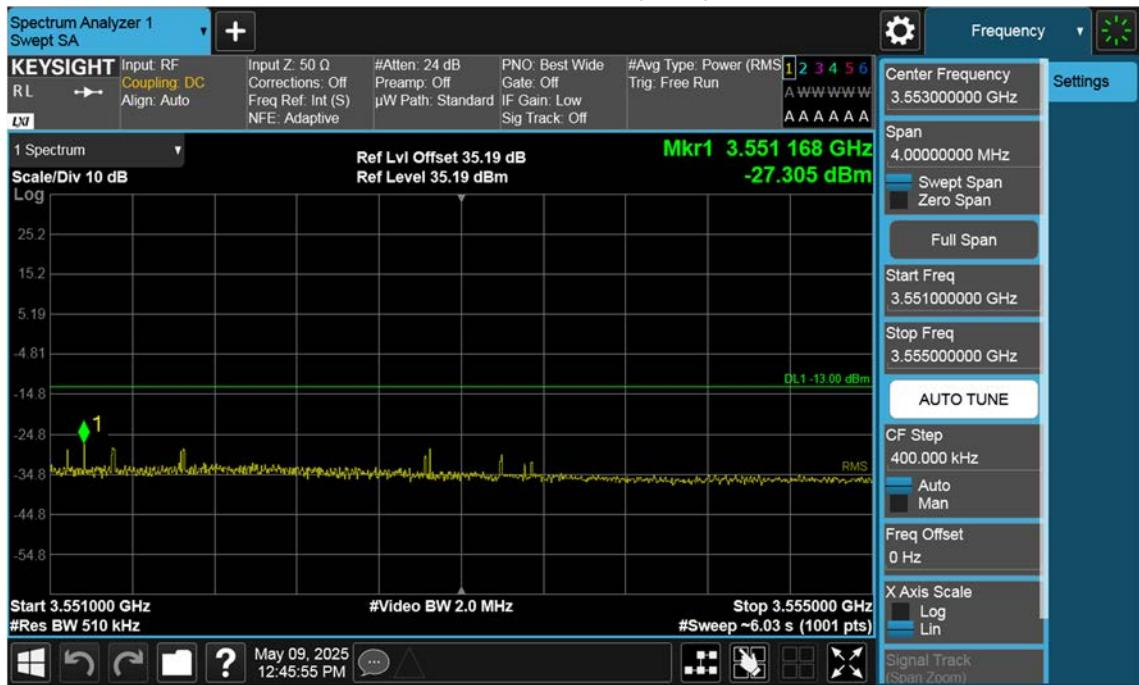
n77(3450~3550 MHz)\_25 M\_Band Edge\_High\_BPSK\_1RB(2)
