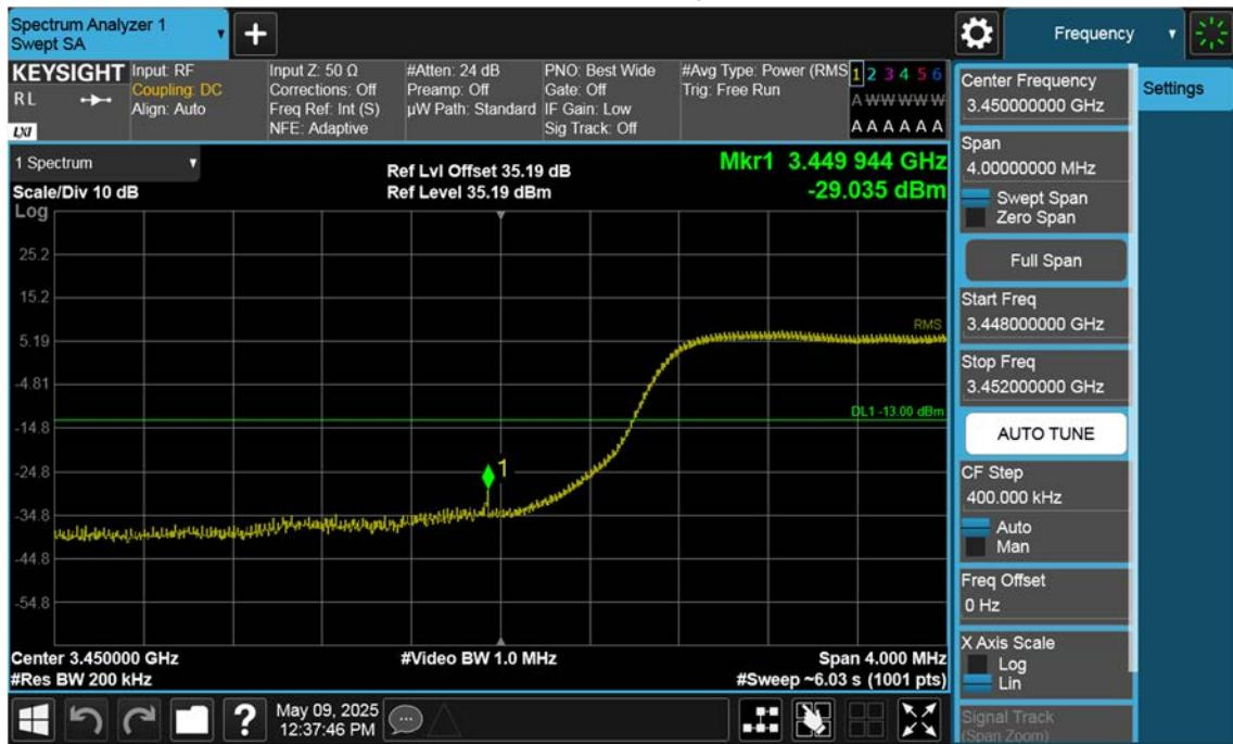
n77(3450~3550 MHz)\_25 M\_Band Edge\_Low\_BPSK\_1RB(1)
