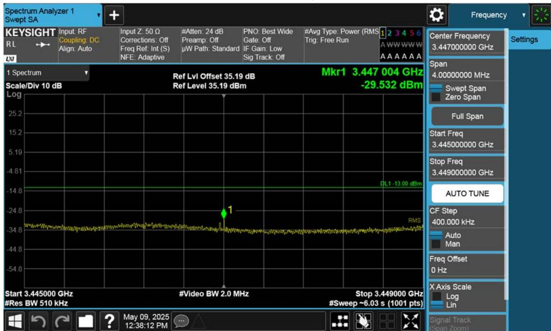
n77(3450~3550 MHz)\_25 M\_Band Edge\_Low\_BPSK\_1RB(2)
