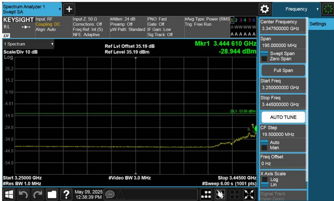
n77(3450~3550 MHz)\_25 M\_Band Edge\_Low\_BPSK\_1RB(3)
