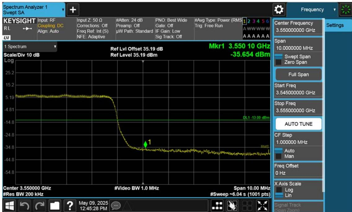
n77(3450~3550 MHz)\_25 M\_Band Edge\_High\_BPSK\_1RB(1)
