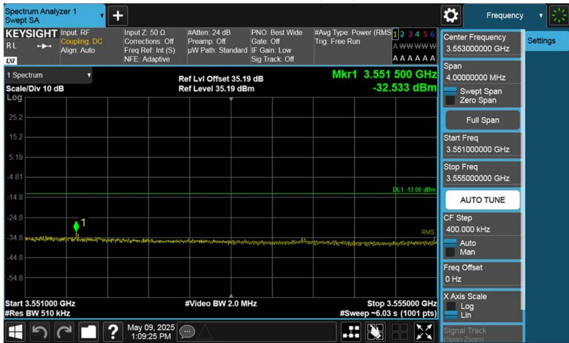
n77(3450~3550 MHz)\_40 M\_Band Edge\_High\_BPSK\_1RB(2)
