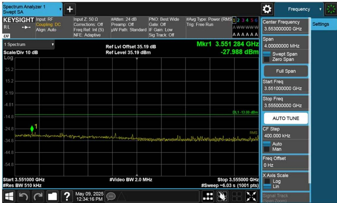
n77(3450~3550 MHz)\_20 M\_Band Edge\_High\_BPSK\_1RB(2)
