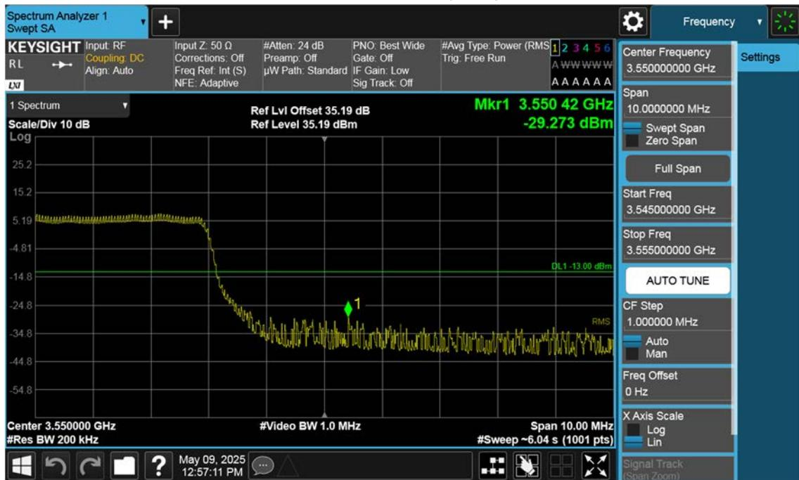
n77(3450~3550 MHz)\_30 M\_Band Edge\_High\_BPSK\_1RB(1)
