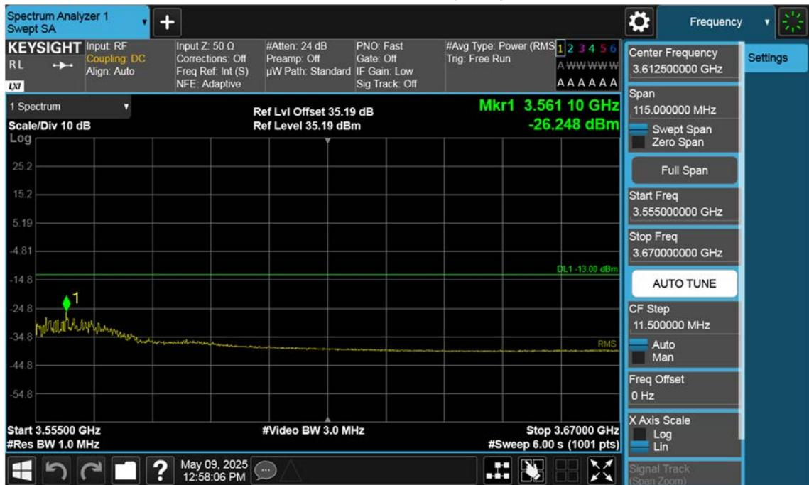
n77(3450~3550 MHz)\_30 M\_Band Edge\_High\_BPSK\_1RB(3)
