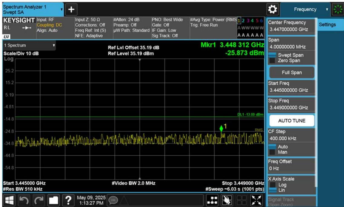
n77(3450~3550 MHz)\_50 M\_Band Edge\_Low\_BPSK\_1RB(2)
