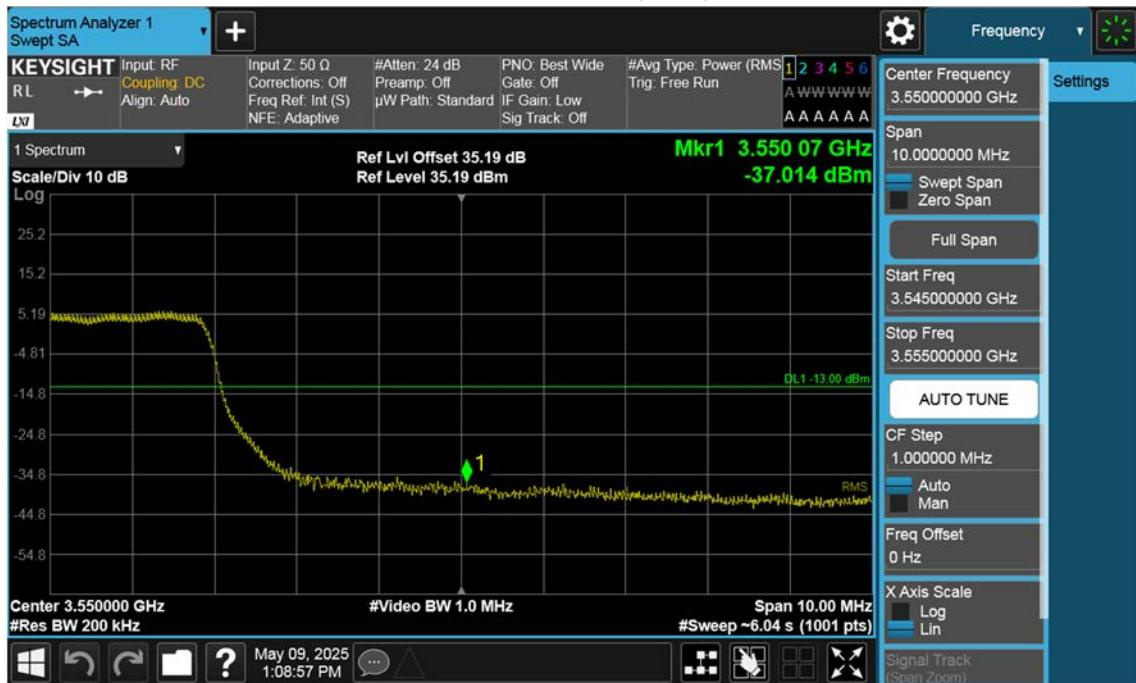
n77(3450~3550 MHz)\_40 M\_Band Edge\_High\_BPSK\_1RB(1)
