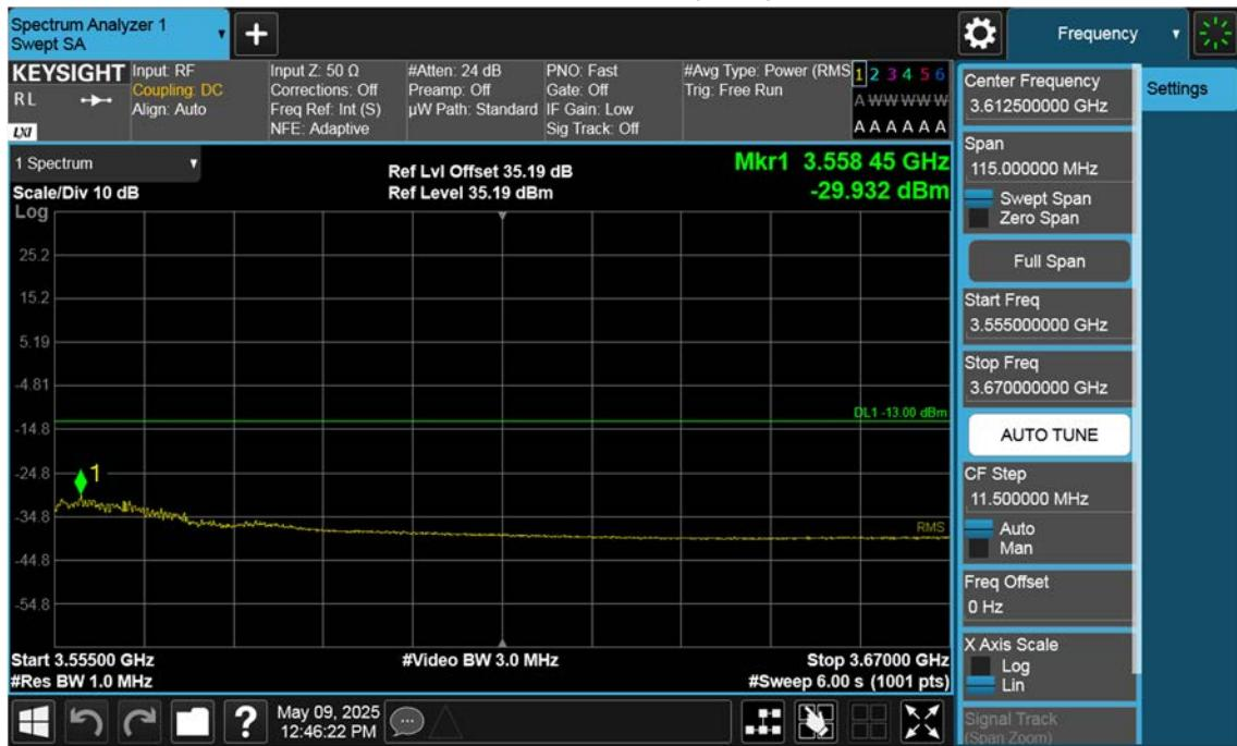
n77(3450~3550 MHz)\_25 M\_Band Edge\_High\_BPSK\_1RB(3)
