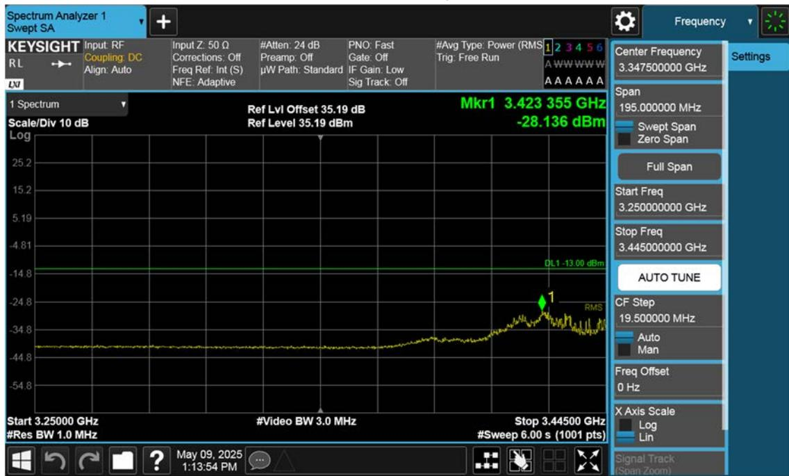
n77(3450~3550 MHz)\_50 M\_Band Edge\_Low\_BPSK\_1RB(3)
