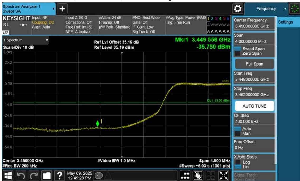
n77(3450~3550 MHz)\_30 M\_Band Edge\_Low\_BPSK\_1RB(1)
