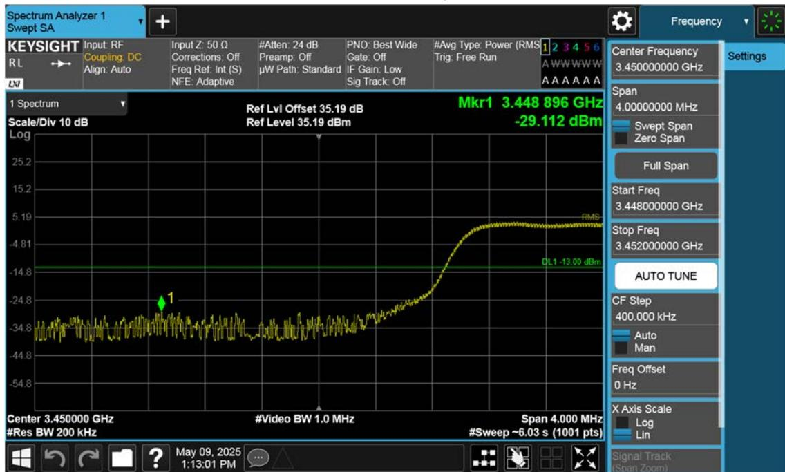
n77(3450~3550 MHz)\_50 M\_Band Edge\_Low\_BPSK\_1RB(1)
