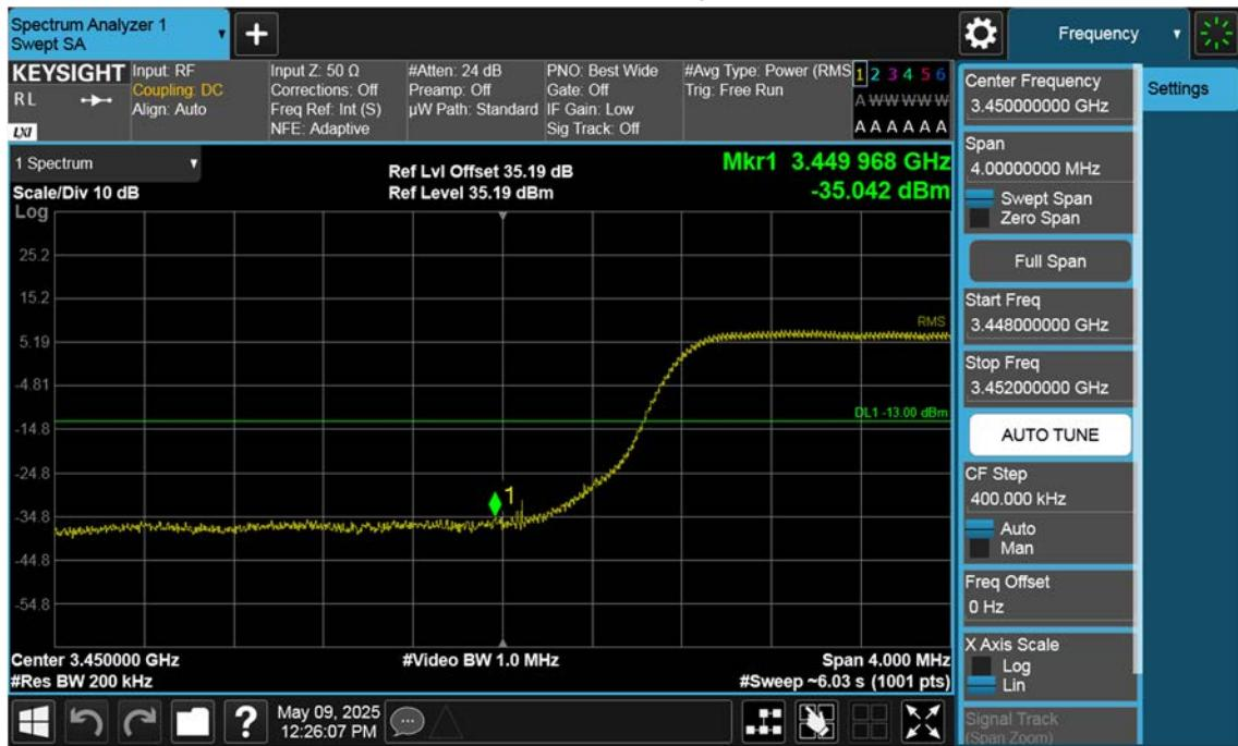
n77(3450~3550 MHz)\_20 M\_Band Edge\_Low\_BPSK\_1RB(1)
