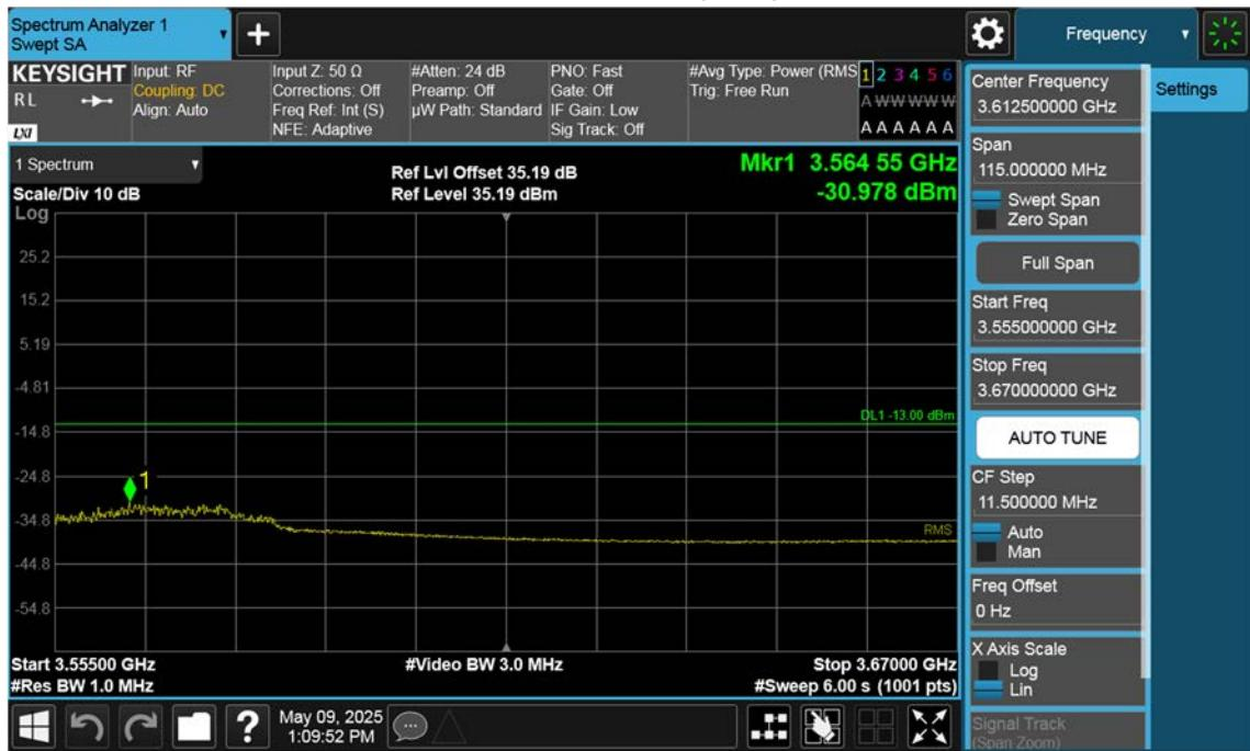
n77(3450~3550 MHz)\_40 M\_Band Edge\_High\_BPSK\_1RB(3)
