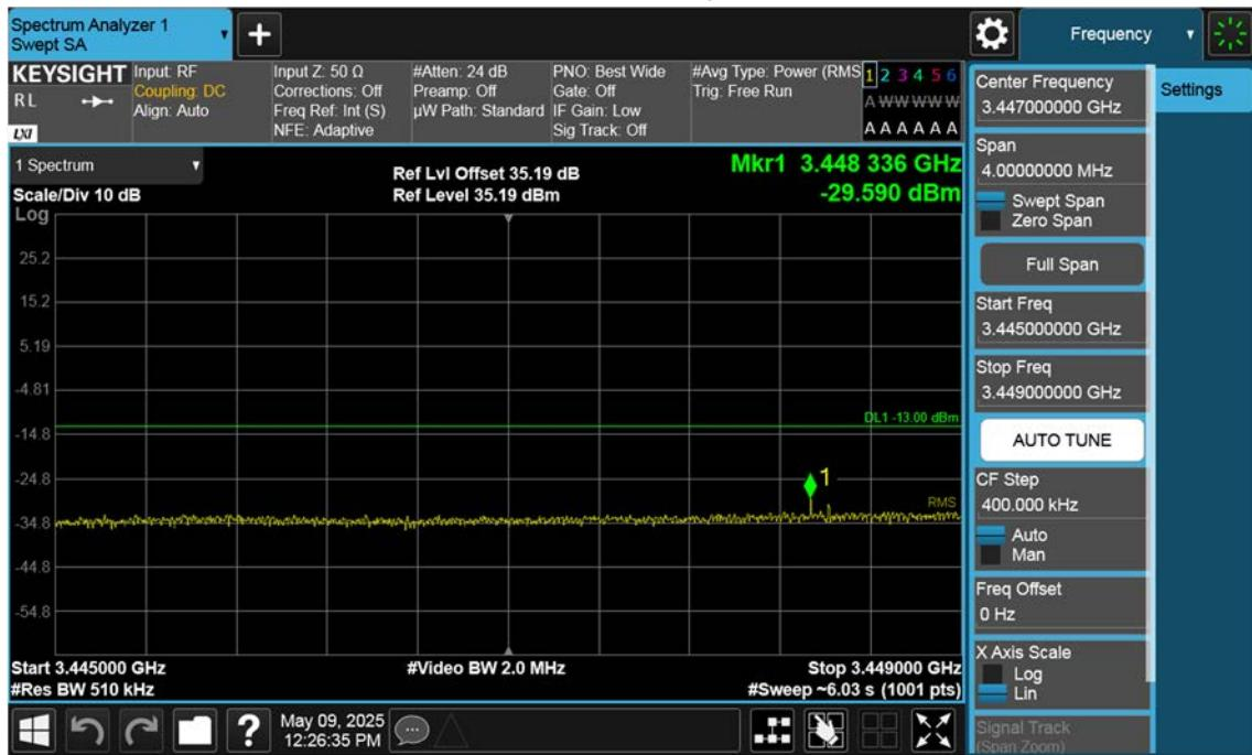
n77(3450~3550 MHz)\_20 M\_Band Edge\_Low\_BPSK\_1RB(2)
