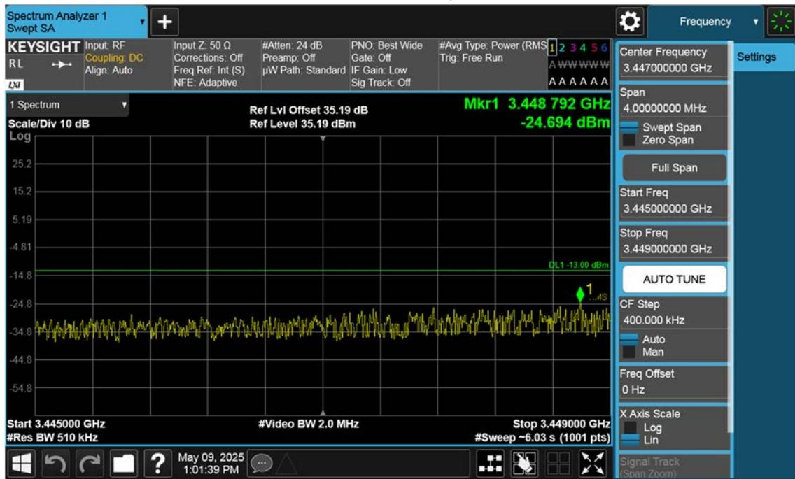
n77(3450~3550 MHz)\_40 M\_Band Edge\_Low\_BPSK\_1RB(2)
