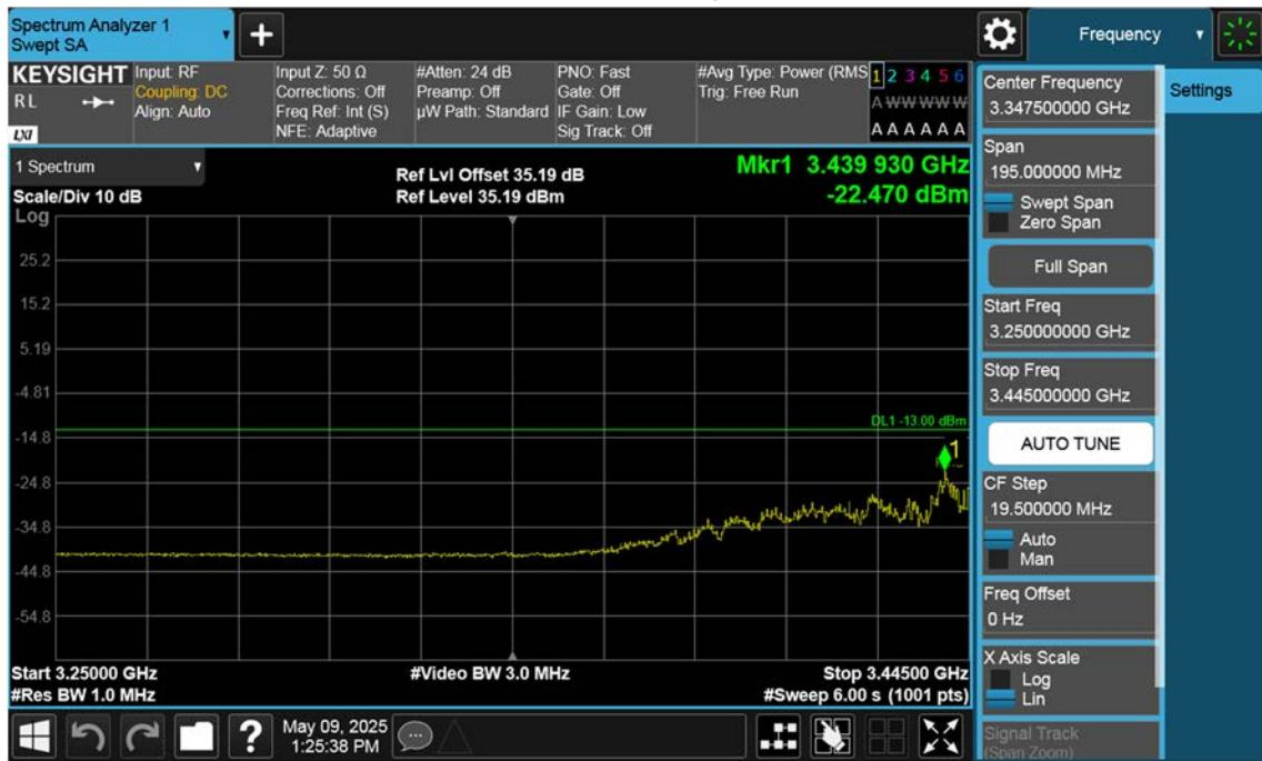
n77(3450~3550 MHz)\_60 M\_Band Edge\_Low\_BPSK\_1RB(3)
