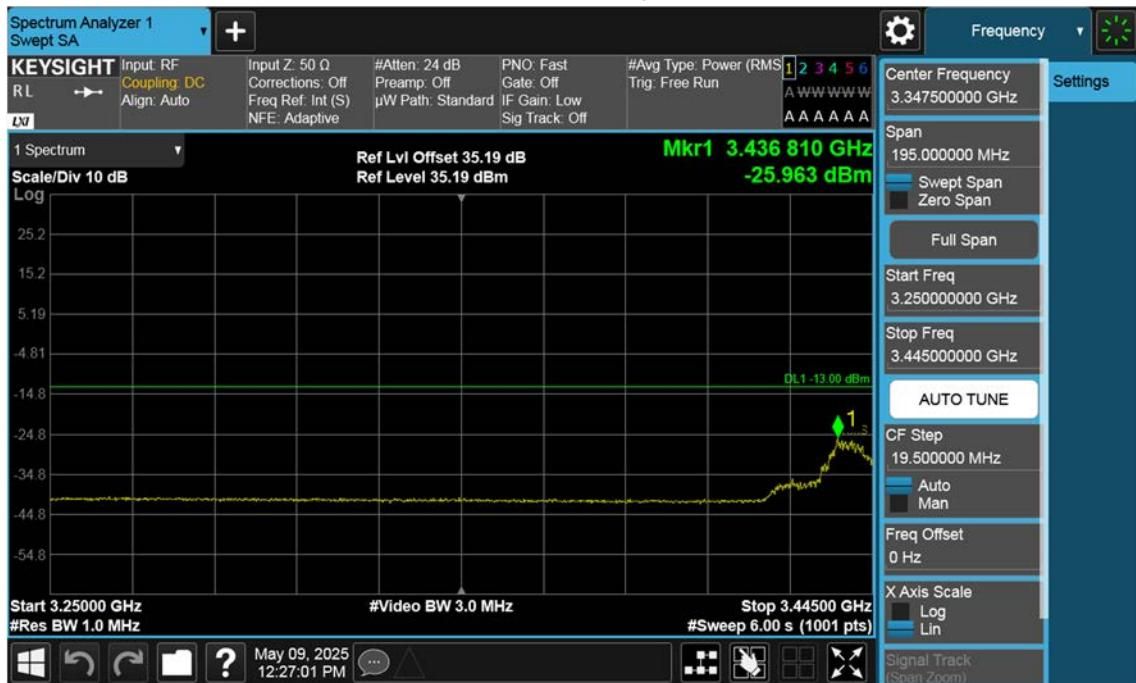
n77(3450~3550 MHz)\_20 M\_Band Edge\_Low\_BPSK\_1RB(3)
