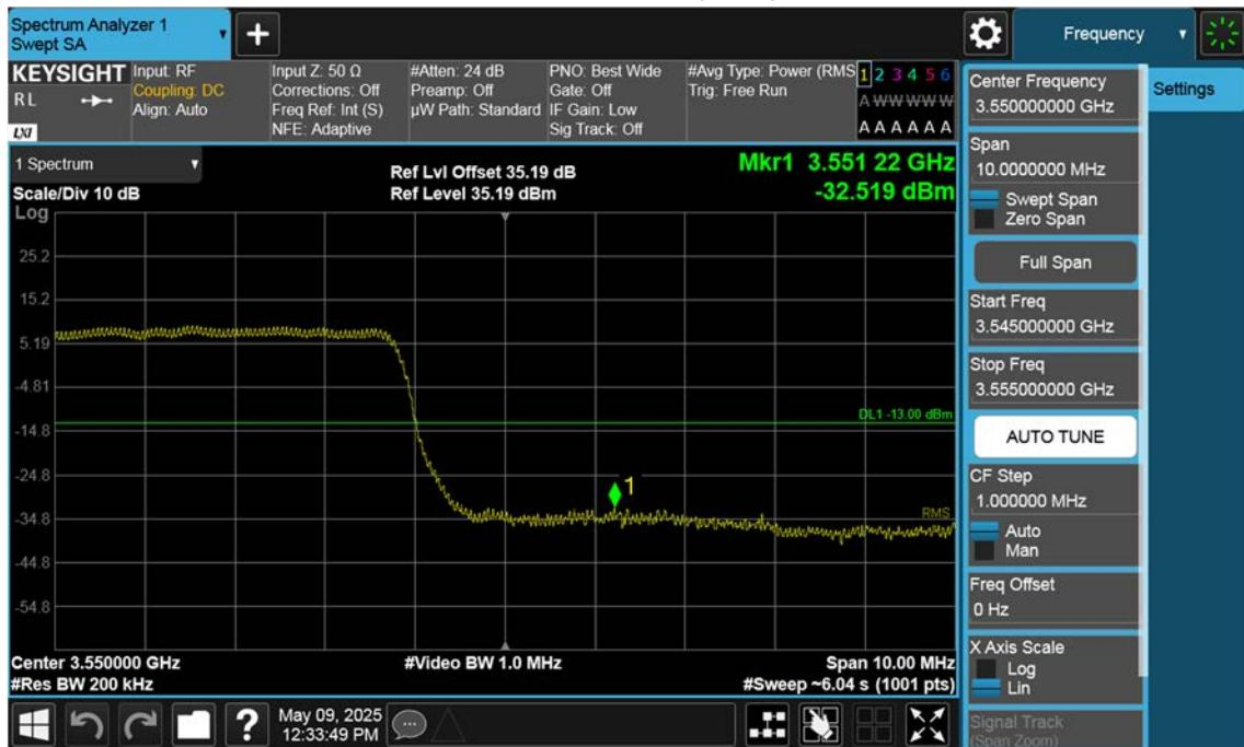
n77(3450~3550 MHz)\_20 M\_Band Edge\_High\_BPSK\_1RB(1)
