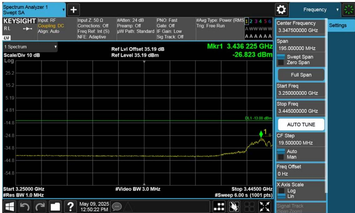
n77(3450~3550 MHz)\_30 M\_Band Edge\_Low\_BPSK\_1RB(3)
