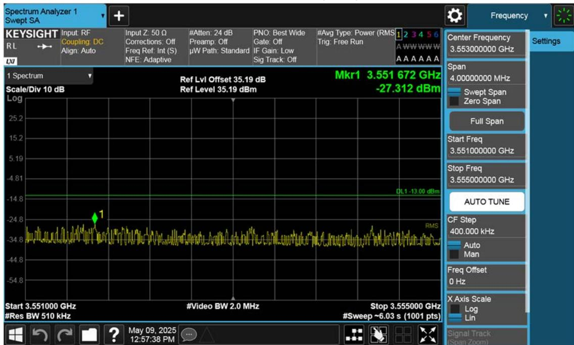
n77(3450~3550 MHz)\_30 M\_Band Edge\_High\_BPSK\_1RB(2)
