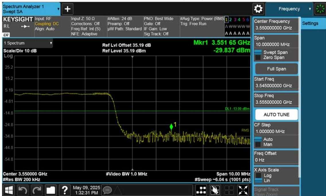
n77(3450~3550 MHz)\_60 M\_Band Edge\_High\_BPSK\_1RB(1)
