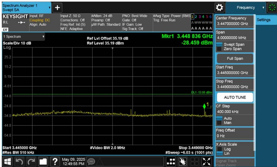
n77(3450~3550 MHz)\_30 M\_Band Edge\_Low\_BPSK\_1RB(2)
