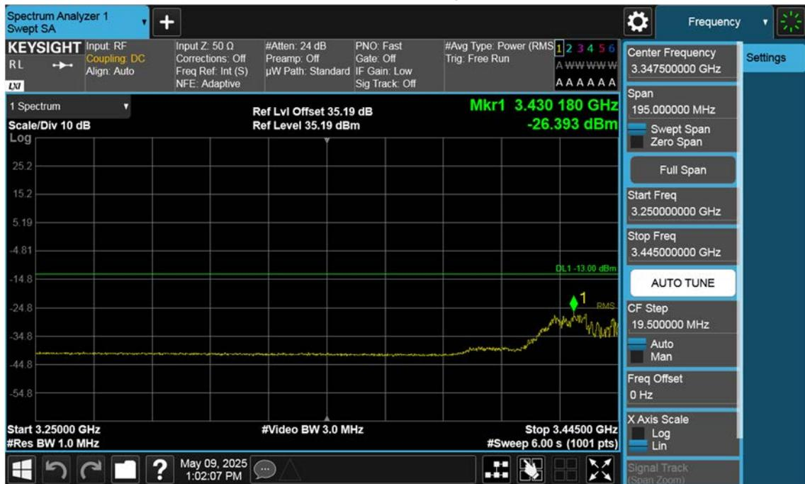
n77(3450~3550 MHz)\_40 M\_Band Edge\_Low\_BPSK\_1RB(3)
