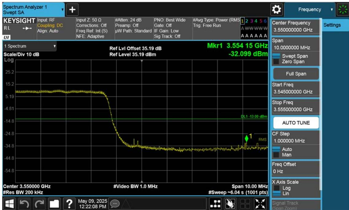
n77(3450~3550 MHz)\_15 M\_Band Edge\_High\_BPSK\_1RB(1)
