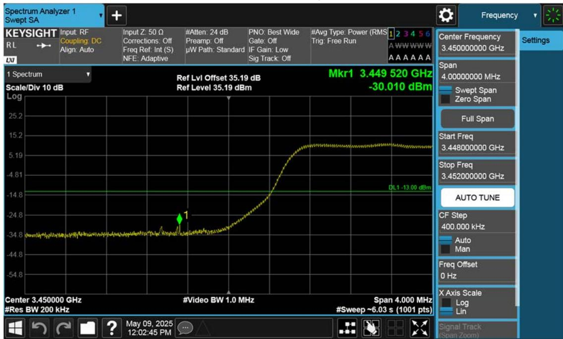
n77(3450~3550 MHz)\_10 M\_Band Edge\_Low\_BPSK\_1RB(1)
