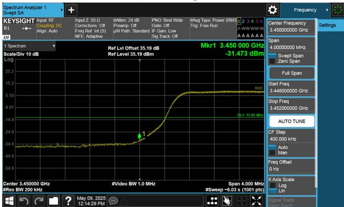
n77(3450~3550 MHz)\_15 M\_Band Edge\_Low\_BPSK\_1RB(1)
