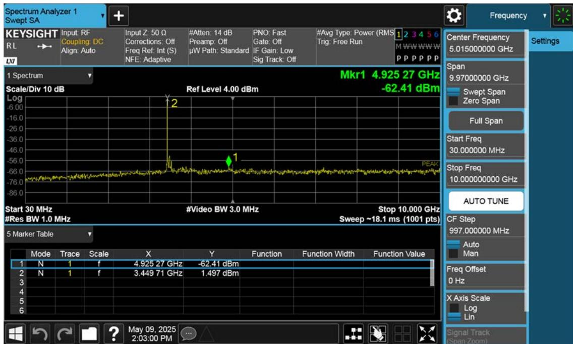
n77(3450~3550 MHz)\_90 M\_Conducted Spurious(30 M-10 G)\_Mid\_BPSK\_1RB
