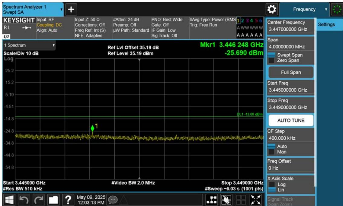
n77(3450~3550 MHz)\_10 M\_Band Edge\_Low\_BPSK\_1RB(2)
