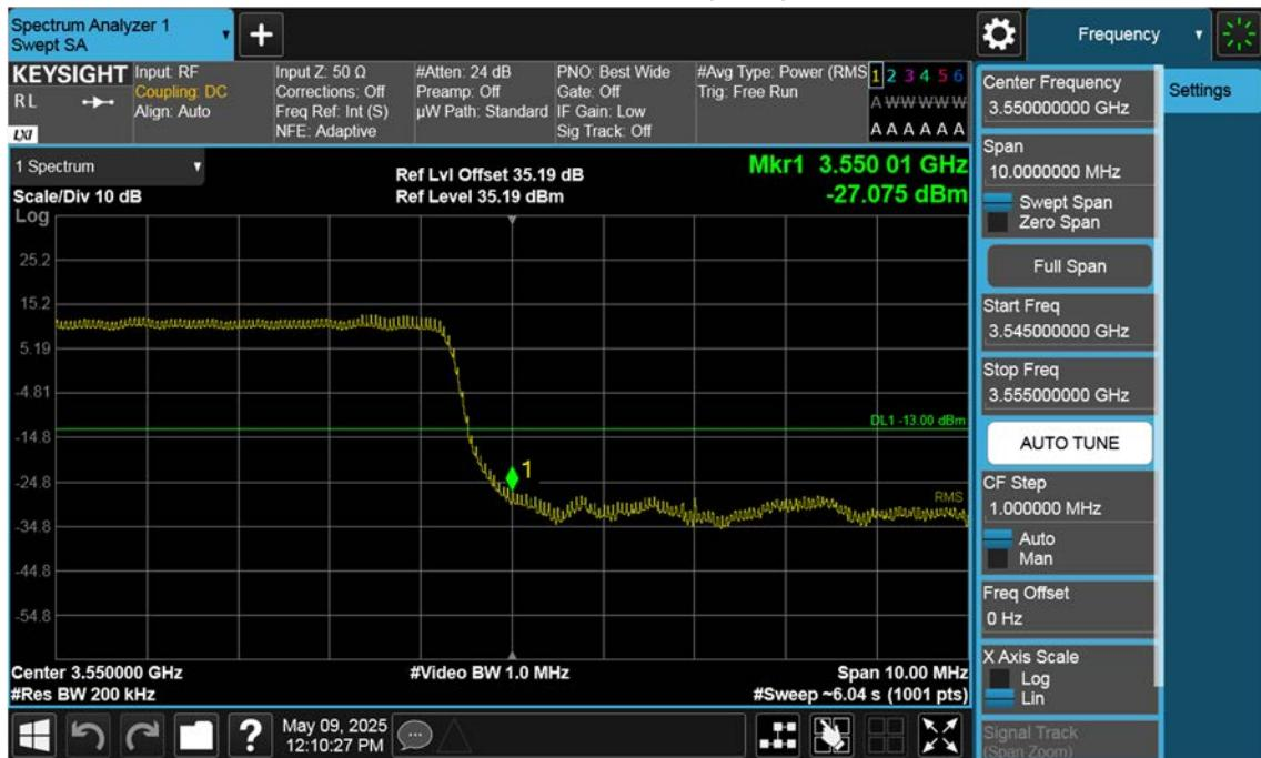
n77(3450~3550 MHz)\_10 M\_Band Edge\_High\_BPSK\_1RB(1)
