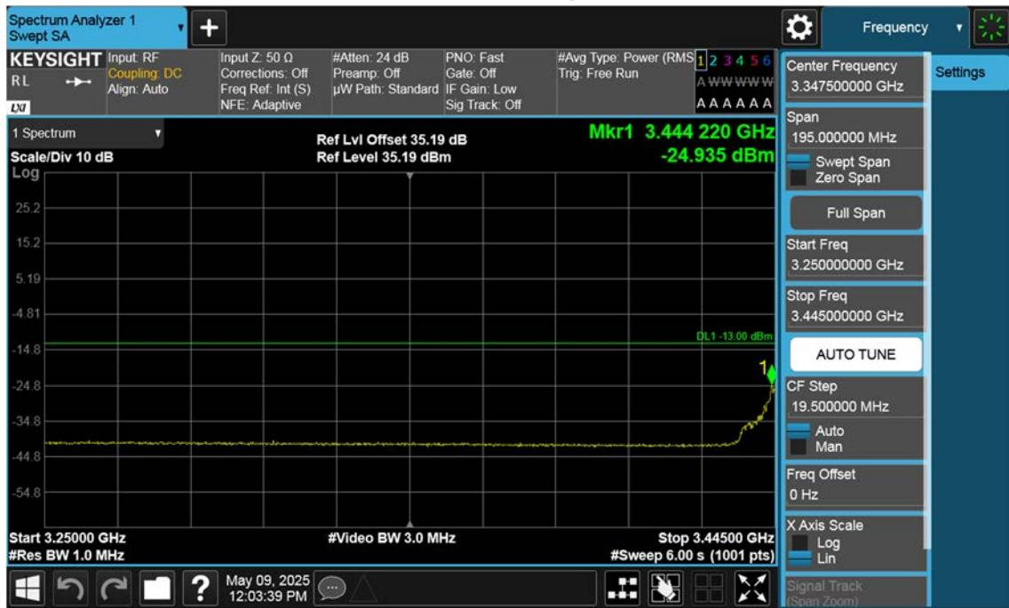
n77(3450~3550 MHz)\_10 M\_Band Edge\_Low\_BPSK\_1RB(3)
