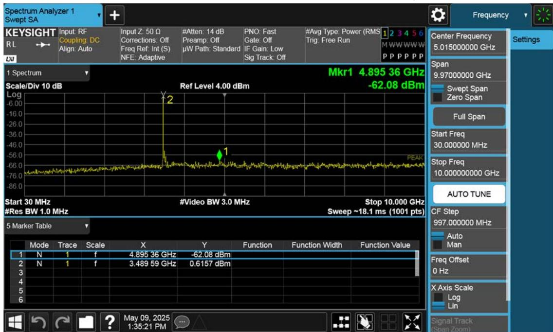
n77(3450~3550 MHz)\_70 M\_Conducted Spurious(30 M-10 G)\_Low\_BPSK\_1RB
