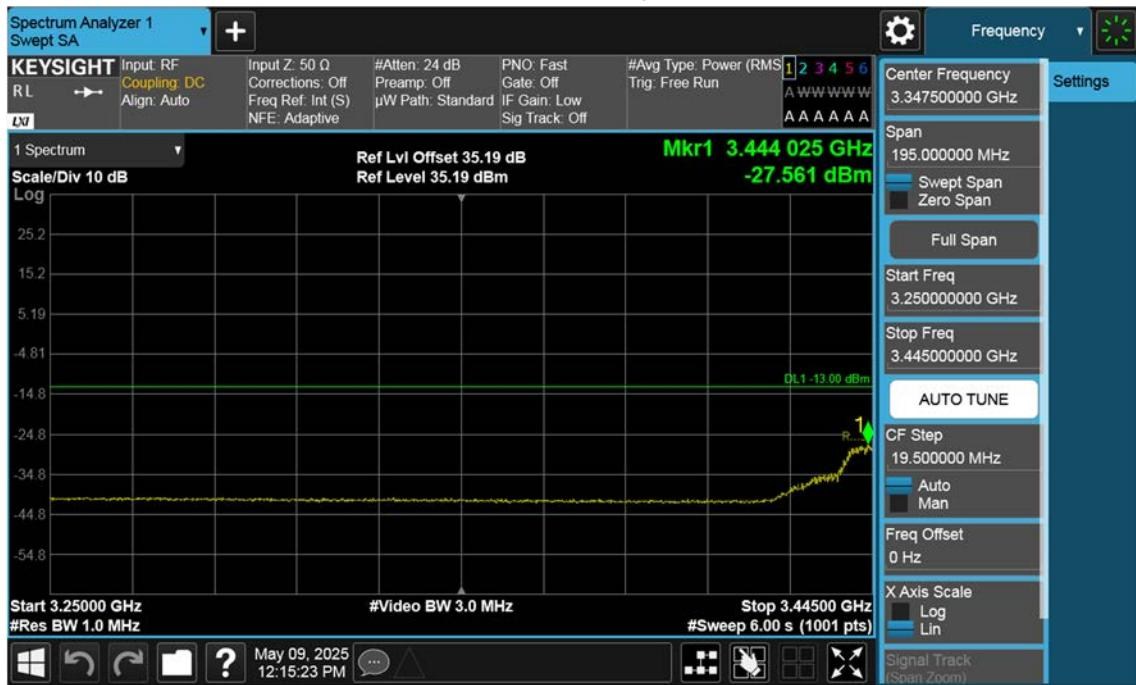
n77(3450~3550 MHz)\_15 M\_Band Edge\_Low\_BPSK\_1RB(3)
