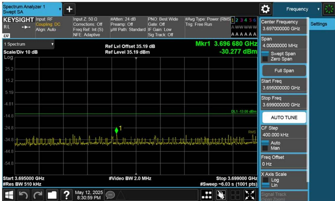
n77(3700~3980 MHz)\_100 M\_Band Edge\_Low\_BPSK\_1RB(2)
