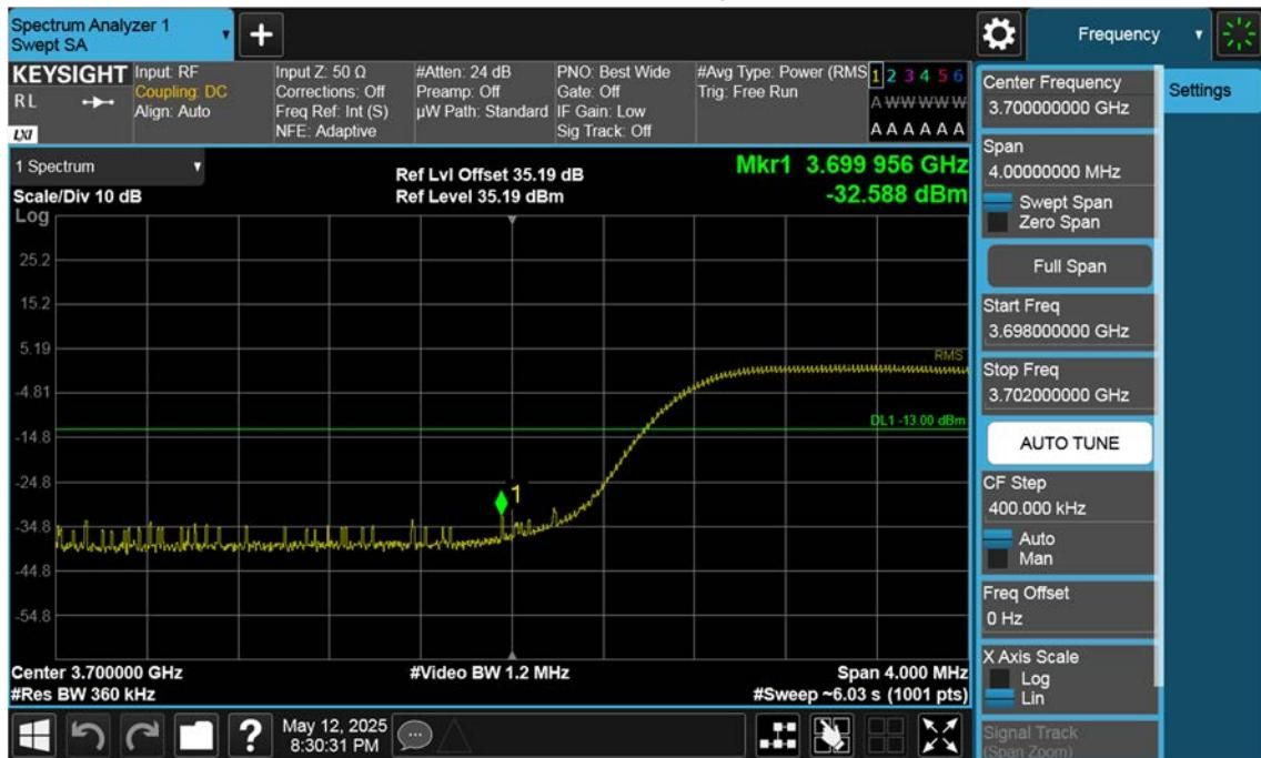
n77(3700~3980 MHz)\_100 M\_Band Edge\_Low\_BPSK\_1RB(1)
