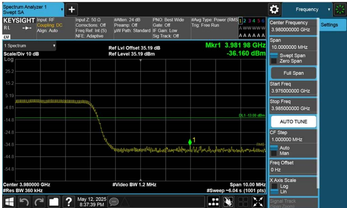
n77(3700~3980 MHz)\_100 M\_Band Edge\_High\_BPSK\_1RB(1)
