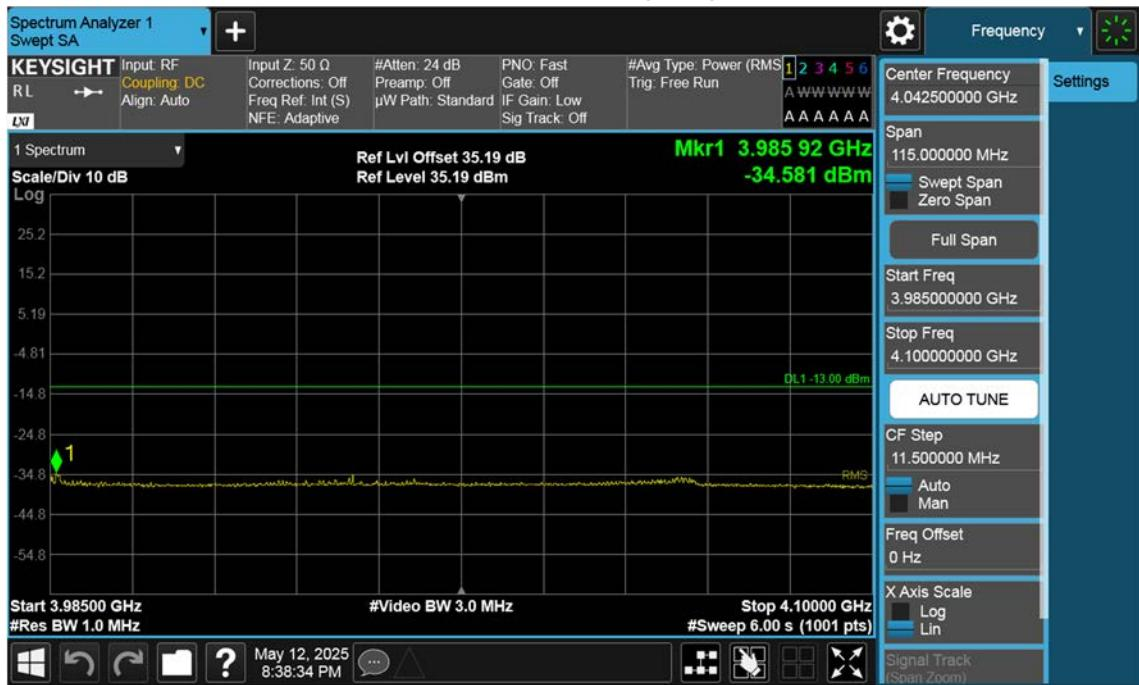
n77(3700~3980 MHz)\_100 M\_Band Edge\_High\_BPSK\_1RB(3)
