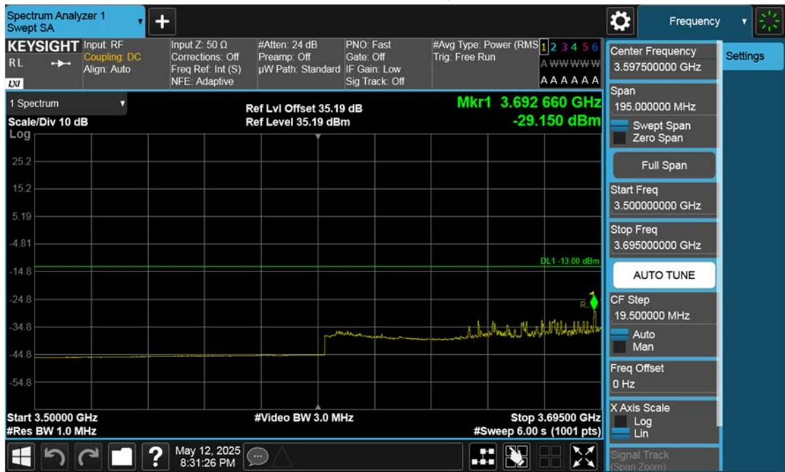
n77(3700~3980 MHz)\_100 M\_Band Edge\_Low\_BPSK\_1RB(3)
