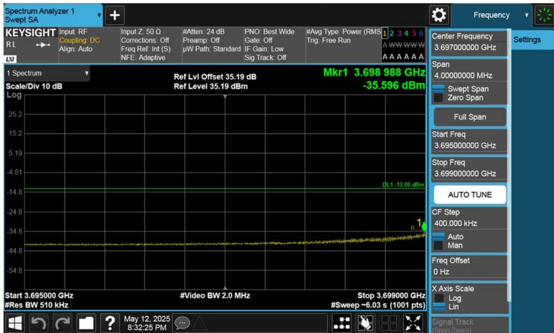
n77(3700~3980 MHz)\_100 M\_Band Edge\_Low\_BPSK\_FullIRB(3)
