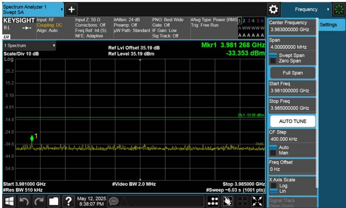
n77(3700~3980 MHz)\_100 M\_Band Edge\_High\_BPSK\_1RB(2)
