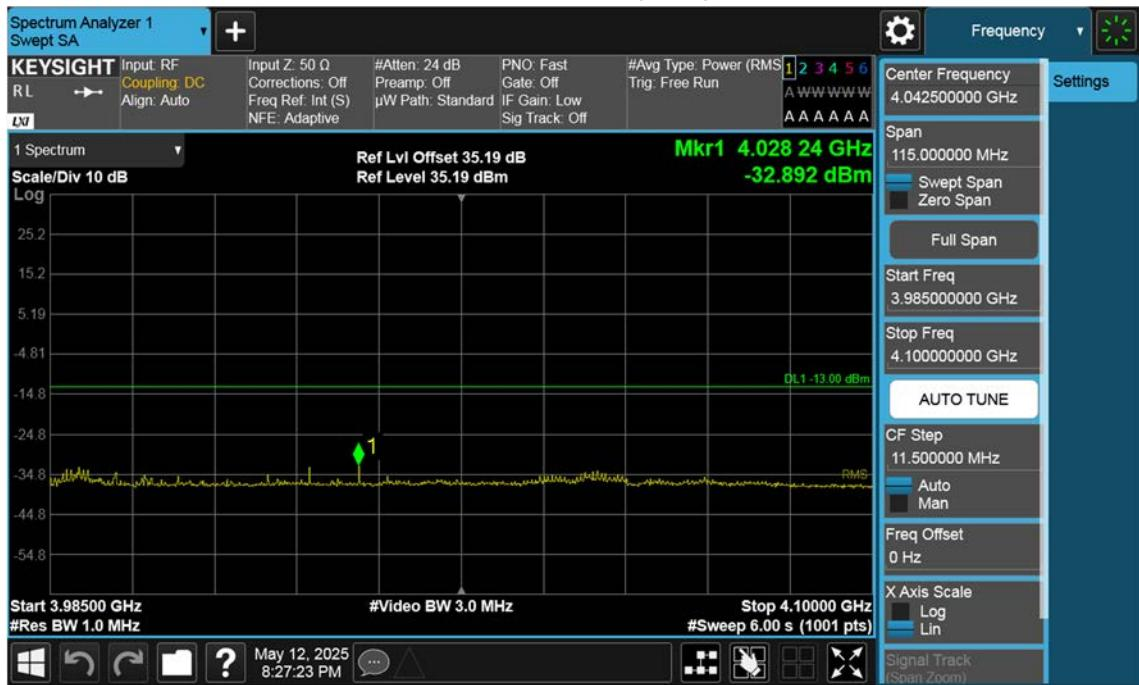
n77(3700~3980 MHz)\_90 M\_Band Edge\_High\_BPSK\_1RB(3)
