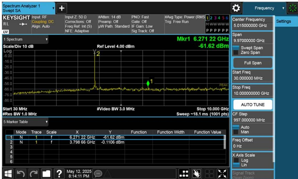
n77(3700~3980 MHz)\_80 M\_Conducted Spurious(30 M-10 G)\_High\_BPSK\_1RB
