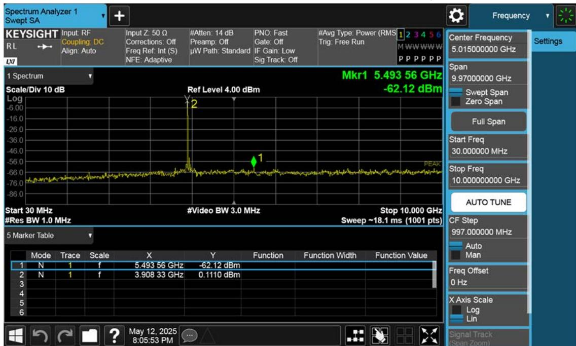
n77(3700~3980 MHz)\_80 M\_Conducted Spurious(30 M-10 G)\_Low\_BPSK\_1RB
