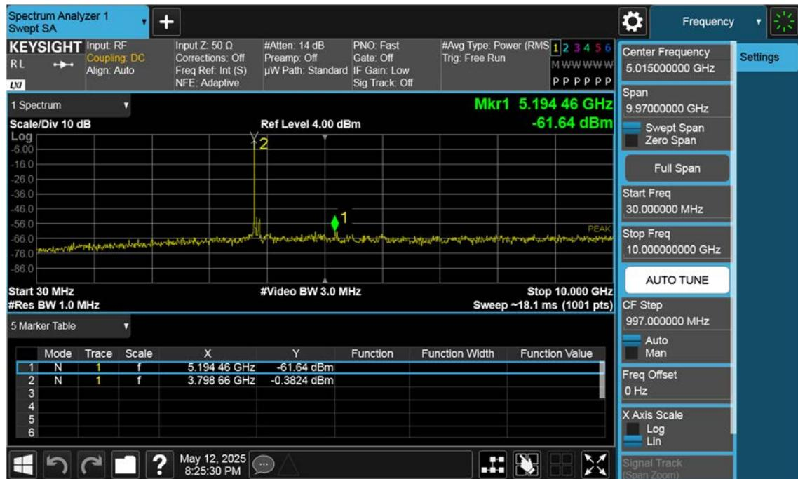
n77(3700~3980 MHz)\_90 M\_Conducted Spurious(30 M-10 G)\_High\_BPSK\_1RB
