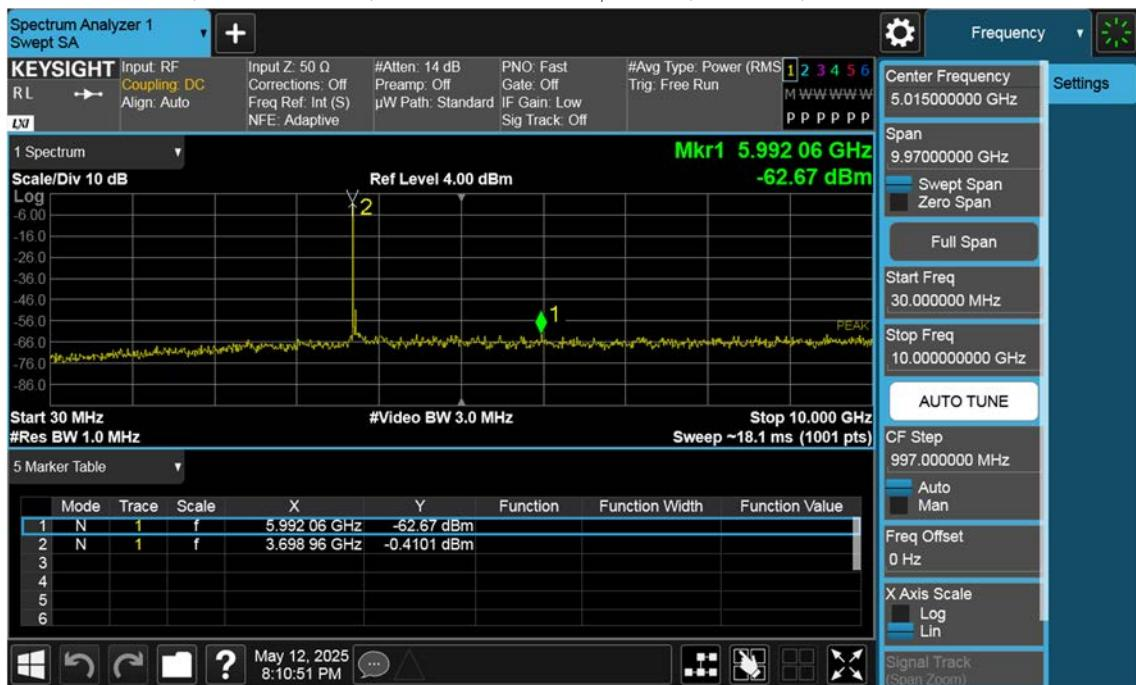
n77(3700~3980 MHz)\_80 M\_Conducted Spurious(30 M-10 G)\_Mid\_BPSK\_1RB
