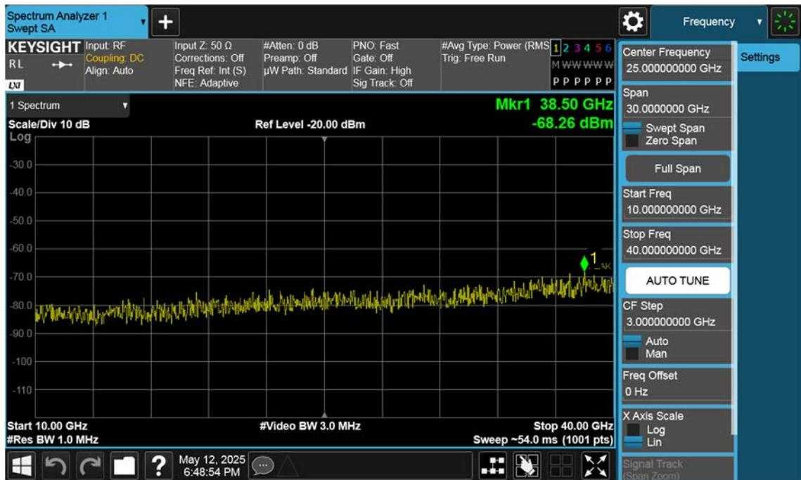
n77(3700~3980 MHz)\_20 M\_Conducted Spurious(Above10 G)\_Mid\_BPSK\_1RB
