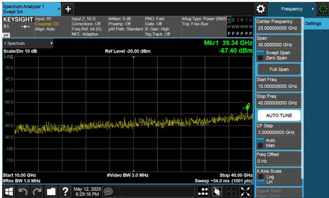
n77(3700~3980 MHz)\_10 M\_Conducted Spurious(Above10 G)\_High\_BPSK\_1RB
