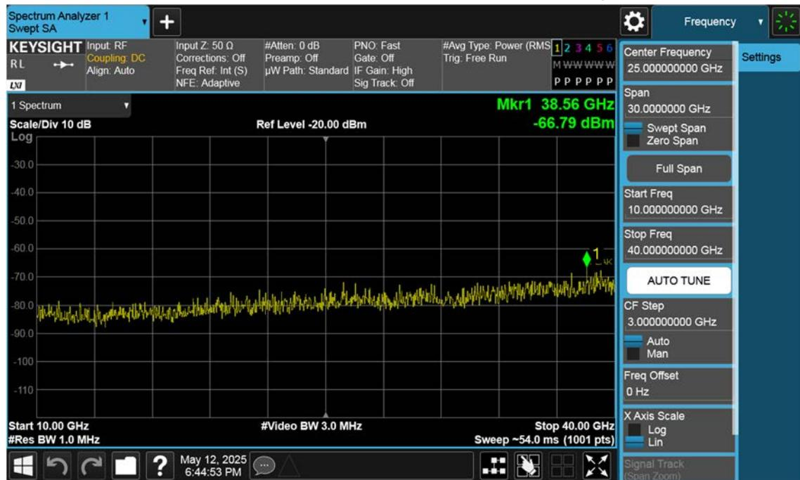
n77(3700~3980 MHz)\_20 M\_Conducted Spurious(Above10 G)\_Low\_BPSK\_1RB
