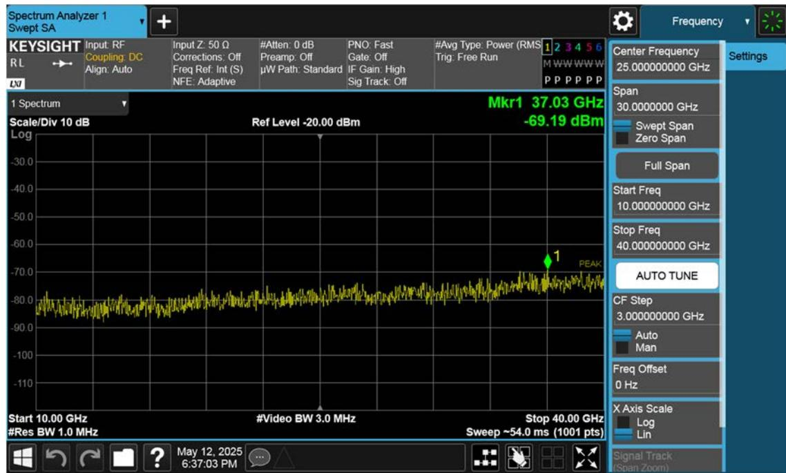
n77(3700~3980 MHz)\_15 M\_Conducted Spurious(Above10 G)\_Mid\_BPSK\_1RB
