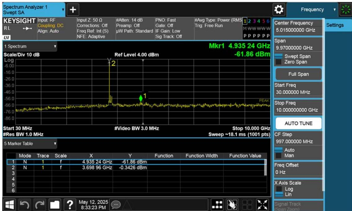
n77(3700~3980 MHz)\_100 M\_Conducted Spurious(30 M-10 G)\_Mid\_BPSK\_1RB
