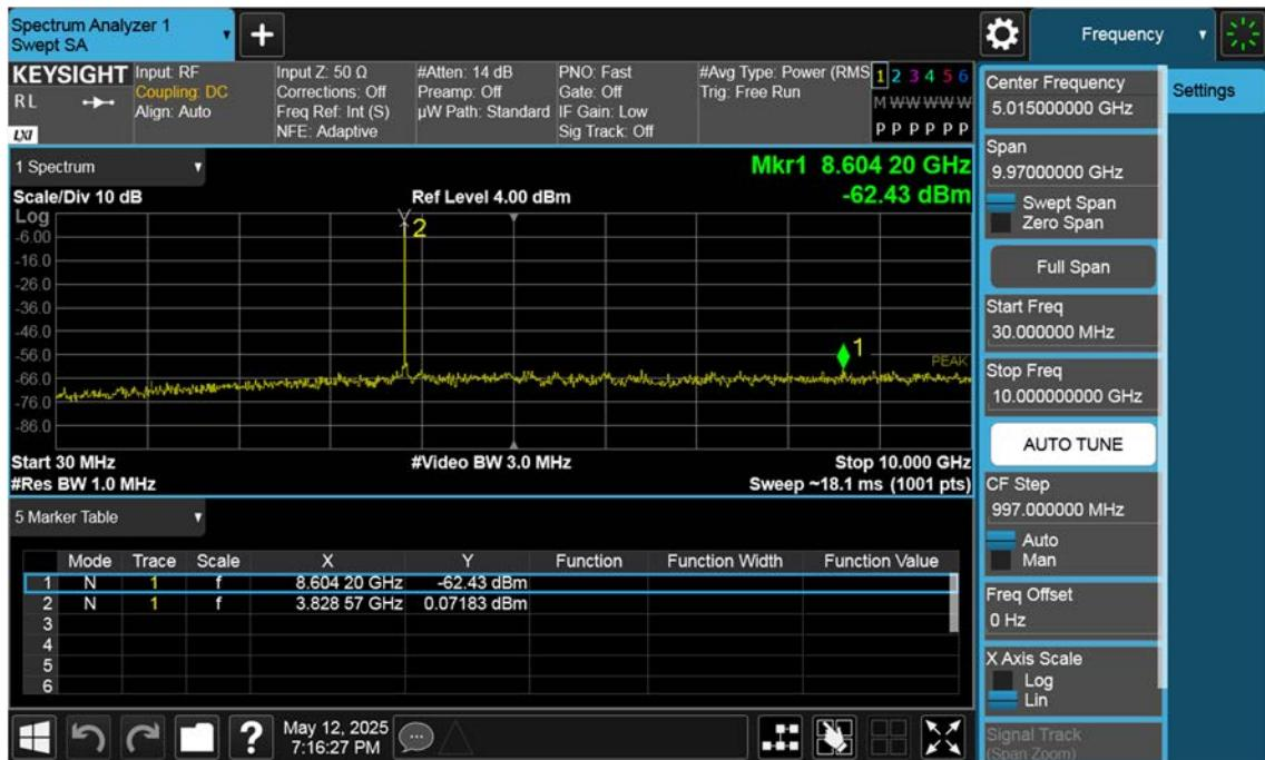
n77(3700~3980 MHz)\_30 M\_Conducted Spurious(30 M-10 G)\_High\_BPSK\_1RB
