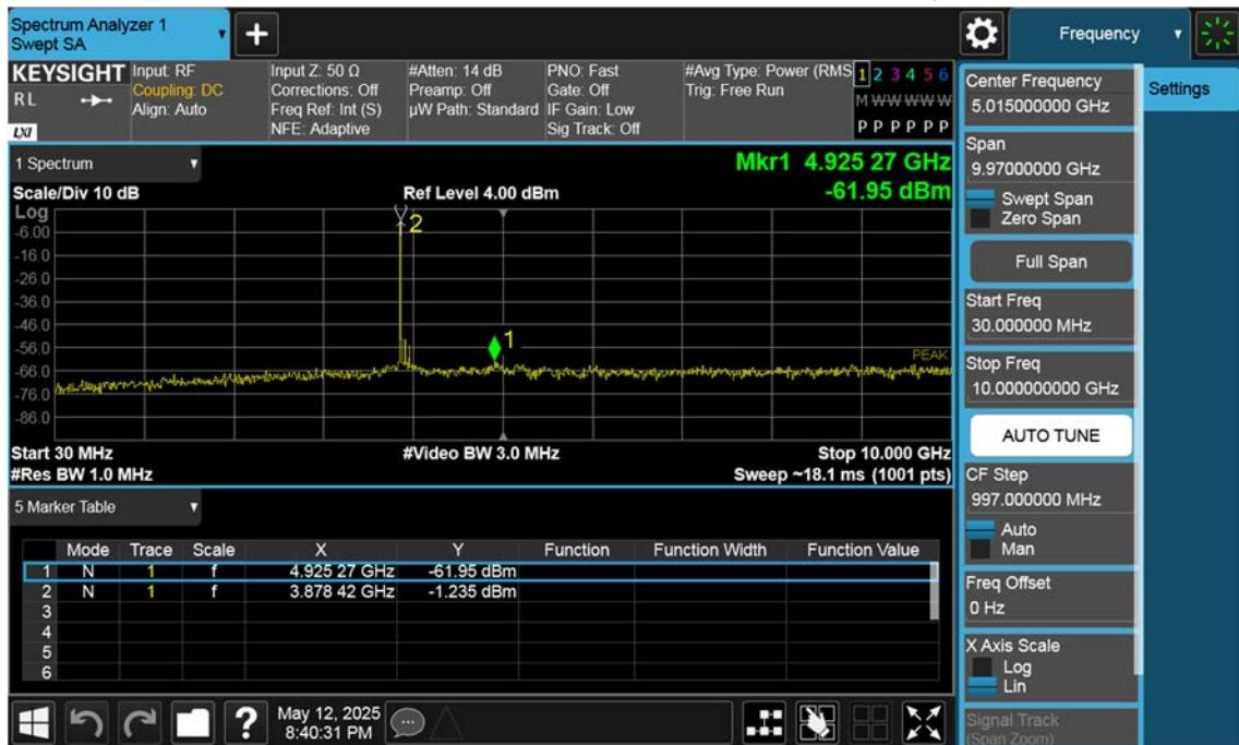
n77(3700~3980 MHz)\_10 M\_Conducted Spurious(Above10 G)\_Low\_BPSK\_1RB
