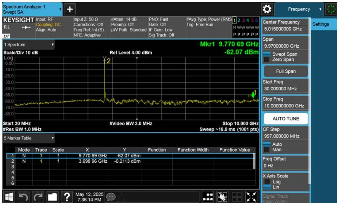
n77(3700~3980 MHz)\_50 M\_Conducted Spurious(30 M-10 G)\_Mid\_BPSK\_1RB
