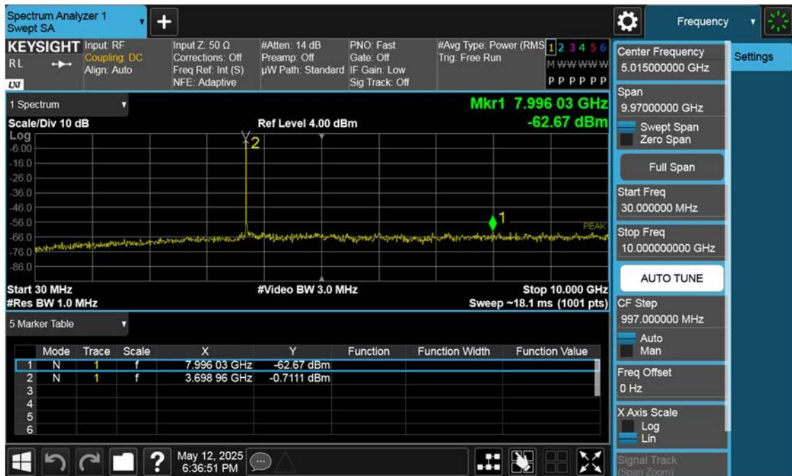
n77(3700~3980 MHz)\_15 M\_Conducted Spurious(30 M-10 G)\_Mid\_BPSK\_1RB
