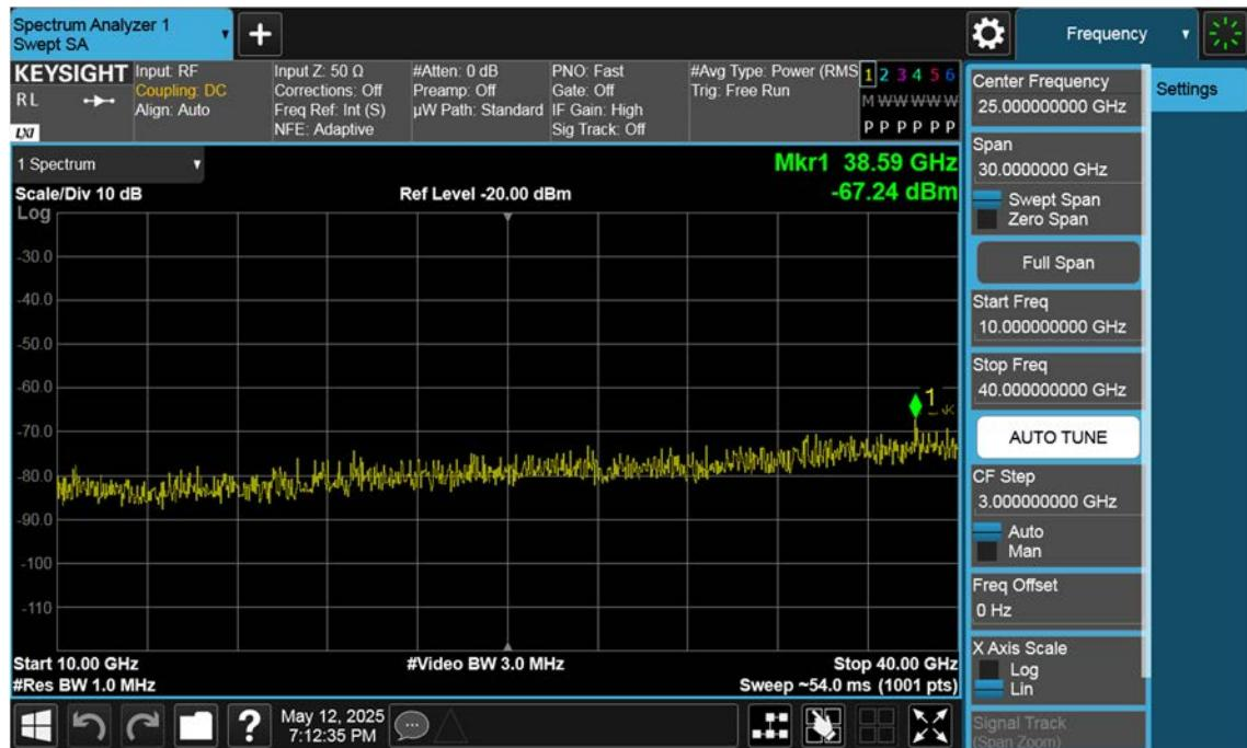
n77(3700~3980 MHz)\_30 M\_Conducted Spurious(Above10 G)\_Mid\_BPSK\_1RB
