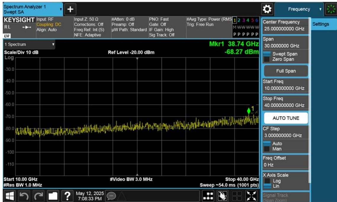
n77(3700~3980 MHz)\_30 M\_Conducted Spurious(Above10 G)\_Low\_BPSK\_1RB
