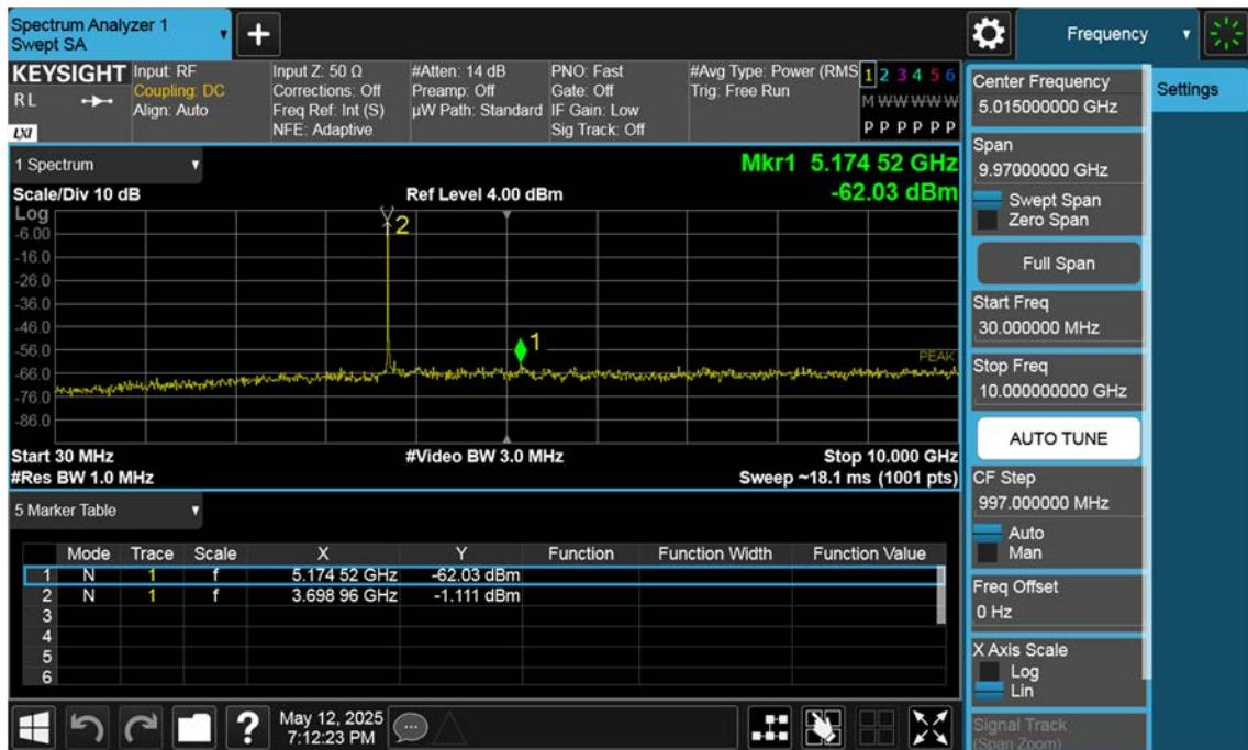
n77(3700~3980 MHz)\_30 M\_Conducted Spurious(30 M-10 G)\_Mid\_BPSK\_1RB
