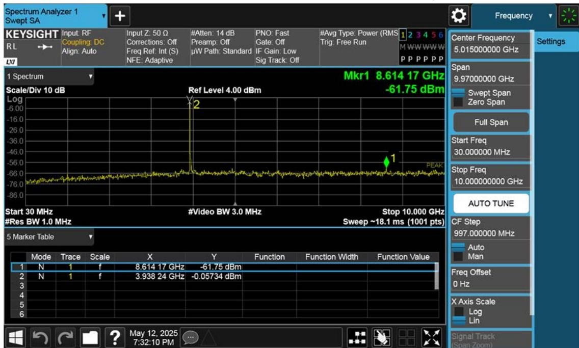
n77(3700~3980 MHz)\_50 M\_Conducted Spurious(30 M-10 G)\_Low\_BPSK\_1RB
