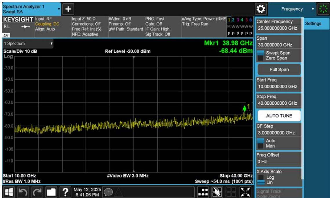
n77(3700~3980 MHz)\_15 M\_Conducted Spurious(Above10 G)\_High\_BPSK\_1RB
