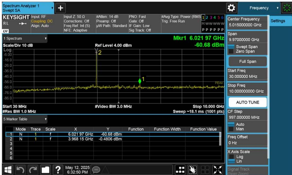
n77(3700~3980 MHz)\_15 M\_Conducted Spurious(30 M-10 G)\_Low\_BPSK\_1RB
