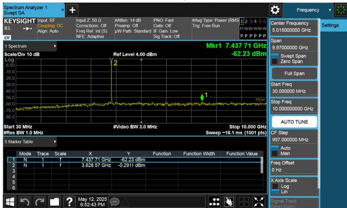
n77(3700~3980 MHz)\_20 M\_Conducted Spurious(30 M-10 G)\_High\_BPSK\_1RB
