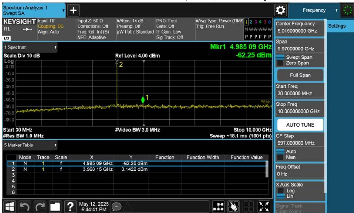
n77(3700~3980 MHz)\_20 M\_Conducted Spurious(30 M-10 G)\_Low\_BPSK\_1RB
