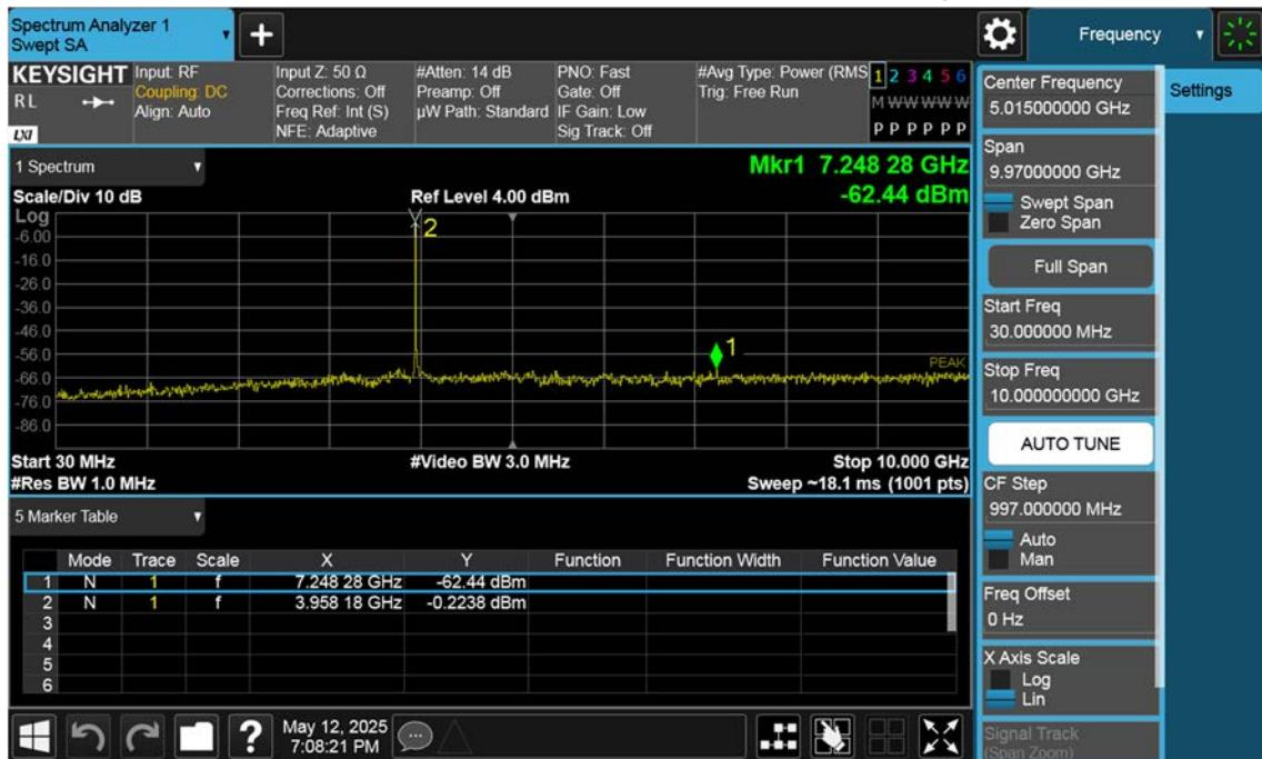
n77(3700~3980 MHz)\_30 M\_Conducted Spurious(30 M-10 G)\_Low\_BPSK\_1RB
