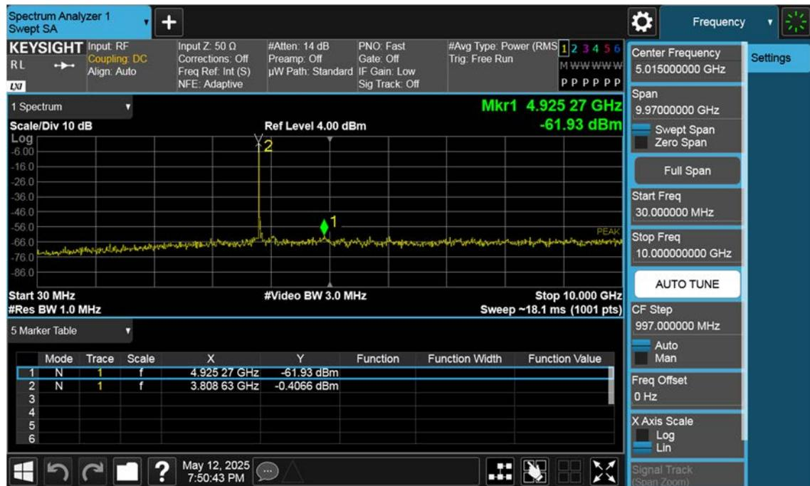
n77(3700~3980 MHz)\_60 M\_Conducted Spurious(30 M-10 G)\_High\_BPSK\_1RB
