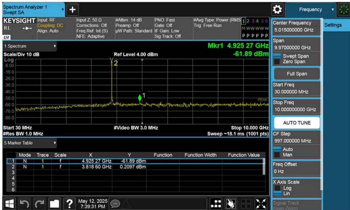
n77(3700~3980 MHz)\_50 M\_Conducted Spurious(30 M-10 G)\_High\_BPSK\_1RB
