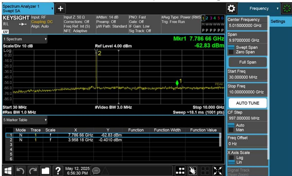
n77(3700~3980 MHz)\_25 M\_Conducted Spurious(30 M-10 G)\_Low\_BPSK\_1RB
