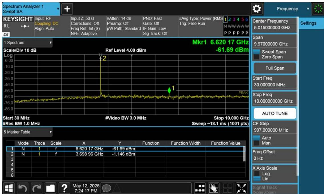
n77(3700~3980 MHz)\_40 M\_Conducted Spurious(30 M-10 G)\_Mid\_BPSK\_1RB
