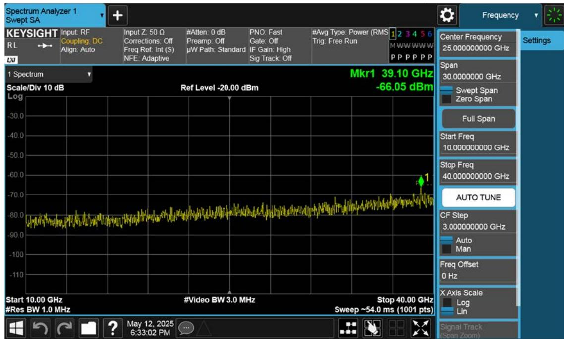
n77(3700~3980 MHz)\_15 M\_Conducted Spurious(Above10 G)\_Low\_BPSK\_1RB
