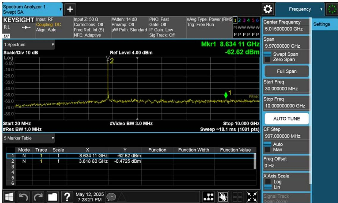
n77(3700~3980 MHz)\_40 M\_Conducted Spurious(30 M-10 G)\_High\_BPSK\_1RB
