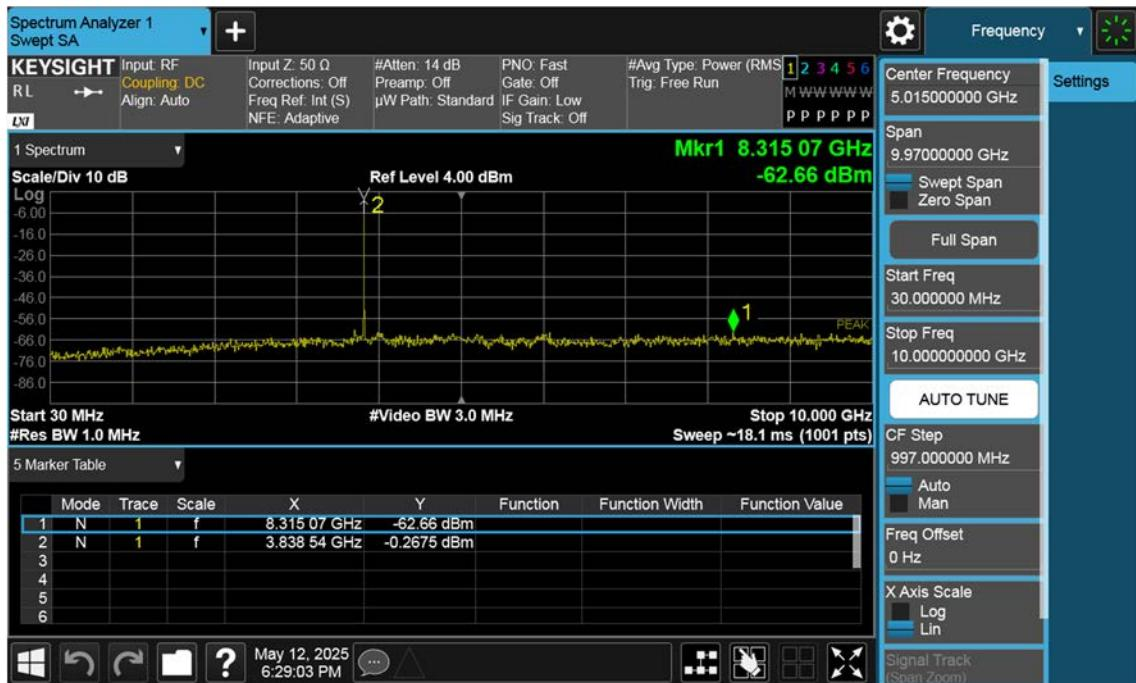
n77(3700~3980 MHz)\_10 M\_Conducted Spurious(30 M-10 G)\_High\_BPSK\_1RB
