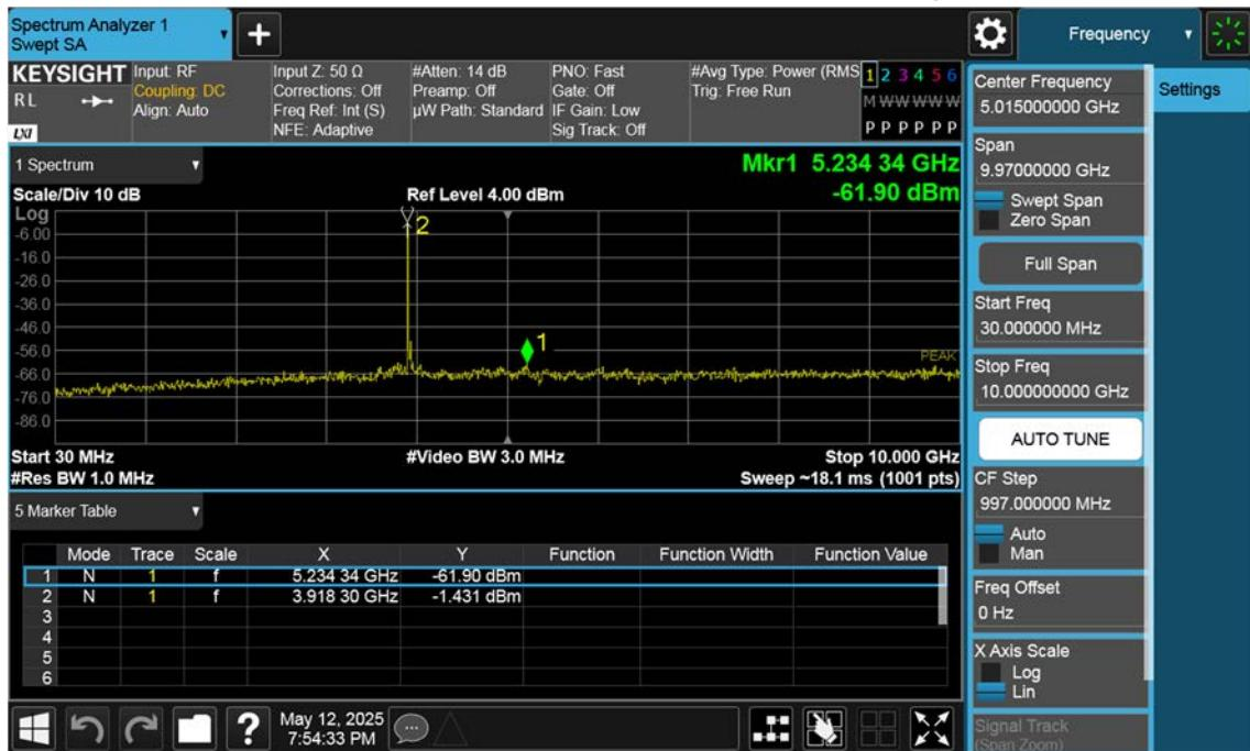
n77(3700~3980 MHz)\_70 M\_Conducted Spurious(30 M-10 G)\_Low\_BPSK\_1RB
