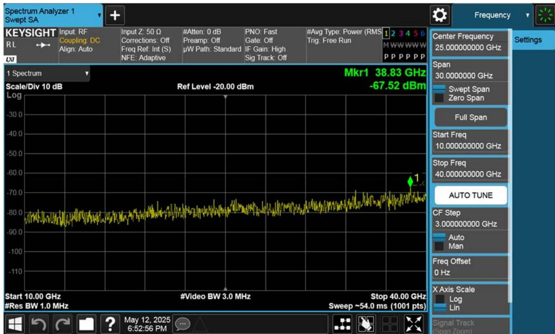
n77(3700~3980 MHz)\_20 M\_Conducted Spurious(Above10 G)\_High\_BPSK\_1RB
