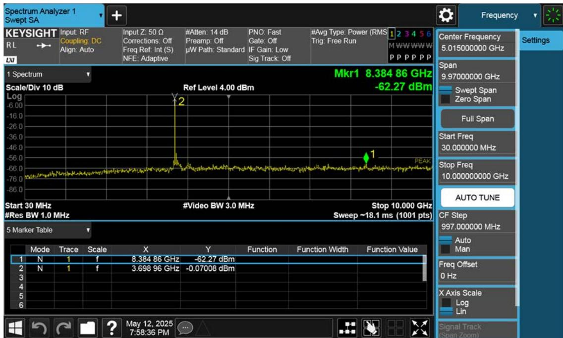
n77(3700~3980 MHz)\_70 M\_Conducted Spurious(30 M-10 G)\_Mid\_BPSK\_1RB
