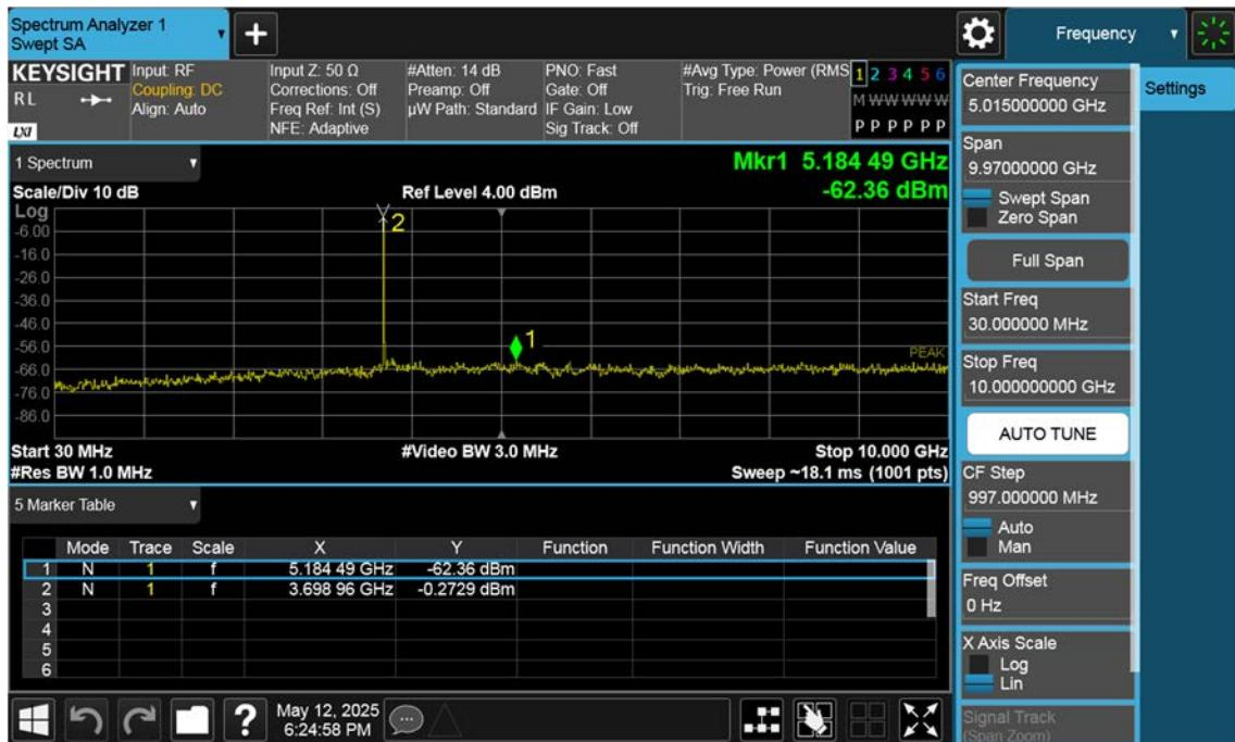
n77(3700~3980 MHz)\_10 M\_Conducted Spurious(30 M-10 G)\_Mid\_BPSK\_1RB
