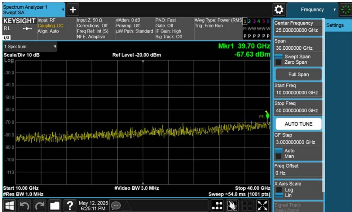
n77(3700~3980 MHz)\_10 M\_Conducted Spurious(Above10 G)\_Mid\_BPSK\_1RB
