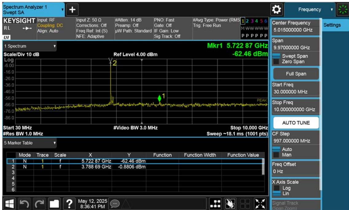
n77(3700~3980 MHz)\_100 M\_Conducted Spurious(30 M-10 G)\_High\_BPSK\_1RB
