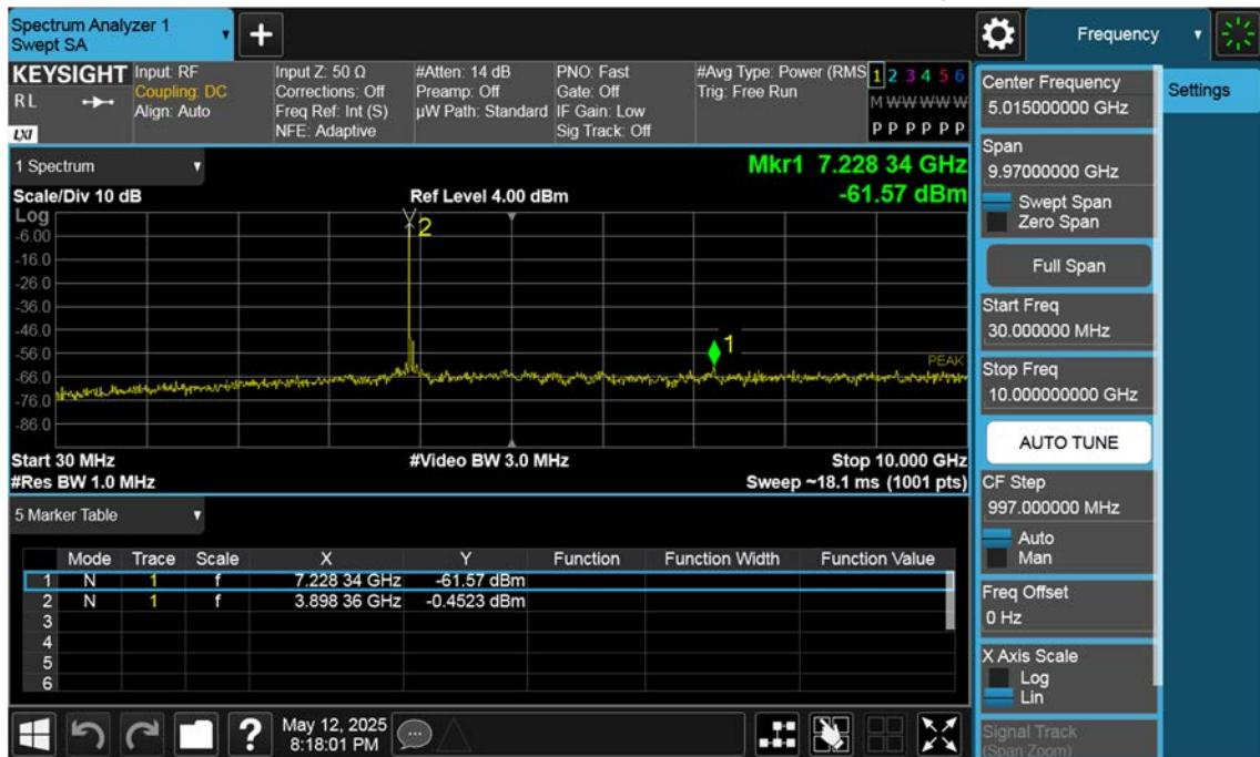
n77(3700~3980 MHz)\_90 M\_Conducted Spurious(30 M-10 G)\_Low\_BPSK\_1RB
