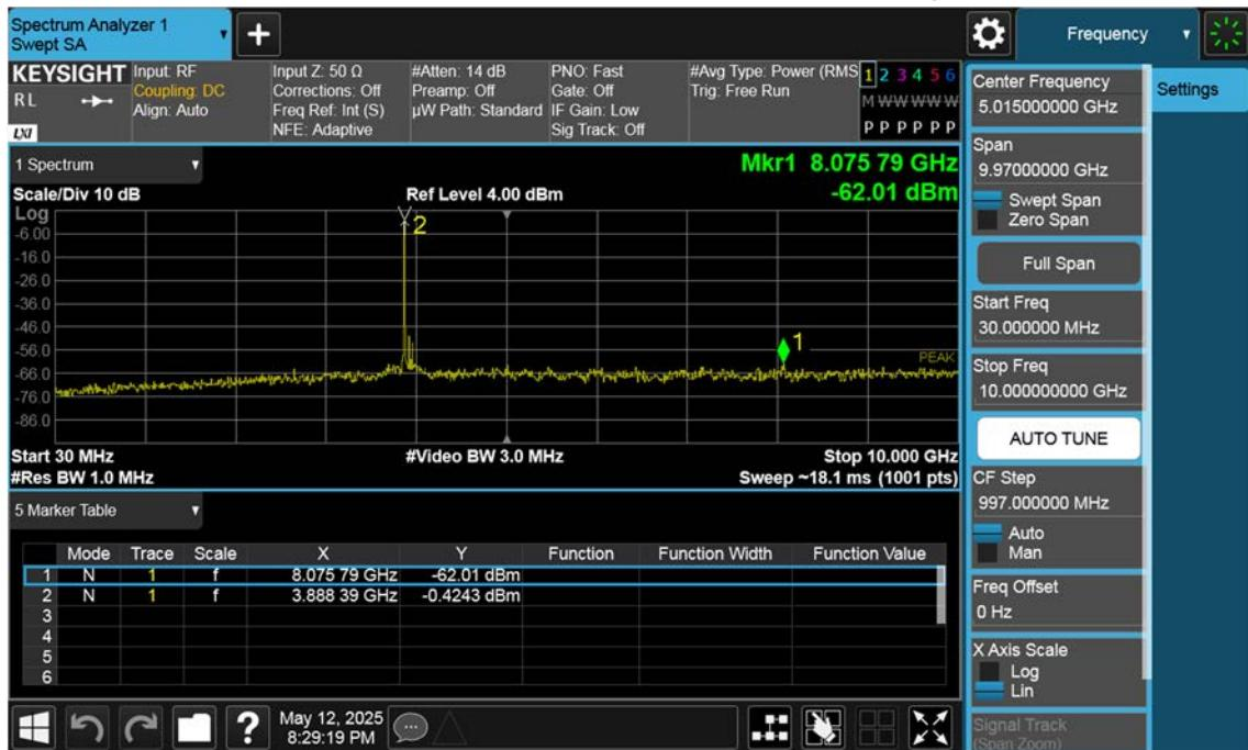
n77(3700~3980 MHz)\_100 M\_Conducted Spurious(30 M-10 G)\_Low\_BPSK\_1RB
