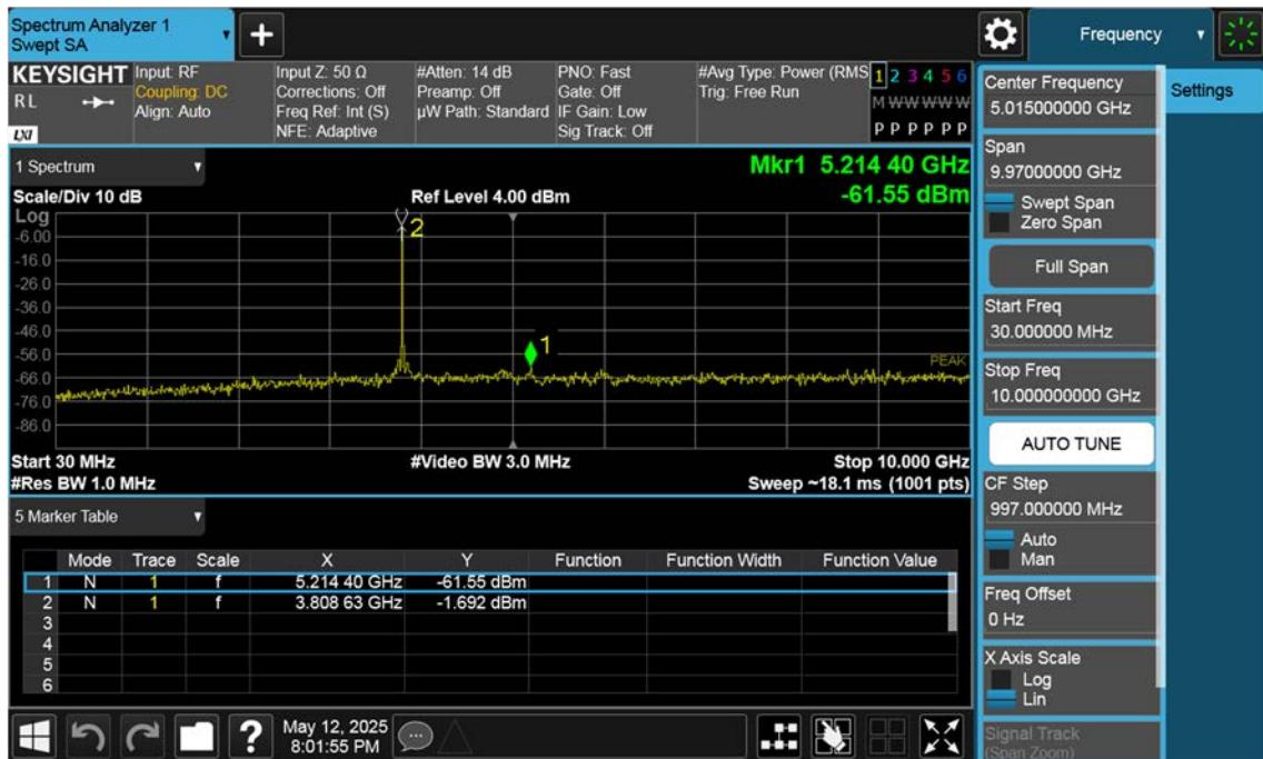
n77(3700~3980 MHz)\_70 M\_Conducted Spurious(30 M-10 G)\_High\_BPSK\_1RB
