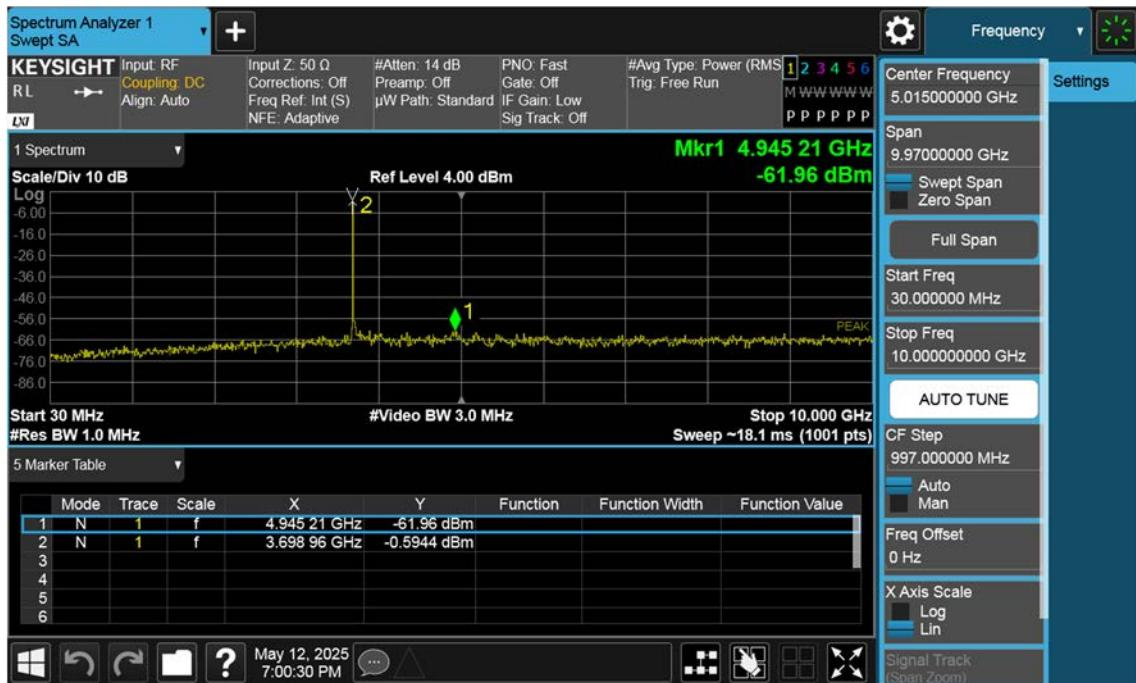
n77(3700~3980 MHz)\_25 M\_Conducted Spurious(30 M-10 G)\_Mid\_BPSK\_1RB
