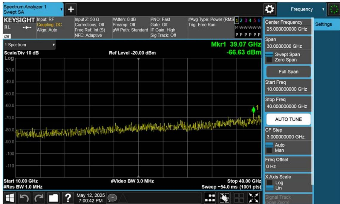
n77(3700~3980 MHz)\_25 M\_Conducted Spurious(Above10 G)\_Mid\_BPSK\_1RB
