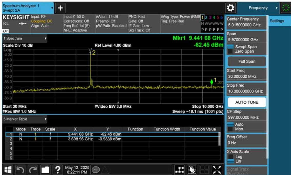
n77(3700~3980 MHz)\_90 M\_Conducted Spurious(30 M-10 G)\_Mid\_BPSK\_1RB
