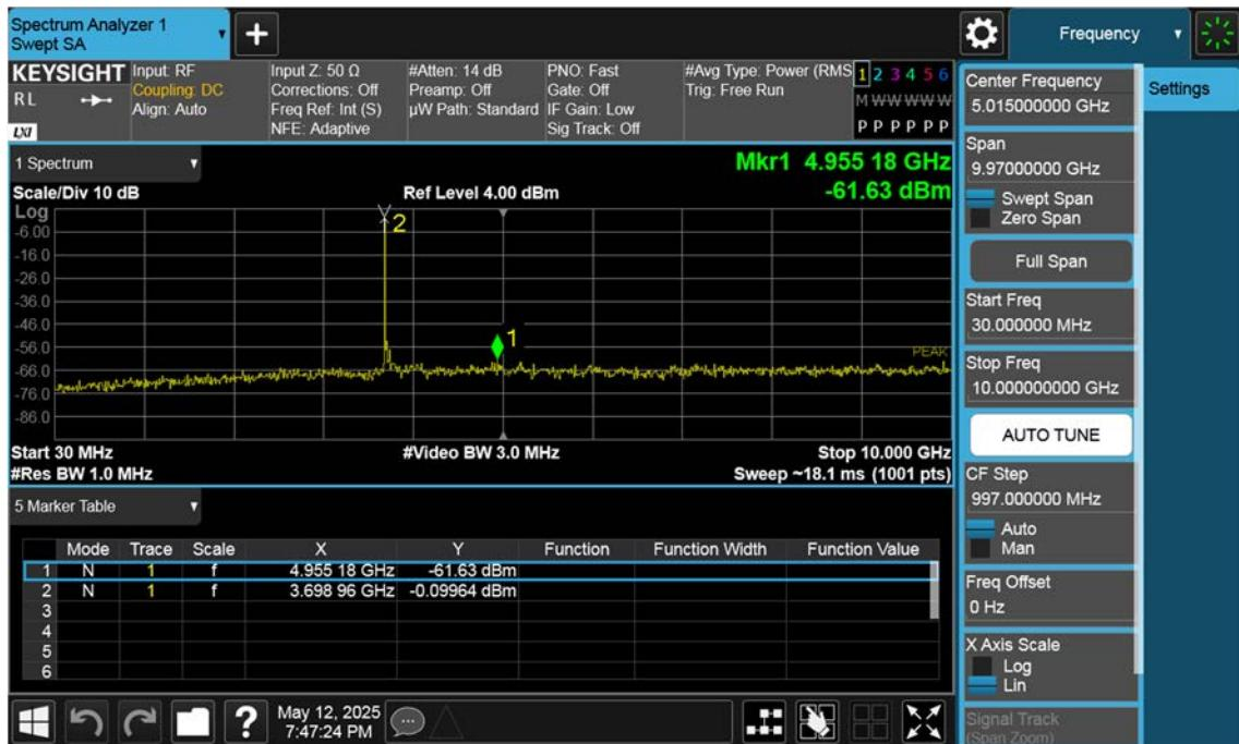
n77(3700~3980 MHz)\_60 M\_Conducted Spurious(30 M-10 G)\_Mid\_BPSK\_1RB
