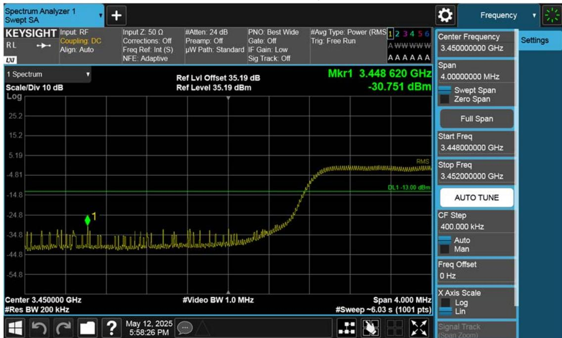
n77(3450~3550 MHz)\_90 M\_Band Edge\_Low\_BPSK\_1RB(1)
