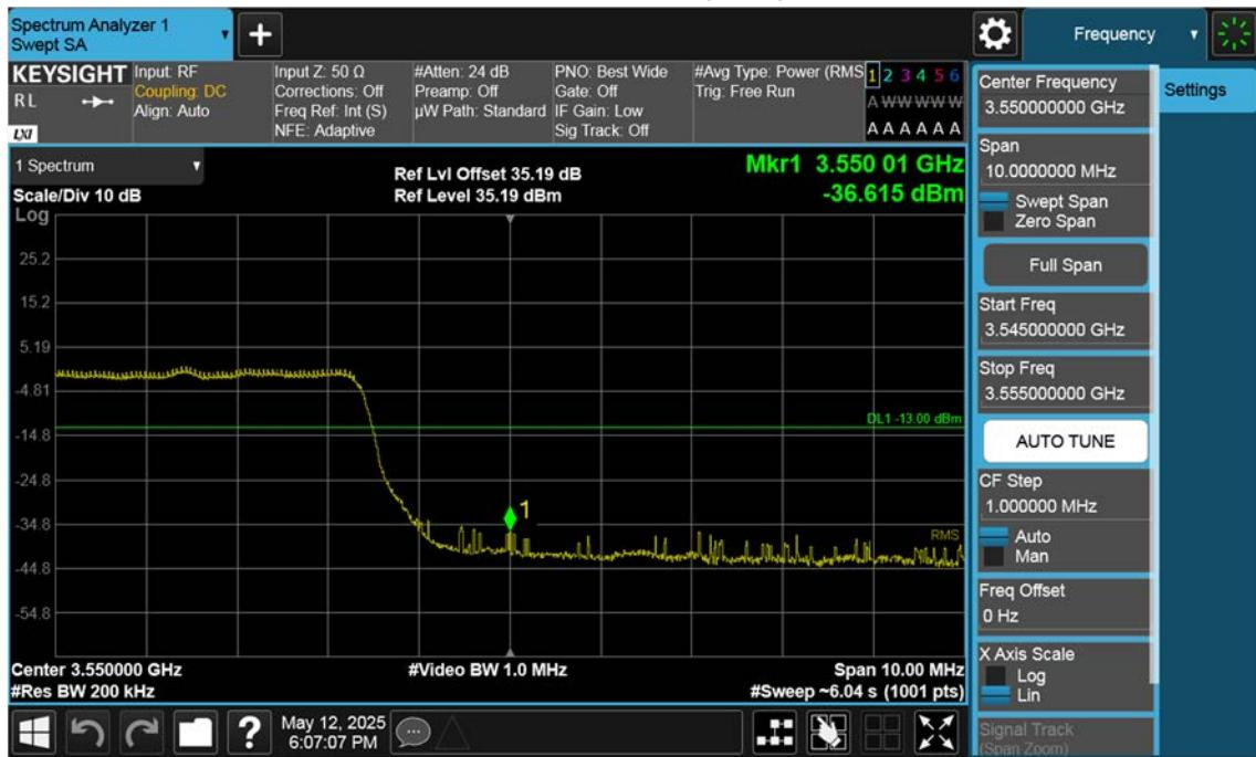
n77(3450~3550 MHz)\_90 M\_Band Edge\_High\_BPSK\_1RB(1)
