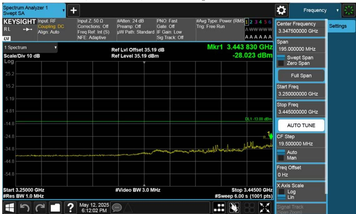
n77(3450~3550 MHz)\_100 M\_Band Edge\_Low\_BPSK\_1RB(3)
