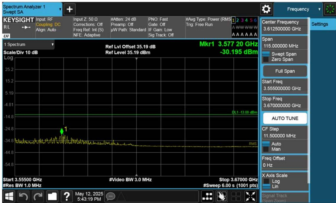
n77(3450~3550 MHz)\_70 M\_Band Edge\_High\_BPSK\_1RB(3)
