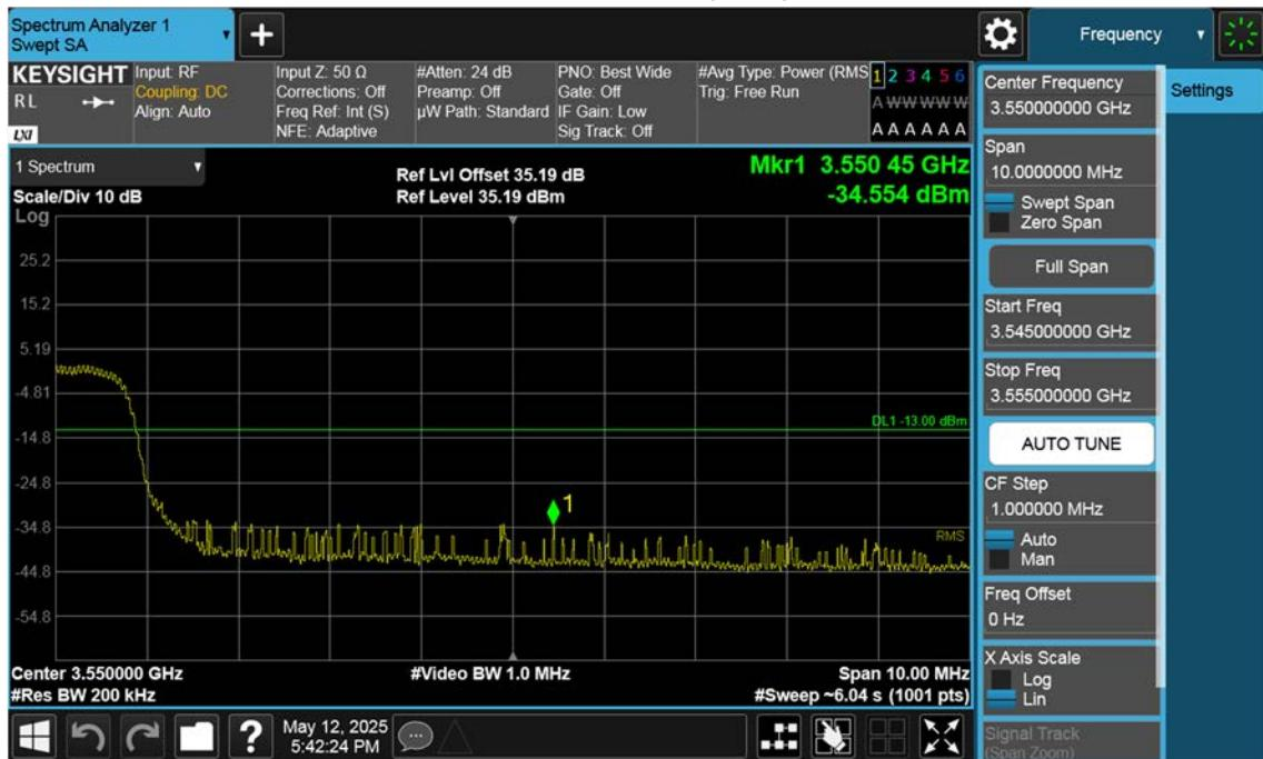
n77(3450~3550 MHz)\_70 M\_Band Edge\_High\_BPSK\_1RB(1)
