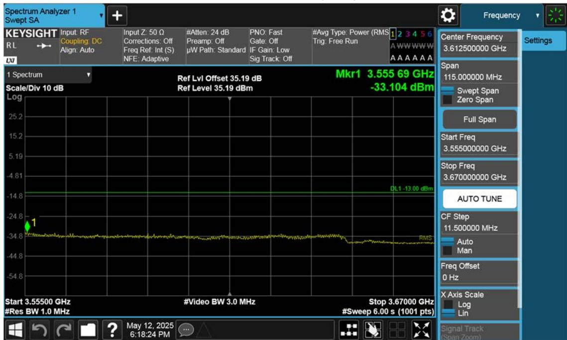
n77(3450~3550 MHz)\_100 M\_Band Edge\_High\_BPSK\_1RB(3)
