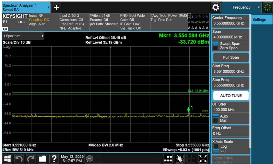
n77(3450~3550 MHz)\_100 M\_Band Edge\_High\_BPSK\_1RB(2)
