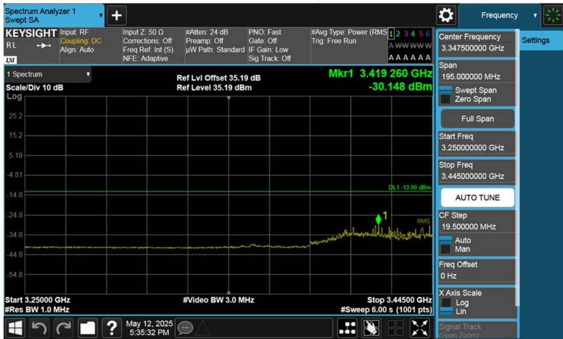
n77(3450~3550 MHz)\_70 M\_Band Edge\_Low\_BPSK\_1RB(3)
