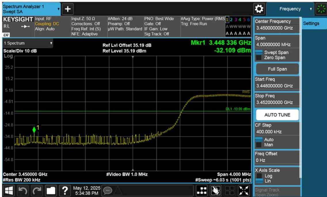
n77(3450~3550 MHz)\_70 M\_Band Edge\_Low\_BPSK\_1RB(1)
