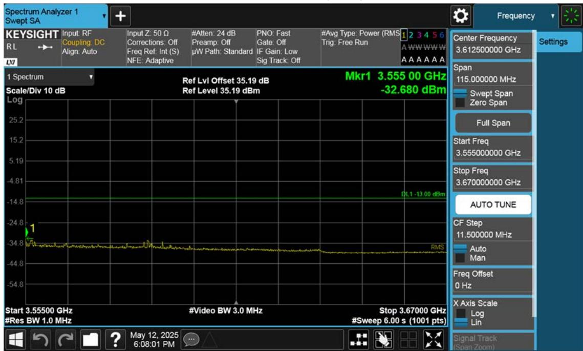
n77(3450~3550 MHz)\_90 M\_Band Edge\_High\_BPSK\_1RB(3)
