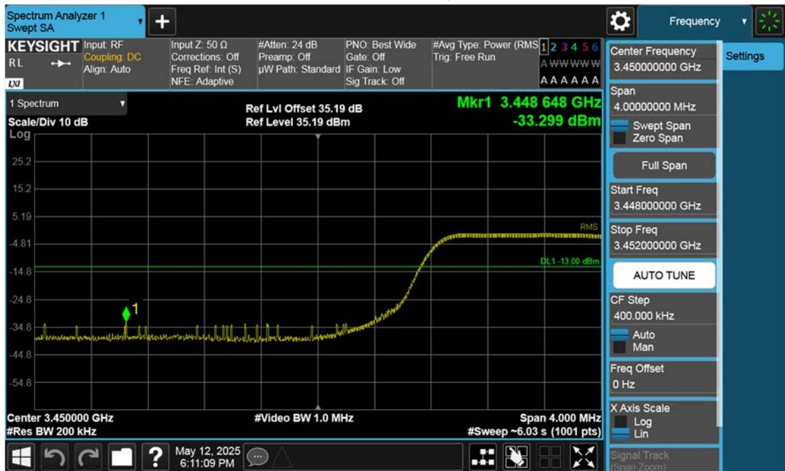
n77(3450~3550 MHz)\_100 M\_Band Edge\_Low\_BPSK\_1RB(1)
