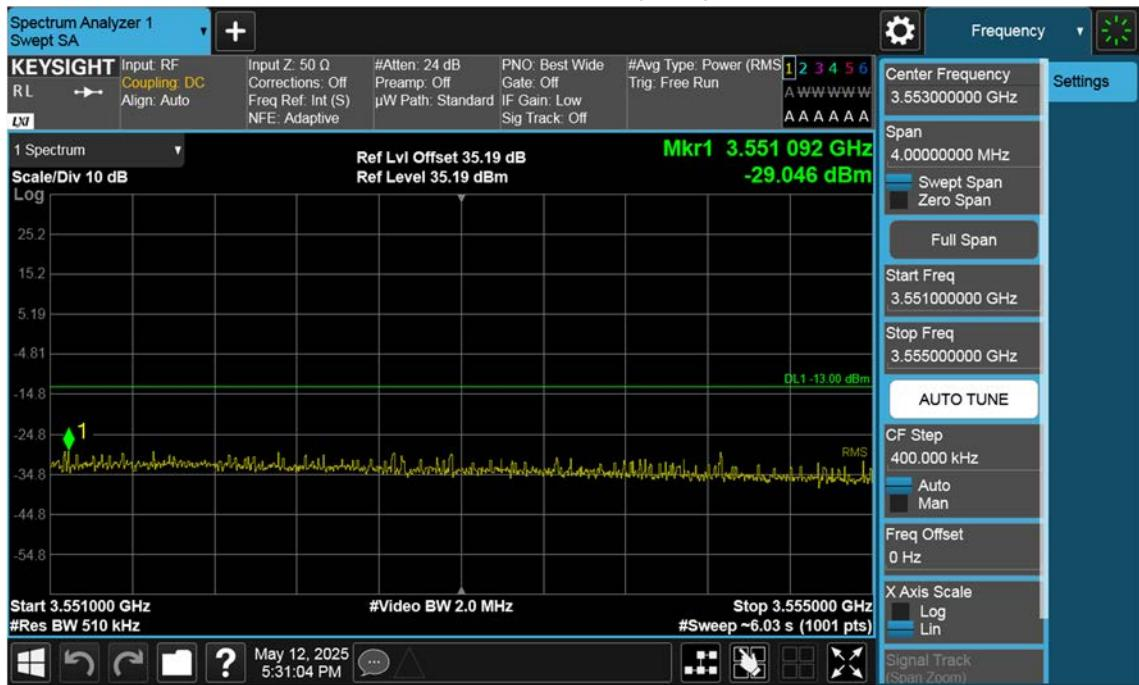
n77(3450~3550 MHz)\_60 M\_Band Edge\_High\_BPSK\_1RB(2)
