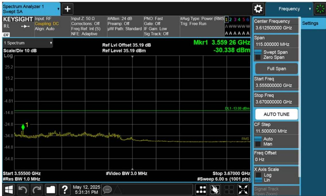
n77(3450~3550 MHz)\_60 M\_Band Edge\_High\_BPSK\_1RB(3)
