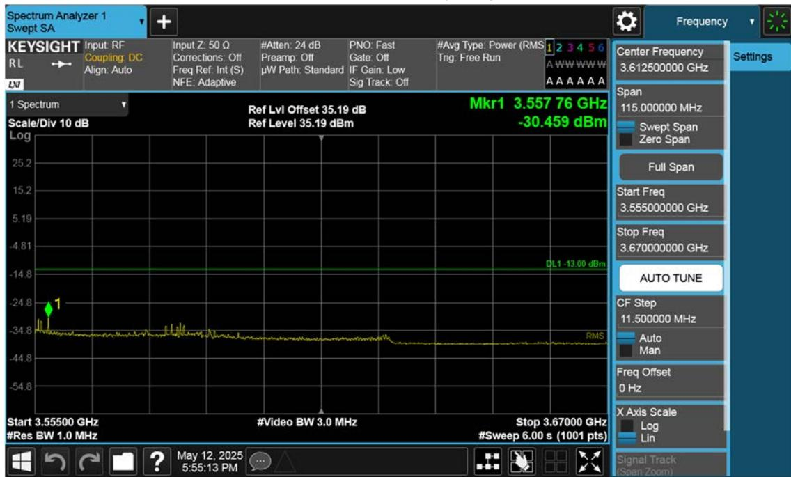
n77(3450~3550 MHz)\_80 M\_Band Edge\_High\_BPSK\_1RB(3)
