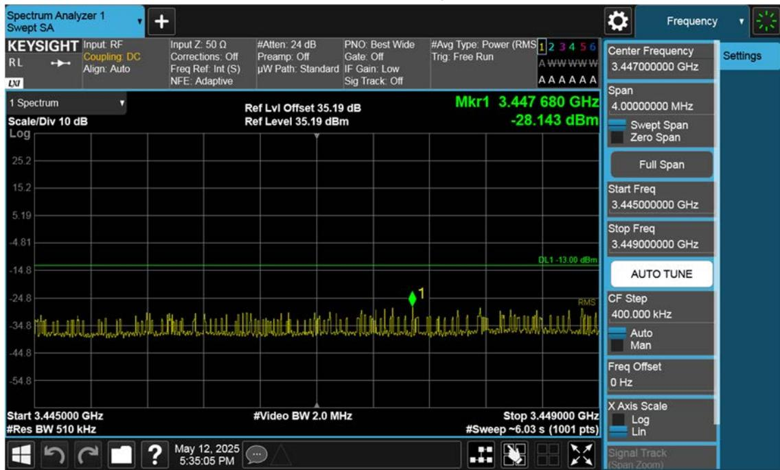
n77(3450~3550 MHz)\_70 M\_Band Edge\_Low\_BPSK\_1RB(2)
