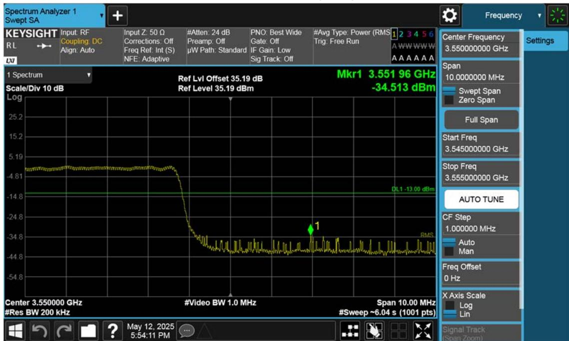
n77(3450~3550 MHz)\_80 M\_Band Edge\_High\_BPSK\_1RB(1)
