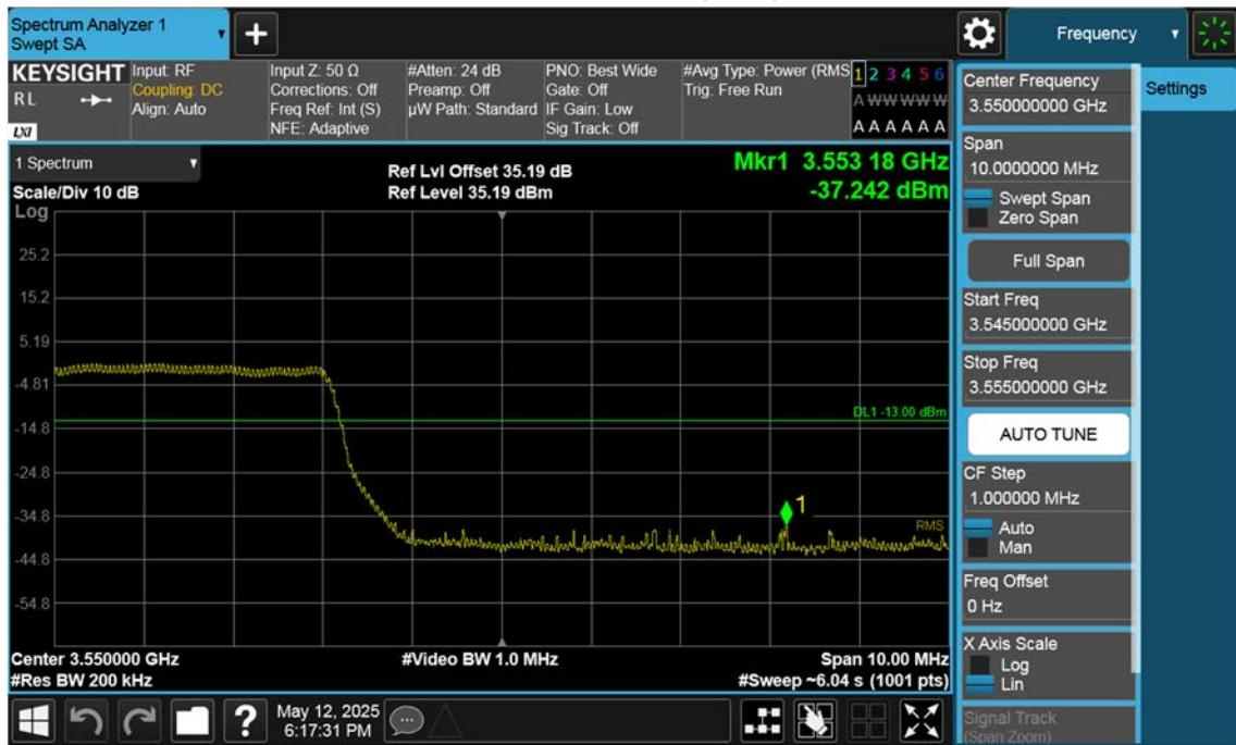
n77(3450~3550 MHz)\_100 M\_Band Edge\_High\_BPSK\_1RB(1)
