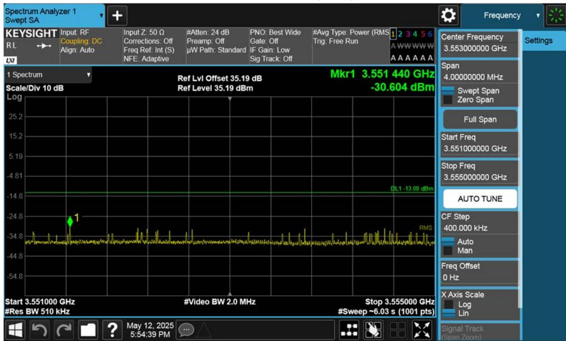
n77(3450~3550 MHz)\_80 M\_Band Edge\_High\_BPSK\_1RB(2)
