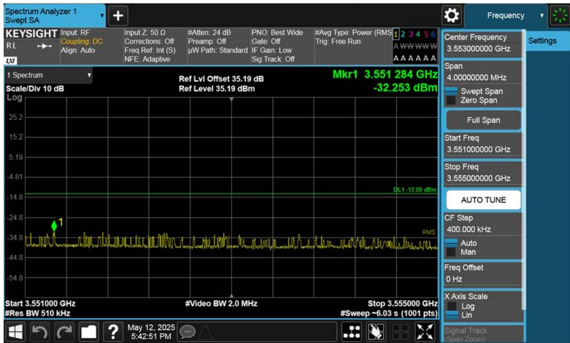
n77(3450~3550 MHz)\_70 M\_Band Edge\_High\_BPSK\_1RB(2)
