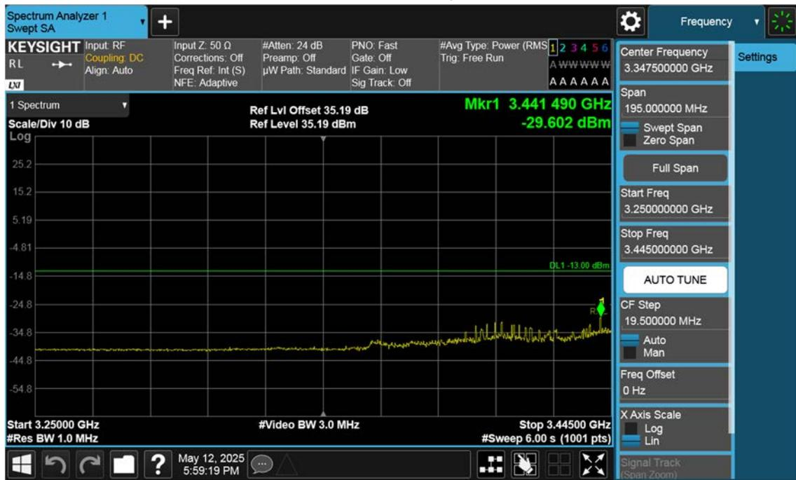
n77(3450~3550 MHz)\_90 M\_Band Edge\_Low\_BPSK\_1RB(3)
