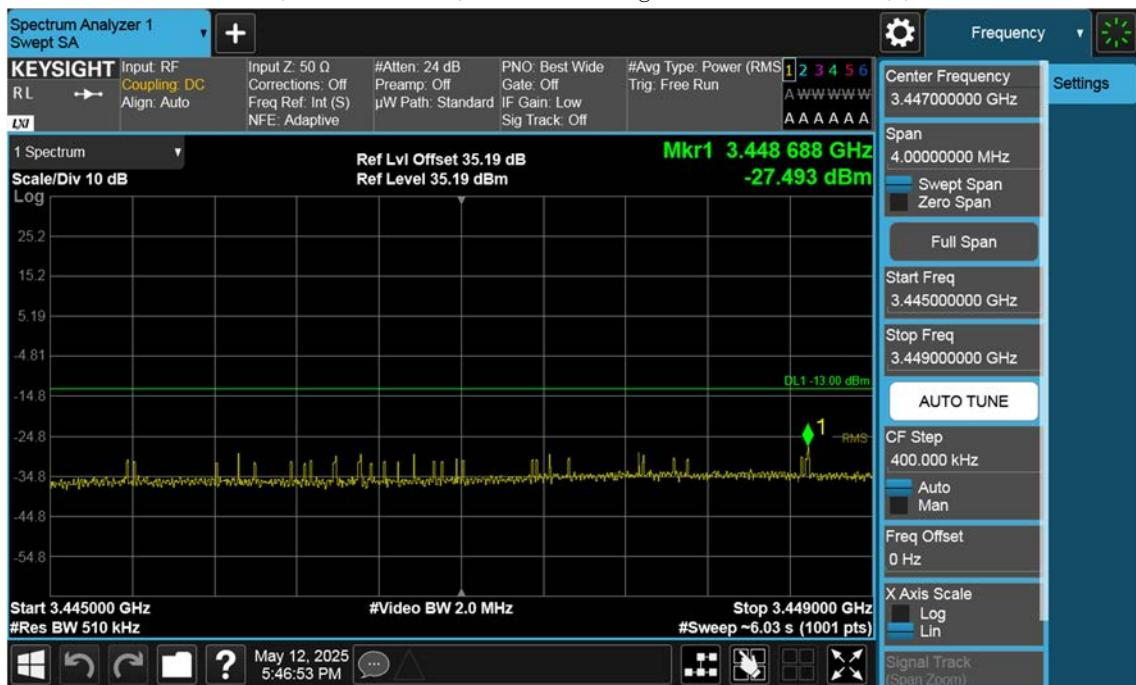
n77(3450~3550 MHz)\_80 M\_Band Edge\_Low\_BPSK\_1RB(2)
