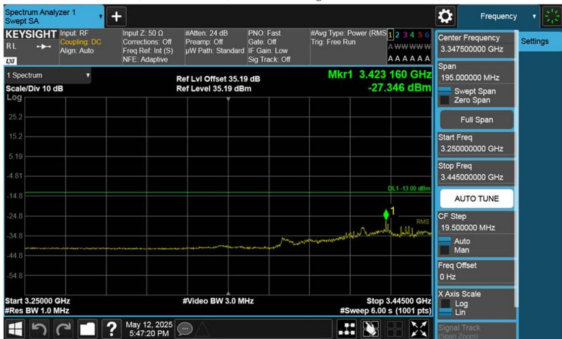
n77(3450~3550 MHz)\_80 M\_Band Edge\_Low\_BPSK\_1RB(3)
