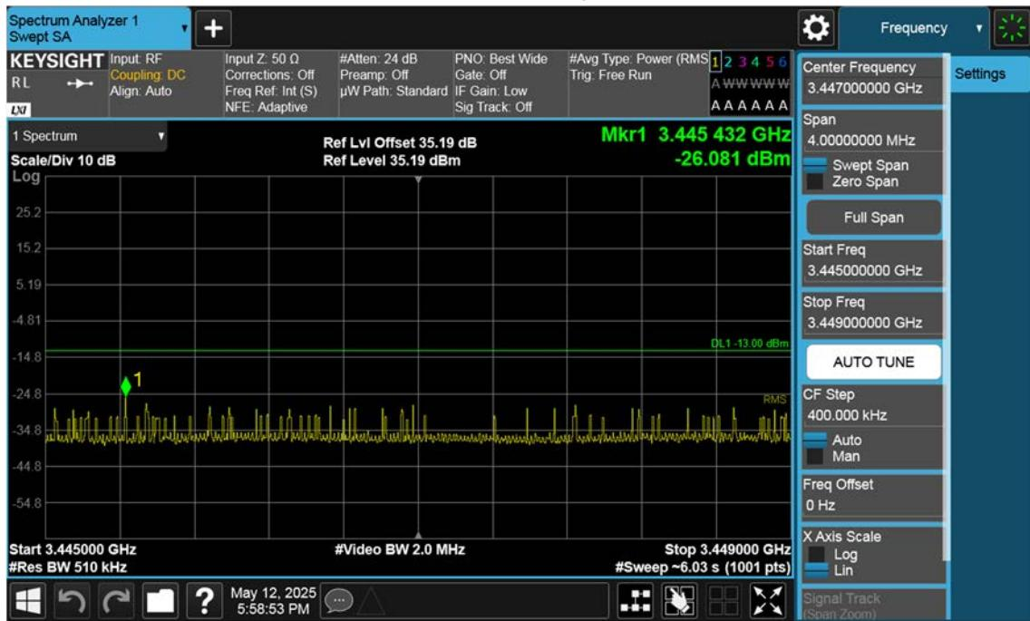
n77(3450~3550 MHz)\_90 M\_Band Edge\_Low\_BPSK\_1RB(2)
