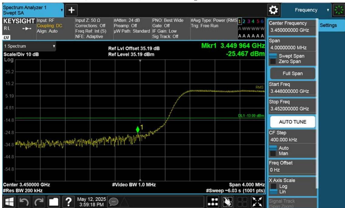
n77(3450~3550 MHz)\_10 M\_Band Edge\_Low\_BPSK\_1RB(1)
