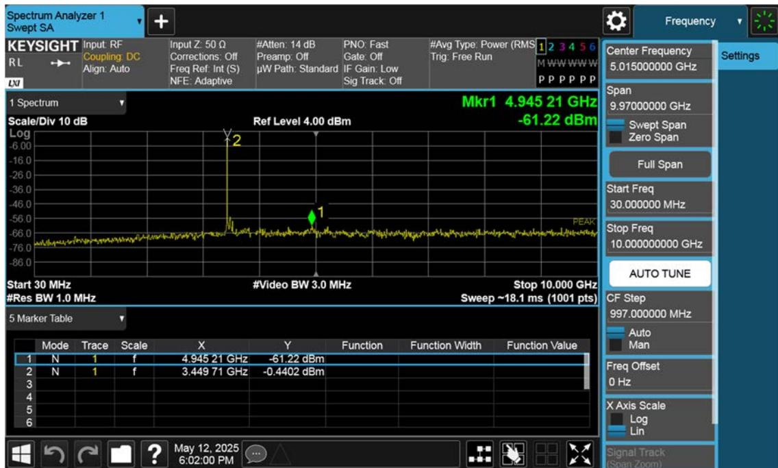
n77(3450~3550 MHz)\_90 M\_Conducted Spurious(30 M-10 G)\_Mid\_BPSK\_1RB
