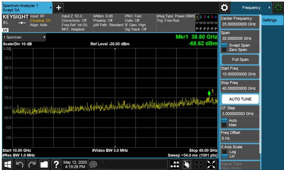
n77(3450~3550 MHz)\_15 M\_Conducted Spurious(Above10 G)\_High\_BPSK\_1RB
