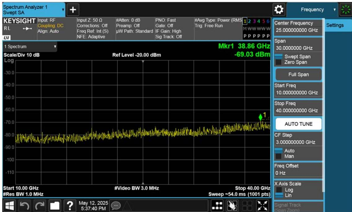
n77(3450~3550 MHz)\_70 M\_Conducted Spurious(Above10 G)\_Mid\_BPSK\_1RB
