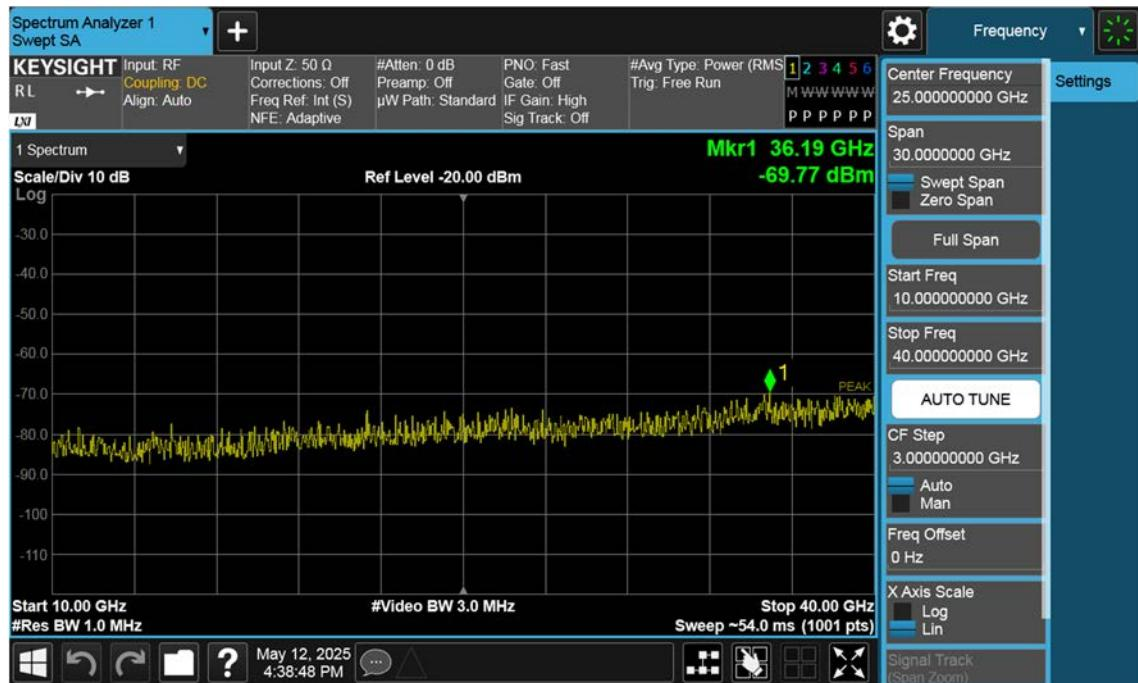
n77(3450~3550 MHz)\_25 M\_Conducted Spurious(Above10 G)\_Mid\_BPSK\_1RB
