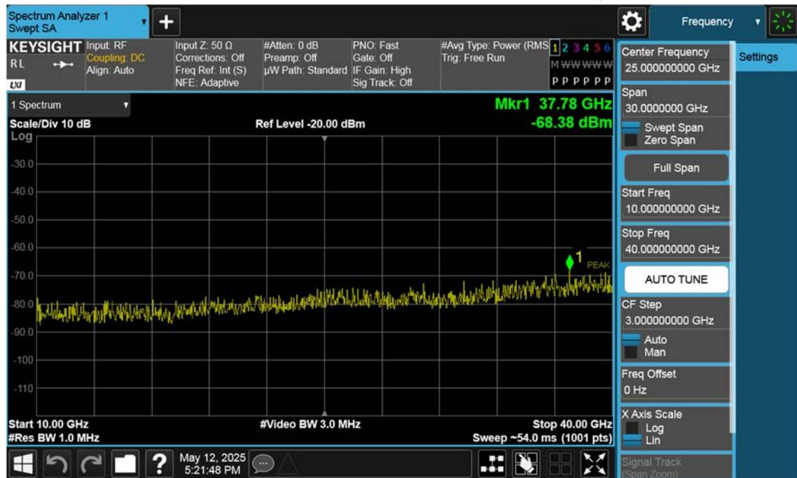
n77(3450~3550 MHz)\_60 M\_Conducted Spurious(Above10 G)\_Low\_BPSK\_1RB
