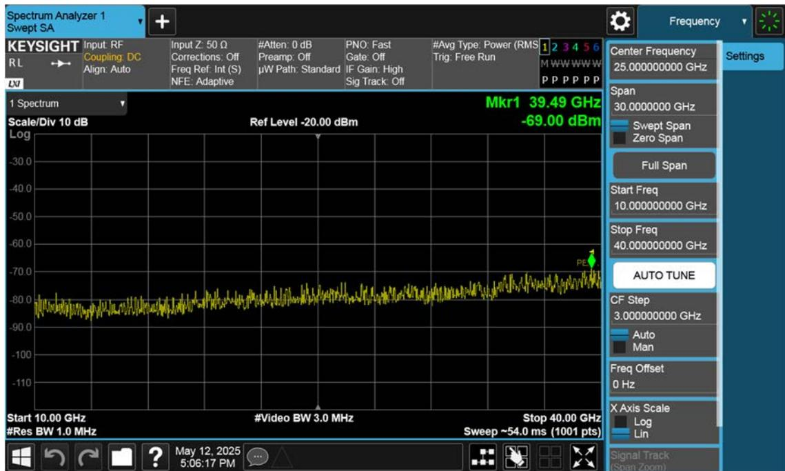
n77(3450~3550 MHz)\_40 M\_Conducted Spurious(Above10 G)\_High\_BPSK\_1RB
