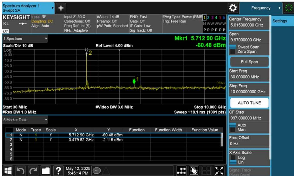
n77(3450~3550 MHz)\_80 M\_Conducted Spurious(30 M-10 G)\_Low\_BPSK\_1RB
