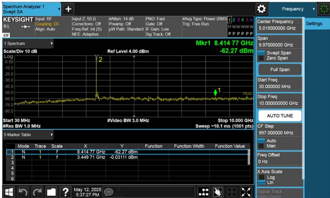
n77(3450~3550 MHz)\_70 M\_Conducted Spurious(30 M-10 G)\_Mid\_BPSK\_1RB
