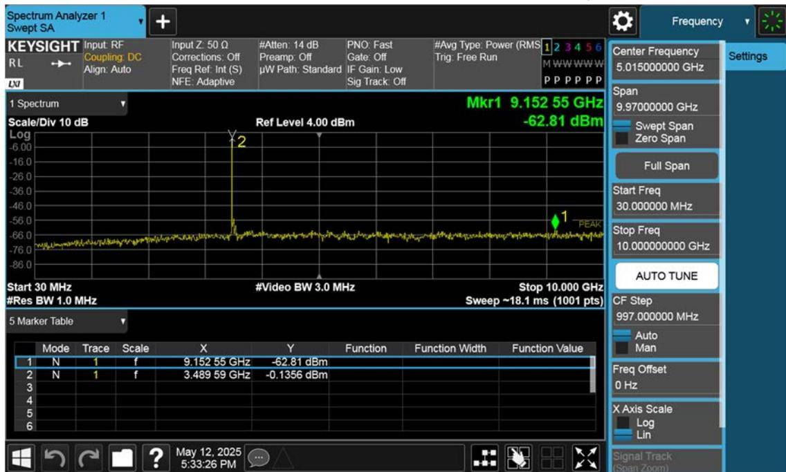
n77(3450~3550 MHz)\_70 M\_Conducted Spurious(30 M-10 G)\_Low\_BPSK\_1RB
