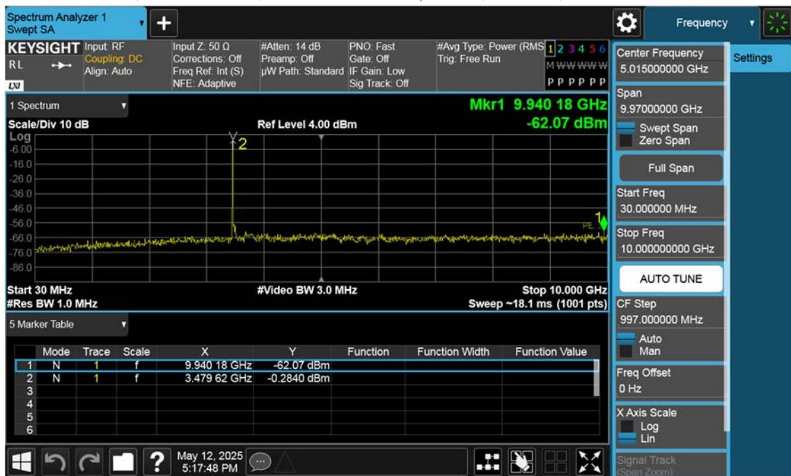
n77(3450~3550 MHz)\_50 M\_Conducted Spurious(30 M-10 G)\_High\_BPSK\_1RB
