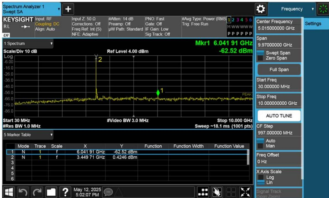
n77(3450~3550 MHz)\_40 M\_Conducted Spurious(30 M-10 G)\_Mid\_BPSK\_1RB
