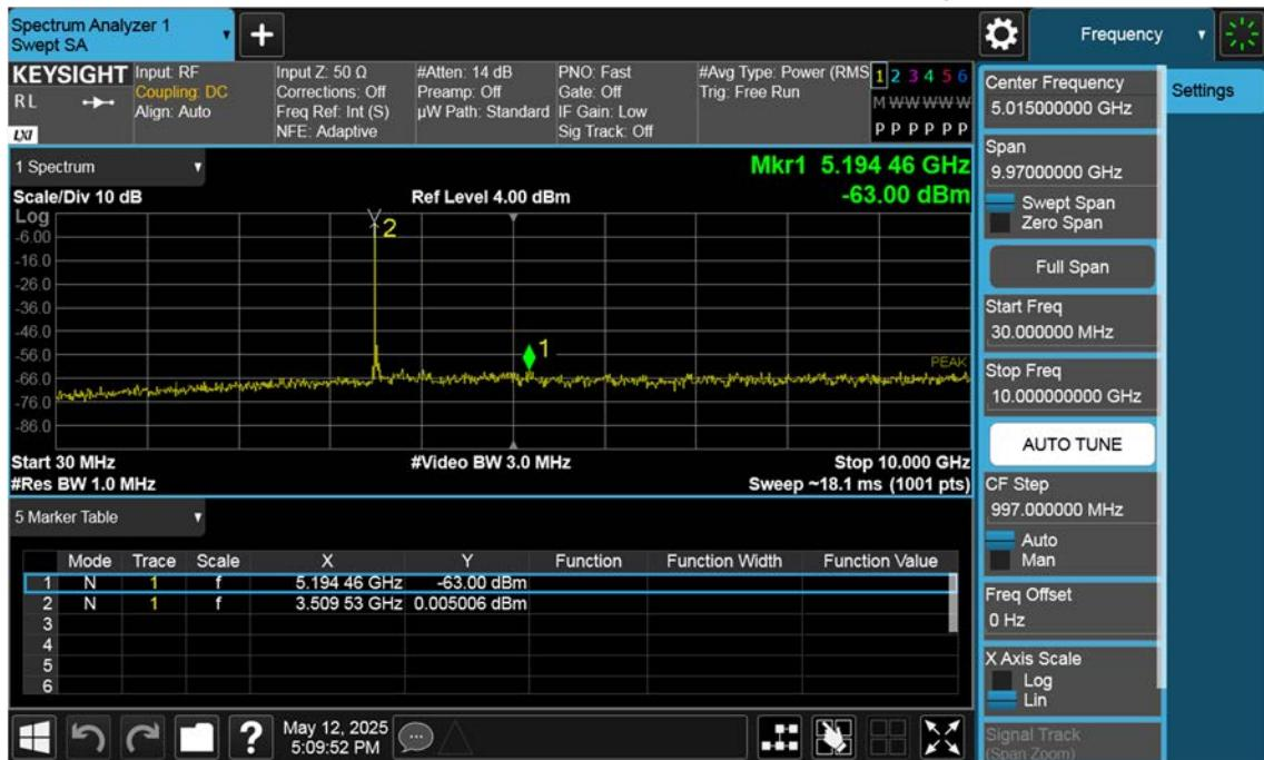
n77(3450~3550 MHz)\_50 M\_Conducted Spurious(30 M-10 G)\_Low\_BPSK\_1RB
