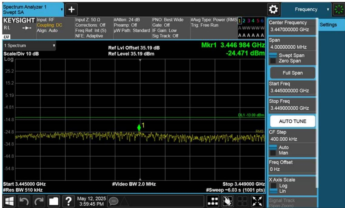
n77(3450~3550 MHz)\_10 M\_Band Edge\_Low\_BPSK\_1RB(2)
