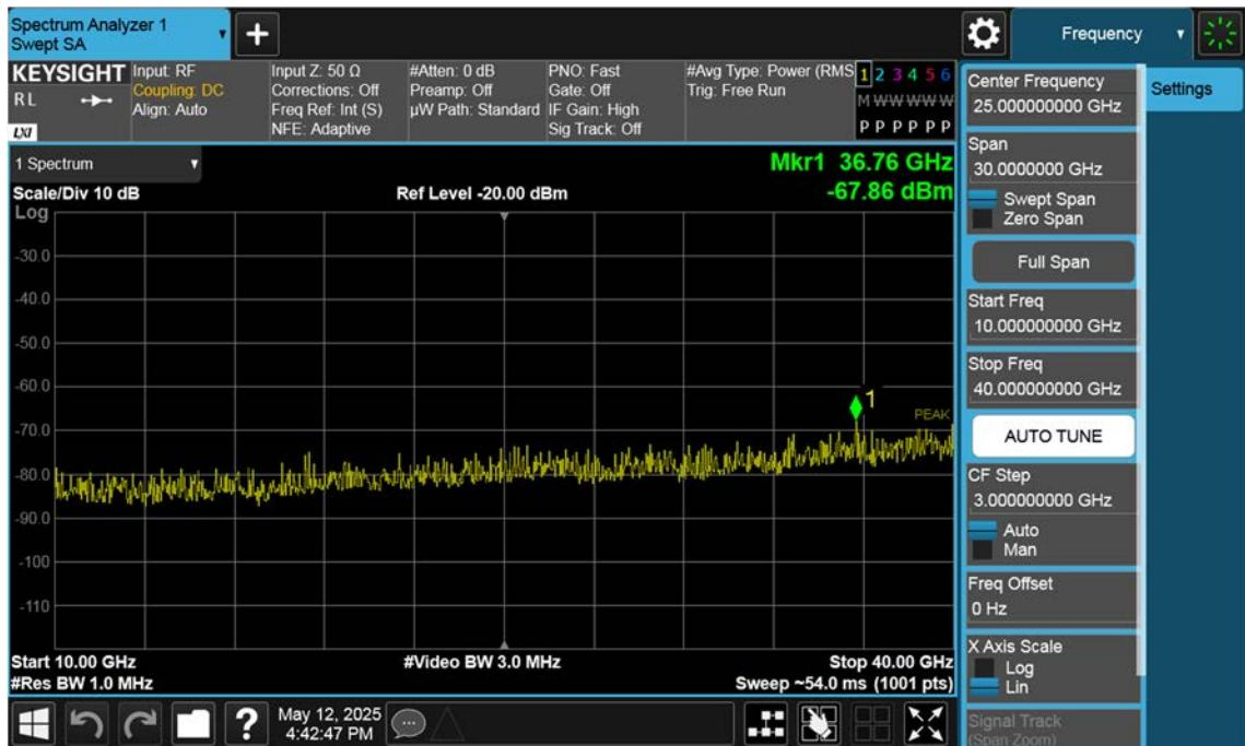
n77(3450~3550 MHz)\_25 M\_Conducted Spurious(Above10 G)\_High\_BPSK\_1RB
