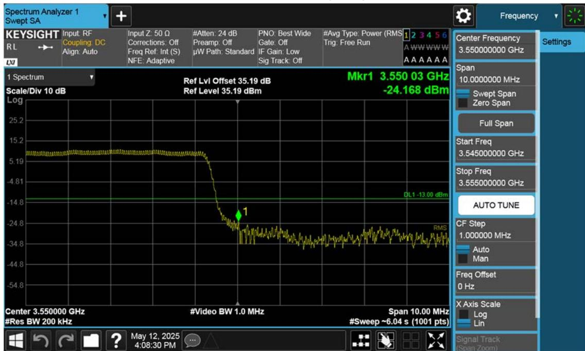
n77(3450~3550 MHz)\_10 M\_Band Edge\_High\_BPSK\_1RB(1)
