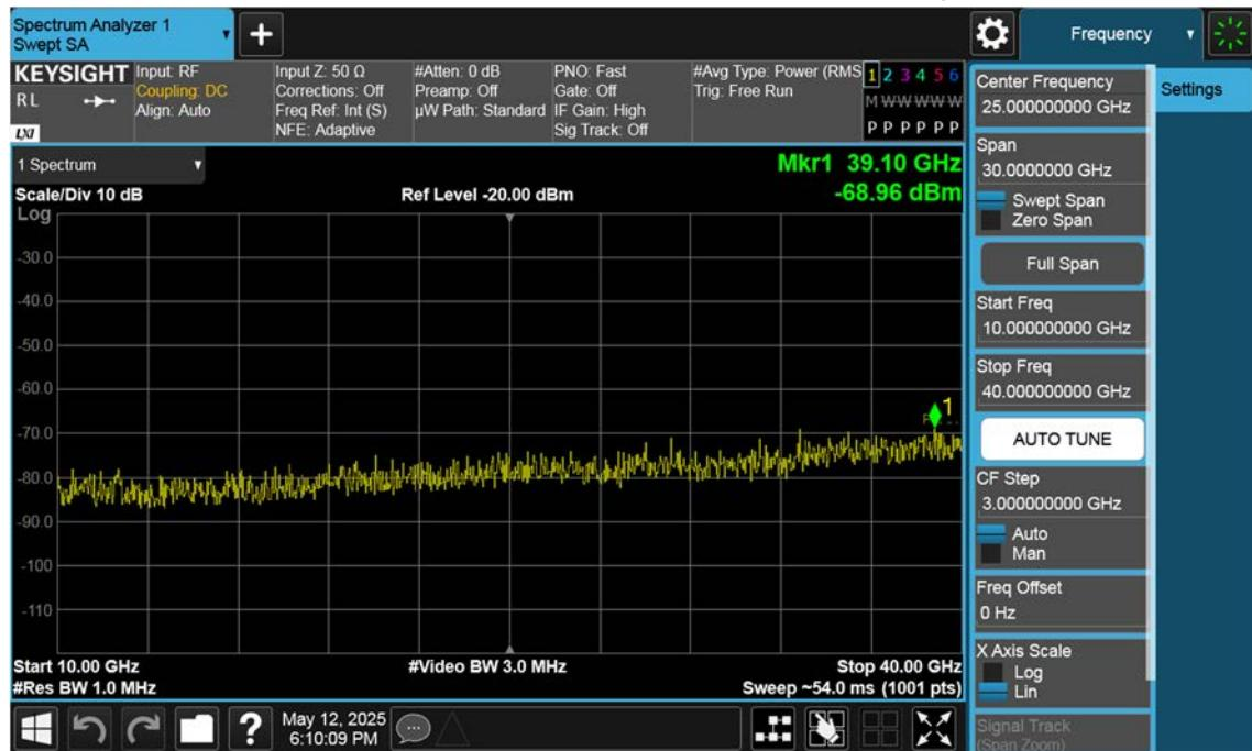
n77(3450~3550 MHz)\_100 M\_Conducted Spurious(Above10 G)\_Low\_BPSK\_1RB
