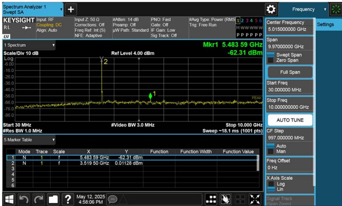
n77(3450~3550 MHz)\_40 M\_Conducted Spurious(30 M-10 G)\_Low\_BPSK\_1RB
