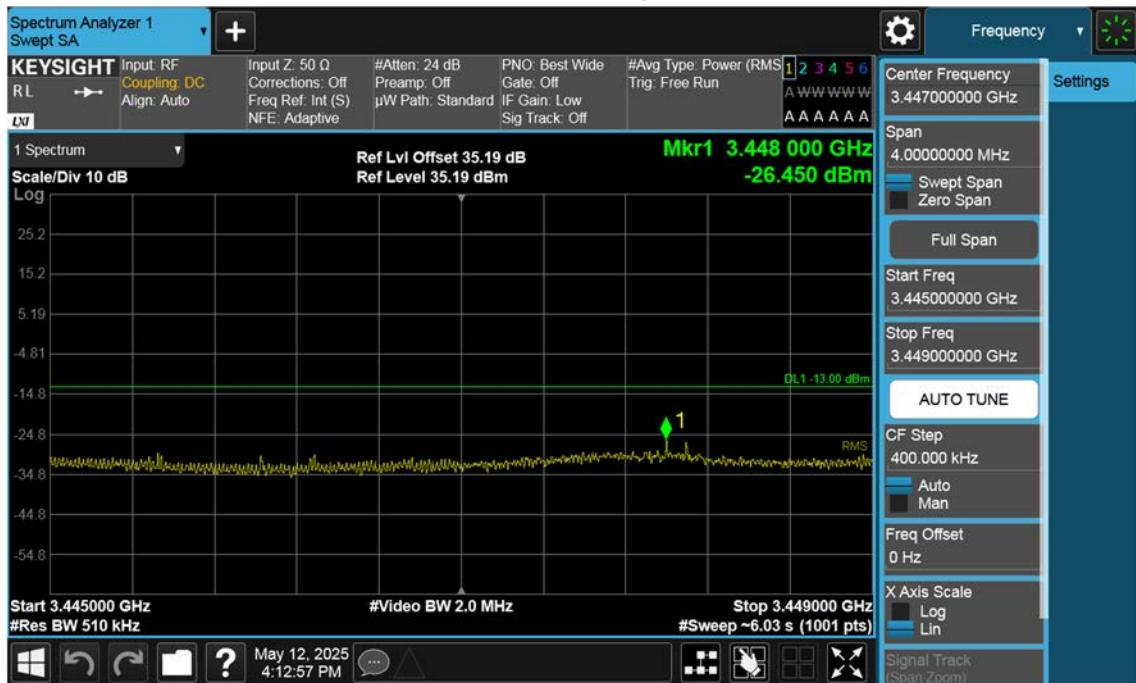
n77(3450~3550 MHz)\_15 M\_Band Edge\_Low\_BPSK\_1RB(2)
