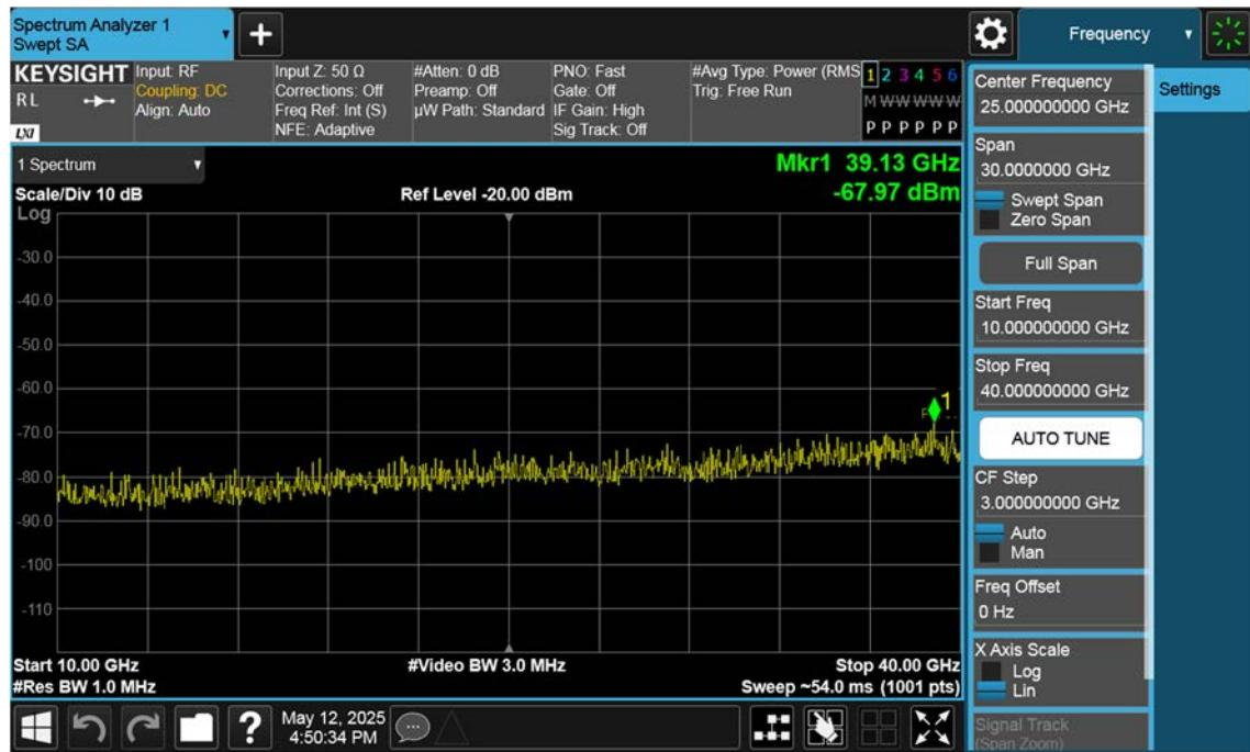
n77(3450~3550 MHz)\_30 M\_Conducted Spurious(Above10 G)\_Mid\_BPSK\_1RB
