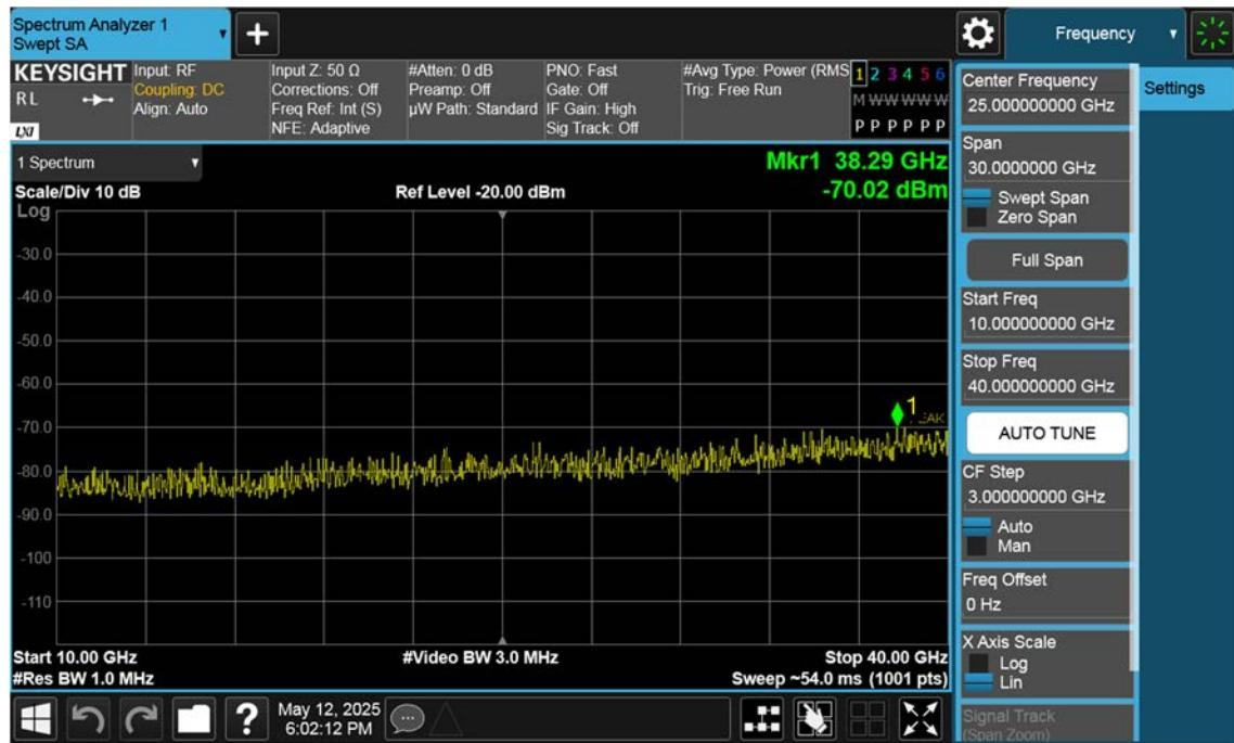
n77(3450~3550 MHz)\_90 M\_Conducted Spurious(Above10 G)\_Mid\_BPSK\_1RB
