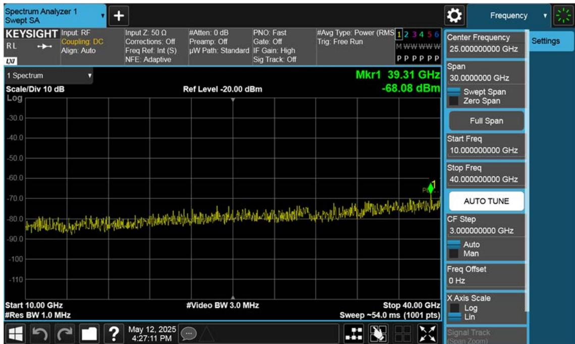
n77(3450~3550 MHz)\_20 M\_Conducted Spurious(Above10 G)\_Mid\_BPSK\_1RB
