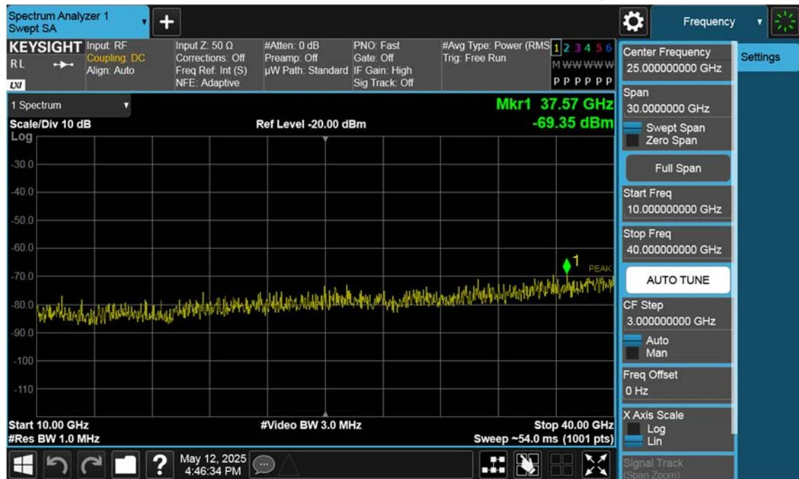
n77(3450~3550 MHz)\_30 M\_Conducted Spurious(Above10 G)\_Low\_BPSK\_1RB
