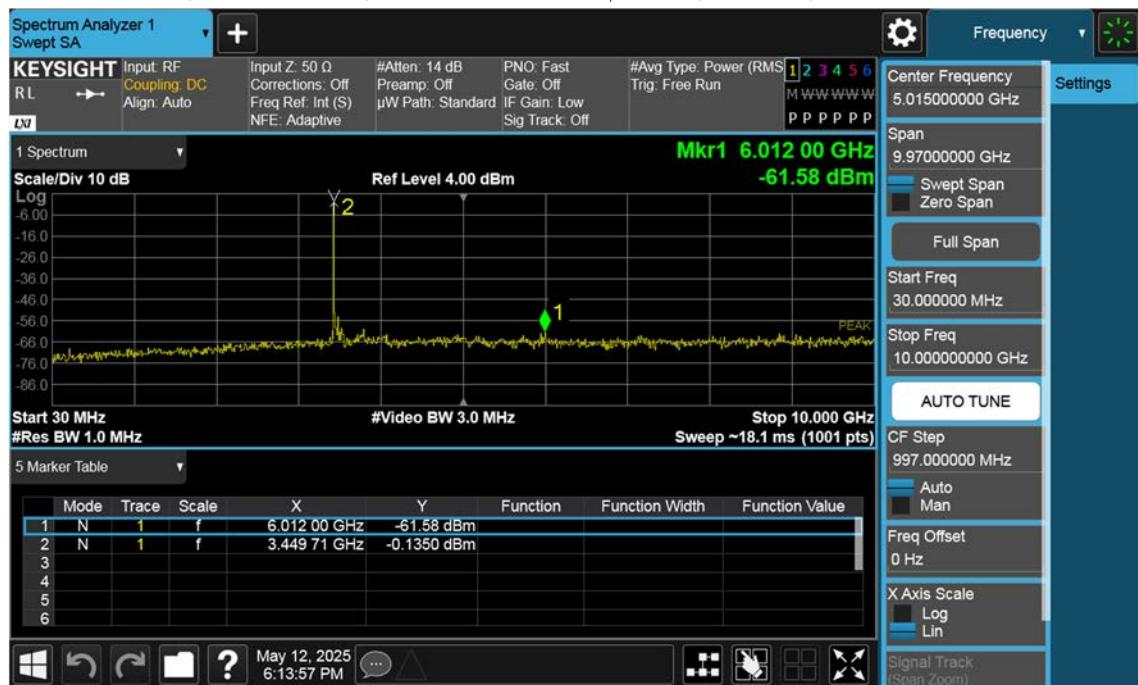
n77(3450~3550 MHz)\_10 M\_Conducted Spurious(Above10 G)\_Low\_BPSK\_1RB
