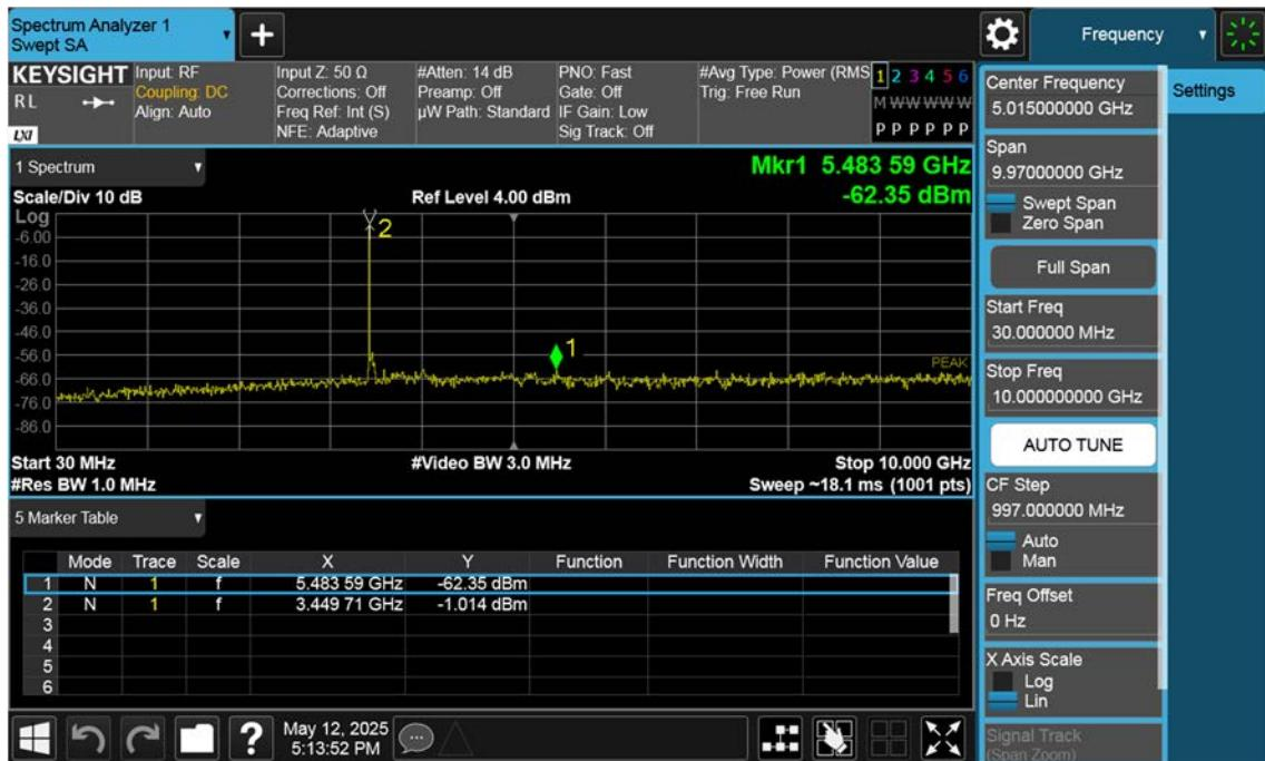
n77(3450~3550 MHz)\_50 M\_Conducted Spurious(30 M-10 G)\_Mid\_BPSK\_1RB
