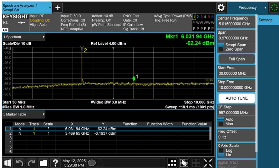
n77(3450~3550 MHz)\_60 M\_Conducted Spurious(30 M-10 G)\_High\_BPSK\_1RB
