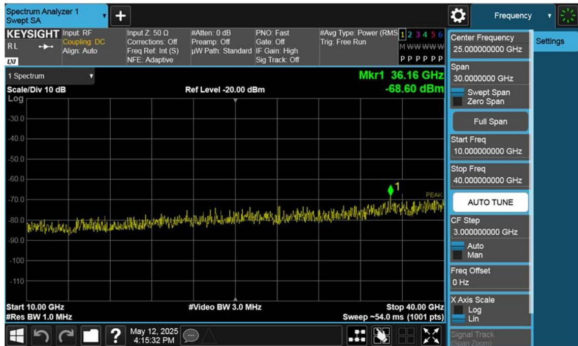
n77(3450~3550 MHz)\_15 M\_Conducted Spurious(Above10 G)\_Mid\_BPSK\_1RB
