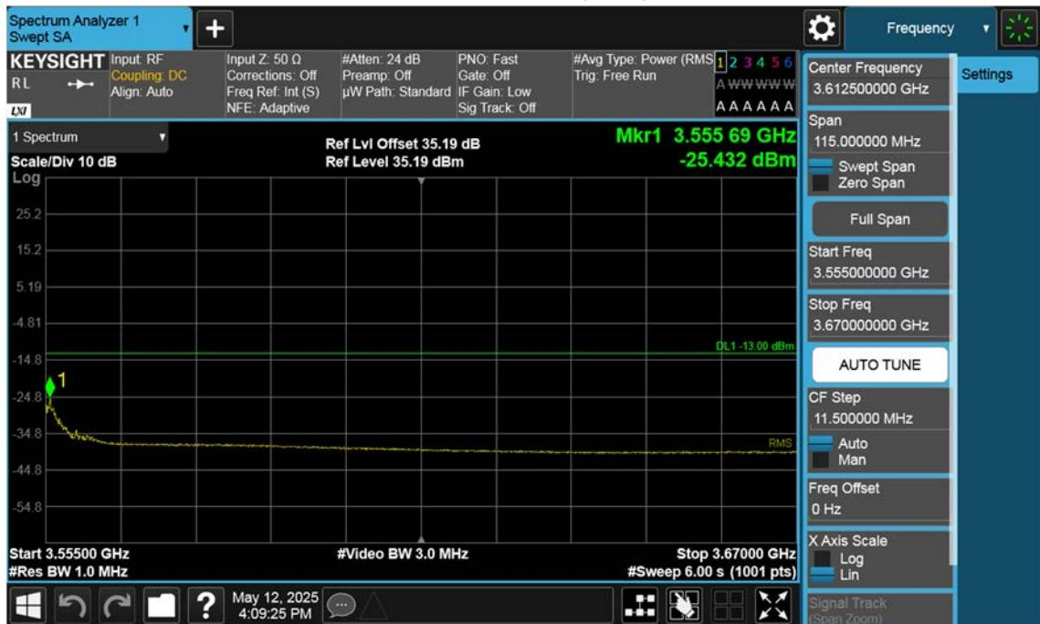
n77(3450~3550 MHz)\_10 M\_Band Edge\_High\_BPSK\_1RB(3)
