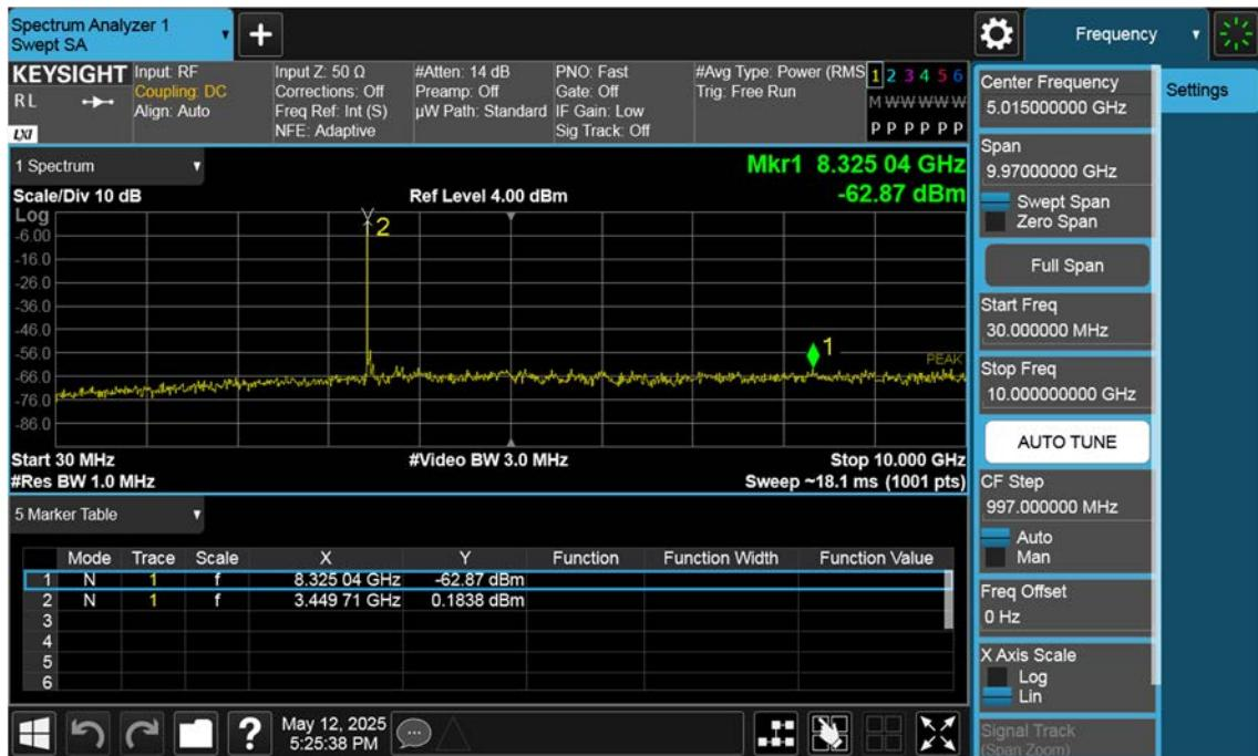
n77(3450~3550 MHz)\_60 M\_Conducted Spurious(30 M-10 G)\_Mid\_BPSK\_1RB
