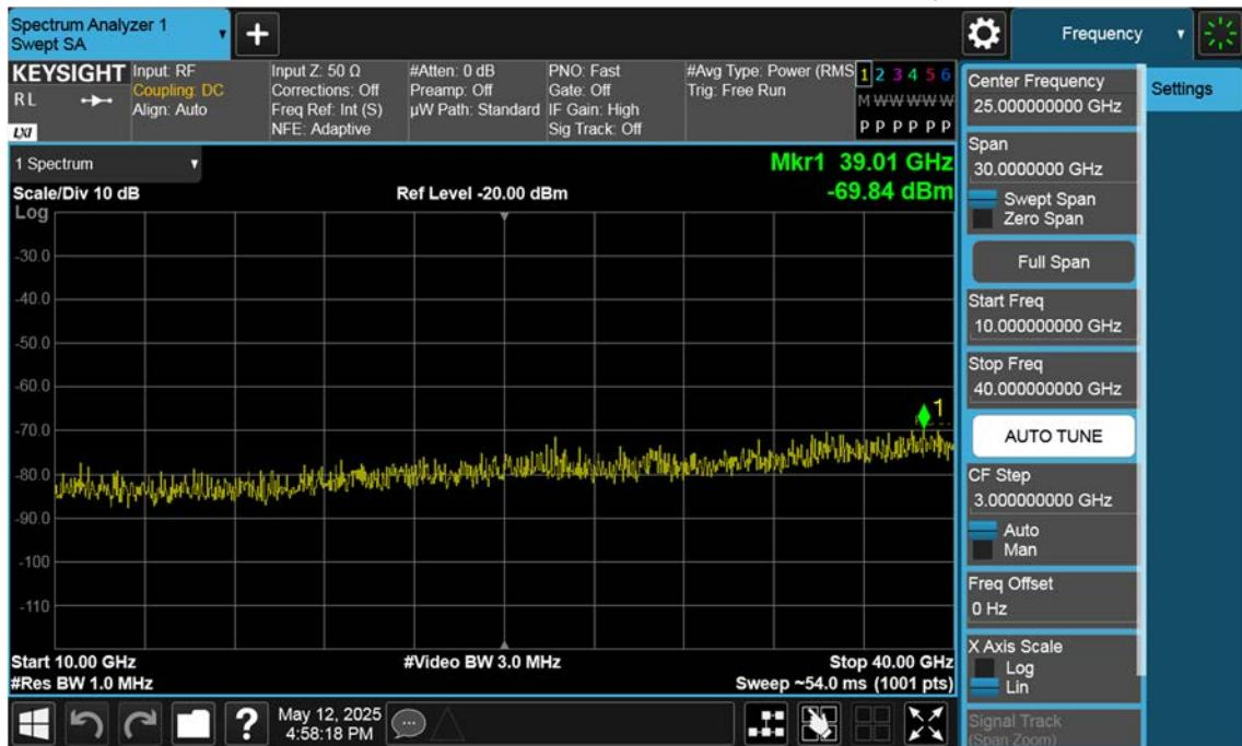
n77(3450~3550 MHz)\_40 M\_Conducted Spurious(Above10 G)\_Low\_BPSK\_1RB
