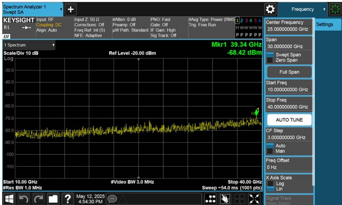
n77(3450~3550 MHz)\_30 M\_Conducted Spurious(Above10 G)\_High\_BPSK\_1RB
