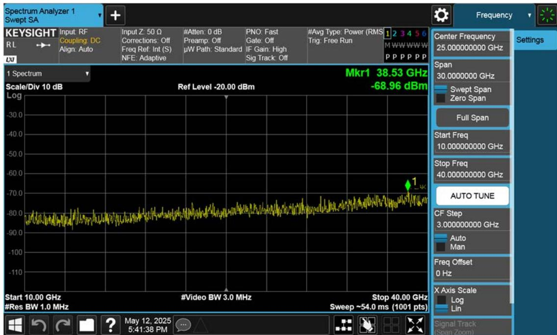
n77(3450~3550 MHz)\_70 M\_Conducted Spurious(Above10 G)\_High\_BPSK\_1RB
