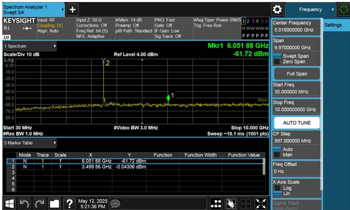
n77(3450~3550 MHz)\_60 M\_Conducted Spurious(30 M-10 G)\_Low\_BPSK\_1RB
