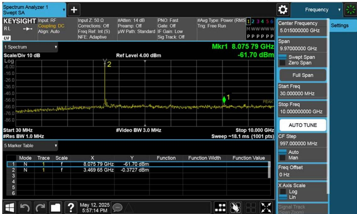
n77(3450~3550 MHz)\_90 M\_Conducted Spurious(30 M-10 G)\_Low\_BPSK\_1RB
