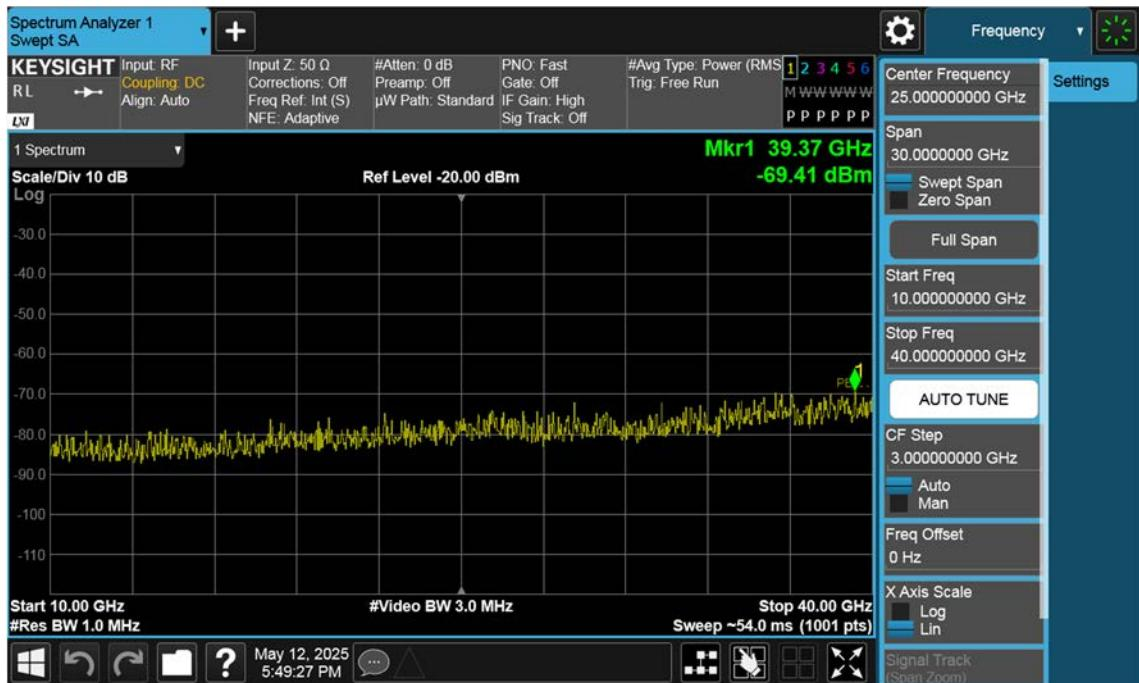
n77(3450~3550 MHz)\_80 M\_Conducted Spurious(Above10 G)\_Mid\_BPSK\_1RB
