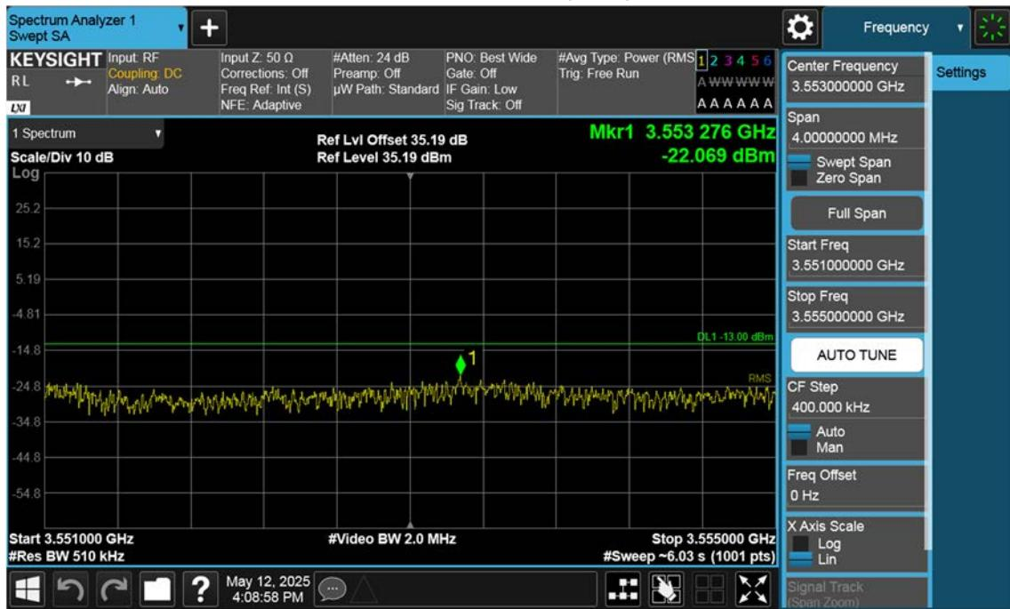
n77(3450~3550 MHz)\_10 M\_Band Edge\_High\_BPSK\_1RB(2)
