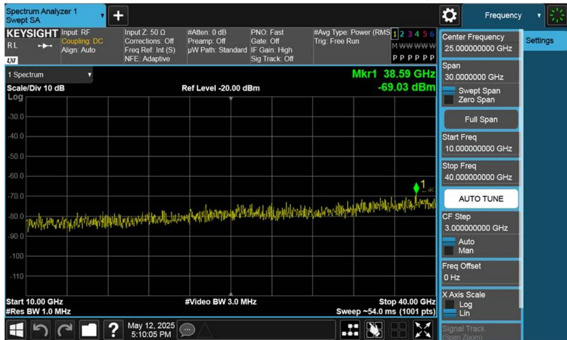
n77(3450~3550 MHz)\_50 M\_Conducted Spurious(Above10 G)\_Low\_BPSK\_1RB
