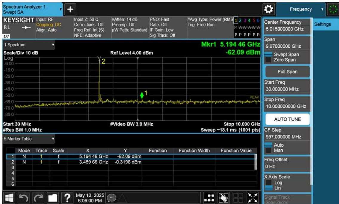
n77(3450~3550 MHz)\_90 M\_Conducted Spurious(30 M-10 G)\_High\_BPSK\_1RB
