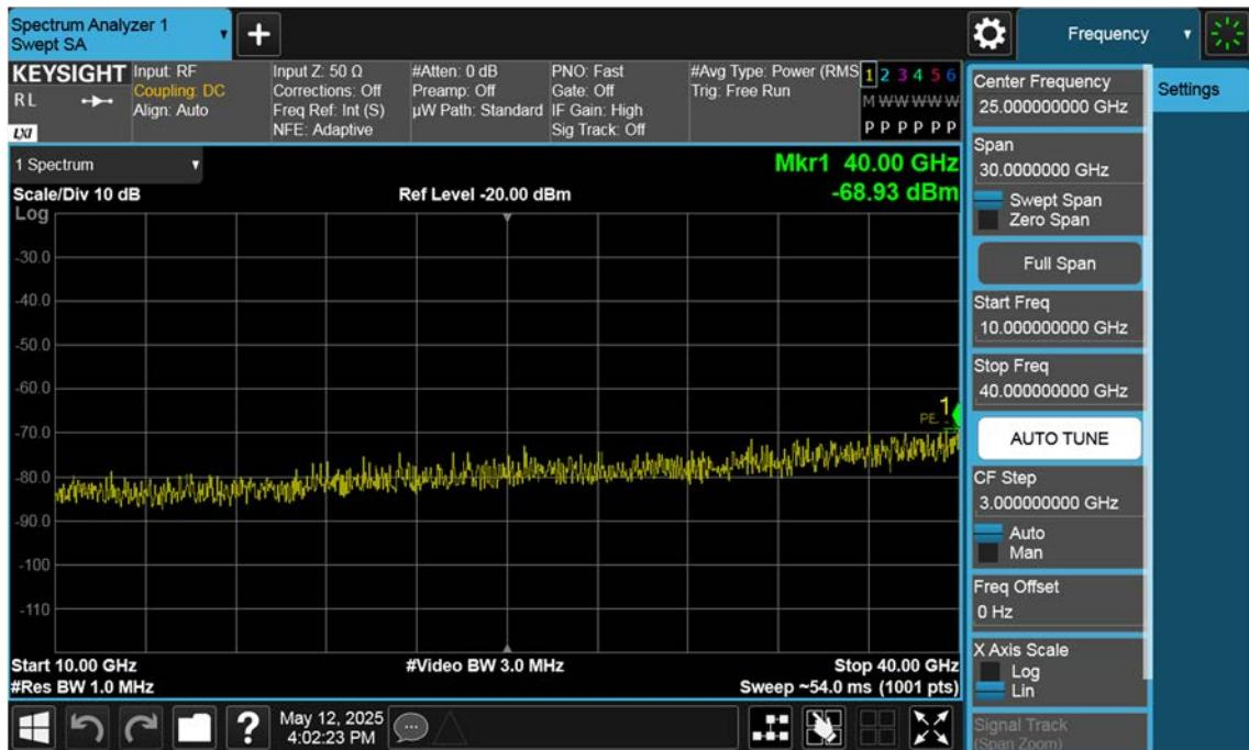
n77(3450~3550 MHz)\_10 M\_Conducted Spurious(Above10 G)\_Mid\_BPSK\_1RB
