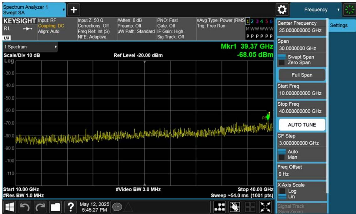
n77(3450~3550 MHz)\_80 M\_Conducted Spurious(Above10 G)\_Low\_BPSK\_1RB
