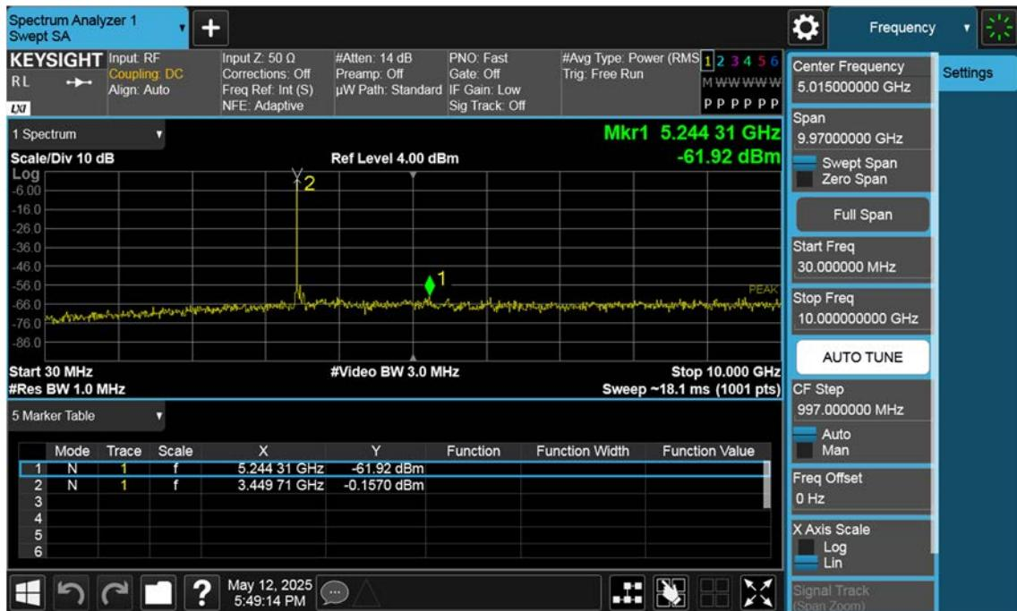
n77(3450~3550 MHz)\_80 M\_Conducted Spurious(30 M-10 G)\_Mid\_BPSK\_1RB
