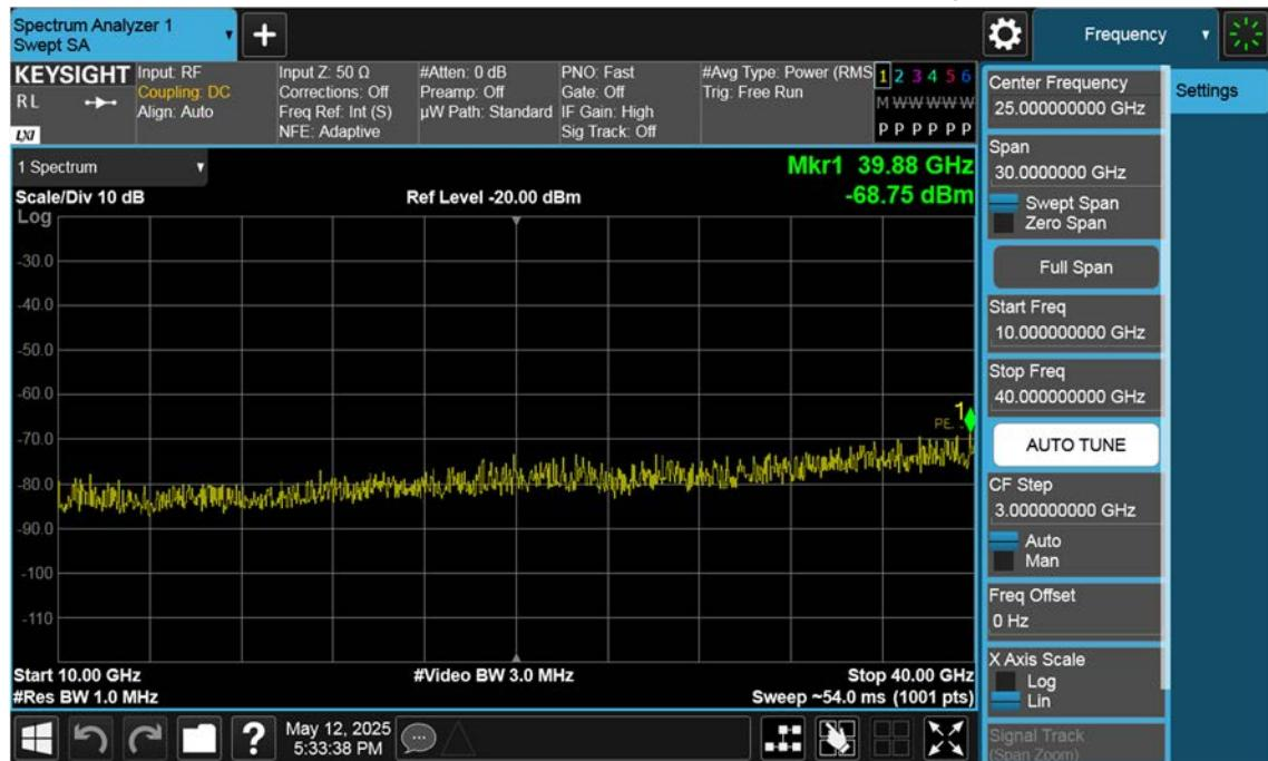
n77(3450~3550 MHz)\_70 M\_Conducted Spurious(Above10 G)\_Low\_BPSK\_1RB
