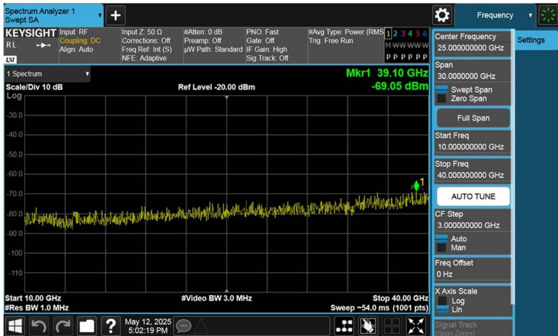
n77(3450~3550 MHz)\_40 M\_Conducted Spurious(Above10 G)\_Mid\_BPSK\_1RB
