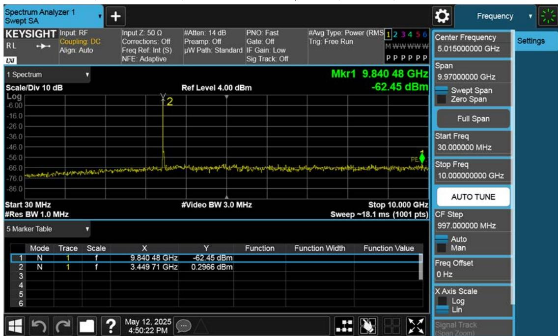
n77(3450~3550 MHz)\_30 M\_Conducted Spurious(30 M-10 G)\_Mid\_BPSK\_1RB
