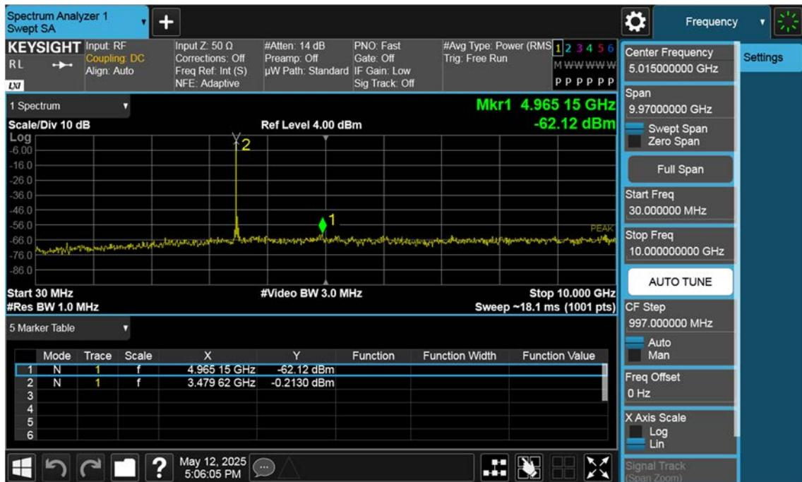
n77(3450~3550 MHz)\_40 M\_Conducted Spurious(30 M-10 G)\_High\_BPSK\_1RB
