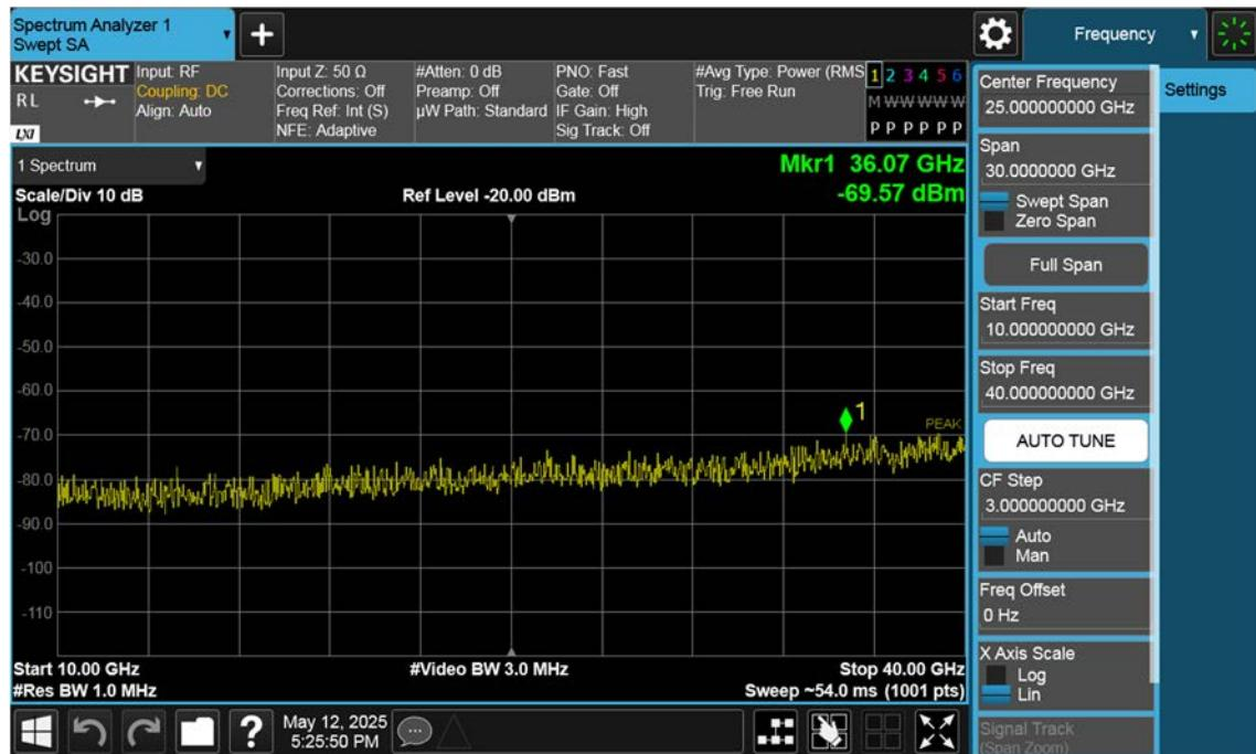
n77(3450~3550 MHz)\_60 M\_Conducted Spurious(Above10 G)\_Mid\_BPSK\_1RB
