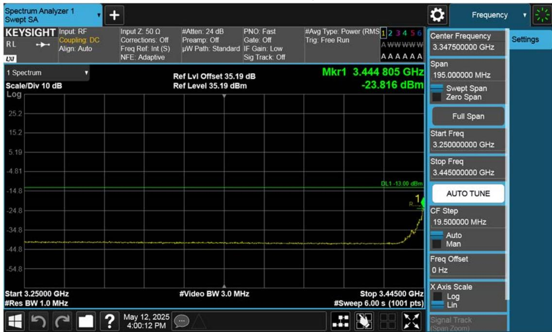
n77(3450~3550 MHz)\_10 M\_Band Edge\_Low\_BPSK\_1RB(3)
