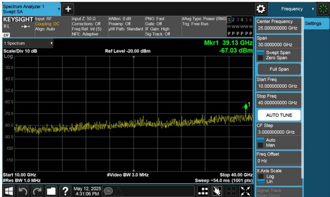
n77(3450~3550 MHz)\_20 M\_Conducted Spurious(Above10 G)\_High\_BPSK\_1RB
