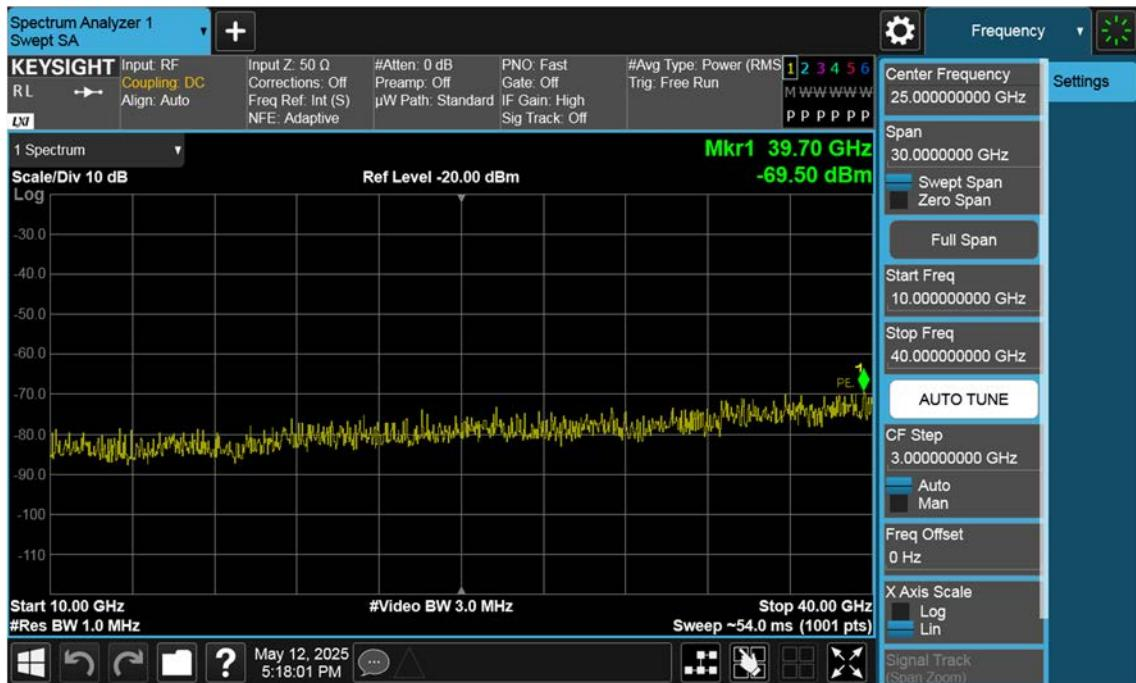
n77(3450~3550 MHz)\_50 M\_Conducted Spurious(Above10 G)\_High\_BPSK\_1RB
