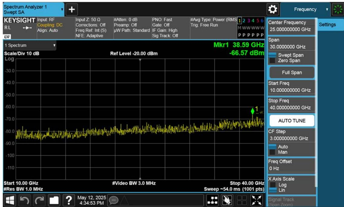
n77(3450~3550 MHz)\_25 M\_Conducted Spurious(Above10 G)\_Low\_BPSK\_1RB
