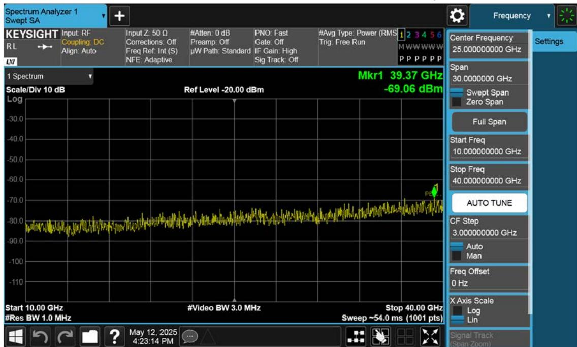
n77(3450~3550 MHz)\_20 M\_Conducted Spurious(Above10 G)\_Low\_BPSK\_1RB
