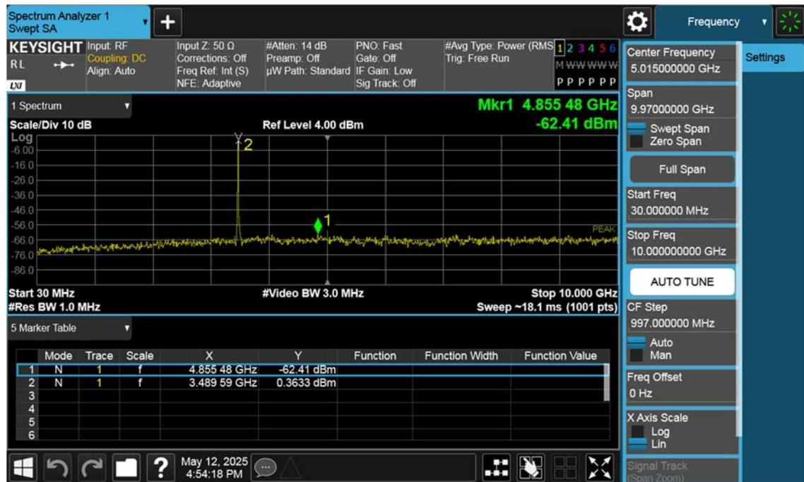
n77(3450~3550 MHz)\_30 M\_Conducted Spurious(30 M-10 G)\_High\_BPSK\_1RB
