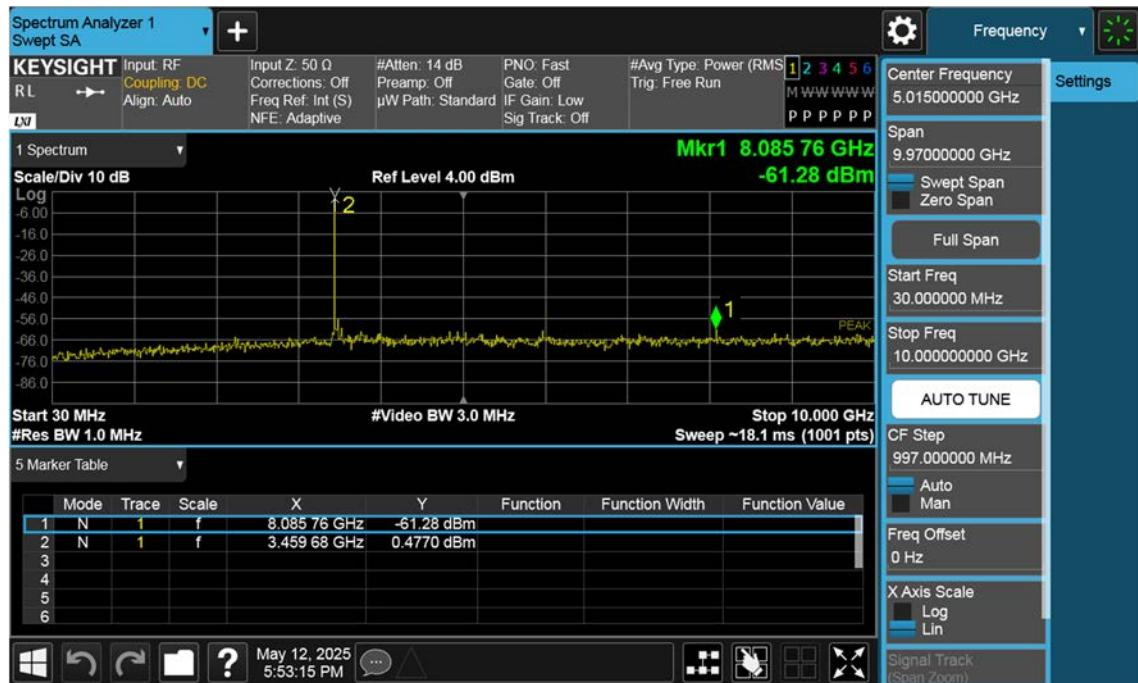
n77(3450~3550 MHz)\_80 M\_Conducted Spurious(30 M-10 G)\_High\_BPSK\_1RB
