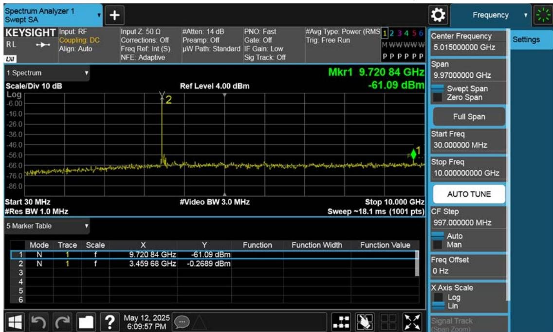
n77(3450~3550 MHz)\_100 M\_Conducted Spurious(30 M-10 G)\_Low\_BPSK\_1RB
