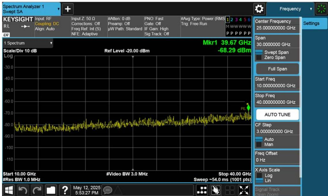
n77(3450~3550 MHz)\_80 M\_Conducted Spurious(Above10 G)\_High\_BPSK\_1RB
