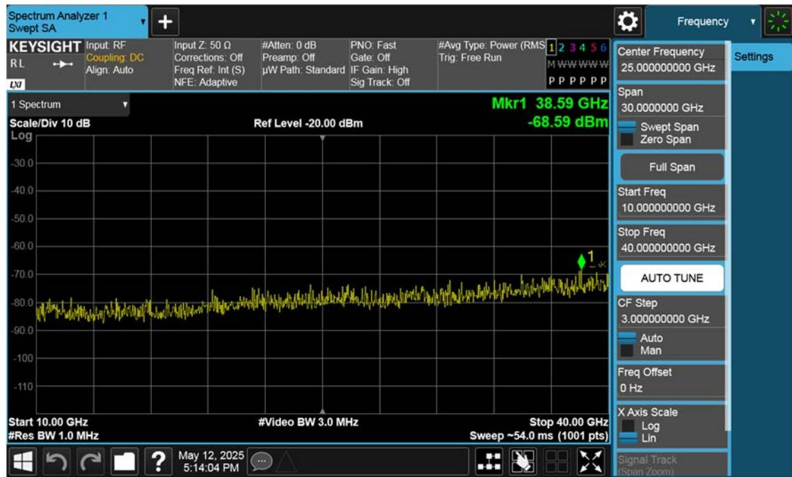
n77(3450~3550 MHz)\_50 M\_Conducted Spurious(Above10 G)\_Mid\_BPSK\_1RB
