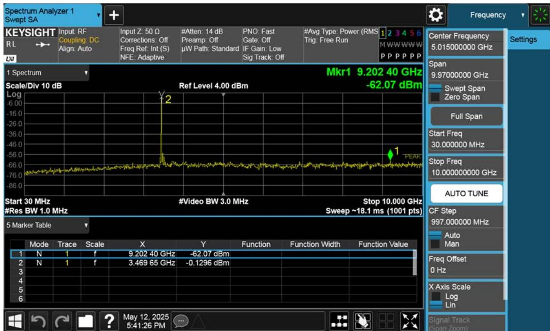
n77(3450~3550 MHz)\_70 M\_Conducted Spurious(30 M-10 G)\_High\_BPSK\_1RB
