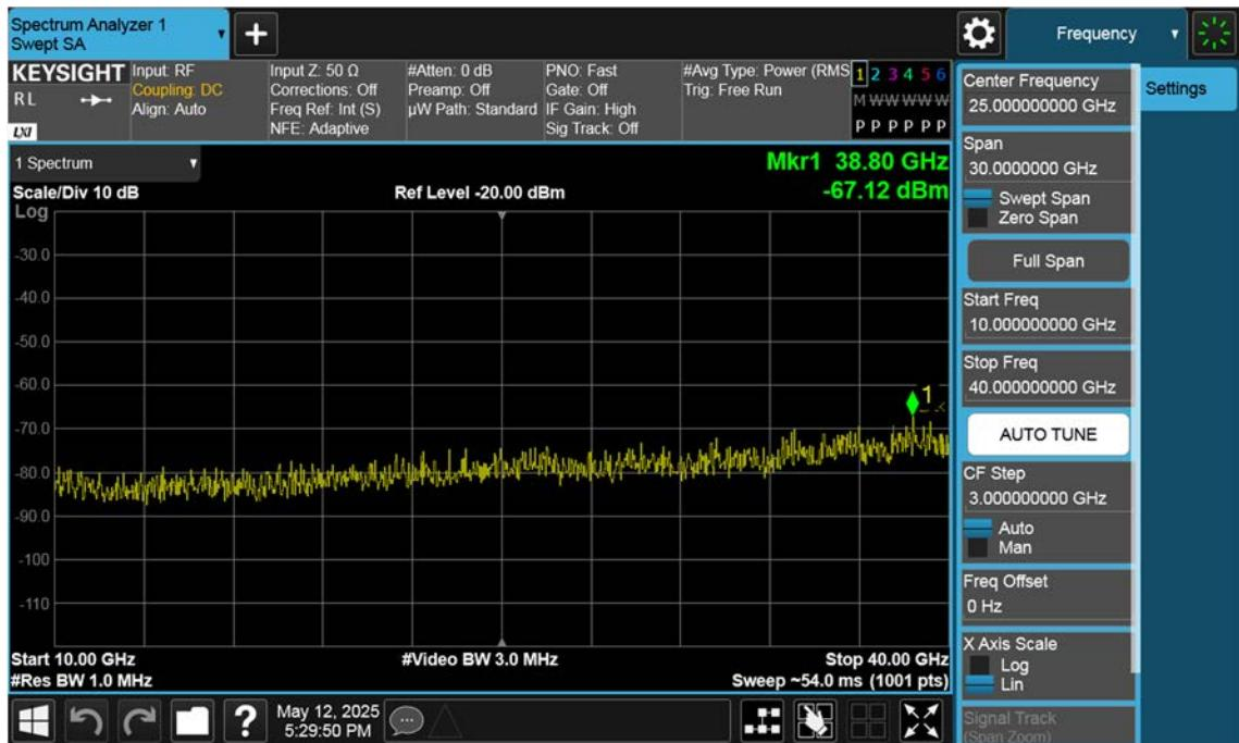
n77(3450~3550 MHz)\_60 M\_Conducted Spurious(Above10 G)\_High\_BPSK\_1RB
