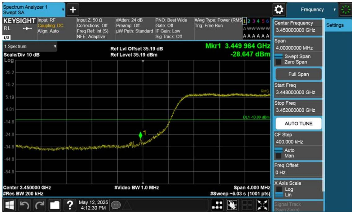
n77(3450~3550 MHz)\_15 M\_Band Edge\_Low\_BPSK\_1RB(1)
