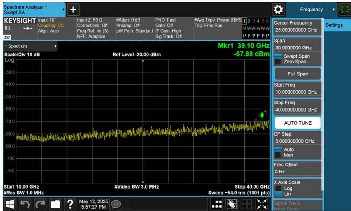
n77(3450~3550 MHz)\_90 M\_Conducted Spurious(Above10 G)\_Low\_BPSK\_1RB
