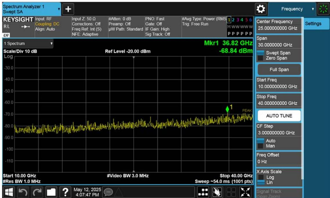
n77(3450~3550 MHz)\_10 M\_Conducted Spurious(Above10 G)\_High\_BPSK\_1RB
