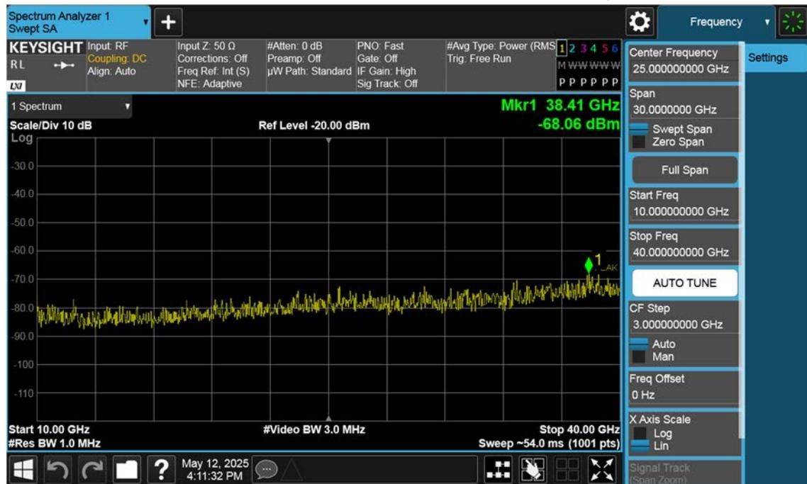
n77(3450~3550 MHz)\_15 M\_Conducted Spurious(Above10 G)\_Low\_BPSK\_1RB
