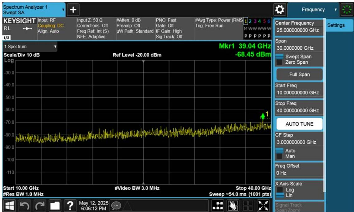
n77(3450~3550 MHz)\_90 M\_Conducted Spurious(Above10 G)\_High\_BPSK\_1RB
