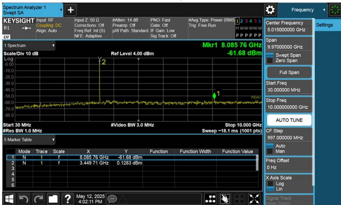
n77(3450~3550 MHz)\_10 M\_Conducted Spurious(30 M-10 G)\_Mid\_BPSK\_1RB
