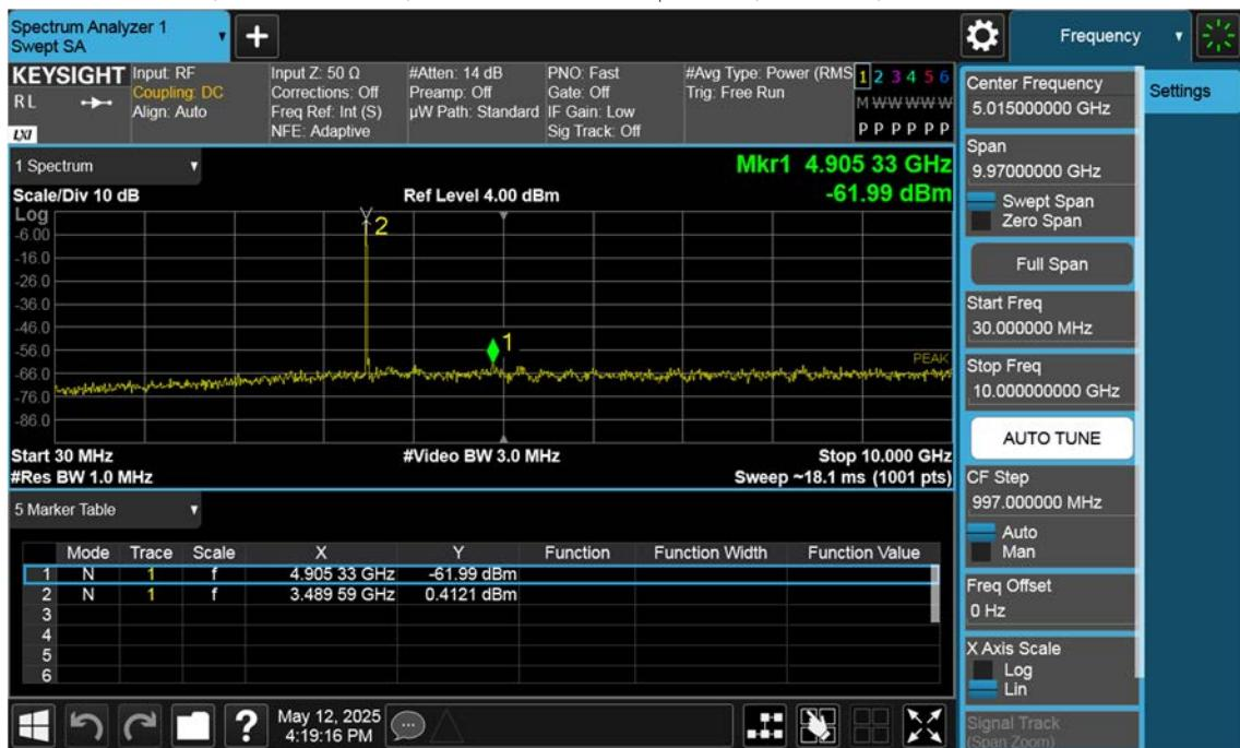
n77(3450~3550 MHz)\_15 M\_Conducted Spurious(30 M-10 G)\_High\_BPSK\_1RB
