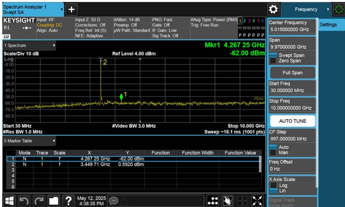
n77(3450~3550 MHz)\_25 M\_Conducted Spurious(30 M-10 G)\_Mid\_BPSK\_1RB
