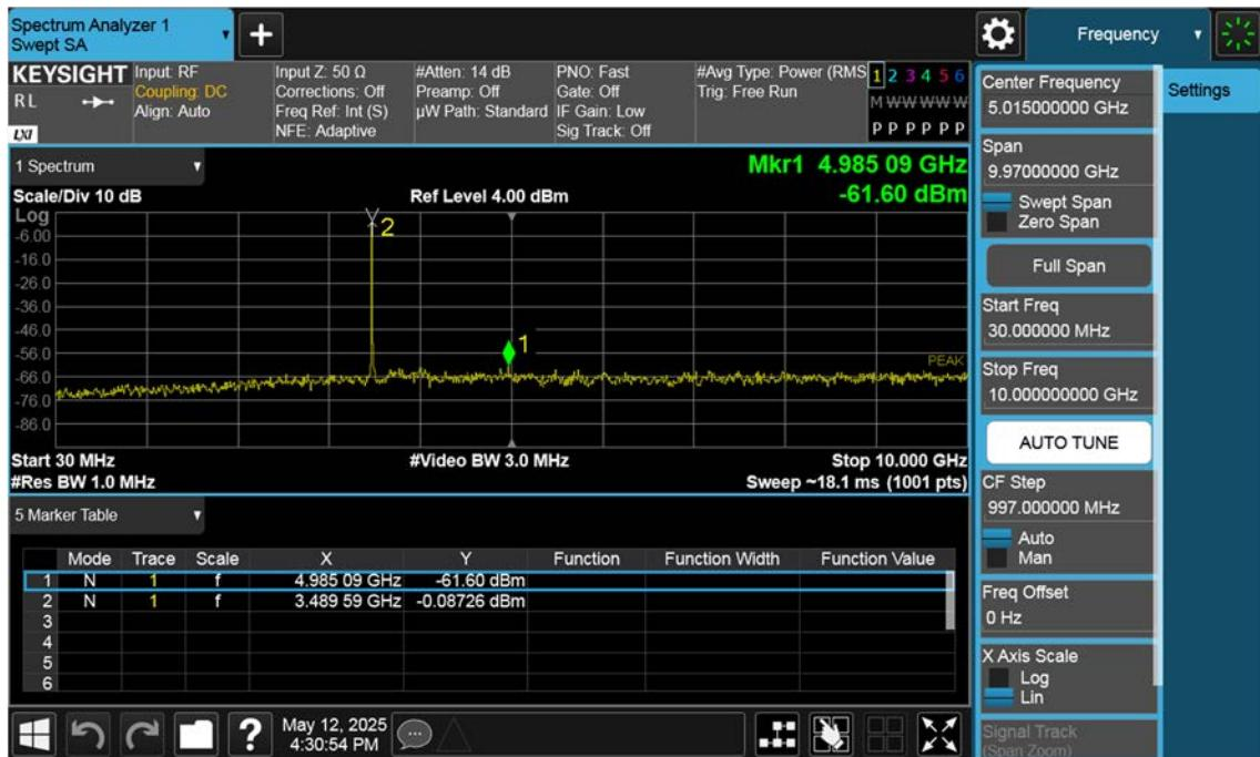
n77(3450~3550 MHz)\_20 M\_Conducted Spurious(30 M-10 G)\_High\_BPSK\_1RB
