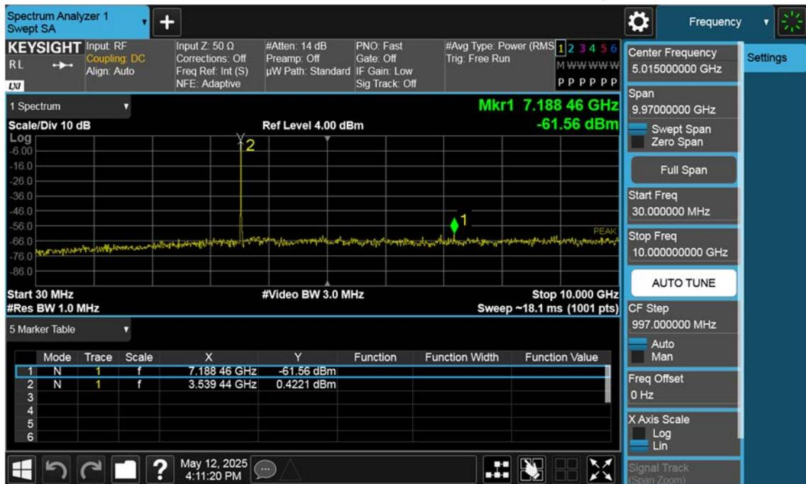
n77(3450~3550 MHz)\_15 M\_Conducted Spurious(30 M-10 G)\_Low\_BPSK\_1RB
