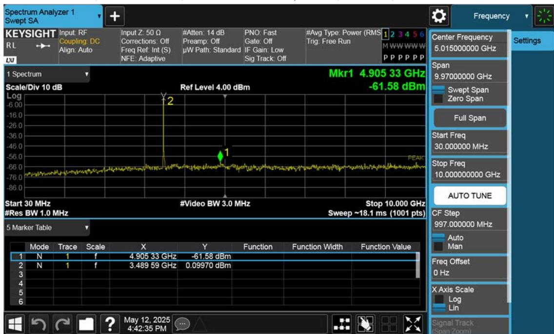
n77(3450~3550 MHz)\_25 M\_Conducted Spurious(30 M-10 G)\_High\_BPSK\_1RB
