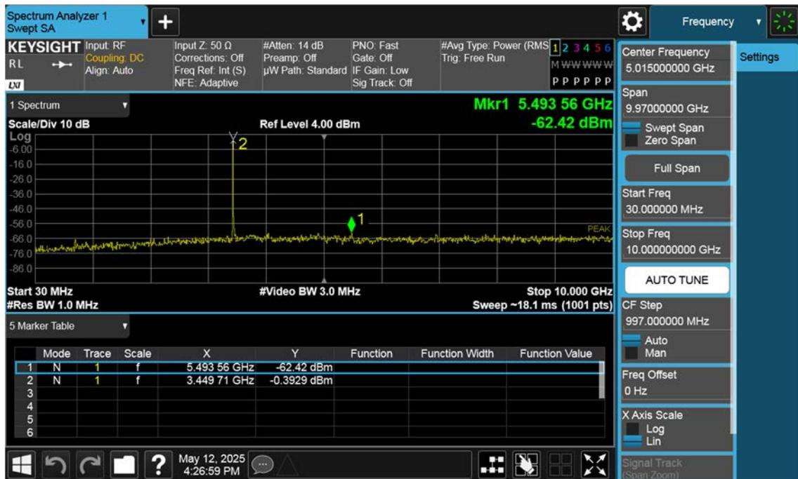
n77(3450~3550 MHz)\_20 M\_Conducted Spurious(30 M-10 G)\_Mid\_BPSK\_1RB
