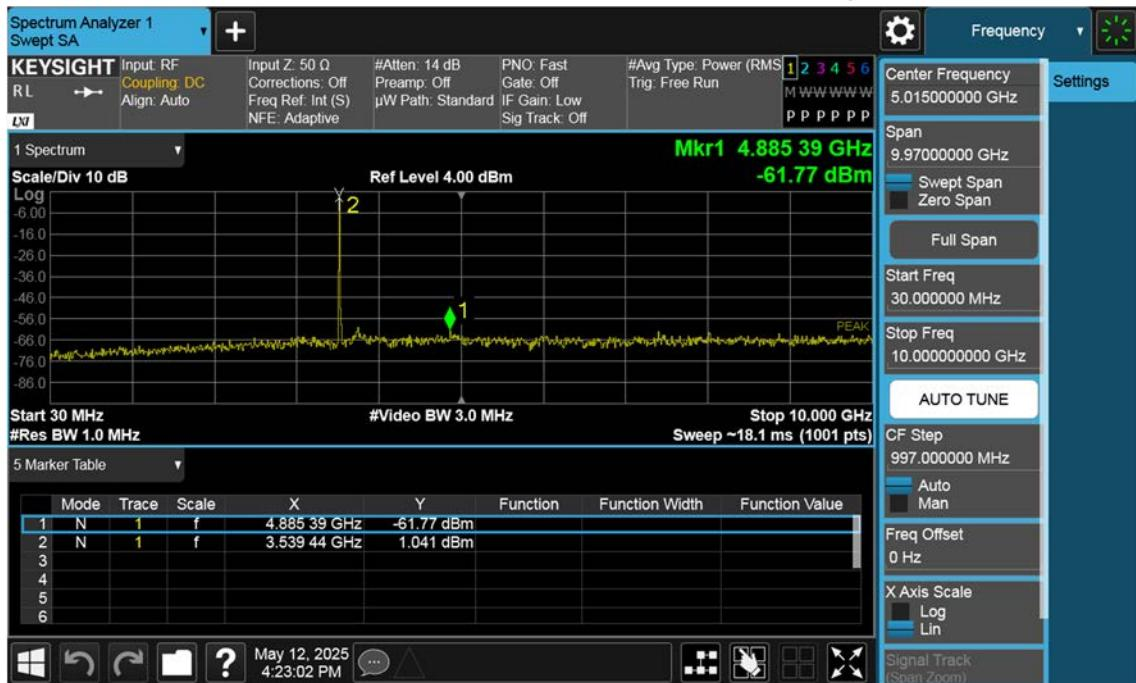
n77(3450~3550 MHz)\_20 M\_Conducted Spurious(30 M-10 G)\_Low\_BPSK\_1RB
