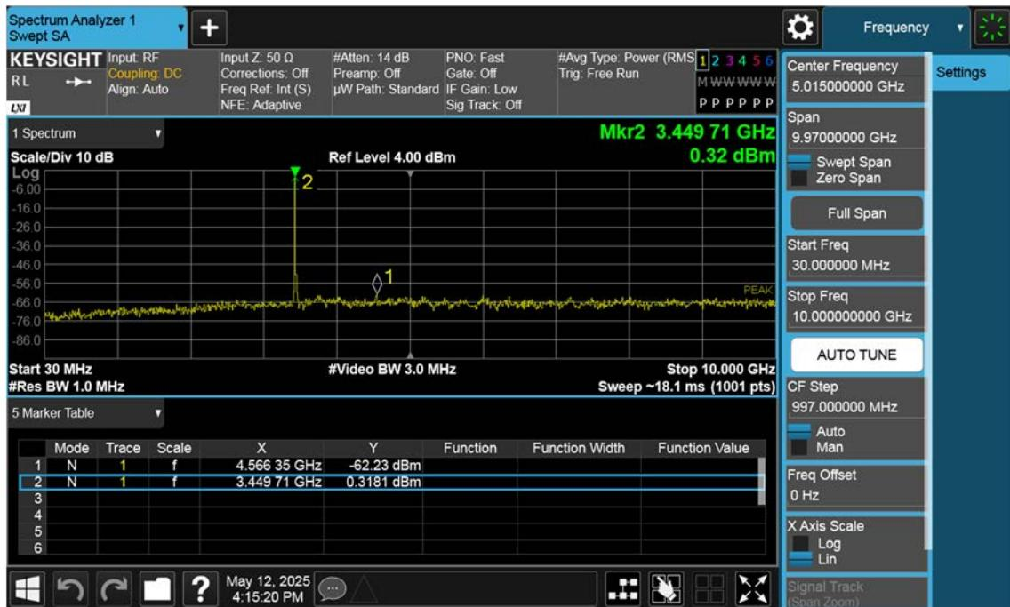
n77(3450~3550 MHz)\_15 M\_Conducted Spurious(30 M-10 G)\_Mid\_BPSK\_1RB
