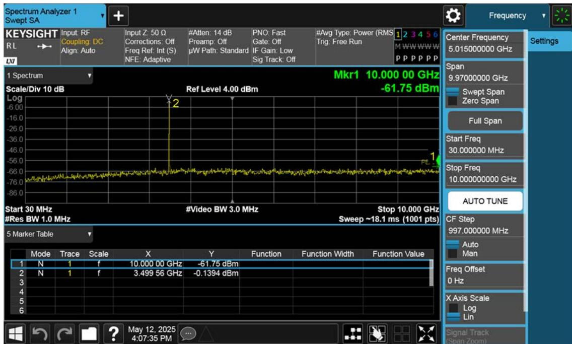
n77(3450~3550 MHz)\_10 M\_Conducted Spurious(30 M-10 G)\_High\_BPSK\_1RB
