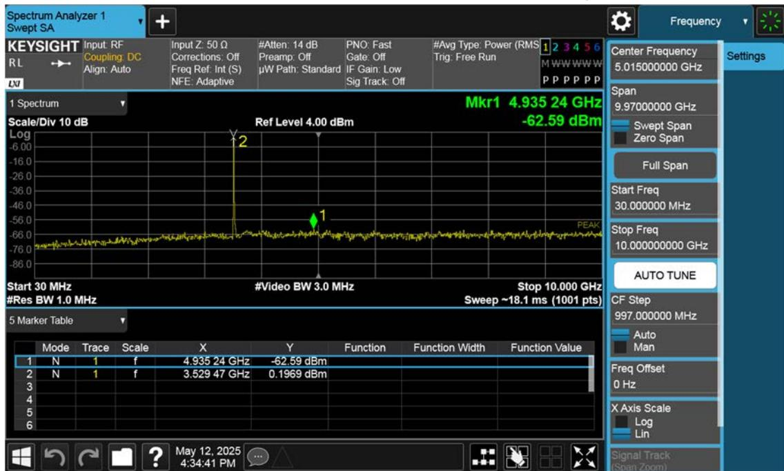
n77(3450~3550 MHz)\_25 M\_Conducted Spurious(30 M-10 G)\_Low\_BPSK\_1RB
