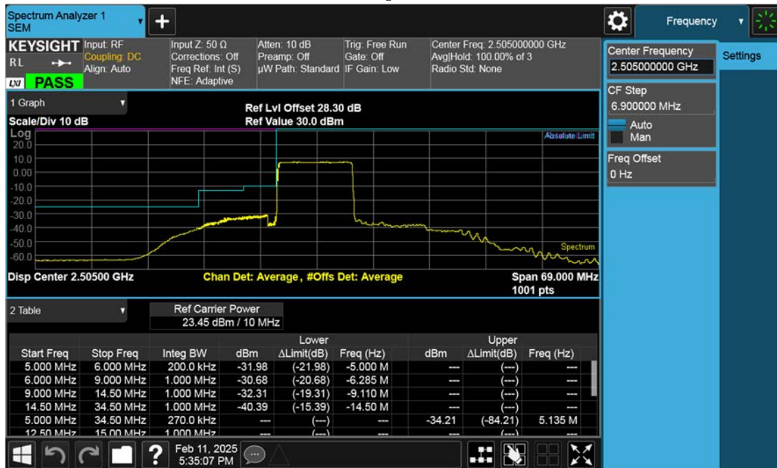
NR7_Low Channel Edge Plot (10 MHz BPSK)-1
