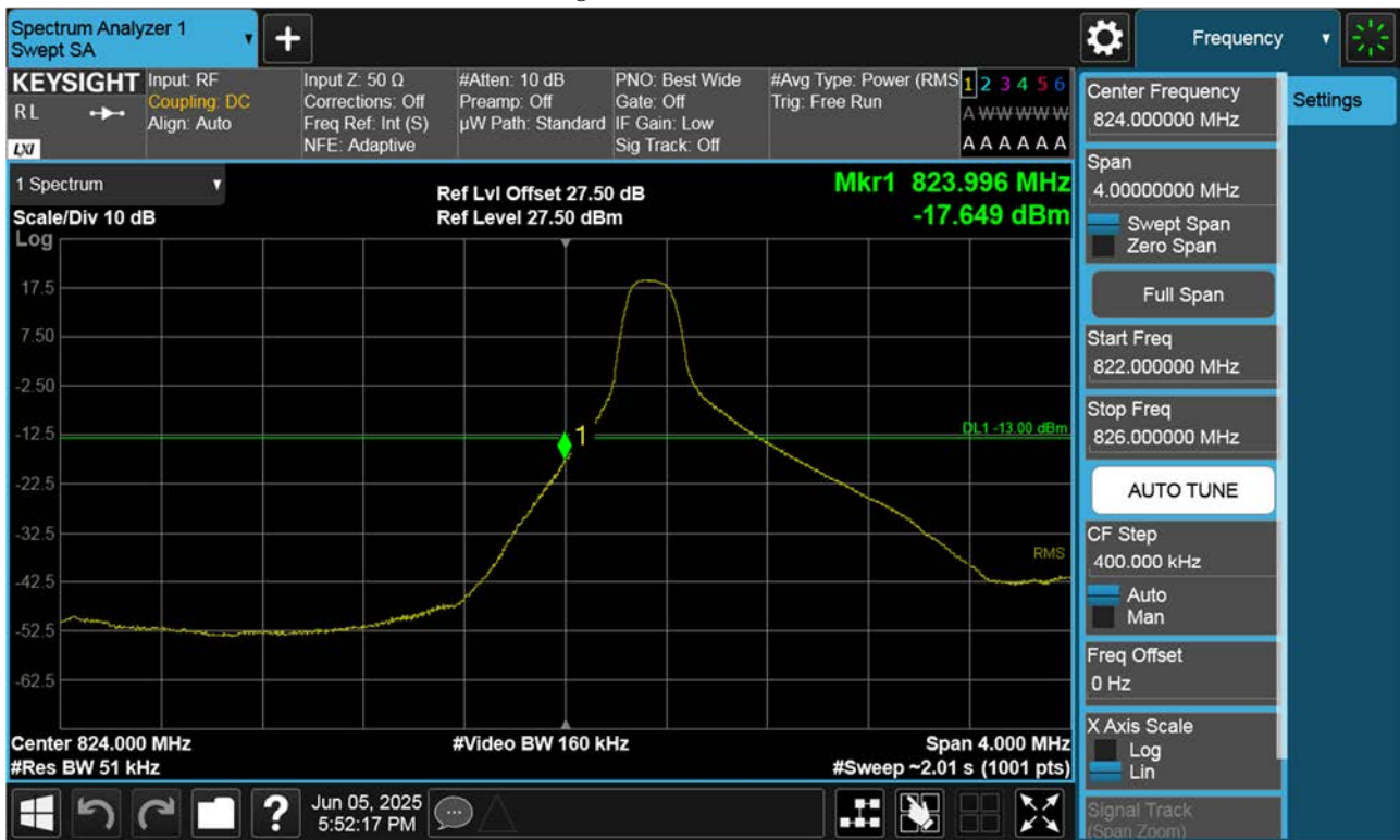
LTE B26_ Lower Band Edge Plot (5 M BW Ch.26815 QPSK_RB1_Offset 0)
