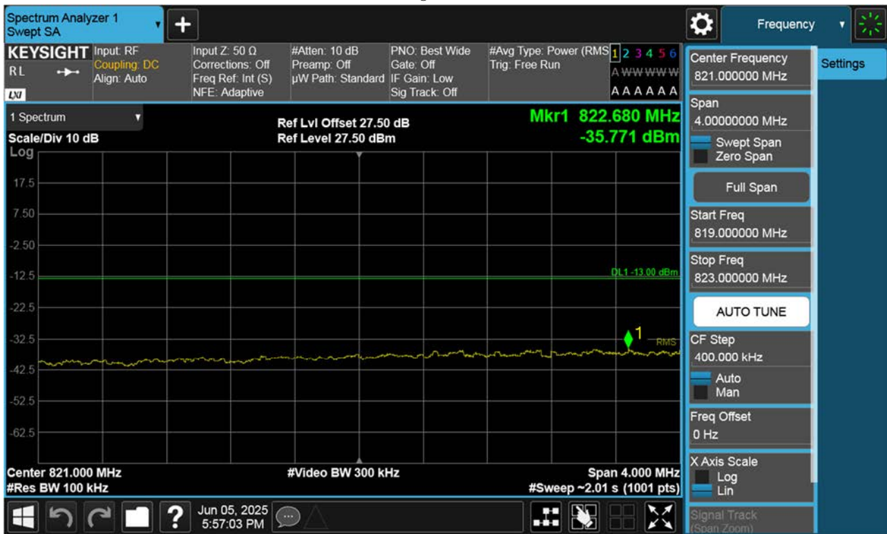
LTE B26_ Lower Extended Band Edge Plot (10 M BW Ch.26840 QPSK_RB50_0)
