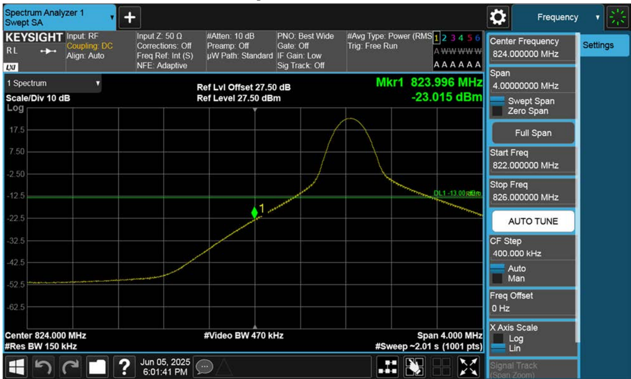
LTE B26_ Lower Band Edge Plot (15 M BW Ch.26865 QPSK_RB1_Offset 0)
