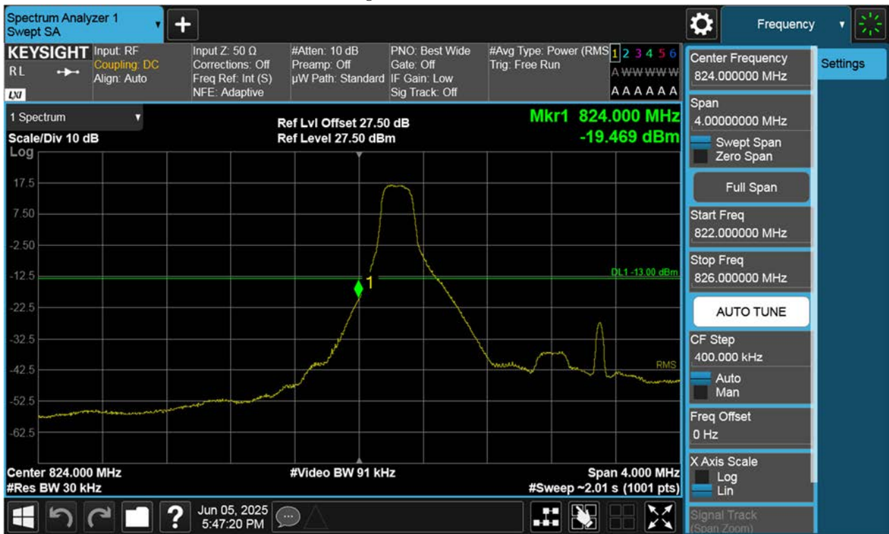
LTE B26_ Lower Band Edge Plot (3 M BW Ch.26805 QPSK_RB1_Offset 0)
