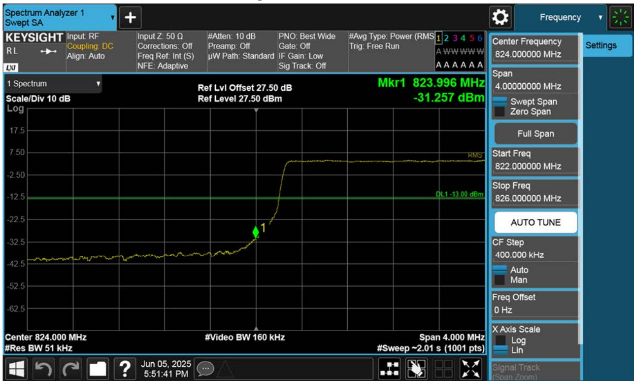
LTE B26_ Lower Band Edge Plot (5 M BW Ch.26815 QPSK_RB25_Offset 0)
