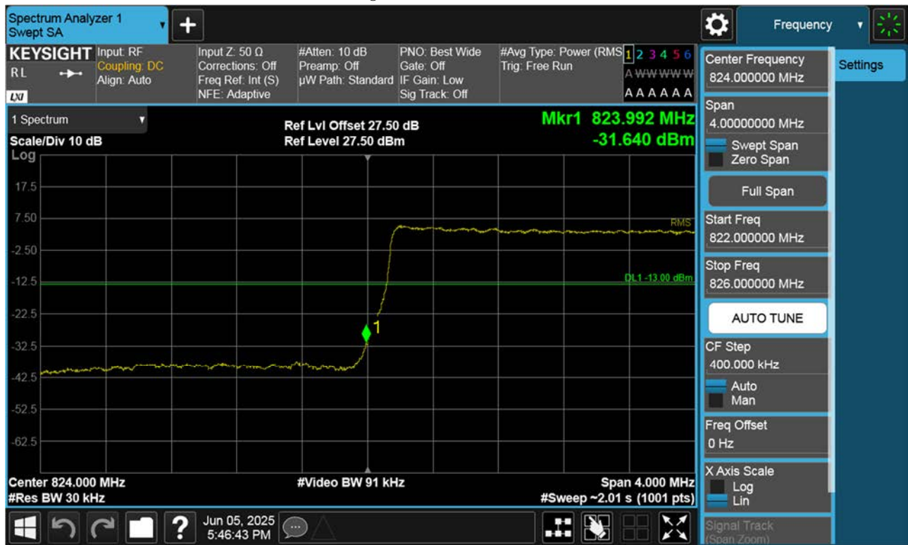
LTE B26_ Lower Band Edge Plot (3 M BW Ch.26805 QPSK_RB15_Offset 0)
