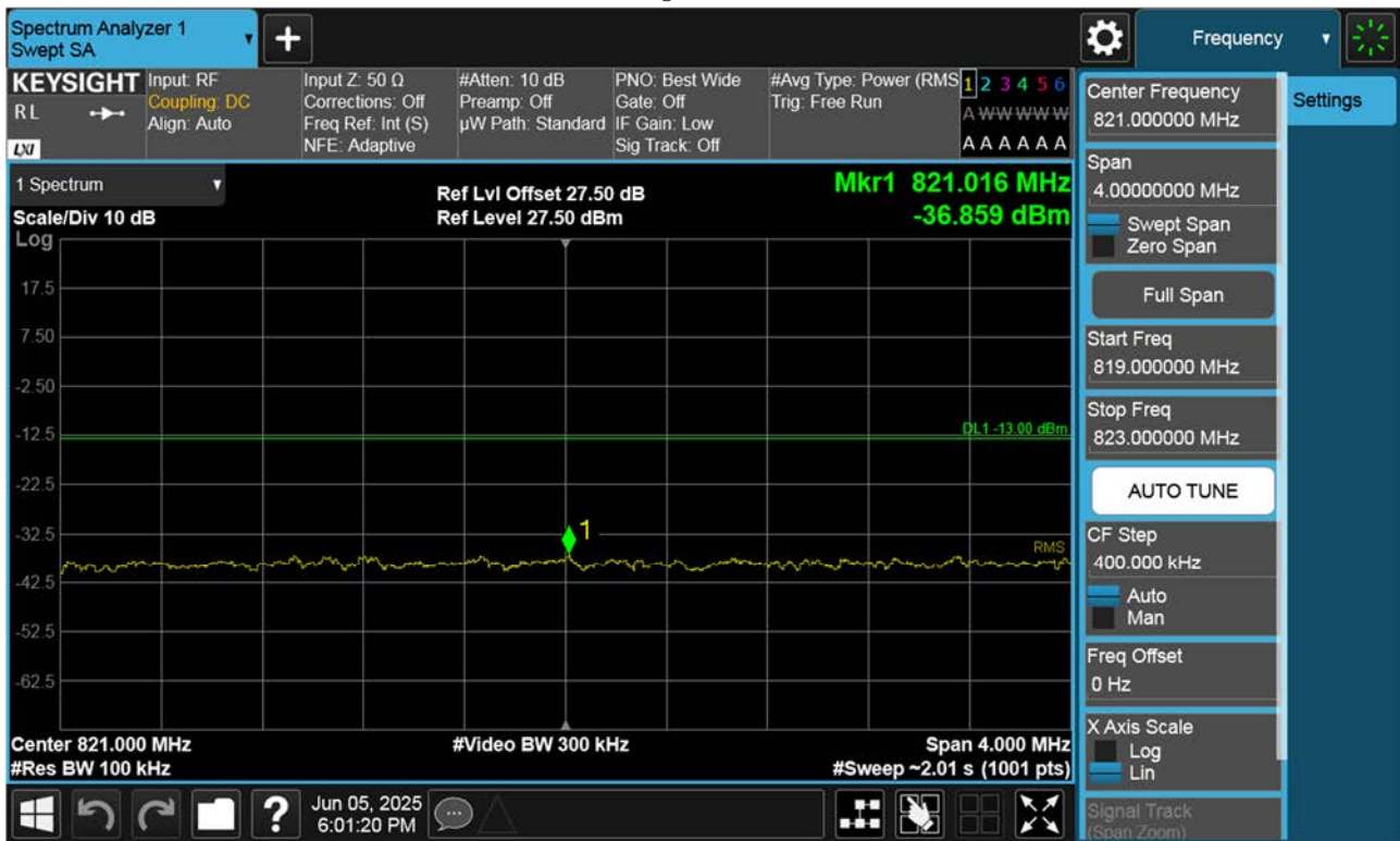
LTE B26_ Lower Extended Band Edge Plot (15 M BW Ch.26865 QPSK_RB75_0)
