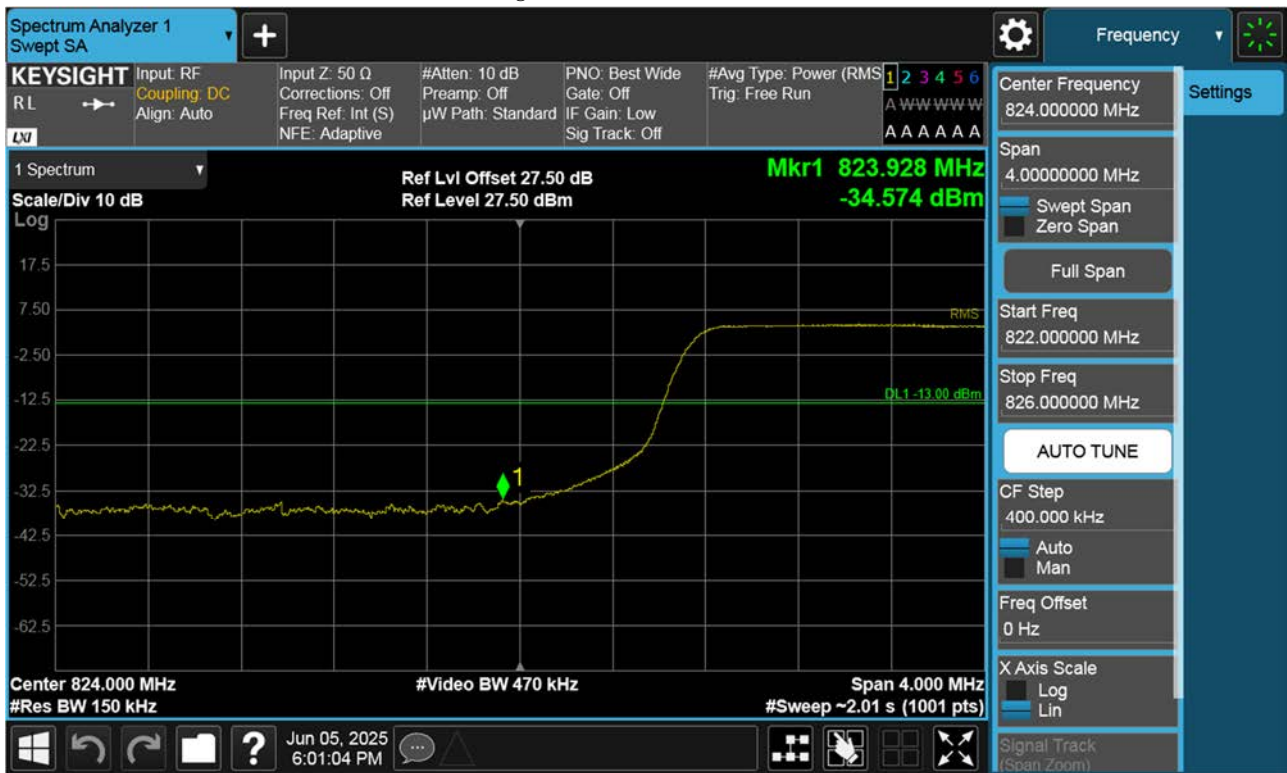
LTE B26_ Lower Band Edge Plot (15 M BW Ch.26865 QPSK_RB75_Offset 0)
