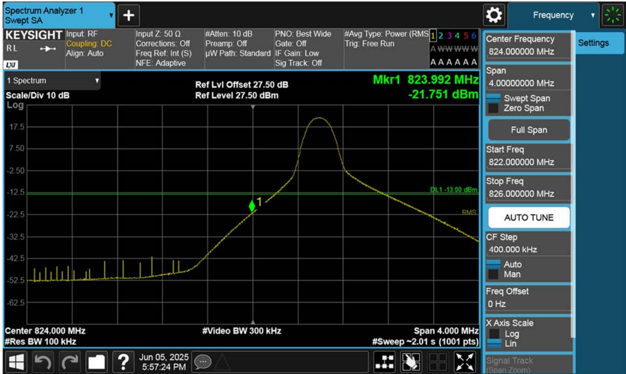
LTE B26_ Lower Band Edge Plot (10 M BW Ch.26840 QPSK_RB1_Offset 0)
